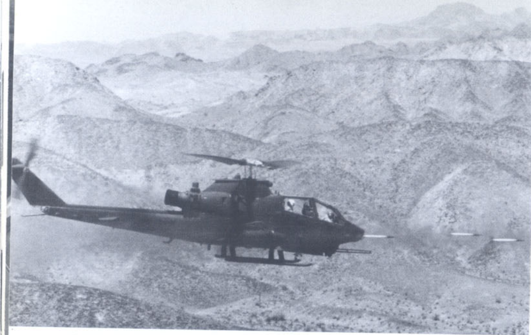
An AH-1F fires 70mm rockets during evaluation of the armament. (Bell)
