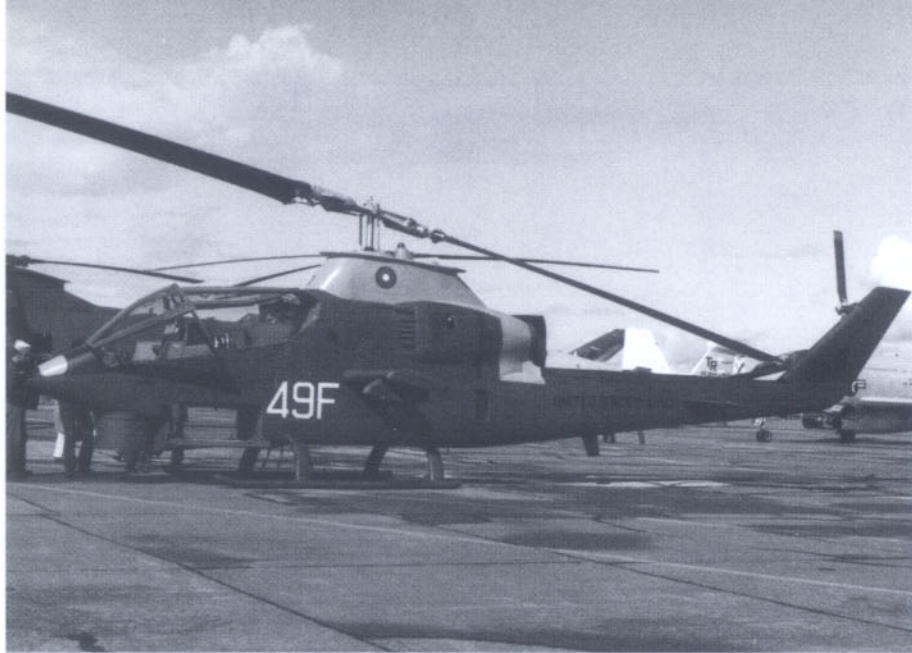
The first production AH-1G (66-15249) served as a TH-1G with the 9th Infantry Division at Ft Lewis, Washington during 1972. The light-colored panels are Orange-Yellow and a divisional emblem appears where the turret barrel openings have been faired over. (AAHS)
