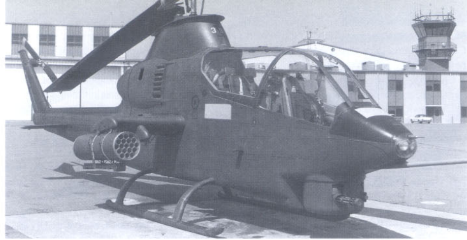
This AH-1G has an XM-18 smoke dispenser attached to the bottom of the rocket pod. Capping the mini-gun is a lead-tipped bullet trap should the weapon be accidentally fired. (Bell)
