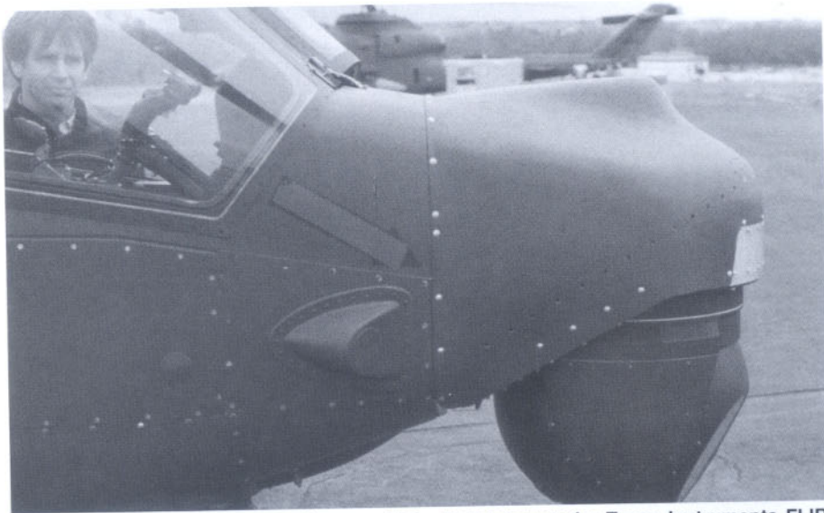
To give the AH-1W night targeting capability, Bell integrated a Texas Instruments FLIR into the nose of an AH-1T (159228) during the early 1980s. Called the "Viper", the sight system never went beyond the research stage. (Bell)
