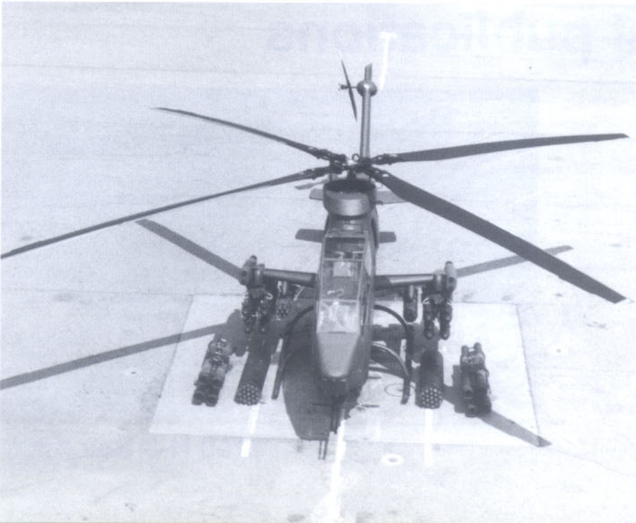
Included among the wide variety of weapons systems evaluated on the Model 249 was the Hellfire missile, initially developed for the Army's Apache. (Bell)
