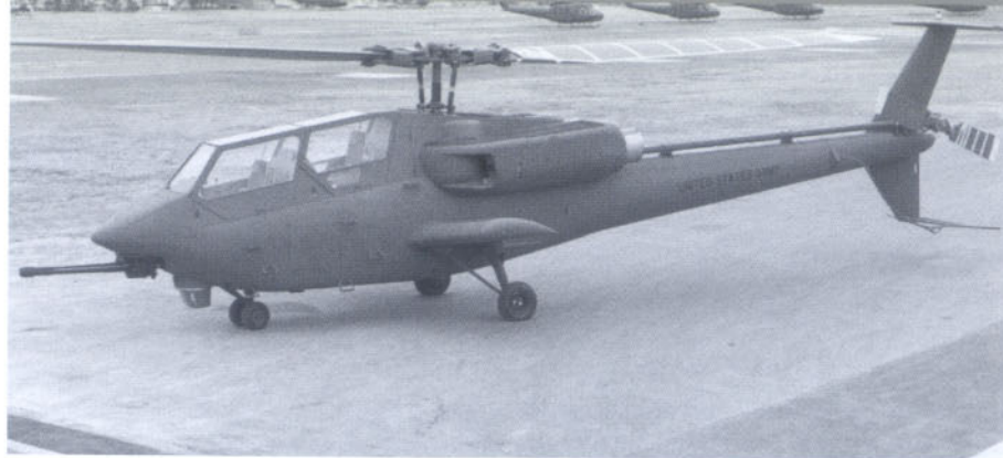
Bell's entry in the Army's AAH competition, held during the 1970s, was the YAH-63. Intended as the Cobra's eventual replacement, the YAH-63 featured a distinctive T-tail. (Bell)
