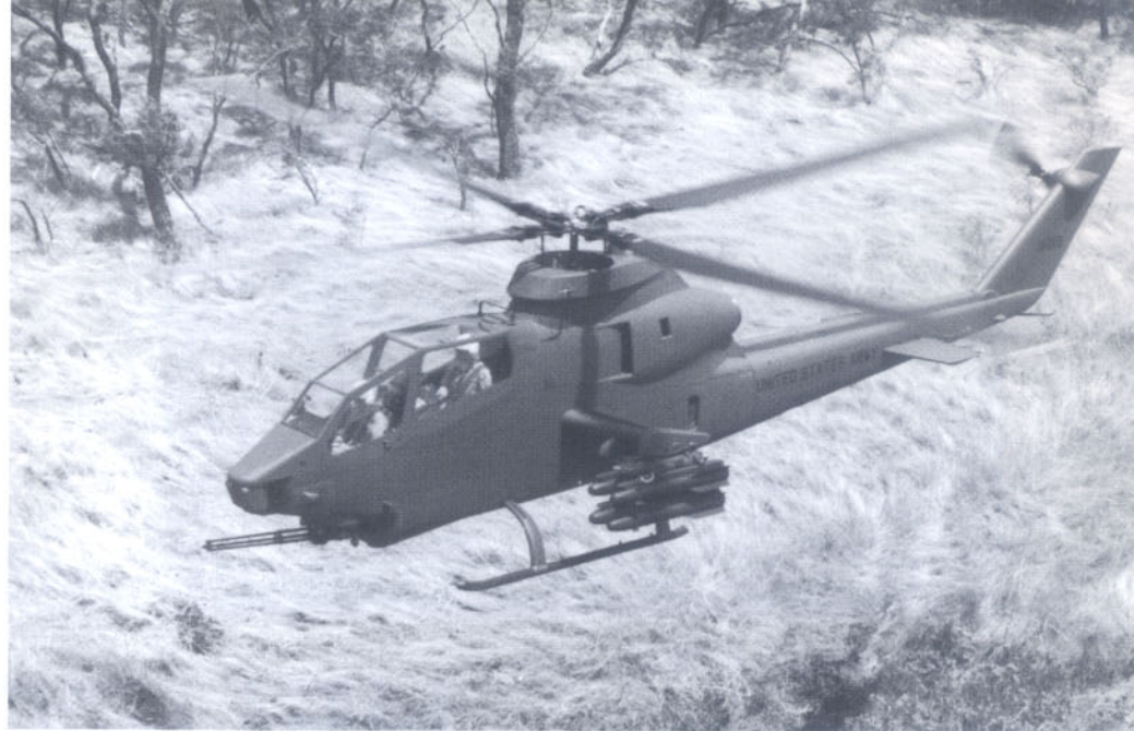
Bell's Model 249, also called the Cobra 2000, flew with the four-blade 412 rotor system. (Bell)
