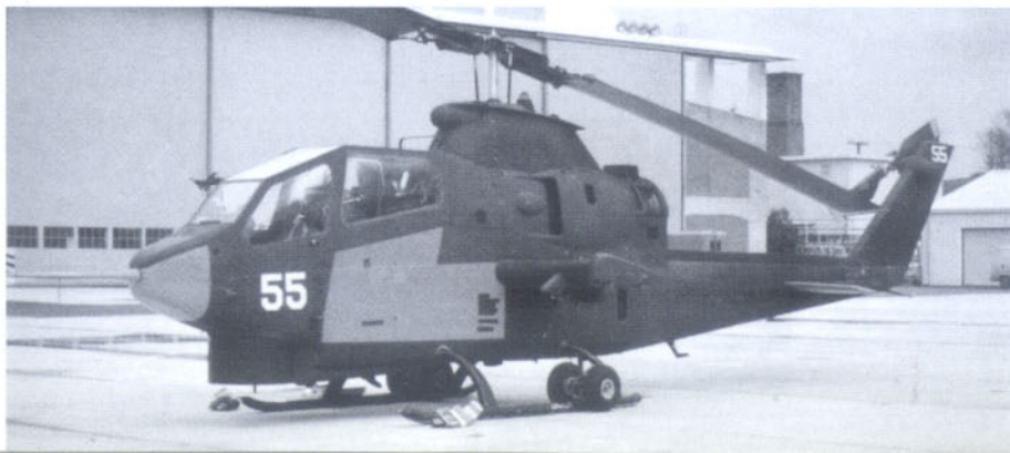
(Left) A TAH-1F during late 1983. Ballast replaced the turret weapons and International Orange was applied on the nose, fuselage and elevators. (Ted Paskowski via Terry Love)
