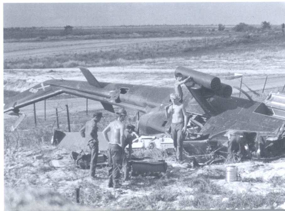
This was one of approximately 200 Cobras lost during combat action in Vietnam. The 1st Cavalry Cobra crashed during its attempt to land at its home base Lai Khe, after enemy gunners scored hits on the aircraft's fuel cell. (Mike Sloniker)
