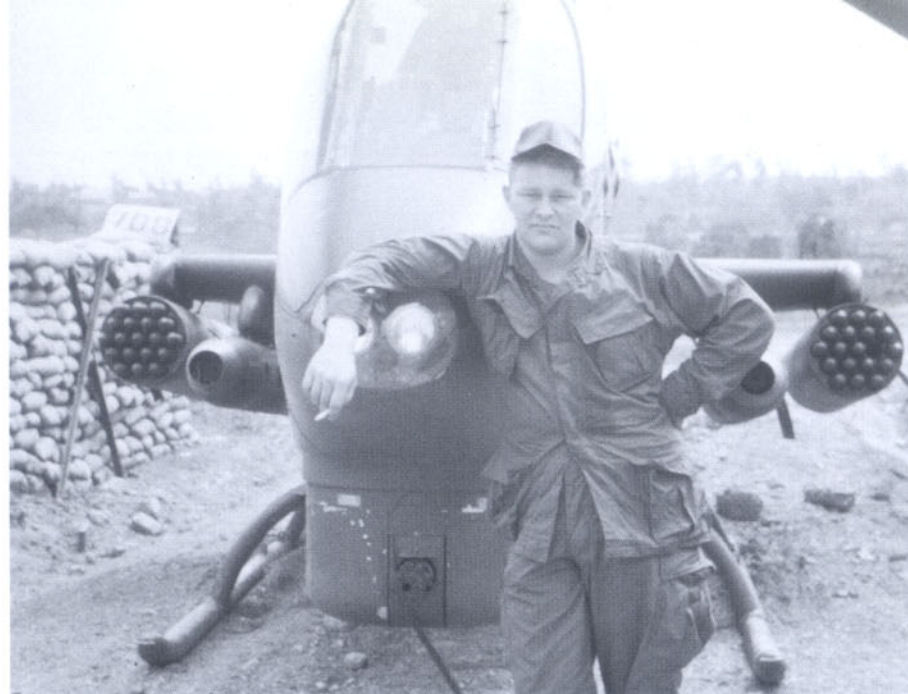
A crew chief poses with his AH-1G, distinguished as an early model by the nose landing lights and single-weapon turret. Inboard of the "Hog" rocket pods are XM-18 podded mini-guns, which crews found much more reliable than the turret minigun. (Ron Osburn)
