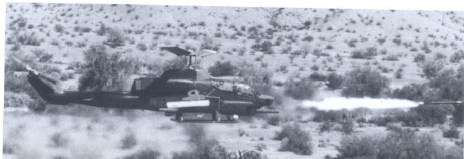
An early AH-1W fires 5 inch rockets during tests. Cameras were mounted on the forward skids to record the evaluations. (Bell)
