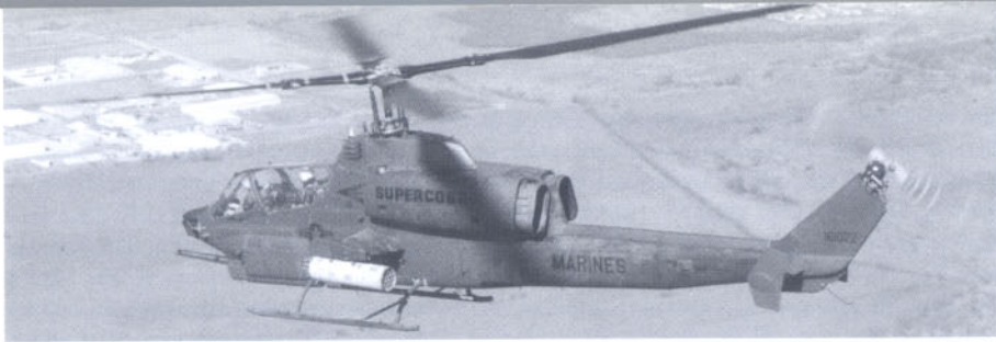
One of the first flights with Bell's Advanced 680 four bladed rotor system during early 1989. A 19 shot rocket pod occupies the outboard wing station. The "VX5" on the forward tail boom denotes assignment to Air Test and Evaluation Squadron Five. (Bell)
