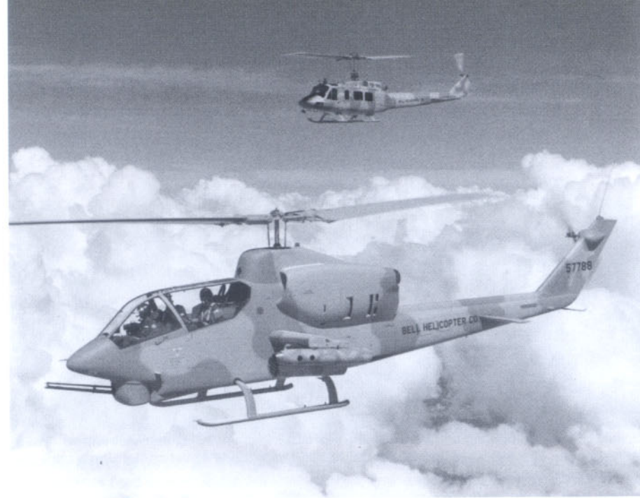
Wearing a two-tone sand camouflage, Bureau Number 157788 was a Bell demonstrator from the first production batch of AH-1Js. Accompanying the SeaCobra on its test flight is a Bell Model 214. (Bell)
