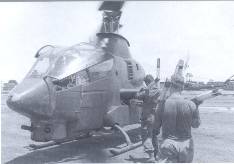
Ground crewmen making a "Hot" re-arm (rotors turning) on a Cobra in Vietnam with 2.75-inch rockets. The AH-1G is armed with an XM-35 cannon and turret containing a mini-gun and grenade launcher. (Bell)
