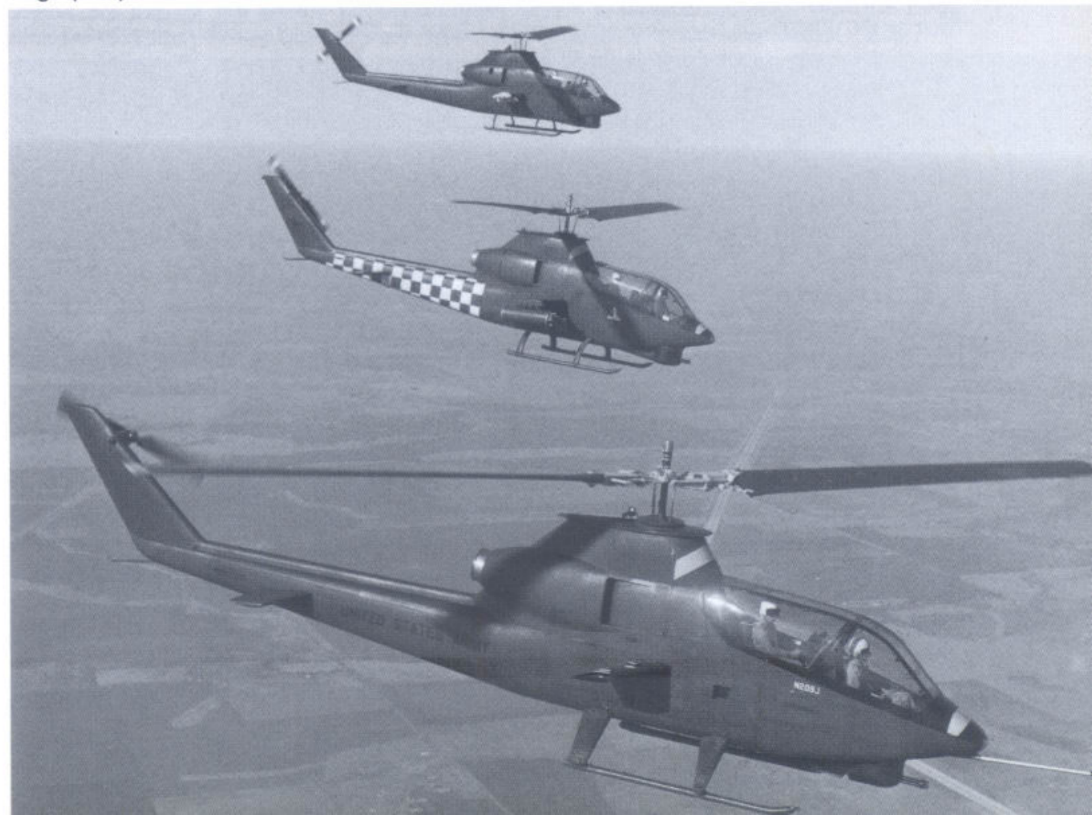
The first three Cobras. The original Model 209 (foreground) is accompanied by the first two prototypes. The tail boom of Serial Number 66-15246 was checked for camera tracking. (Bell)
