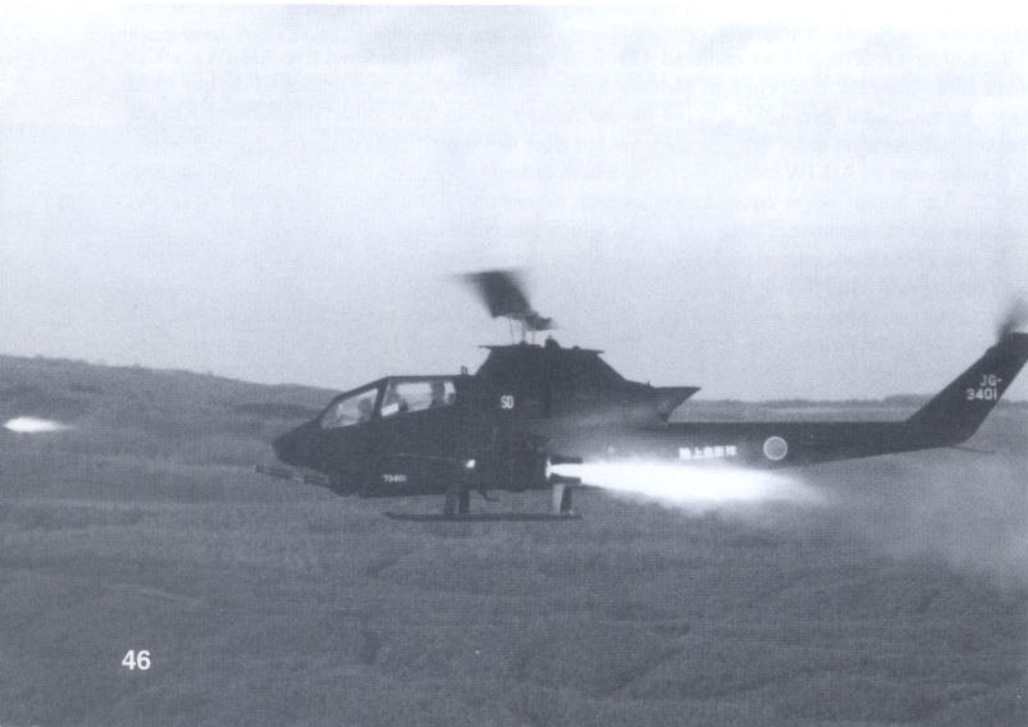
The first AH-1S(TOW) built under license by Fuji fires 2.75-inch rockets from a launcher mounted inboard of the TOW launcher. (Bell)
