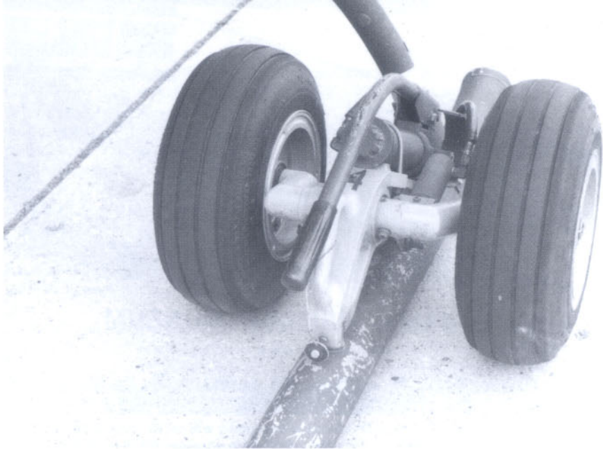
Standard on all Cobra models were attachment points atop the skids for installation of ground handling wheels. (Author)
