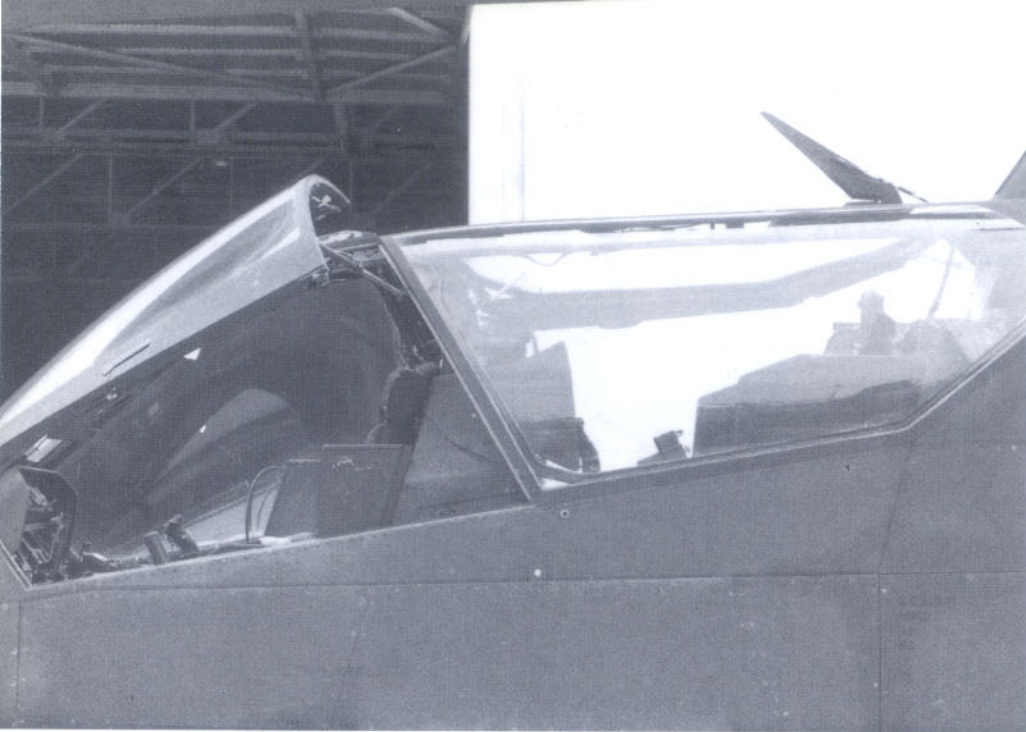
Mounted atop the AH-1S canopy was a wire-cutting blade, part of a kit deemed necessary in view of the helicopter's low level environment. The gunner's armored seat panels were significantly smaller than those of the pilot. (Author)
