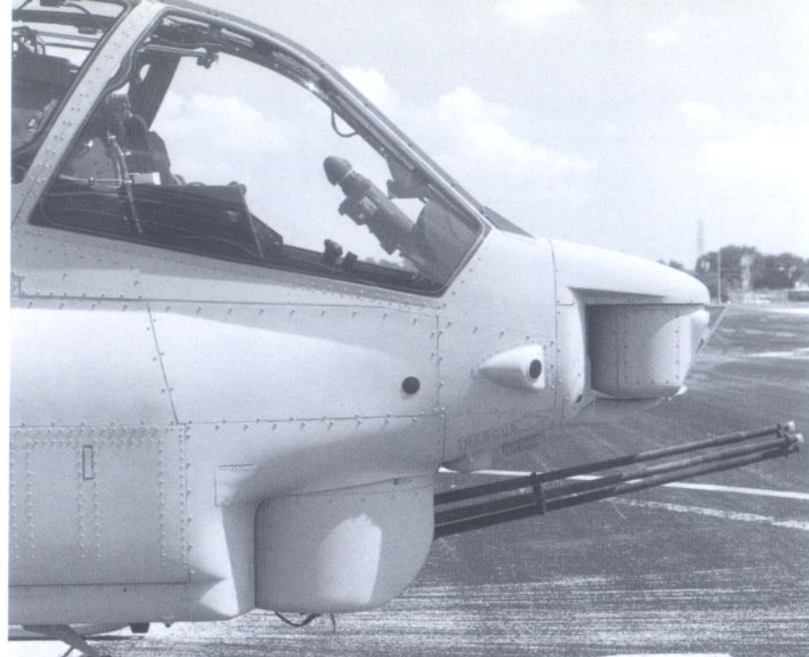
One of four E-Systems AN/APR-39 radar warning antennas (above the rescue arrow) that was installed on later Cobras. (Bell)
