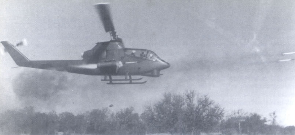
An early AH-1G fires 2.75-inch rockets. The breakaway nose fairing can be seen tearing away from the launcher. (Bell)
