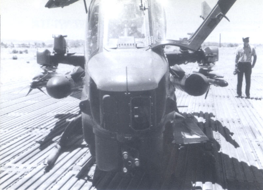
The AH-1W retained the original Cobra's curved canopy. The prototype is seen carrying Sidarm missiles mounted to the outboard stations. (Bell)
