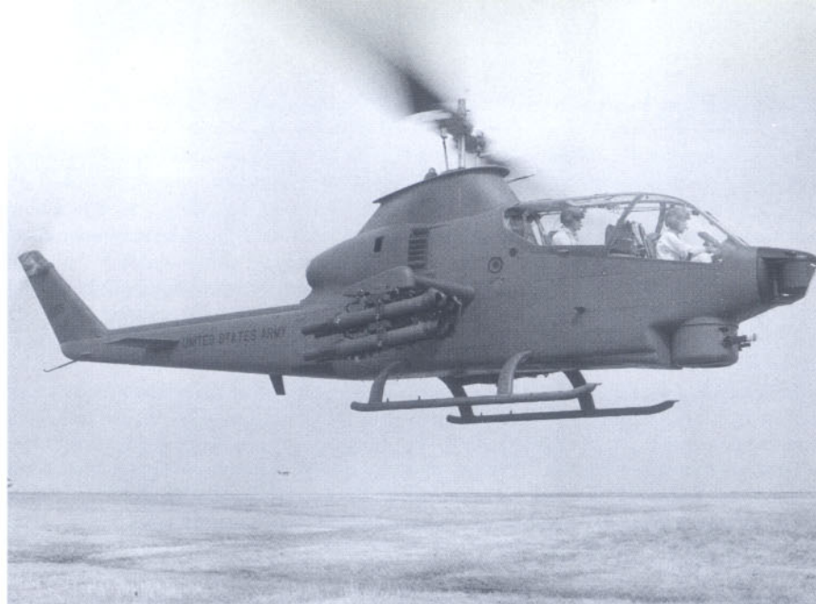
The AH-1Q, derived basically from an integration of TOW with the AH-1G, was the first deviation from the original Huey Cobra. The TOW system's Telescopic Sighting Unit (TSU) installation required that the pitot tube be relocated to the rotor pylon. Serial number 70-16055 was the first AH-1G converted to "Q" standards. (Bell)
