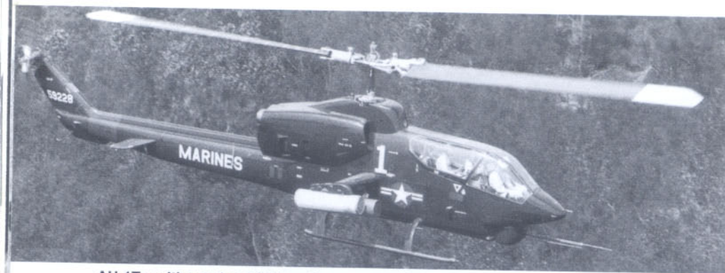
AH-1Ts without the TOW system were called "Slicks." The 33 acquired by the Marine Corps were later fitted with M65 TOW systems. This, the first AH-1T (which was actually the second to the last AH-1J produced) evaluates a "heavy" armament load of 76 rockets. (Bell)
