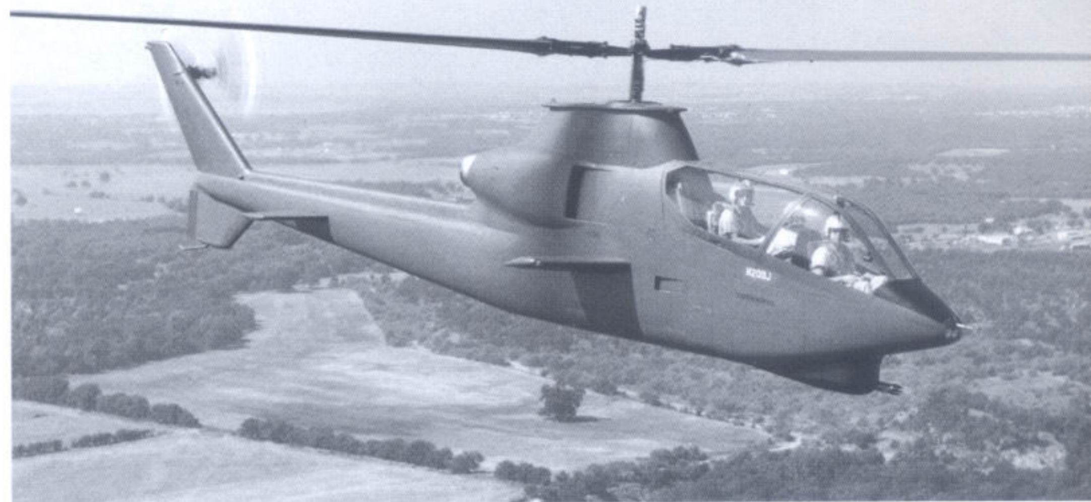
The original Model 209 featured retractable landing gear and a ventral fin, both of which were later deemed unnecessary and deleted from successive models. (Bell)
