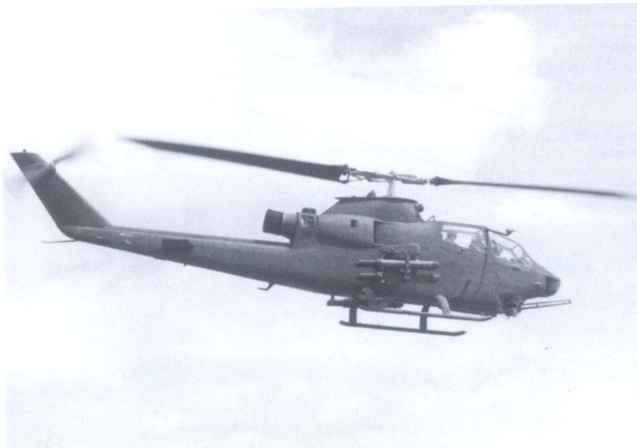
An AH-1F armed with TOW missiles. The omni directional airspeed system extending from the cockpit frame provides input for cannon and rocket accuracy. (Bell)
