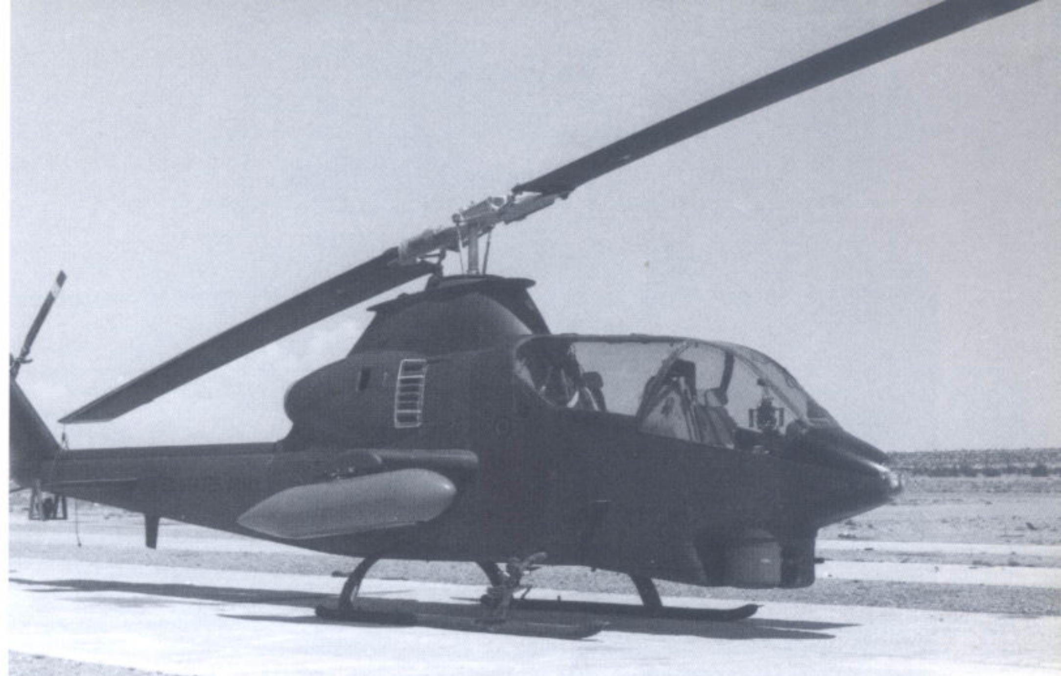
Cameras are mounted to the sixth-built AH-1G during armament tests. The 19-shot rocket pod has fore and aft fairings which were rarely in place during operational use. (Bell)
