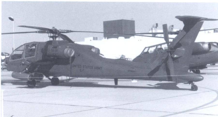
The Army Cobra's replacement during the AAH competition; the Army assigned both YAH-64 prototypes serial numbers consecutive with those of the YAH-63s. Alongside is Bell's competitor during evaluation of both types. (MAP)
