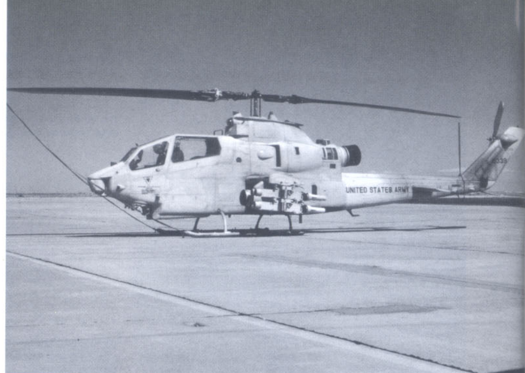
This sand colored AH-1F began life as an AH-1G. The teardrop fairing just forward of the engine intake houses fire control system components. (via Terry Love)
