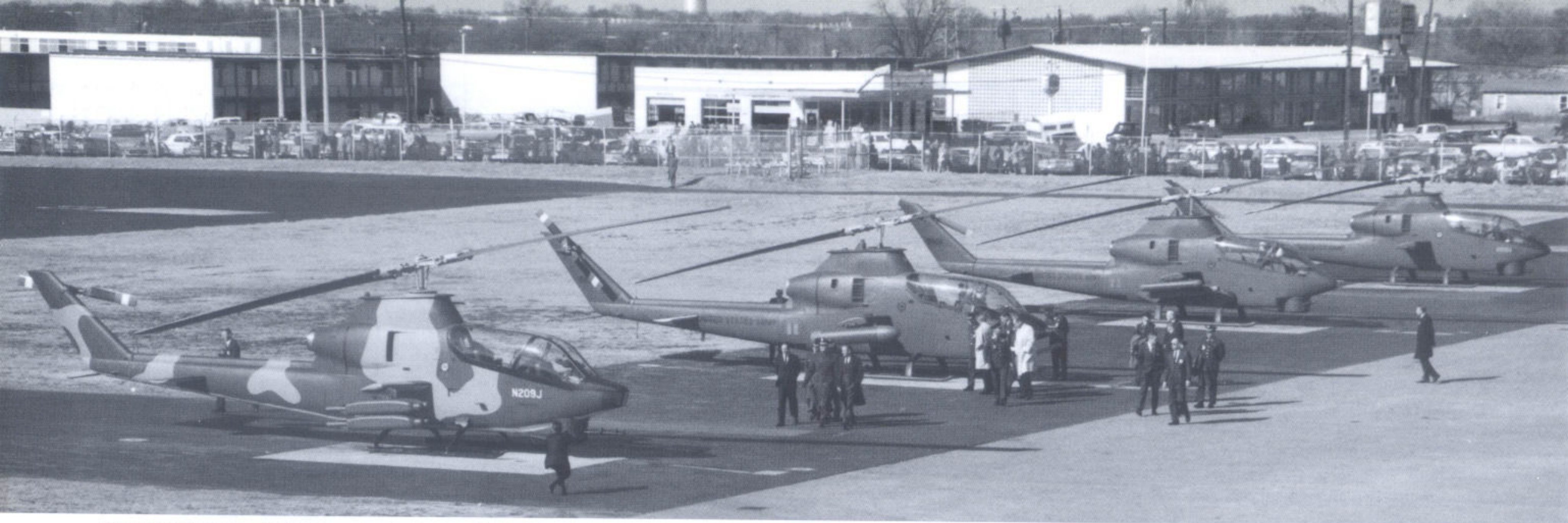
The second prototype (66-15247), armed with a single mini-gun in the turret, undergoes armament tests at Ft Hood during 1967. Red bands were painted on the nose and rotor pylon. (Ron Osburn)
