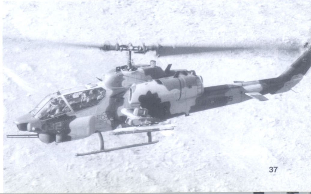
A Sidarm missile equipped AH-1W. The chaff/flare dispenser cartridge has been removed from the launcher on the wing. (Bell)
