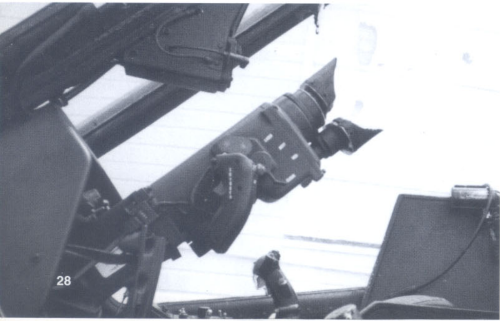
The AH-1S gunner's TOW sighting unit. "Armchair" flight controls are visible along with a cockpit light attached to the armored seat side panel. (Keith Lovern)
