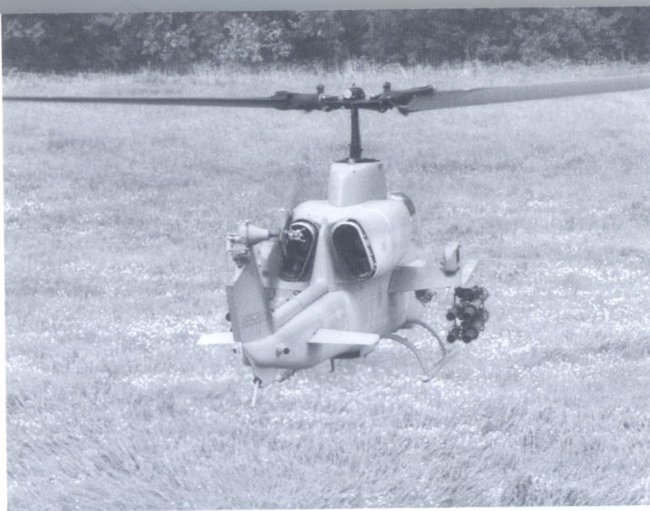
The AH-1W's offset trailing edge of the vertical fin combined with the cambered tail to offset torque induced yaw. (Bell)
