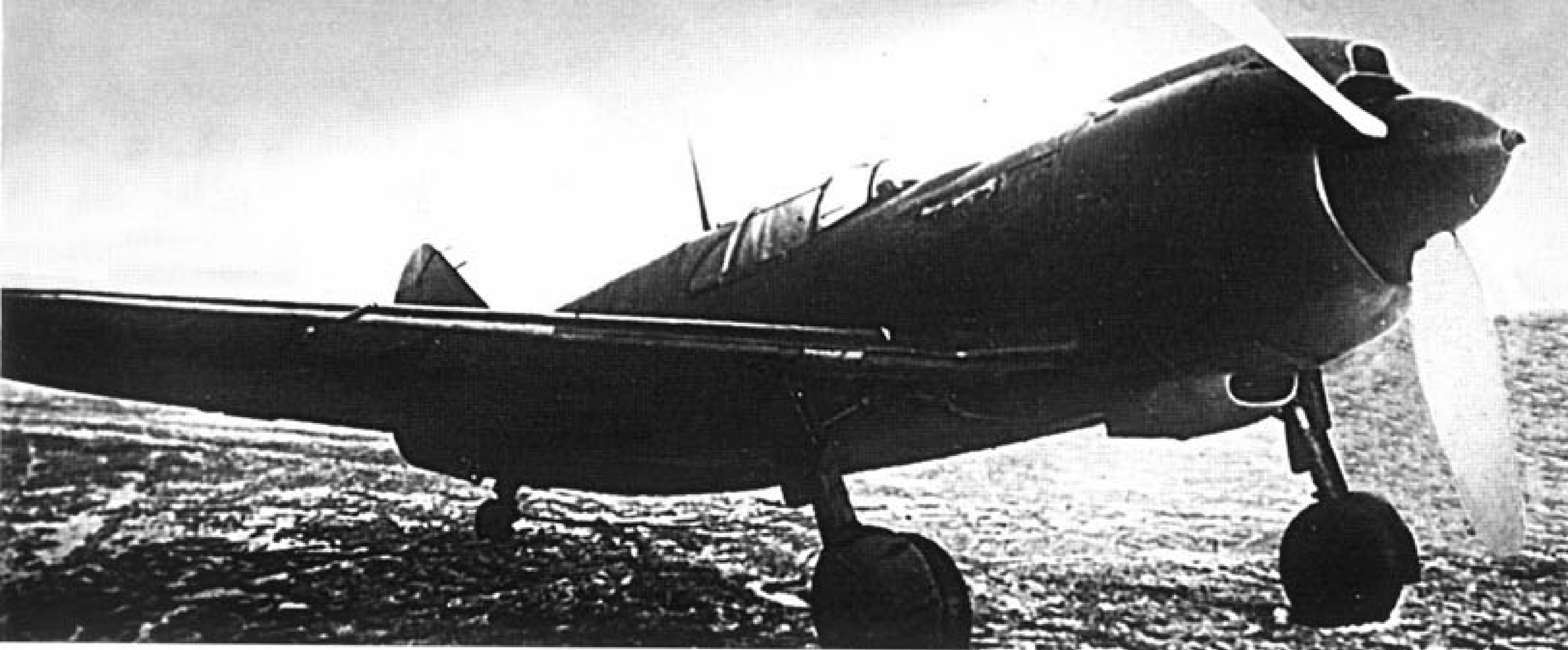
This early production La-5 has a supercharger air intake and trunking similar to the later La-5FN. The aircraft is equipped with an aft sliding canopy similar to that of the LaGG-3 (66th Series), but has the windscreen of the early LaGG-3 versions. (Ivan Ivanov)
