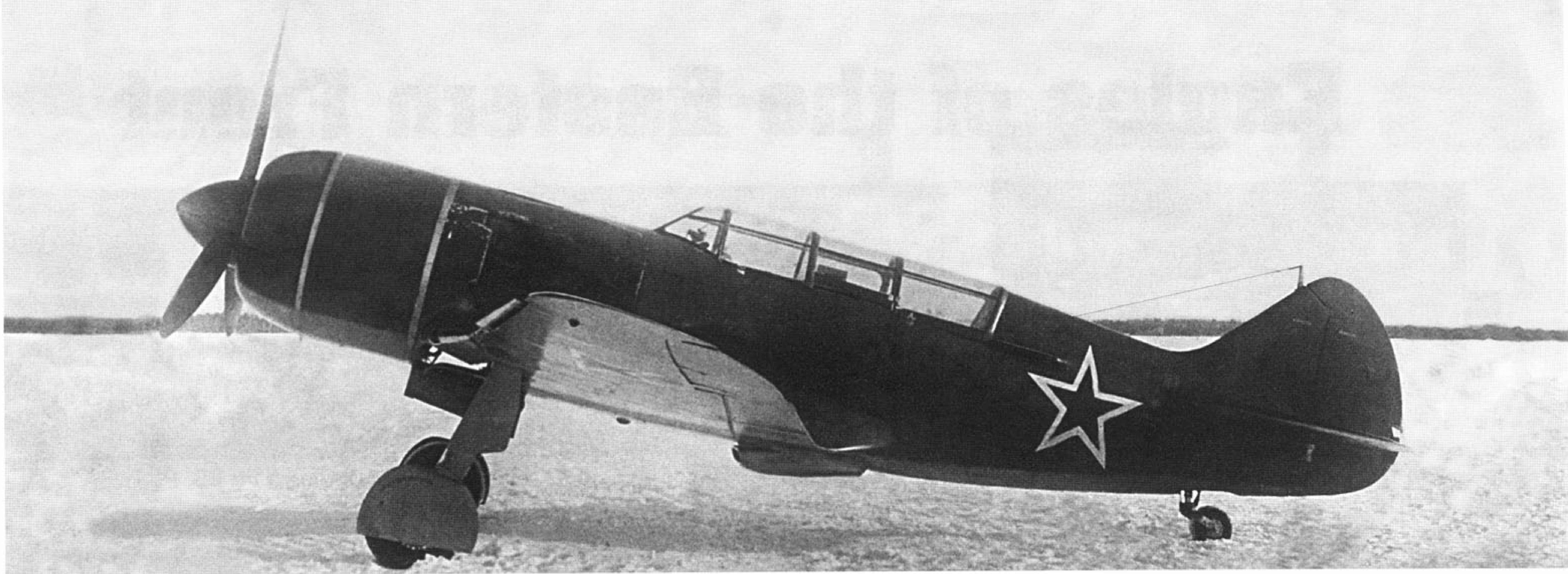
(Above) The La-7UTI had an additional instructor cockpit. The aircraft lacked an antenna mast. The tail wheel was locked down and the tail wheel doors were deleted. The Soviet national marking was only applied to the rear fuselage and wing under surfaces. The silver bands on the nose are metal straps used to hold the cowling together. They were often left unpainted. (Ivan Ivanov)
