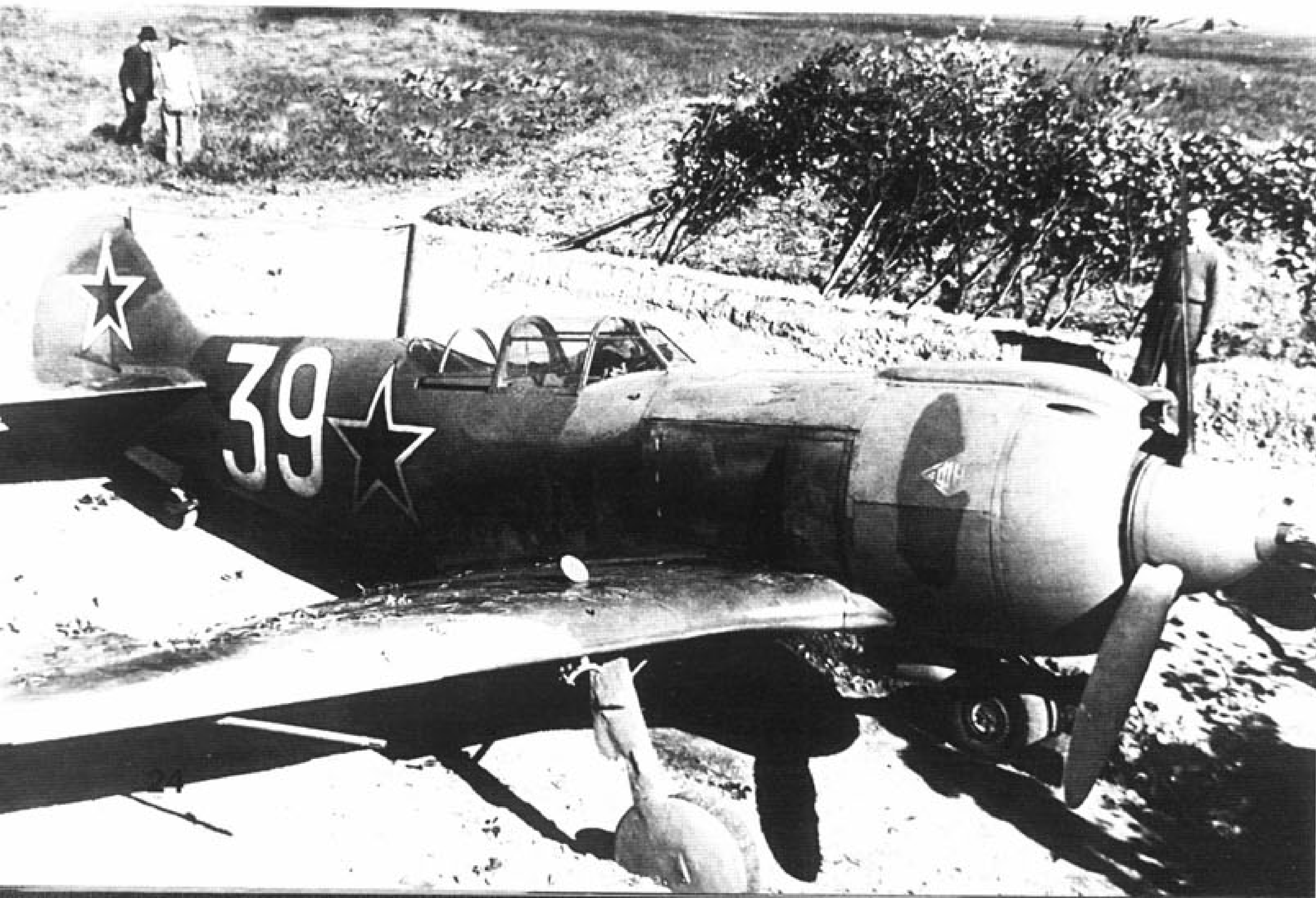
(Below) This La-5FN (white 39) is being readied for a mission while parked on Polish airstrip. The fuel tank cap on the upper wing surface is open and the cut trees used to camouflage the aircraft have been laid to one side. This is a late production La-5FN with the wire leading into the port side of the aft canopy glazing. The fighter is also equipped with the D3-40 bomb racks. (Andrzej Morgala)
