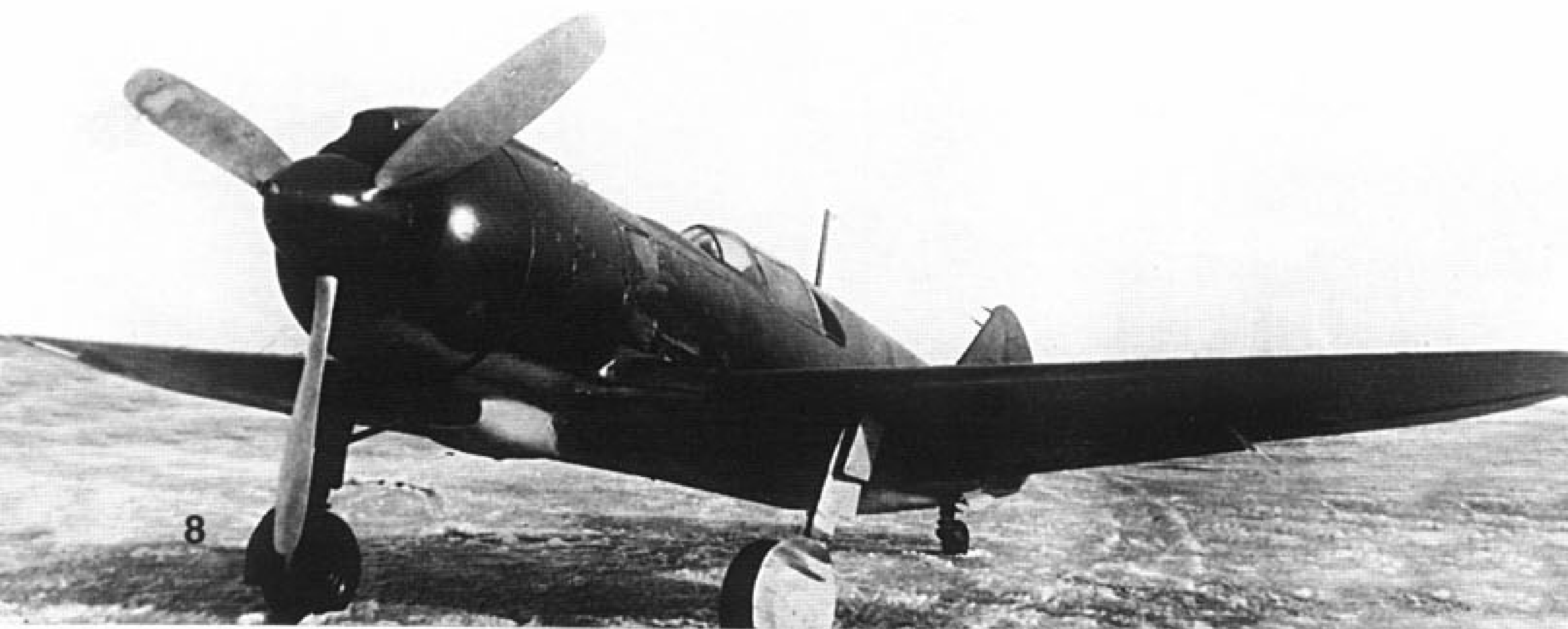
The early production La-5 featured an additional door above the main strut cover. This door was deleted on production La-5s. The aerial stub on the tail is also missing and both antenna cables lead directly into the vertical fin's leading edge. (Ivan Ivanov)
