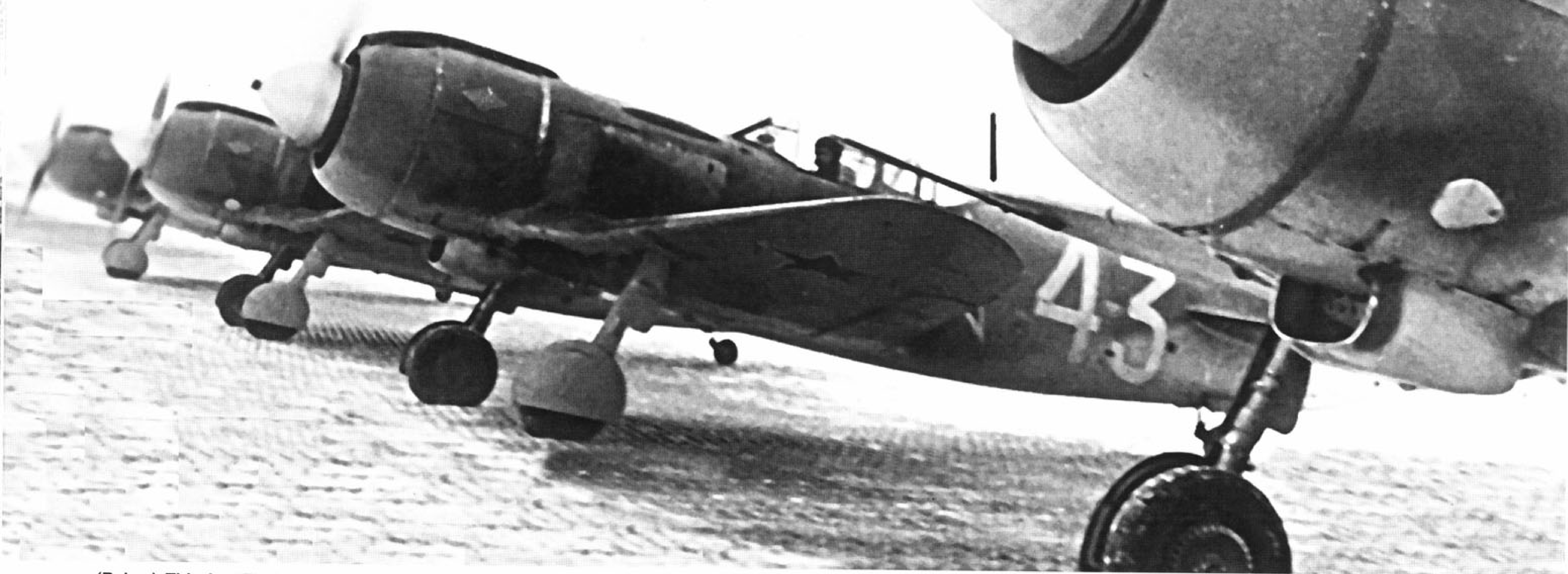
(Above) Late production La-5FNs were fitted with an additional, semi-circular access hatch in the lower cowl. All of these aircraft have yellow spinners and rudders. (Ivan Ivanov)
