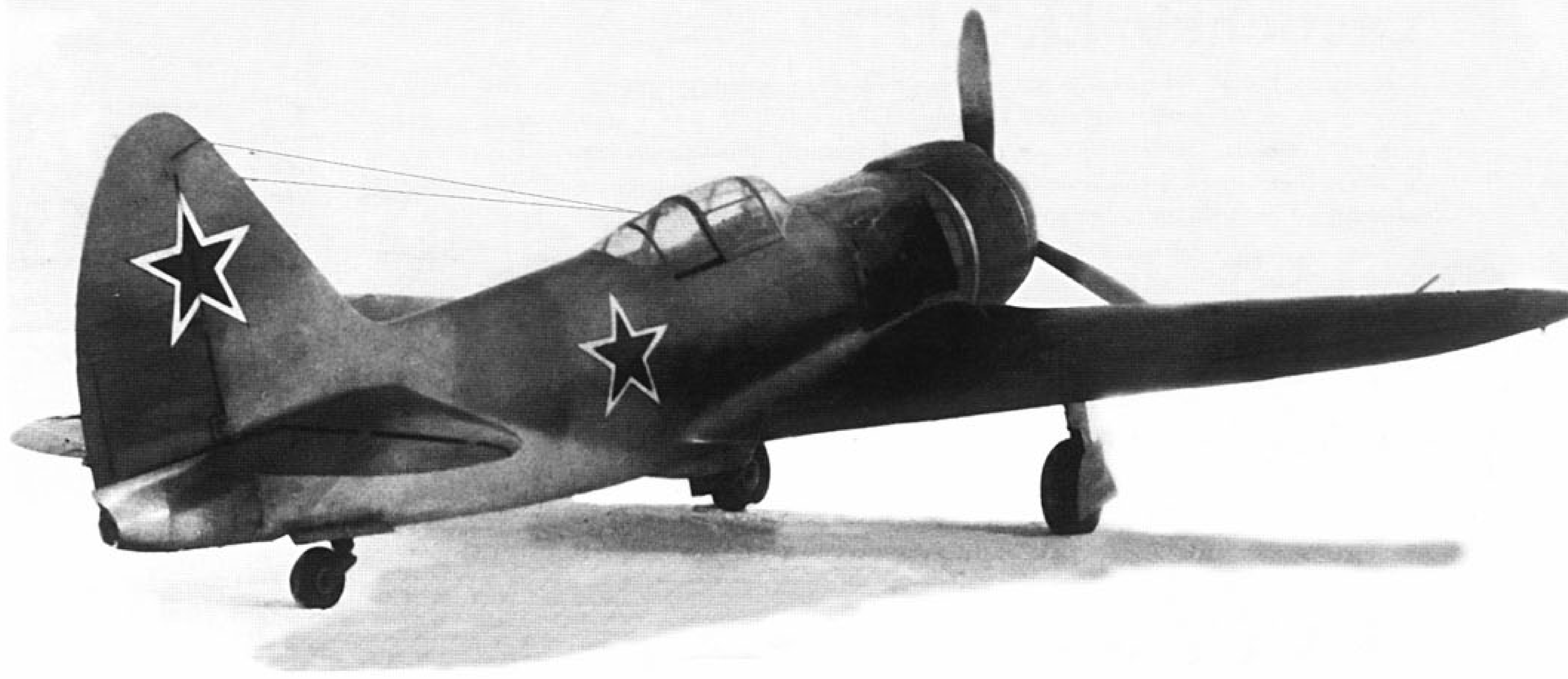
The La-7R had an enlarged tail and lacked the fuselage antenna mast and the vertical fin aerial stub. The RD-1KhZ rocket engine was mounted in the tail adjacent to the fifteenth fuselage bulkhead. (Ivan Ivanov)
