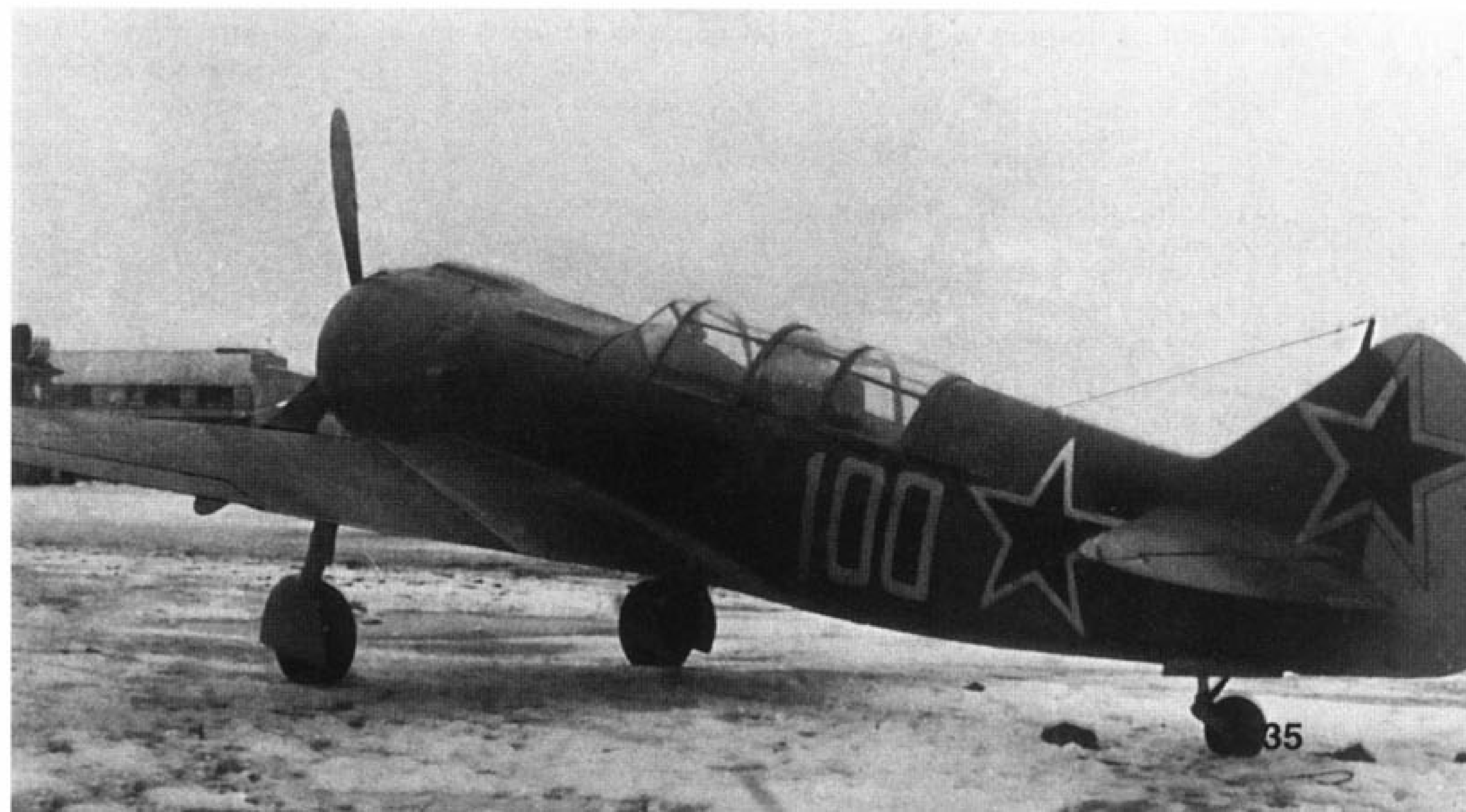
This La-5UTI (white 100) was converted from a single-seat fighter by the 1st Air Depot at Leningrad. The slanted cross frame in the windscreen indicates the aircraft was an La-5 powered by an ASh-82A engine. This trainer has been equipped with a radio system. (Ivan Ivanov)
