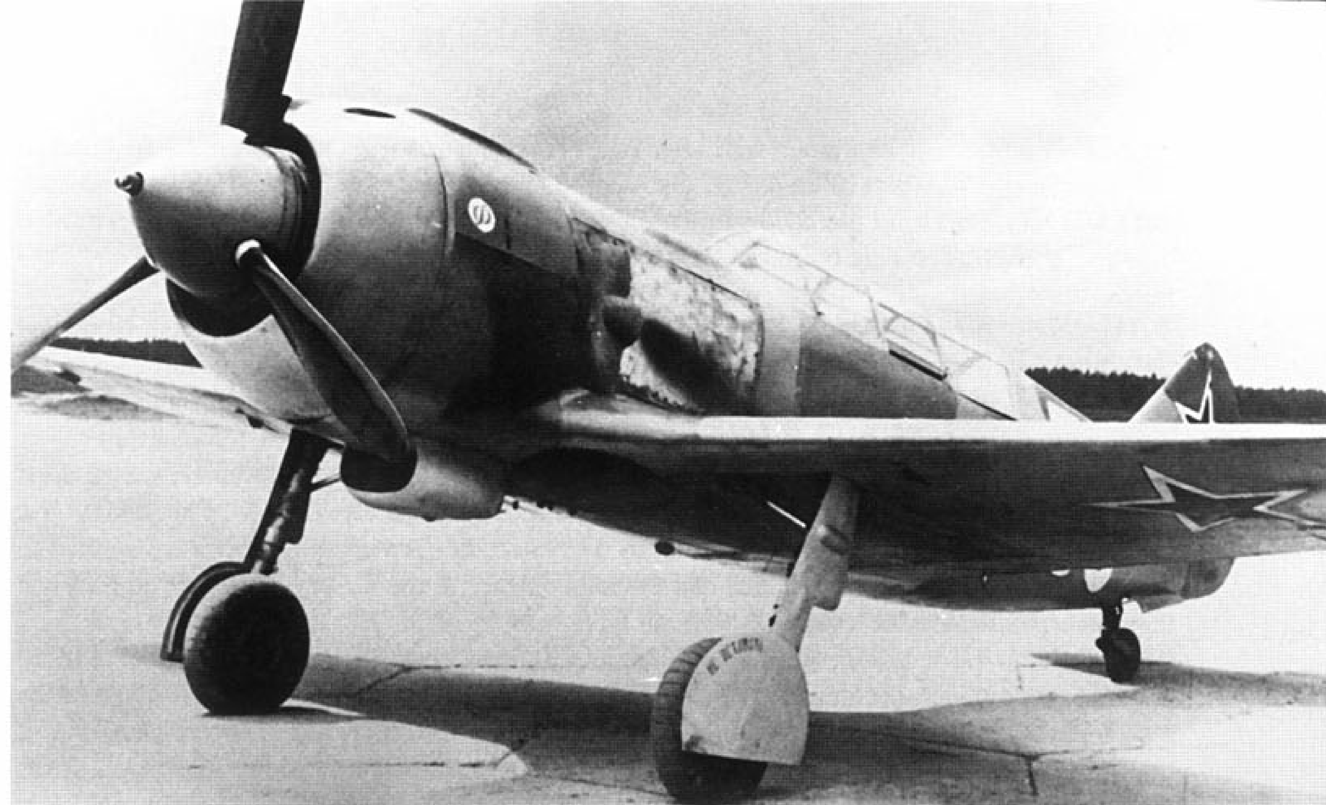
The early La-5UTIs were powered by an ASh-82F engine. These early trainers lacked radio systems and were equipped with a squared off rear canopy over the instructor. (Ivan Ivanov)
