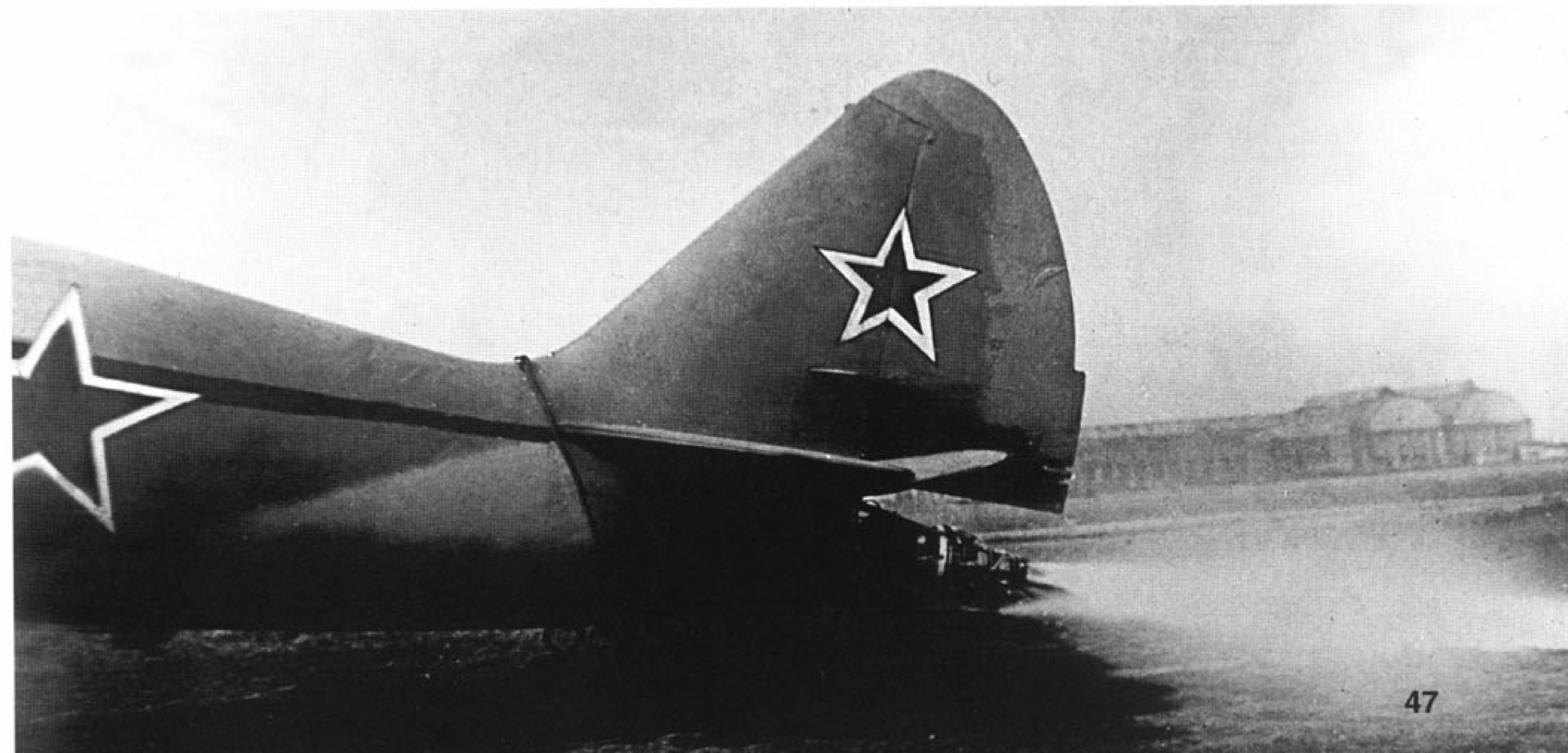
The RD-1KhZ rocket engine was powered by a 90 liter (23.7 gal) kerosene tank and a 180 liter (47.5 gal) nitric acid tank mounted in the fuselage. The engine had a burn duration of 3.5 minutes. Special pumps driven by the ASh-82FN radial engine supplied the fuel to the rocket motor. (Ivan Ivanov)
