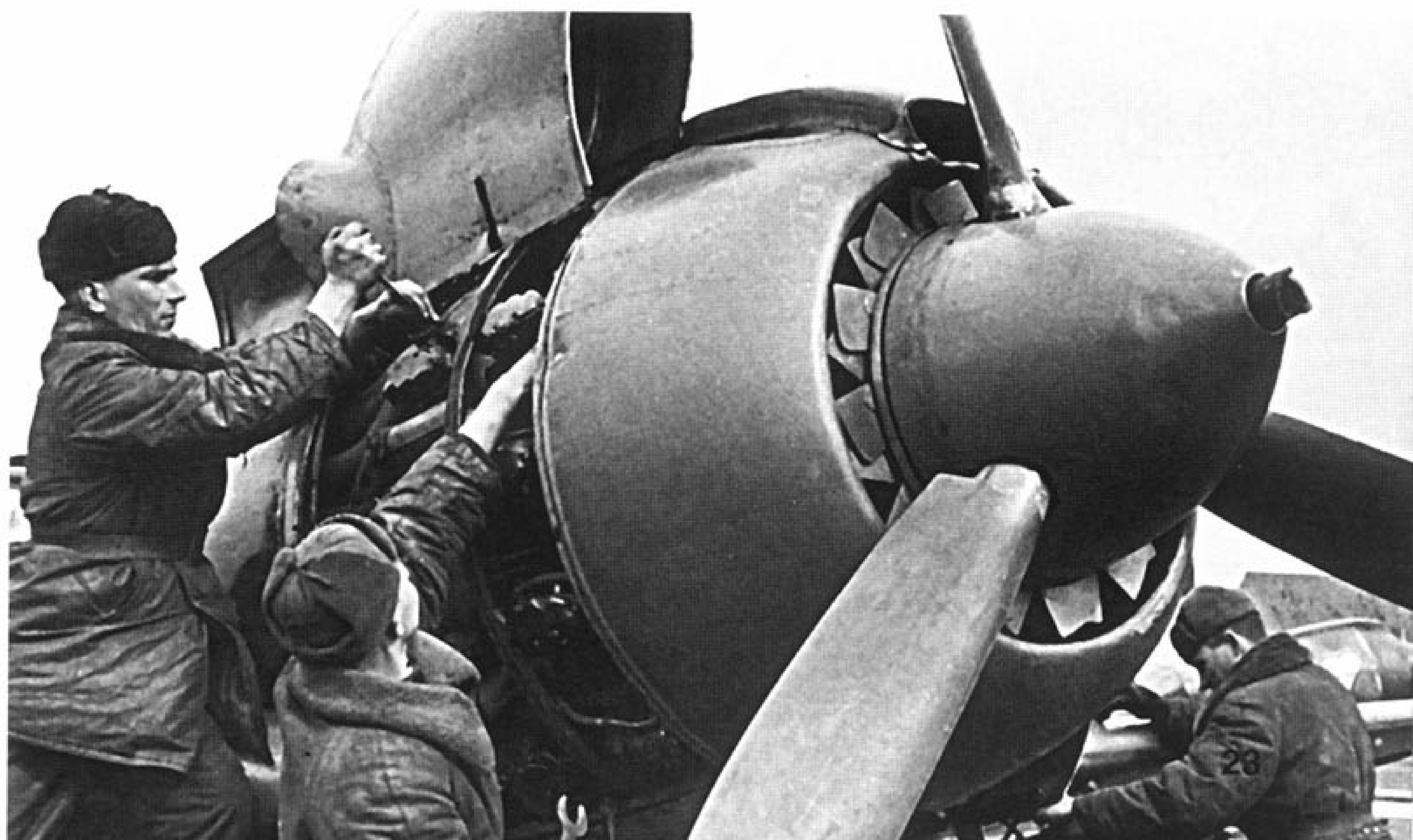
A late production La-5FN of the 41st Guards Fighter Aviation Regiment, 5th Air Army is readied for a mission during early 1945. The ASh-82FN engine was closely cowled. The vanes behind the spinner were variable to permit additional cooling air into the cowl. The Hucks type start dog protrudes through the spinner. (Ivan Ivanov)
