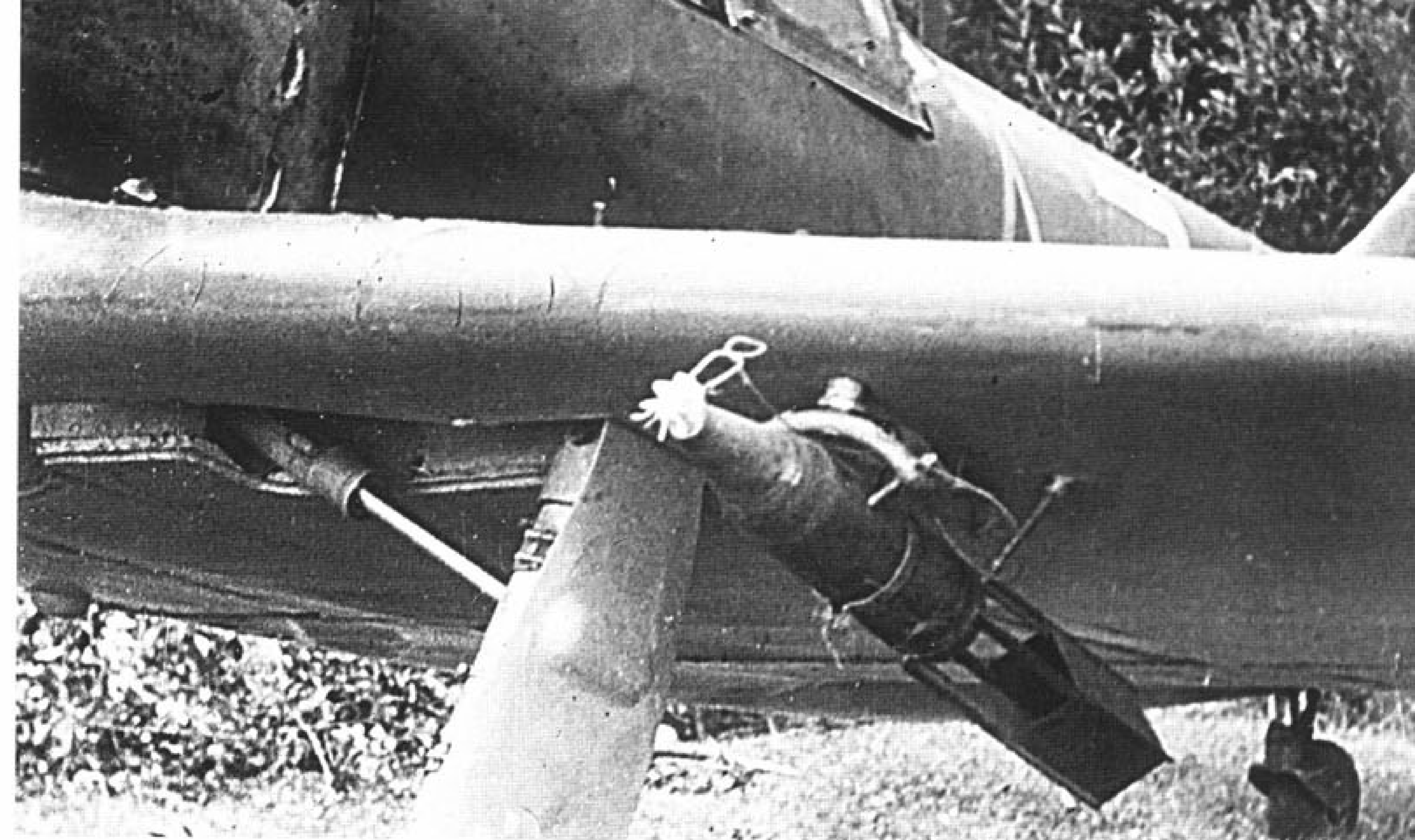
This La-5FN is carrying an AO-25M fragmentation bomb on a D3-40 bomb rack. The AO-25M weighed approximately 25kg (55 lbs) and had a 3.1kg (6.8 lbs) explosive warhead. The AO-25M was equipped with an extended AV-4 fuse which allowed the bomb to detonate above the ground. The inlets in the fuselage exhaust shield are a standard feature of the La-5FN. (Ladislav Valousek)
