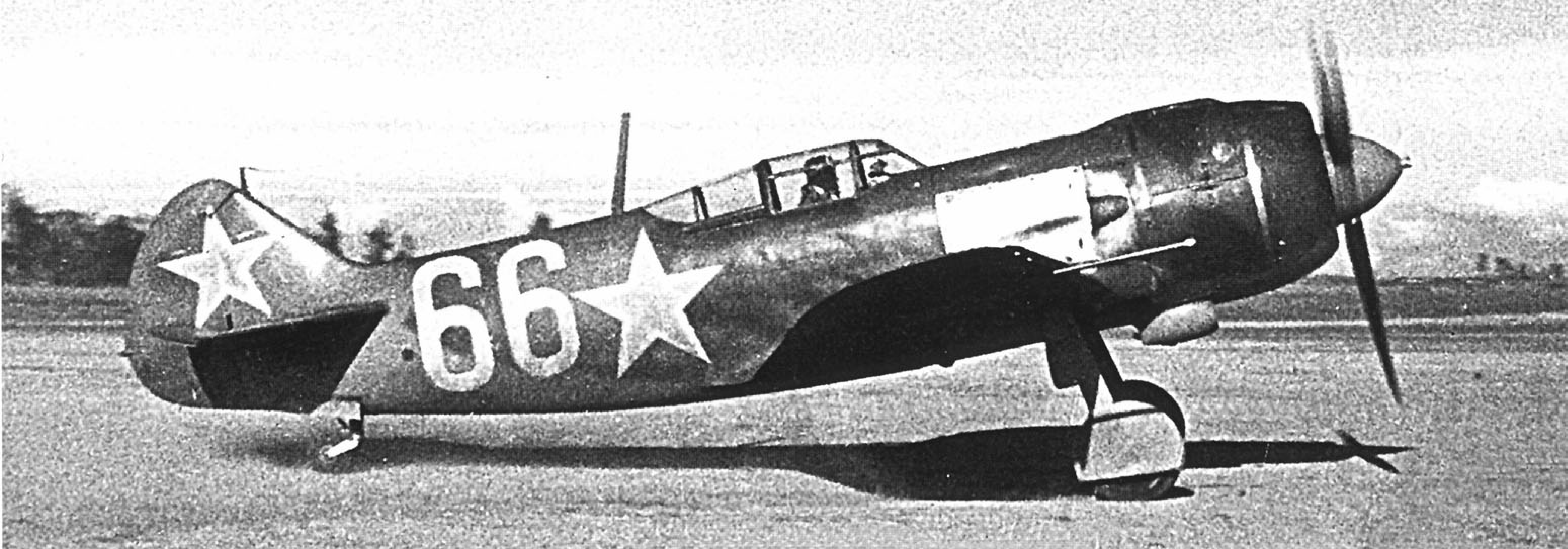
(Above) An La-5F (white 66) of the 21st Fighter Aviation Regiment taxis out for a mission during the summer of 1944. The silver bands on the cowling are flexible metal straps designed to hold the cowl together. Most La-5Fs had a forward slanted antenna mast while the initial production variants had a vertical antenna mast. The cut down rear fuselage and aft canopy glazing of the La-5F greatly improved the pilot's rearward vision over that of the LaGG-3-based La-5. (Ivan Ivanov)
