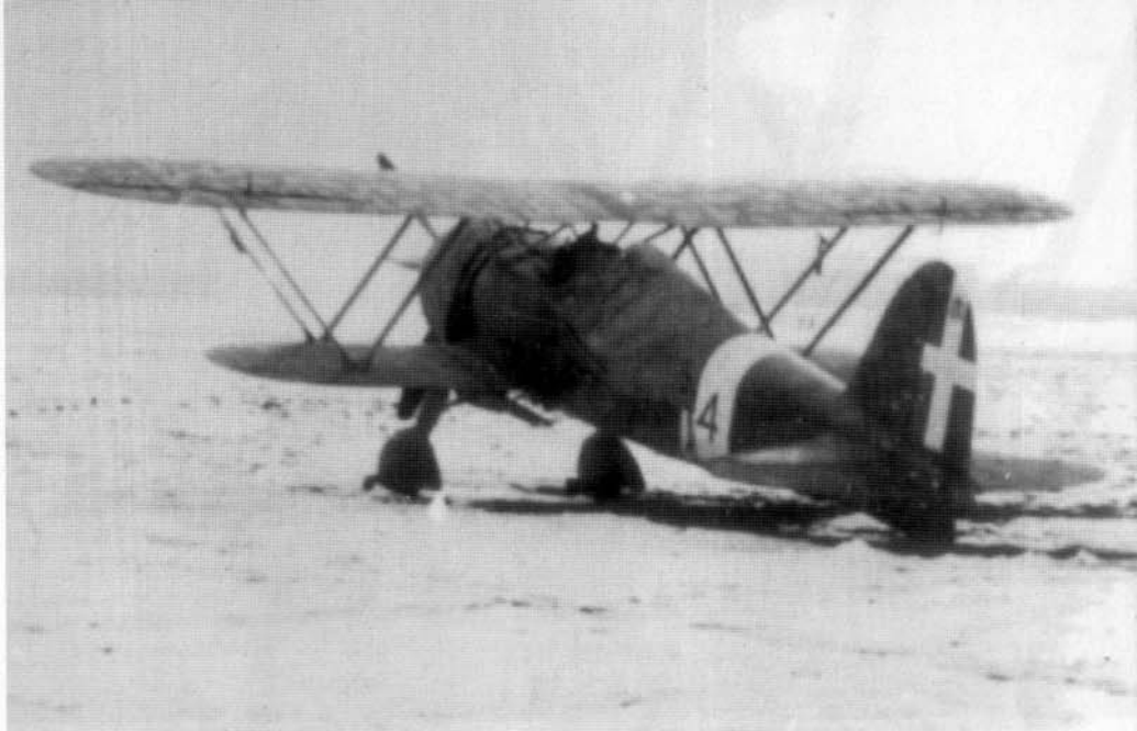
A canvas cover keeps the snow out of this CR 42's cockpit during the winter of 1942-43. This Falco was modified for night attack missions with an exhaust flame damper installed under the fuselage. Italian national insignia are not painted on the upper wings of this aircraft. Uppersurfaces were camouflaged in dark green and medium green. (SMA)
