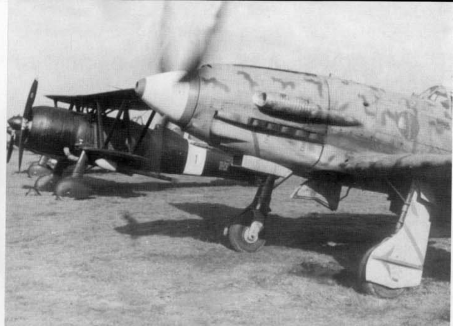
This black CR 42CN is equipped with a long flame damper. Night fighter Falcos built for the Regia Aeronautica employed both long and short dampers. A 220.5 lb bomb is installed under the starboard wing for night attack duties. The aft fuselage band and lettering are in white. An MC 200 fighter runs its engine in the foreground. (Bundesarchiv)
