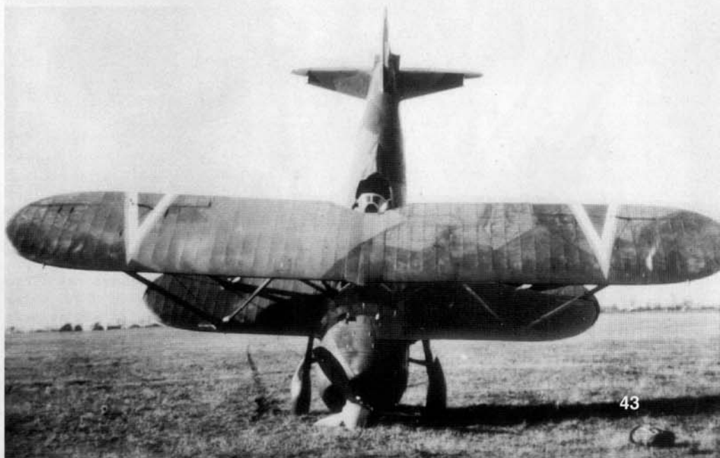
The nosed-over CR 42 wears the Hungarian national markings worn from 1 September 1938 until 1 March 1942. These consisted of chevrons in green (inside), white, and red painted from trailing edge to leading edge. The upper wing span of the Falco was 31.8 ft (9.7 m), while that of the lower wing was 21.3 ft (6.5 m). (Kovács)
