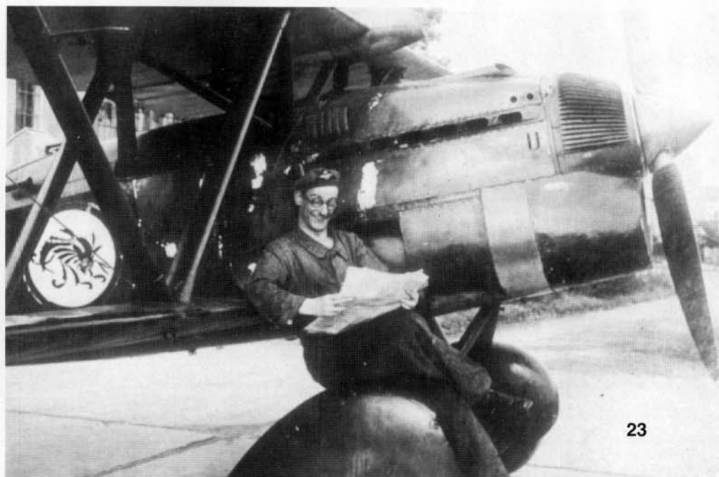
(Below) An apparently amused ground crewman reads a newspaper while seated on the starboard wheel spat of a 1/5. 'Dongó' Squadron CR 32. A series of 42 cooling fins were mounted over the oil tank, which was located behind the propeller. Cooling air for the oil and water radiators was ducted through the chin intake below the propeller spinner. The water radiator is left in natural metal. (Kovács)
