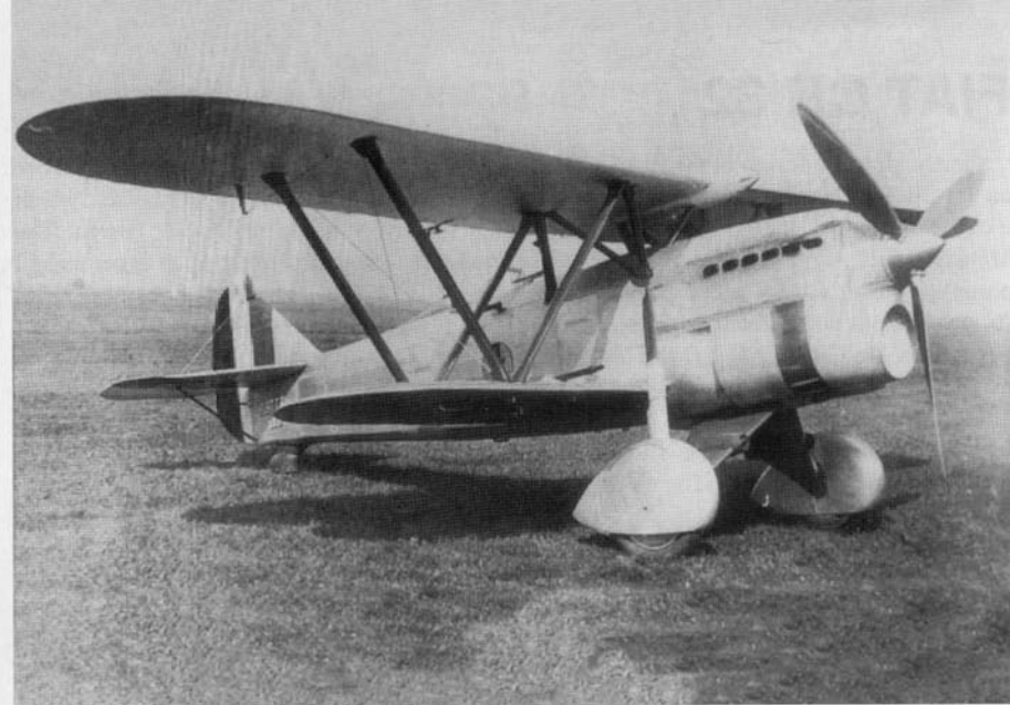
The CR 33 employed a 700 hp FIAT A.33 R.C. 35 engine on a CR 32 airframe. Flown for the first time in 1937, this aircraft employed a three-bladed propeller and modified landing gear struts. A 7.7mm machine gun was mounted in each lower wing. The CR 33 reached a maximum speed of 262 mph (421.6 kmh) in tests; however, this aircraft did not enter operational service. (Punka)
