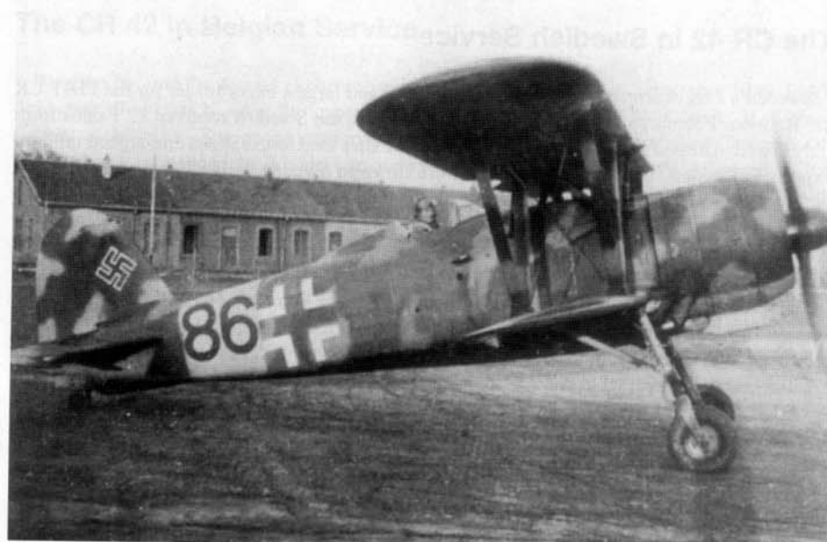
This Luftwaffe CR 42AS taxis at its base near Strasbourg, France on 28 October 1943. A red tactical number 86 is painted on the yellow aft fuselage band. The aircraft is painted dark green over light gray, using Italian colors. The main landing gear fairings were removed to facilitate operations from muddy airfields. (Petrick)
