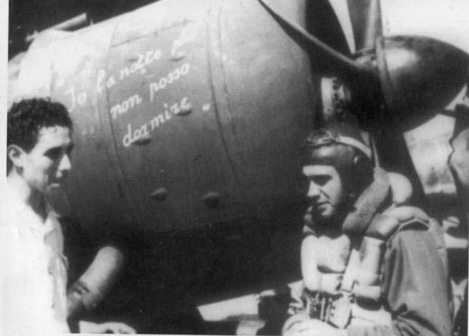
Capt Ricci poses with fellow pilots by the cowling of his CR 42CN at Ciampino on the outskirts of Rome. The inscription on the cowling reads " Il la notte piu non posso dormire " ("I can't sleep tonight"). The small blisters on the cowling provided clearance for the engine rocker arm covers. Ricci served as commanding officer of 167 o Gruppo Autonomo during 1942. (LUCE)
