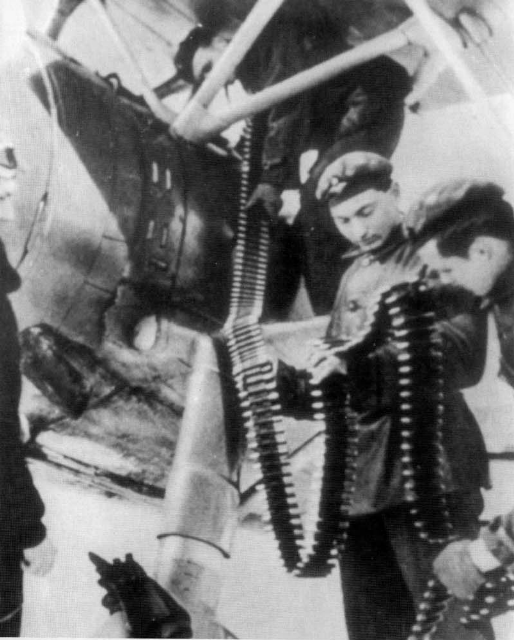
MKHL ( Magyar Királyi Honvéd Légiero ; Royal Hungarian Air Force) armorers feed 12.7mm machine gun ammunition belts into the port ammunition bin of a CR 42. Each 12.7mm Breda-SAFAT was provided with a maximum of 400 rounds of ammunition. The wingroot oil cooler intake has been covered on this aircraft during servicing. (Punka)
