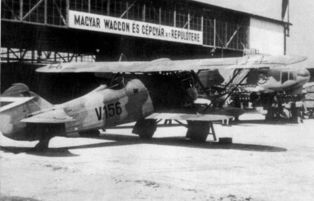
CR 32 (V.156) is parked in front of a hangar at a Hungarian maintenance facility. The aircraft is camouflaged in dark green, dark brown and medium gray uppersurfaces. The fuselage code is black. The V on the fuselage stood for vadász (fighter). The 'benches' appearing on the upper wing are outriggered aileron balance tabs. (Punka)
