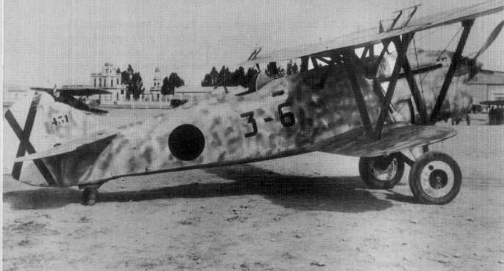
CR 32bis (451) is parked at Republican-held Don Benito airfield after its Italian pilot landed there by mistake on 19 September 1936. The wheel spats were removed from the CR 32 – a normal practice when operating from muddy airfields. A Republican Nieuport-Delage 52 fighter is parked behind the CR 32's tail. (de Celis Borrell)
