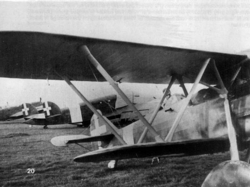
(Above Left) A camouflaged CR 32 is parked in front of other CR 32s at an Italian air base early in World War Two. The front propeller blades remained in natural metal, while the back of the blades was painted flat black to eliminate glare. The Italian insignia on the wings consisted of three fasces on a white disc trimmed in black. The Italian upper surface camouflage of dark green and sand wrapped around the leading edges of the wings and horizontal tail surfaces. (Punka)
