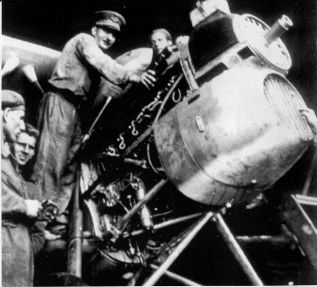
Maintenance crewmen service the 690 hp FIAT A30 RA engine of a first production series CR 32. This liquid-cooled, V-12 engine also powered the earlier CR 30 fighter. The FIAT two-bladed steel propeller has been removed. Oil cooling fins were mounted on the oil tank in front of the open engine. (Punka)
