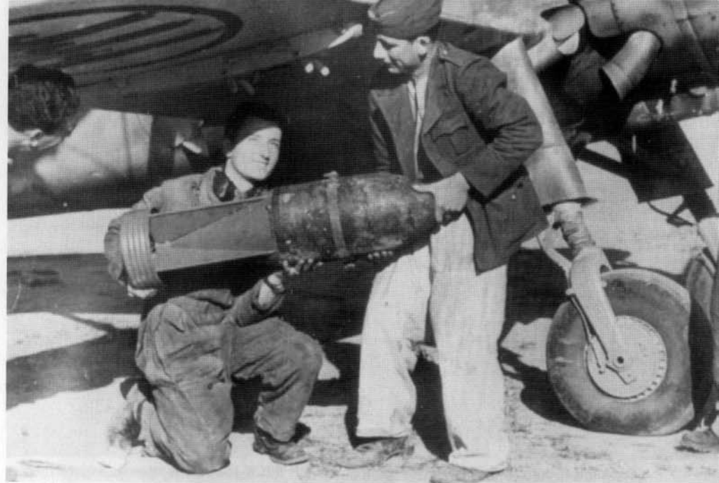
Armors lift a 220.5 lb (100 kg) bomb up to the starboard bomb rack of a CR 42AS assigned to 164 a Squadriglia , 161 o Gruppo Autonomo in the Mediterranean. The lower main landing gear fairings were often removed from ground attack Falcos to facilitate maintenance. Oil cooler intakes were located in both wing roots. (Punka)
