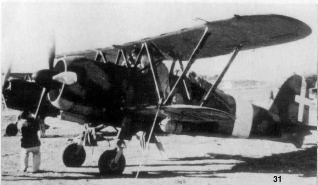
A CR 42AS is prepared for a ground attack mission in North Africa in 1941. The wheel fairings have been removed and a 220.5 lb bomb is mounted on the starboard bomb rack. The aircraft is camouflaged in dark green and dark brown with light gray undersurfaces. (Punka)
