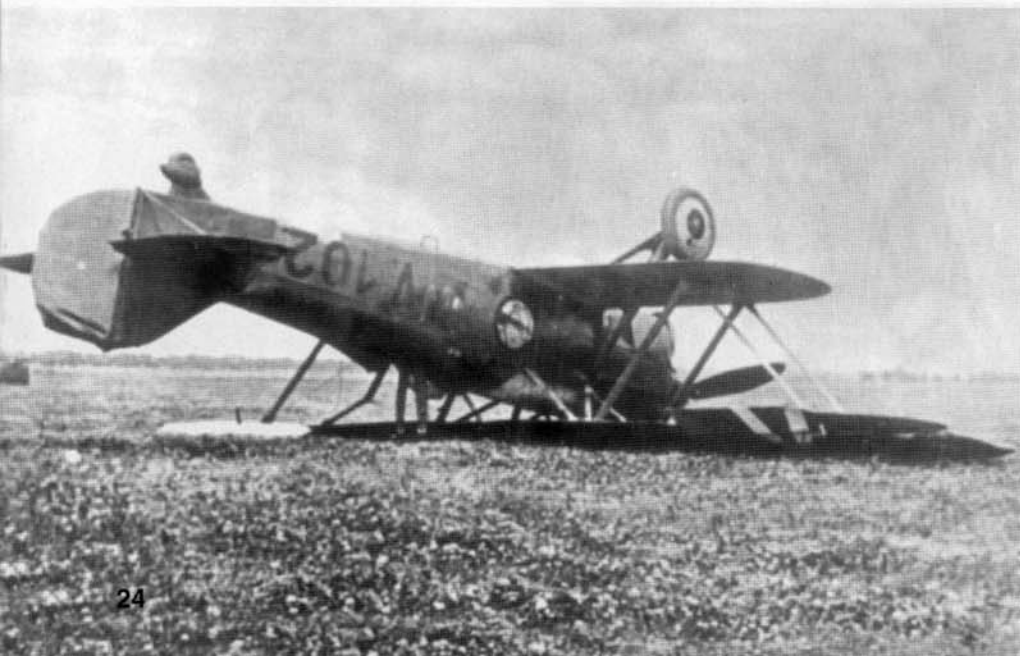
CR 32 (V.102) overturned at a Hungarian airfield, causing damage to the top of the rudder and upper wing. This aircraft wears the insignia of 1/1. 'Ijász' (Archer) Fighter Squadron. This CR 32 is missing the national insignia on its tail. (Punka)
