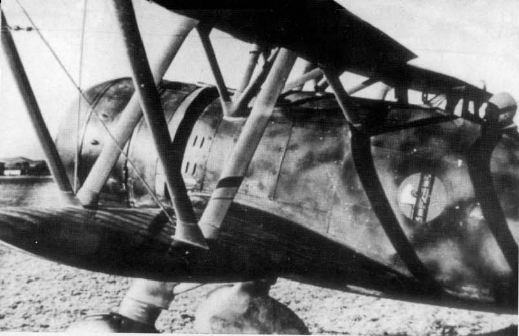
The fuselage fascies emblem was located under the windshield on CR 42s. A kick step for cockpit access is placed aft of the fascies. Access panels on the forward fuselage near the base of the upper wing struts open to allow servicing of the fuel tanks and ammunition bins. The panels were hinged at the top and secured for flight with screws. (Punka)
