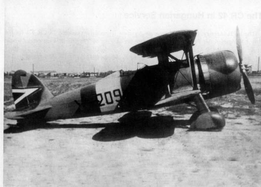
The Hungarians modified this CR 42 (V-209) to accept a 930 hp Manfred Weiss WMK-14A engine in 1941. This air-cooled radial engine was a French Gnome-Rhone 14Kfs powerplant built under license. The WMK-14A also powered the Hungarian-produced Regianne Re 2000 Héja (Hawk) fighter. (Kovács)
