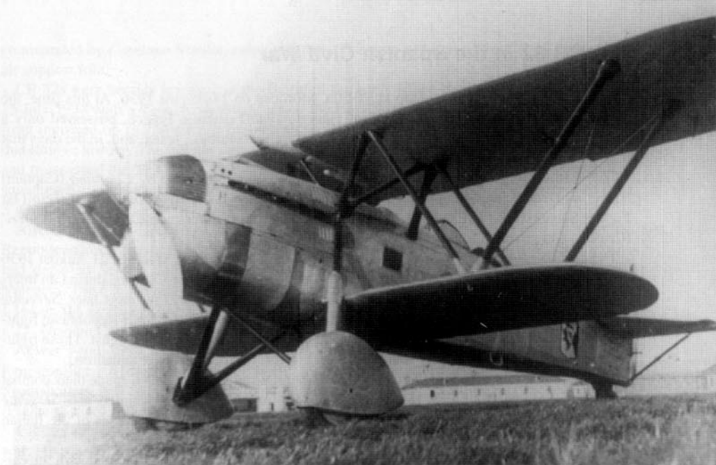
The bullet fairing mounted in the center of the upper wing of this 4 o Stormo CR 32 contained a 6.6 gallon (25 L) auxiliary fuel tank. The main fuel tank housing 90 gallons (341 L) was mounted between the cockpit and the engine firewall. The wing struts were usually painted black on silver finished CR 32s before World War Two. (Punka)
