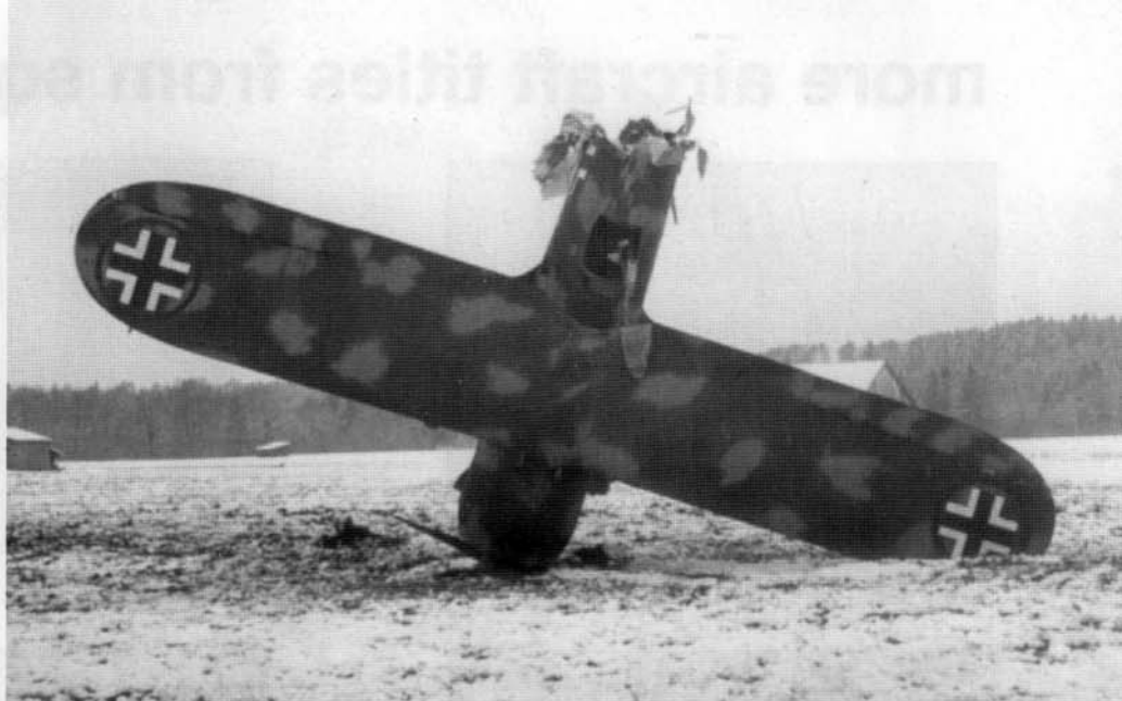
The nosed over CR 42AS (M.M. 90823) reveals the damage caused by the crash landing at Andelfingen. Despite the loss of the tail, the wings and their Warren Truss support structure are remarkably intact. German crosses were painted over the Italian roundels on the upper wings, however, the black rings of the former markings surround the crosses. The aircraft is painted Italian dark green over Italian light gray. (Stapfer)
