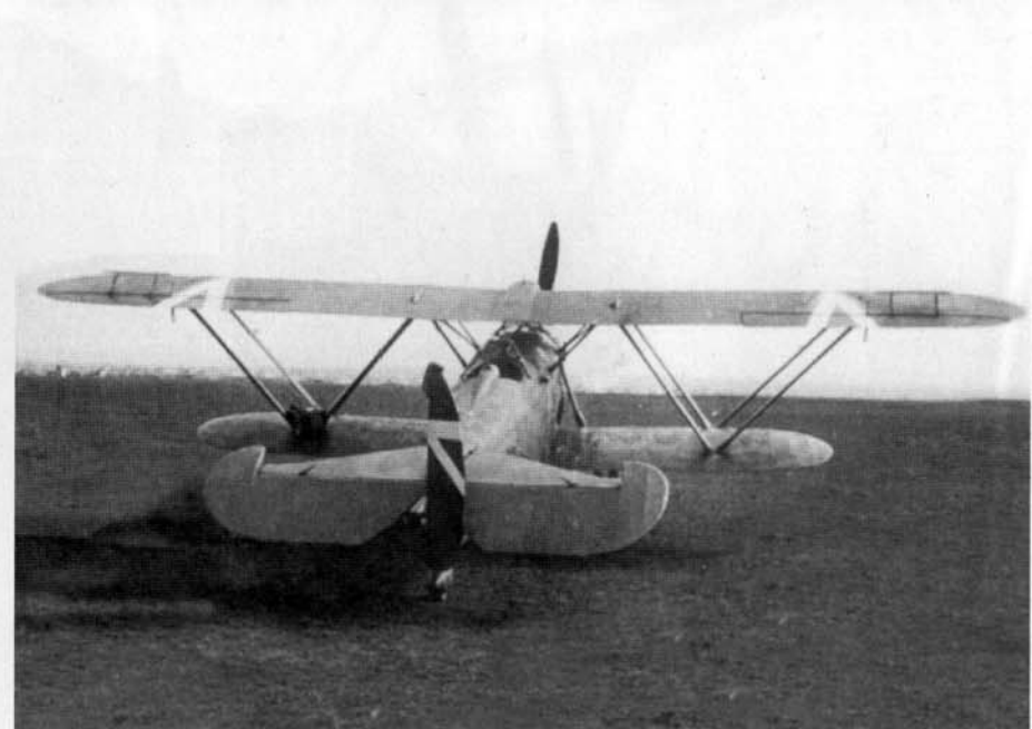
This Hungarian CR 32 displays the Warren Truss struts supporting the wings and the N-type cabane struts connecting the upper wing to the fuselage. The last pilot operating this aircraft left the elevator lowered and the rudder turned to starboard. (Punka)
