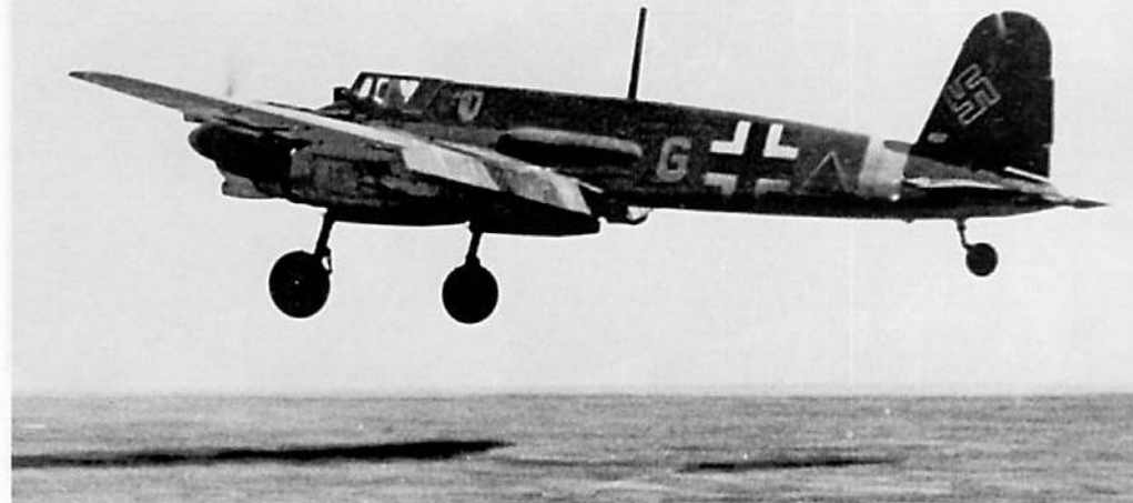
An Hs 129B-1, Yellow G, takes off on a ground attack mission over the Eastern Front during the summer of 1942. This aircraft was assigned to II./Sch.G 1 and the Gruppe's insignia was placed aft of the canopy. The Hs 129B-1 was armed with a 30mm MK 101 cannon under the fuselage for engaging Soviet armored vehicles. (Dabrowski)
