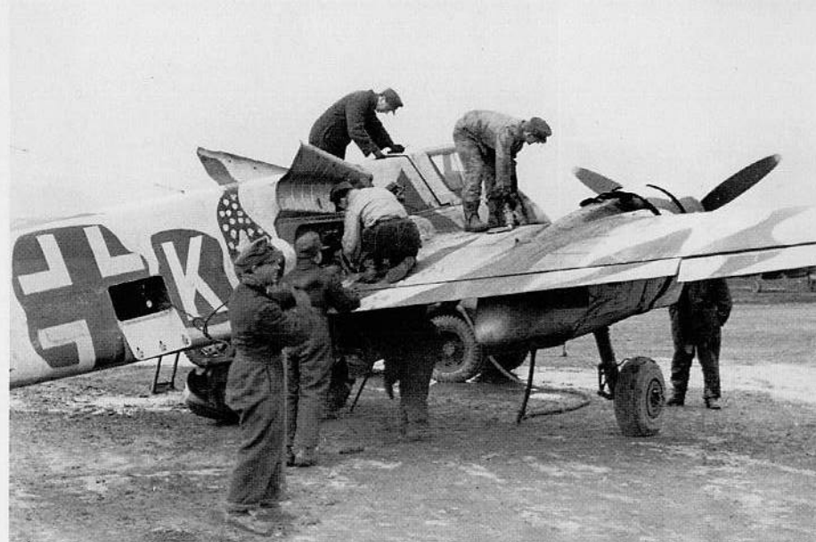
Ground crewmen service an Hs 129B-2, White K, prior to a mission over the Eastern Front in early 1944. While fuel was pumped into the starboard wing tanks, armorers fed 20mm ammunition to the MG 151/20 cannon on the fuselage sides. This aircraft was assigned to 10.(Pz)/SG 9 (10th Anti-Tank Squadron, Ground Attack Wing 9) in the Ukraine.
