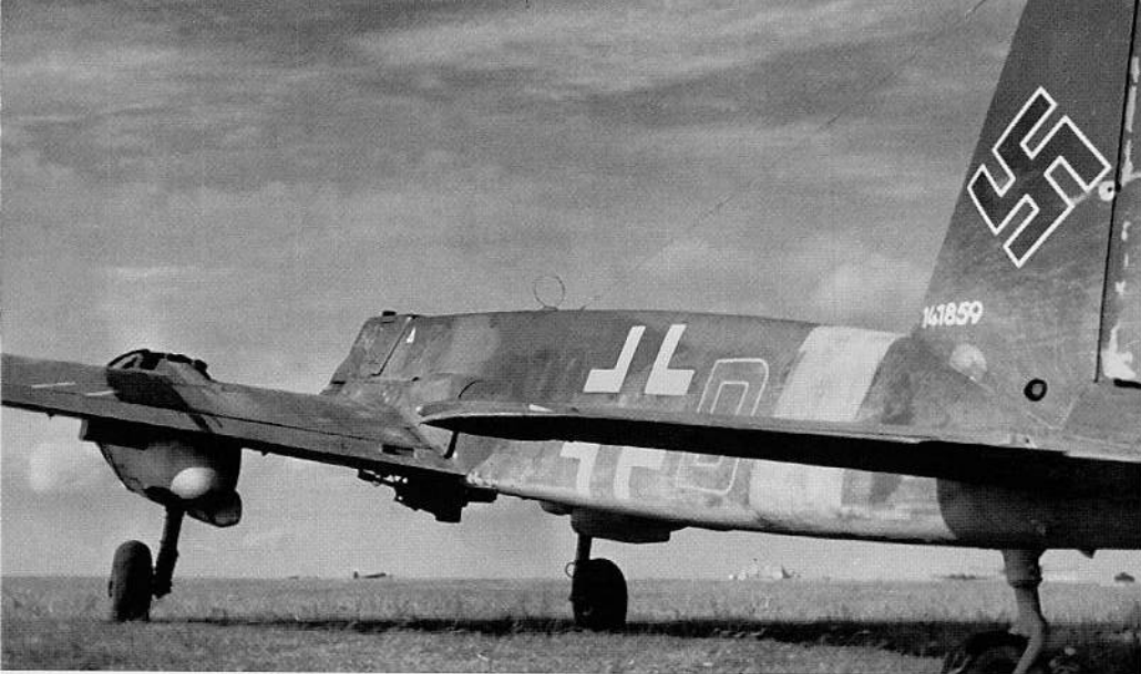
An Hs 129B-2 (Red D, W. Nr. 141859) prepares to takeoff on another 'tank busting' mission over the Eastern Front, armed with a 30mm MK 103 cannon under the fuselage. The bulge over the wing root enclosed the breech of the 20mm MG 151/20 cannon mounted on each side of the aircraft. An RDF loop antenna was placed on the upper fuselage, while a wire radio antenna ran from the upper mid-fuselage to the vertical stabilizer.
