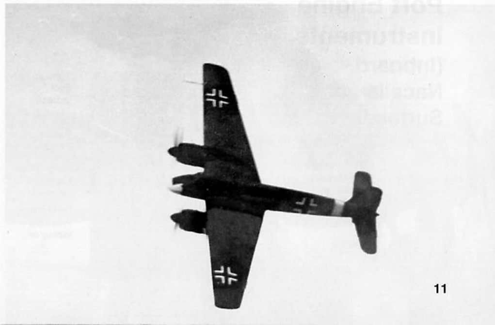
An Hs 129B-1 banks to port while flying at low level over its base. The Berta (B model) had straight wing leading and trailing edges, replacing the swept leading edges of the Anton (A Model) wings. Axis Eastern Front identification markings included RLM27 Yellow (FS33637) noses and aft fuselage bands. (Petrick)
