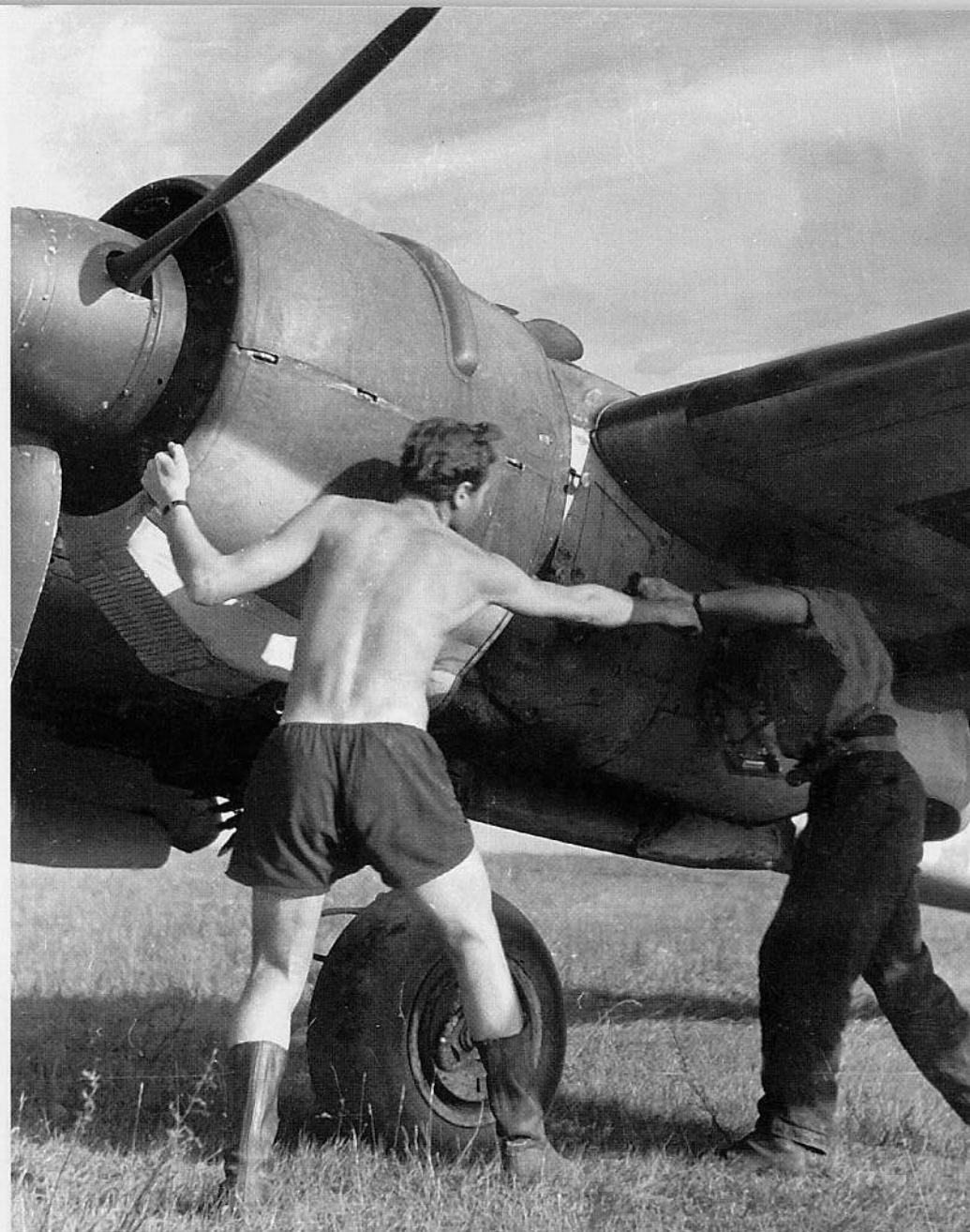
Two Luftwaffe ground crewmen team up to start the port engine of this Hs 129B-2 during the summer of 1943. Both Gnome & Rhône 14M engines were started using inertial cranks, which required considerable strength on the crewman's part. The Hs 129B upper and lower cowling halves were secured using three flush fasteners on each side.
