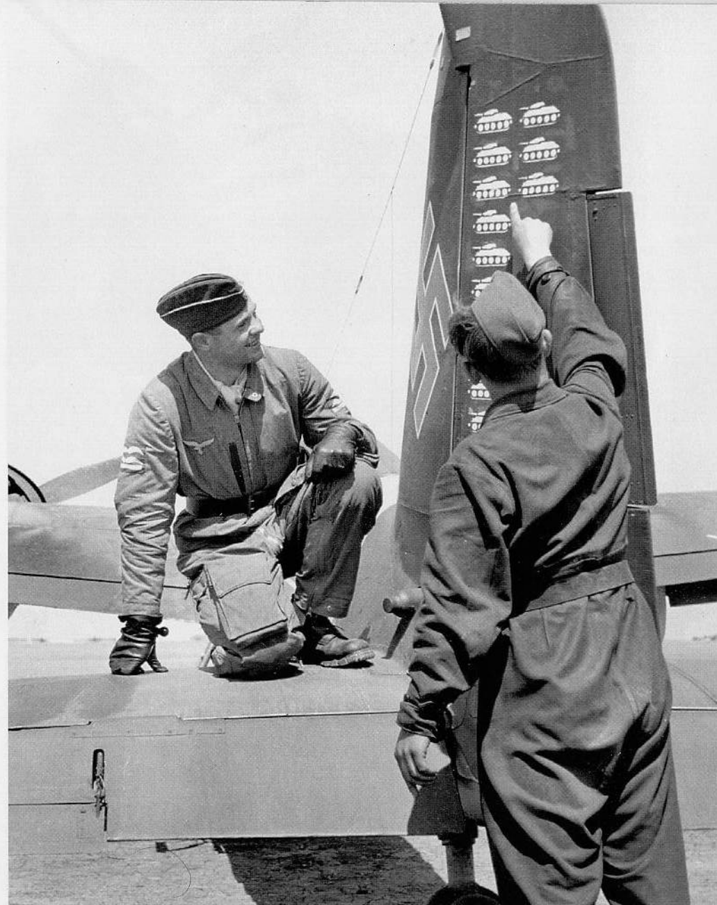
Oberleutnant (1/Lt) Rudolf-Heinz Ruffer looks at the rudder of his Hs 129B-2, Red G, while a ground crewman points to one of the white tank 'kill' marks painted on the aircraft's rudder. The Hs 129's control surfaces – rudder, elevator, and ailerons – were fabric-covered metal framing. Ruffer was later promoted to Hauptmann (Capt) and destroyed over 80 Soviet tanks before he was killed in action on 16 July 1944. (Pegg)
