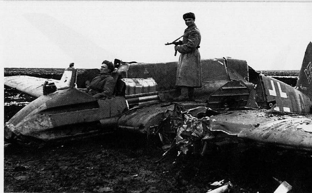
A Soviet soldier sits in the cockpit of an Hs 129B-3 (NK+DA), which made a forced landing in Moldavia, Rumania on May of 1944. The impact broke this aircraft's fuselage in half; however, the Hs 129's forward fuselage remained intact. The canopy and engines were removed from this aircraft. (Geust)
