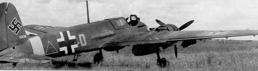
An early production Hs 129B-2, Yellow D (W. Nr. 0226), rests at a forward airbase in southern Russia during the summer of 1942. This aircraft featured the straight antenna mast on the upper fuselage and the long engine exhaust pipes. Yellow D crash landed due to poor visibility on 4 August 1942 and sustained 35 percent damage. This Hs 129B-2 was repaired at a front Werft (large repair shop) and returned to service. (Griehl)
