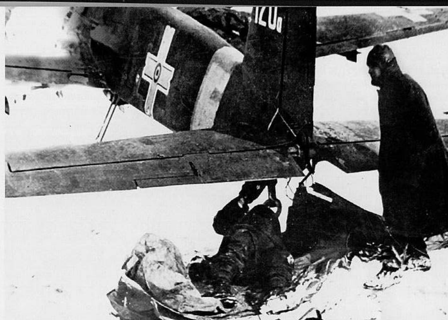
A mechanic repairs the tail wheel of Hs 129B-2 No. 120a (W. Nr. 140715) at Nikolayev in November of 1943. He had only a tent sheet placed on the snow-covered ground for his work platform. German and Rumanian Hs 129 ground crewmen performed their duties under all weather conditions. (Bernád)
