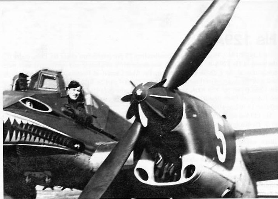
The pilot of White 5 leans out of the cockpit of this Hs 129A-0 (W. Nr. 3005). The vanes placed on the propeller spinner controlled the pitch of the two-bladed Argus propeller. The large opening under the propeller spinner was the oil cooler intake, while the two smaller flanking orifices fed air to cool the Argus As 410A-1 engine. This same combination of Argus engines and propellers was used on the Focke-Wulf Fw 189 reconnaissance aircraft. (Möller)
