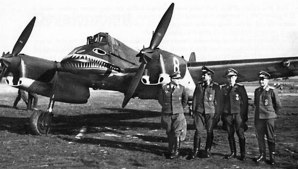
Luftwaffe pilots pose in front of White 8, an Hs 129A-0 (W. Nr. 3008, GM+OE) assigned to the Ergänzungszerstörergruppe for training Hs 129 pilots. Hs 129As and early Bs had a large circular landing light mounted on the port wing. The pilot used this light to illuminate the ground below and in front of his aircraft during approach, landing, and taxiing. White 8 was destroyed in an accident in Poland on 15 July 1942. (Möller)
