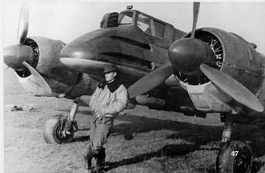
Tech Sgt Trifan Bulhac leans against his bomb-laden Hs 129B-2 (No. 100, W. Nr. 141879) during the fall of 1944. The Rumanians overpainted the Axis yellow nose of this captured German aircraft with dark green over light blue after Rumania's defection to the Allies in August of 1944. Four 110.2 lb SC 50 bombs were carried under the fuselage. (Avram)
