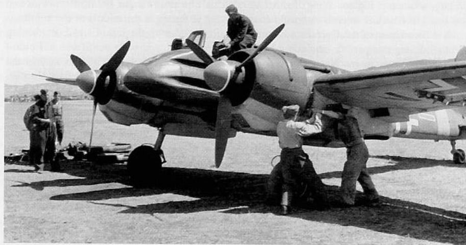
A ground crewman secures the pilot into the seat of his Hs 129B-2 prior to a mission over the Russian steppe during the summer of 1942. Two other ground crewmen are starting the port engine using an inertia crank; this same method started the starboard engine. An ETC 50 bomb rack was mounted under the port wing. Each rack could hold one 110.2 lb (50 kg) SC 50 bomb.
