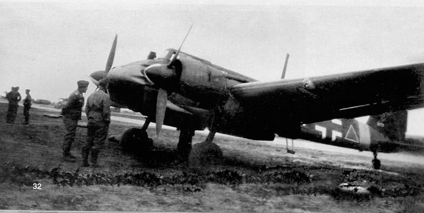
Curious Luftwaffe airmen study one of the first Hs 129B-1s (W. Nr. 0175) assigned to the Eastern Front. The white-bordered black triangle on the aft fuselage indicated ground attack aircraft. This Hs 129B-1 was assigned to Stab II. (Staff II Group)/Sch.G. ( Schlachtgeschwader ; Ground Attack Wing) 1. The propeller spinners were painted white and black on Stab aircraft. Prior to arriving at the front, W. Nr. 0175 developed engine trouble and force landed at its home base of Lippstadt, Germany on 23 August 1942. (Crow)
