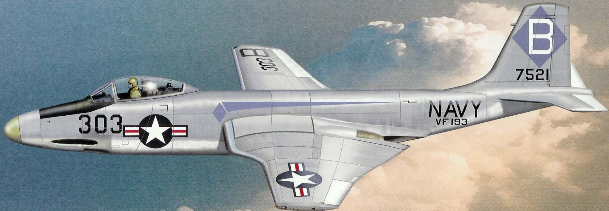
(Above) VF-193 flew this F2H-3 (B-303/BuNo 127521) from USS YORKTOWN (CVA-10) during the mid-1950s. It is painted in the Light Gull Gray over White scheme adopted by the Navy and Marine Corps after studying a variety of finishes, which included Sea Blue and anodized aluminum schemes.
