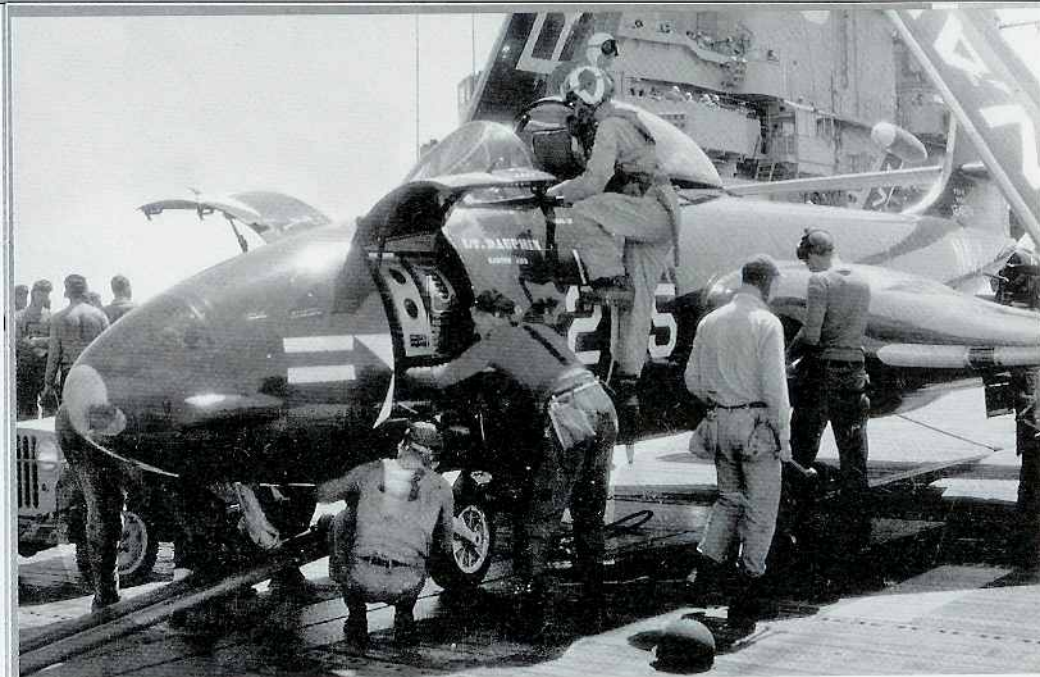
A pilot climbs aboard an F2H-2 (BuNo 124974) prior to a mission from ESSEX. Armors check the ammunition feeds for the nose-mounted 20MM cannon, which were each supplied with 150 rounds. Other deck crewman make last minute checks on the Banshee prior to launch. (USN)
