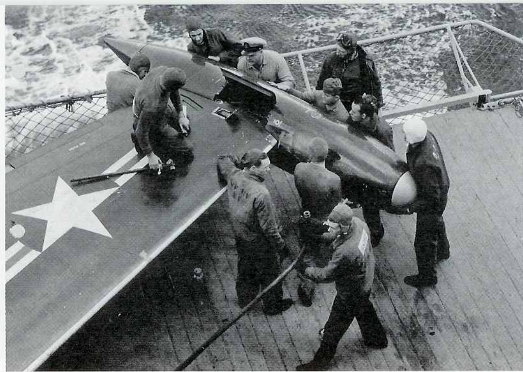
The F2H-2 tip tanks were not permanently attached to the wing tips, but could be removed as needed for maintenance or repair. This deck crew aboard FRANKLIN D. ROOSEVELT (CVB-42) replaces a tip tank during operations in the Mediterranean. The crew held the tank in position while it was fastened to the wing. (USN)
