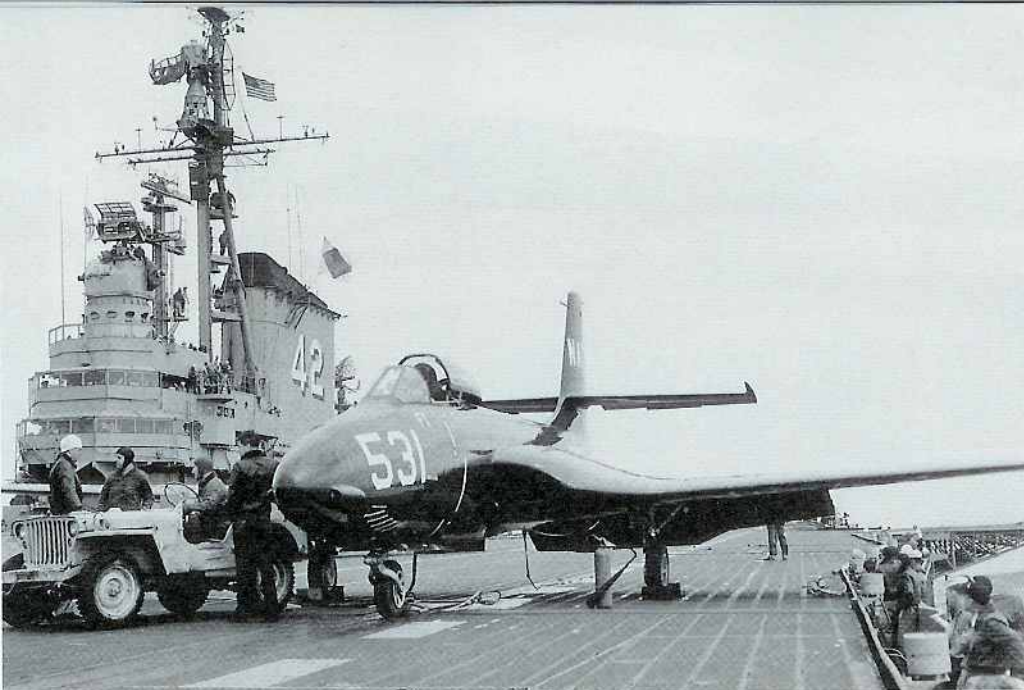
Deck hands wait while an F2H-1 is prepared for a 'cat' shot off ROOSEVELT. The forward cockpit position and tricycle landing gear provided the pilot with excellent forward and downward visibility during all phases of landing and take-off. Older pilots, especially those who flew the F4U Corsair, readily appreciated this feature. The yellow World War Two jeep was used as a tow vehicle. (MDC)
