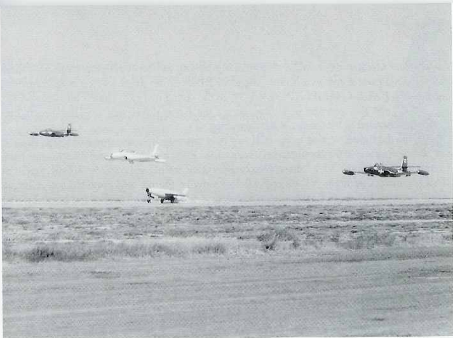
In December of 1952, two specially fitted F2H-2Ps were used to radio guide a Vought Regulus missile to land on San Nicolas Island off southern California. The missile and the two Banshees were launched from USS PRINCETON (CVA-37). One of the F2H-2Ps flies low as the Regulus lands along with an F2H-2 fighter and a TV-2 (T-33). (USN)
