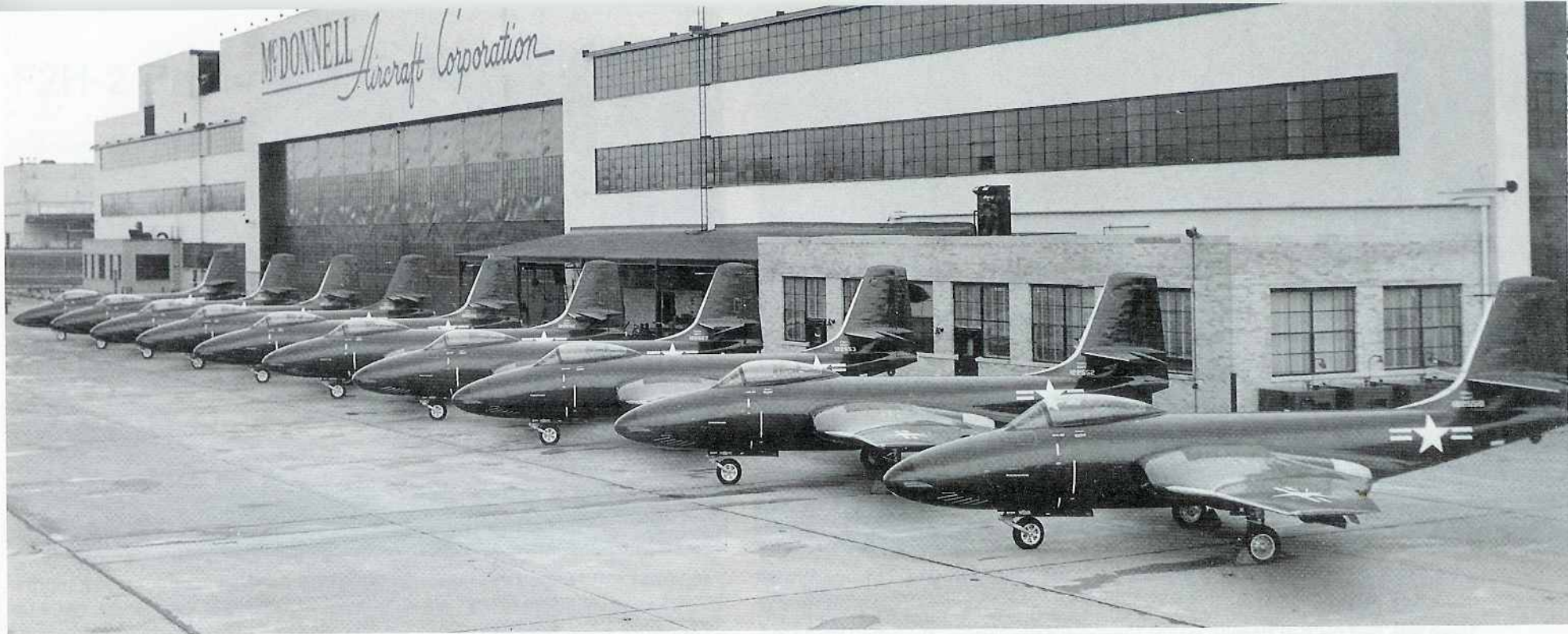
Ten new F2H-1s, the last of the initial production order, are parked in front of the McDonnell plant in St. Louis awaiting delivery to the Navy. The Banshees are overall Glossy Sea Blue (FS15042), with natural metal leading edges. Only basic markings –
