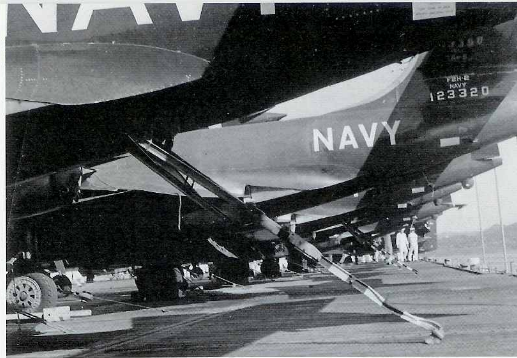
All Banshees were equipped with a hydraulically activated arresting hook for carrier landings. This hook was lowered from the aft fuselage undersurface to catch one of the carrier's arresting cables. The tail hook appears to be painted in red and white bands, although US Navy regulations called for tail hooks to be painted in black and white bands for visibility by deck crews.
