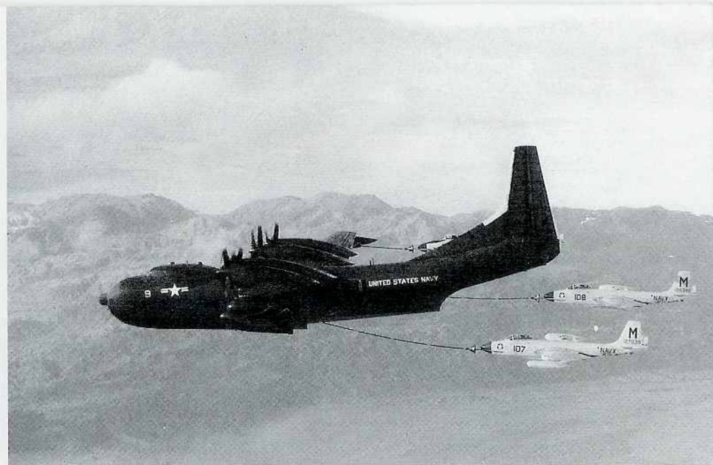
Three VF-23 F2H-3s refuel in flight from a Convair R3Y-2 Tradewind flying boat, whose tail has obscured one of the Banshees. This 1956 exercise over the California mountains tested the Tradewind's ability in the aerial refueling role. The R3Y-2 was cleared for aerial refueling, but saw no tanker service due to engine problems and early retirement. (USN)
