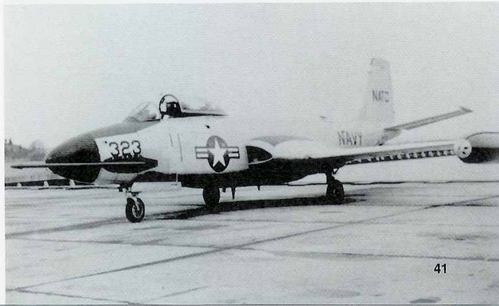
This F2H-3 assigned to the Naval Air Test Center (NATC) has its aerial refueling probe installed. The probe replaced the port upper 20mm cannon and a ventral fairing was placed over the refueling piping. This feature allowed Banshees to deploy over long distances during exercises and in times of crisis. (USN/NA)
