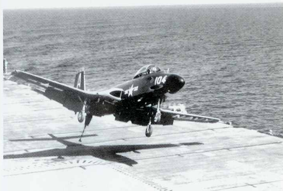
The pilot of this F2H-3 (A-104) just missed the arresting cable while coming down to land on USS RANDOLPH (CVA-15) and started to climb away for another try. The forward position of the cockpit and the large bubble shaped canopy gave the pilot excellent visibility during a landing approach. This made the Banshee one of easier aircraft to land aboard a carrier, not withstanding this particular case. (USN/NA)
