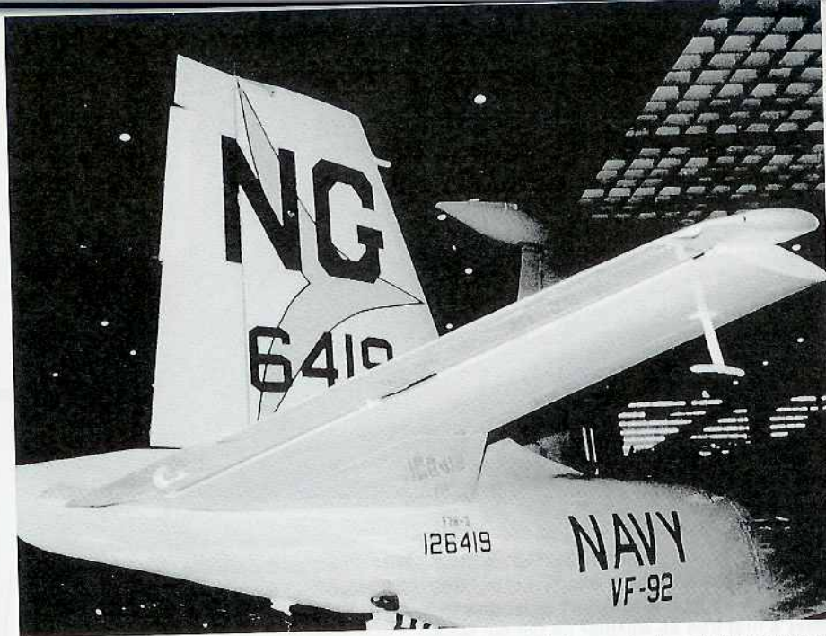
This beautifully restored F2H-3 Banshee (BuNo 126419) is on display at the National Museum of Naval Aviation in Pensacola, Florida. It has the 'horsal' extension fitted to the leading edge of the horizontal stabilizer (tailplane). F2H-3 tailplanes had a 10° dihedral. (Ward)
