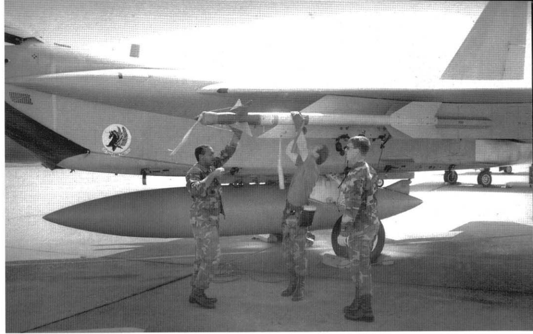
The AIM-9 Sidewinder missile is slid along the port outer stores pylon. Once locked in place, a red REMOVE BEFORE FLIGHT flag is pinned to the missile. A grounding cable is affixed to the stores pylon to prevent any accidental electrical sparking. The yellow cover over the seeker head will be removed before flight. (AI Adcock)
