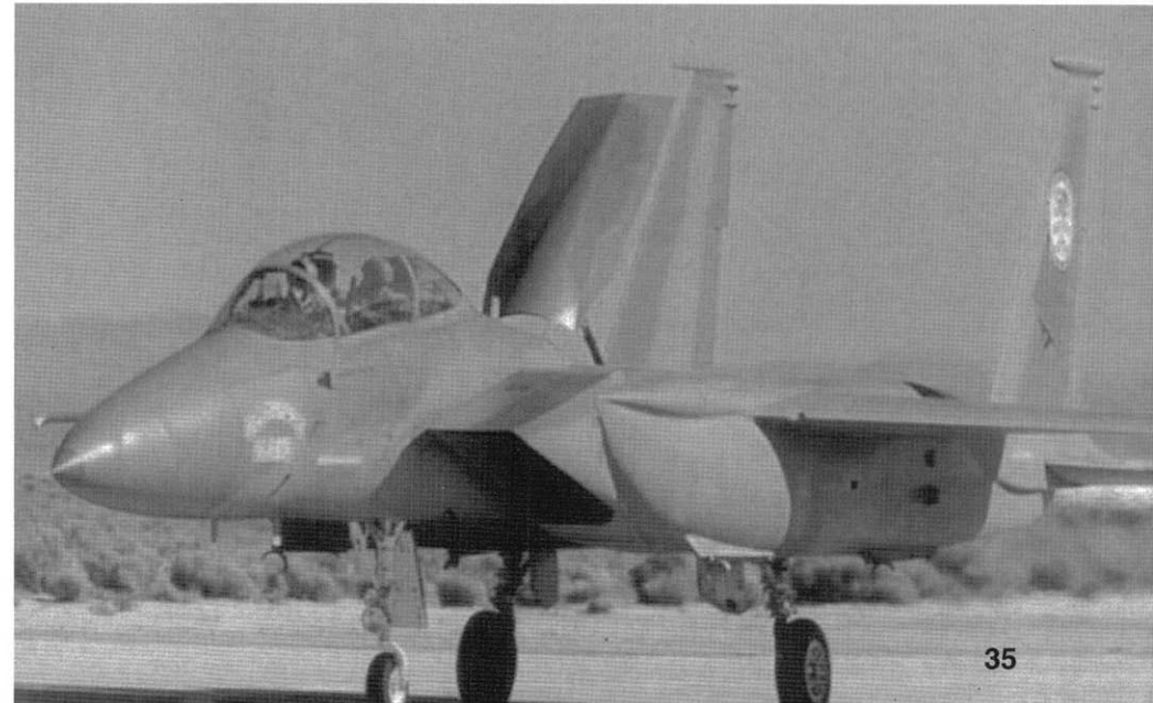
The speed brake is extended soon after GLAMOROUS GLENNIS, an F-15D-38-MC (84-0046) landed at Edwards AFB, California on 14 October 1997. BGen Chuck Yeager flew the Eagle on the 50th anniversary of his breaking the sound barrier in the Bell X-1, also named GLAMOROUS GLENNIS. Conformal Fuel Tanks (CFTs) are mounted on this F-15D. (USAF)
