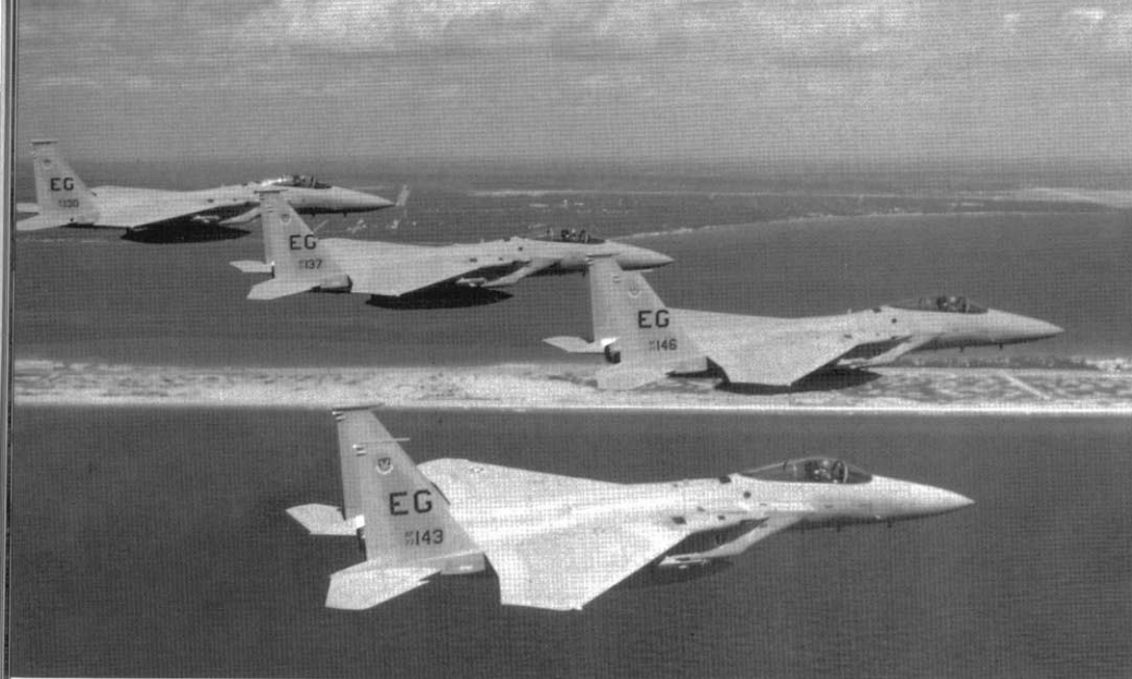
Four F-15A-20-MCs from the 59th TFS, 33rd TFW at Eglin AFB fly along Florida's Gulf Coast in the late 1970s. The Block 20 aircraft were the last F-15As built by McDonnell-Douglas before production switched to the F-15C. The tail stripes are yellow and the Eagles are each fitted with a single 600 gallon centerline fuel tank. (McDonnell Douglas)
