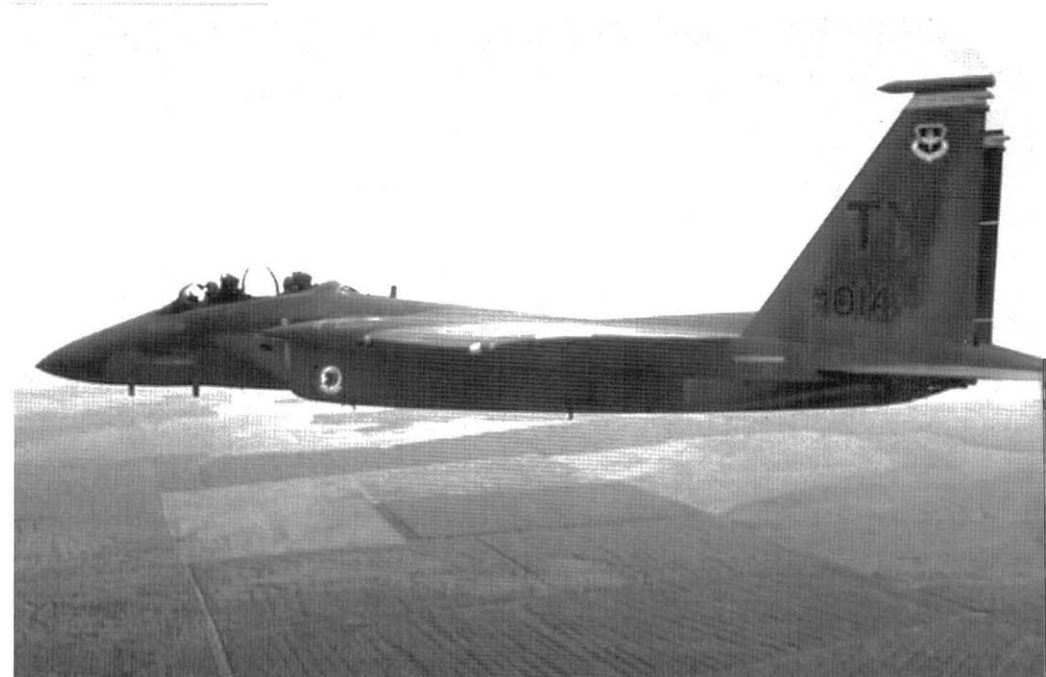
This F-15D-26-MC (79-0014) is assigned to the 2nd FS, 325th FW at Tyndall AFB, Florida. The Eagle is used in the training role, with a secondary role of air defense of the southern United States. The vertical stabilizer has the Air Education and Training Command (AETC) badge below the yellow tail band. The 2nd FS badge is affixed to the air intake. (USAF)
