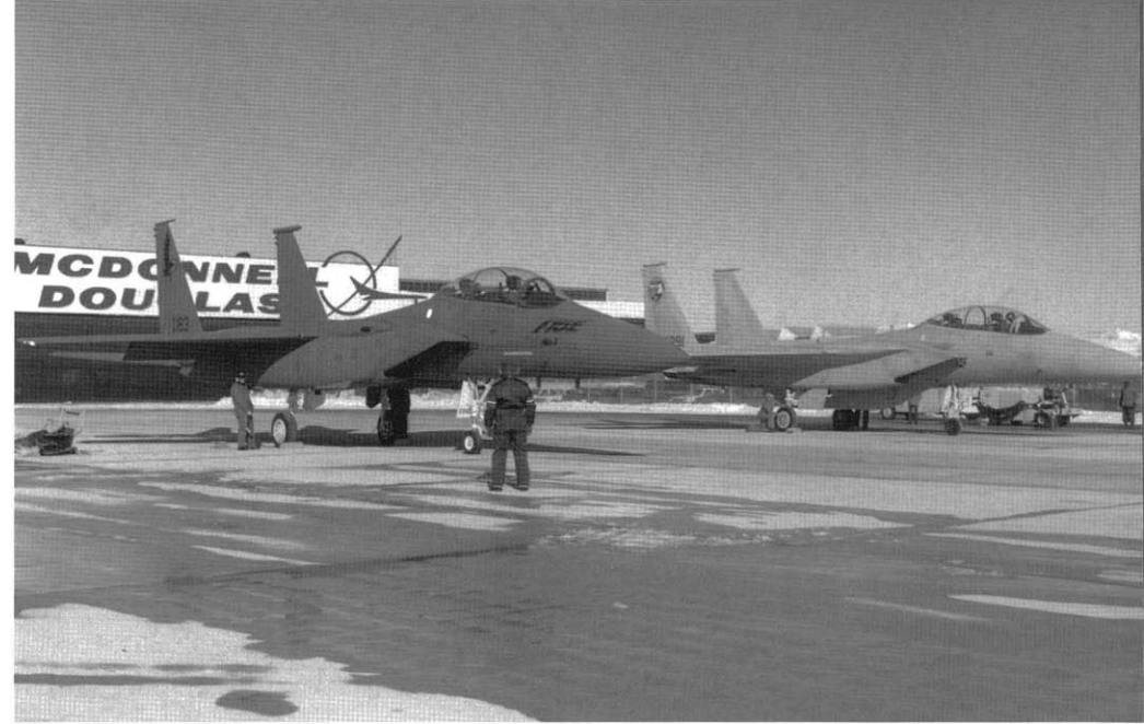
The first F-15E (86-0183) is parked alongside the second F-15B (71-291) outside McDonnell Douglas' St. Louis plant in January of 1987. This F-15B was used in the 'Strike Eagle' tests, which led to the F-15E. The Eagle's engine inlets move from -11° to +4° to provide optimum airflow at all speeds. (McDonnell Douglas)
