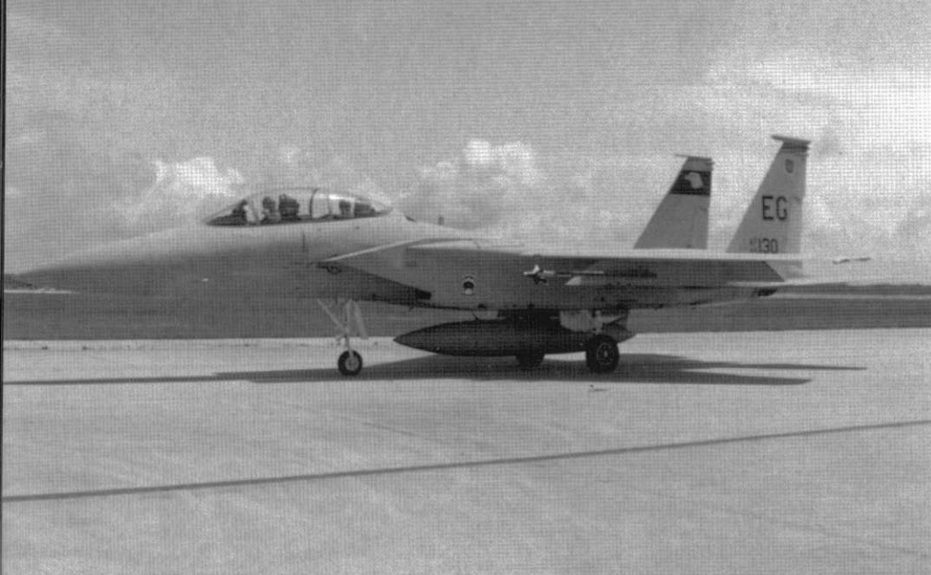
An F-15D-39-MC (85-0130) from the 58th FS, 33rd FW taxis to the active runway at Eglin AFB, Florida in July of 1992. The tail band is blue and the Squadron's badge is painted on the air intake. This Eagle is fitted with a 600 gallon centerline fuel tank and one AIM-9 Sidewinder missile on the port wing pylon. (AI Adcock)
