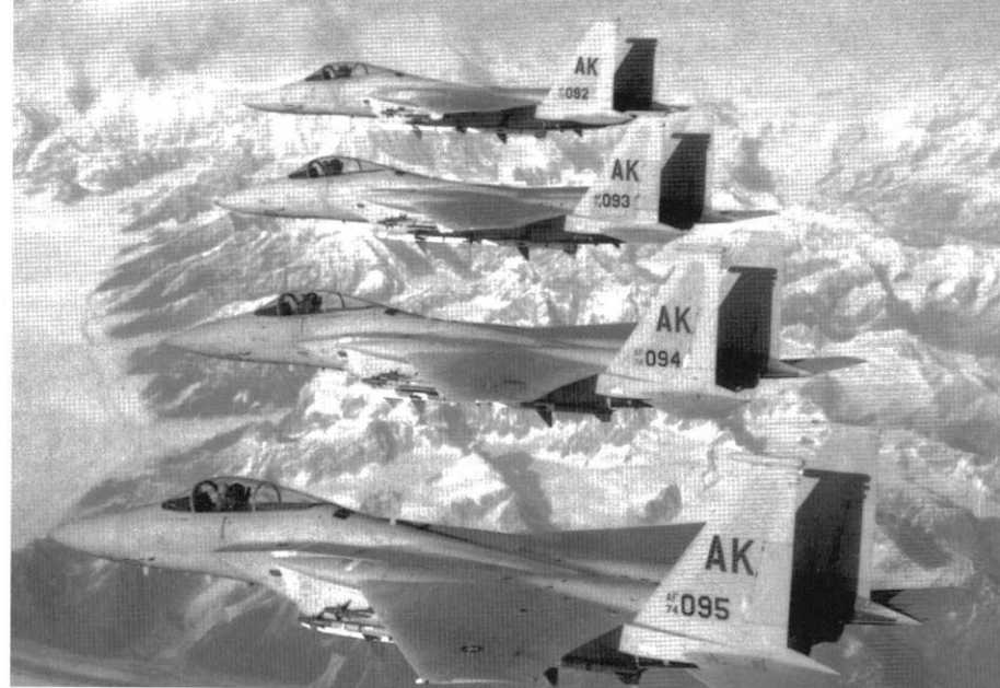
Four F-15A-11-MCs (74-092 through 095) fly over snow covered mountains in Alaska. The Eagles are assigned to the 43rd TFS, 21st TFW at Elmendorf AFB, Alaska. All aircraft are armed with four AIM-7 Sparrow missiles along the fuselage sides and four AIM-9 Sidewinder missiles on the wing pylons. (McDonnell Douglas)
