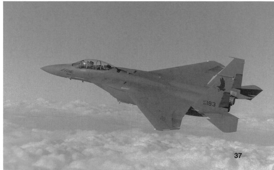
The first F-15E (86-0183) was an F-15D Block 41 airframe upgraded to E model standards. The aircraft is camouflaged in the overall Gunship Gray (FS36118) scheme, which became standard for all USAF F-15Es. A black eagle motif is painted on the outboard vertical stabilizers. (USAF)
