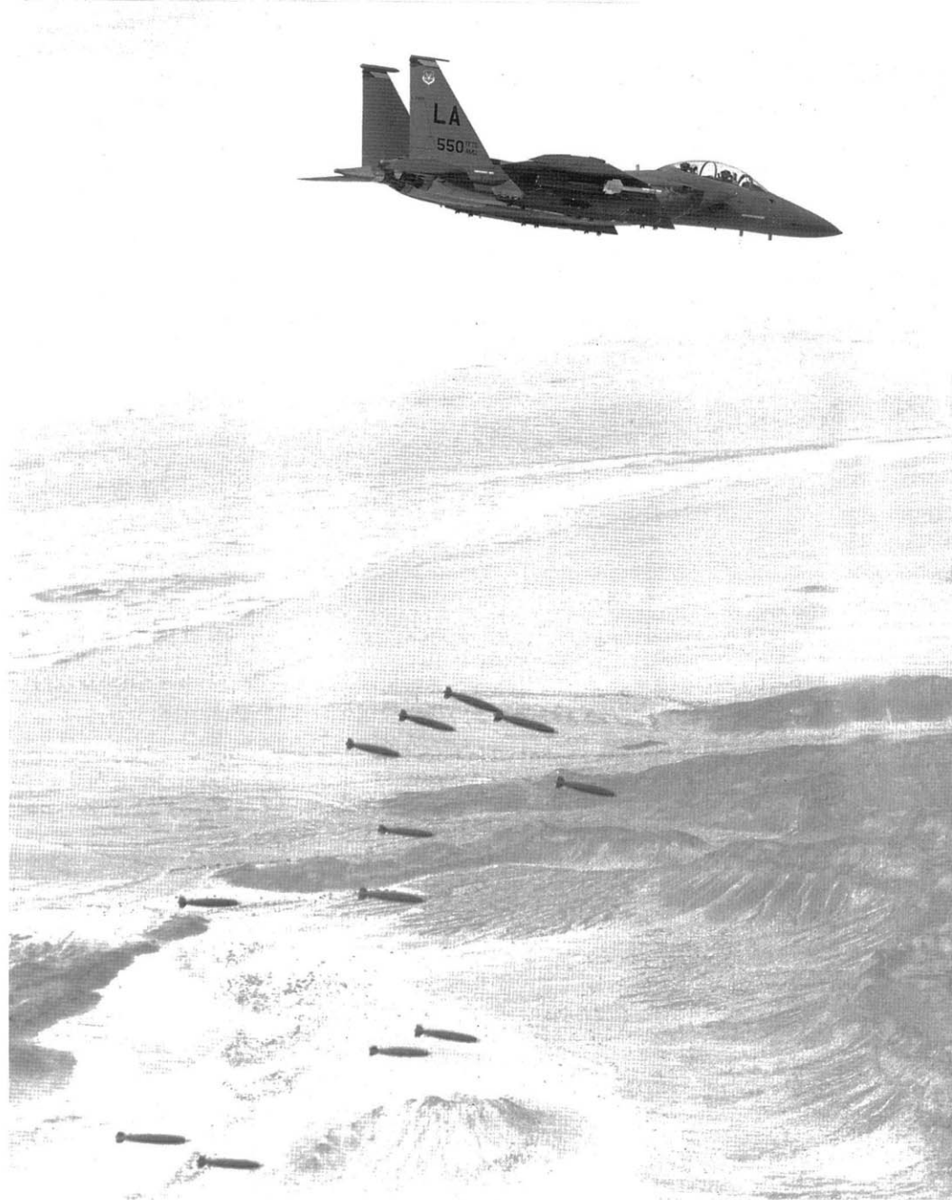
A 550th TFTS F-15E-43-MC (87-0187) drops twelve 500 pound Mk 82 bombs on the Goldwater Test Range in June of 1989. These weapons were released from tangentially mounted pylons fitted to the Conformal Fuel Tanks (CFTs). Markings on the vertical stabilizer indicate this F-15E is the 'flagship' of the 550th Aircraft Maintenance Unit (AMU), which coordinates aircraft maintenance for the 550th TFTS. (McDonnell Douglas)
