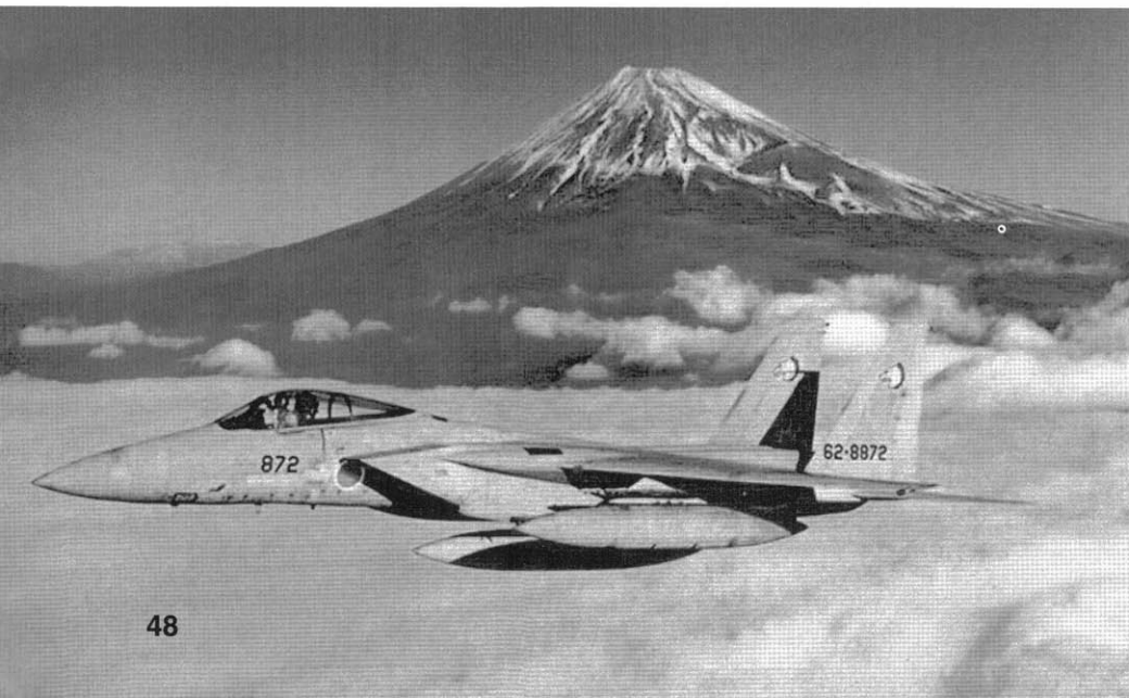
An F-15J (62-8872) of 204 Hikotai , 7 Kokudan flies past Mount Fuji. The Squadron is based at Hyakuri on the main Japanese Island of Honshu. This Eagle is fitted with three 600 gallon fuel tanks and displays the Squadron's eagle's head on all vertical tail surfaces. (JASDF)
