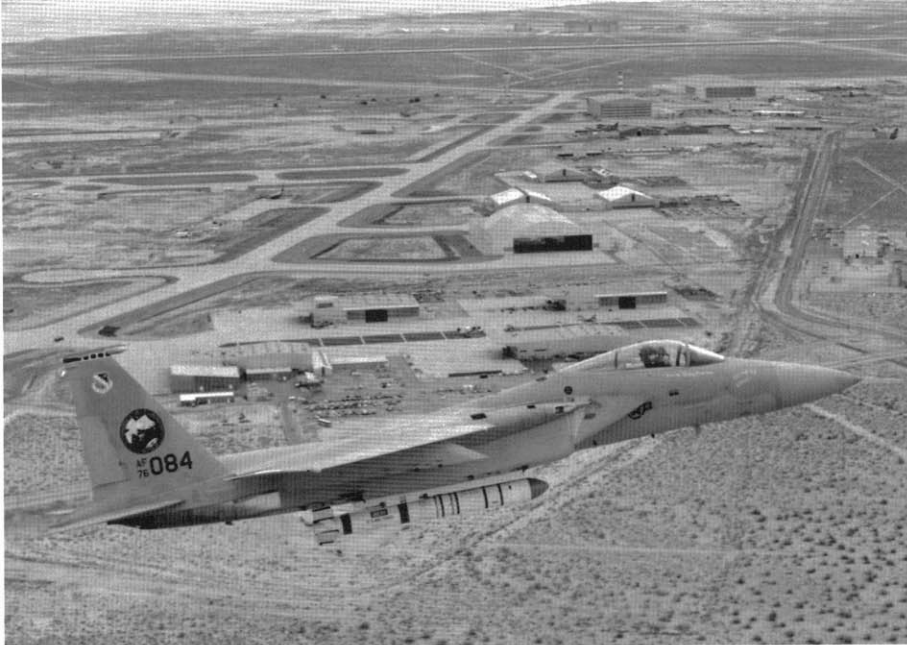
This 6512th TS F-15A-17-MC (76-0084) from Edwards AFB was used to test and launch the Vought ASM-135A Anti-Satellite (ASAT) missile in the mid 1980s. The 17-foot (5.2 m) long, 2650 pound (1202 kg) ASAT missile successfully shot down the Solwind P78-1 satellite on 13 September 1985. The ASM-135A violated a US/Soviet treaty against ASAT weapons and no production was undertaken. (LTV)
