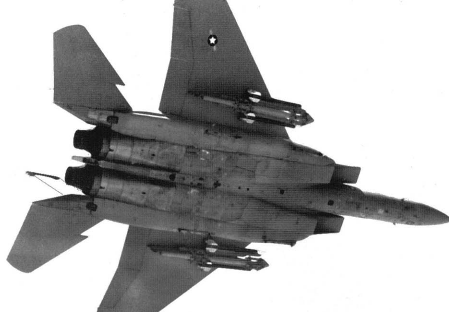
An F-15C banks away from the camera aircraft to reveal the FAST Pack Conformal Fuel Tanks (CFTs) and four practice AIM-9 Sidewinder missiles on the wing pylons. Low-visibility insignia on air superiority F-15s replaced the full color national insignia in the 1980s. The 'turkey feathers' that once covered the engine afterburners' actuators are removed. (USAF)
