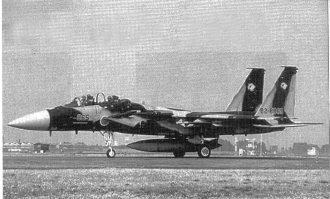
This F-15DJ (82-8865) is one of six two-seat Eagles assigned to the Hiko Kyodo-tai (Aggressor Group) at Nyutabaru. This unit acts as 'enemy' fighters against JASDF aircraft in training exercises. The Hiko Kyodo-tai's F-15DJs have colored bands painted over their Compass Ghost Gray finish; green in the case of 82-8865. (JASDF)
