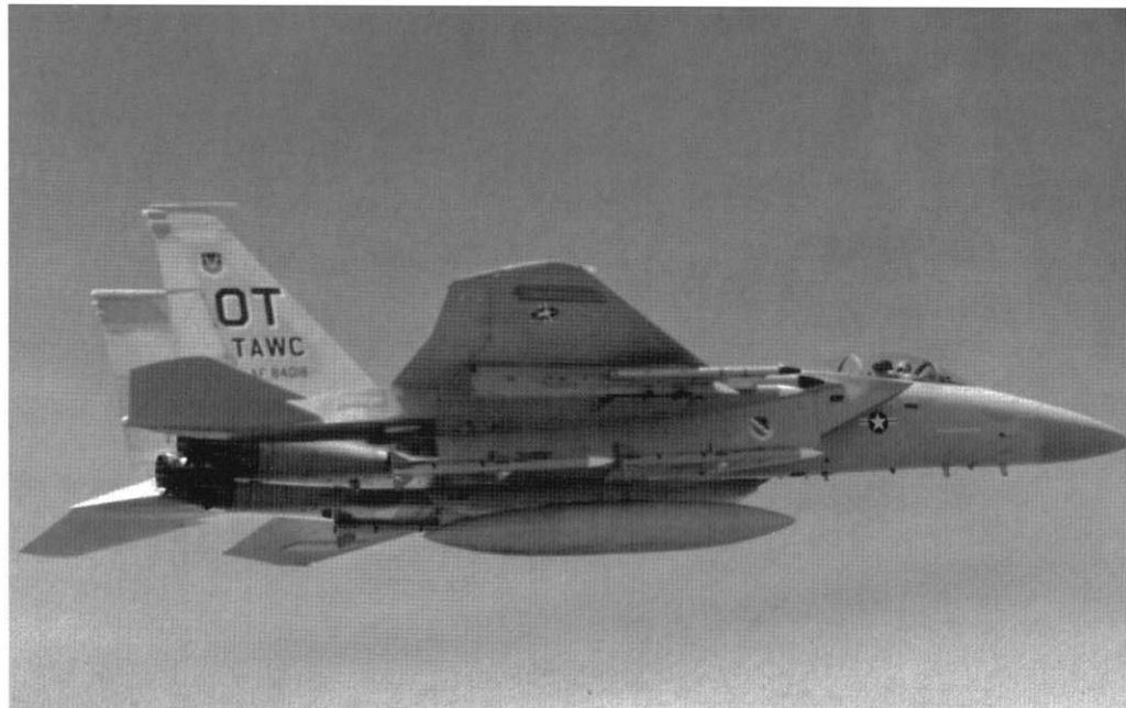
The 4485th TS borrowed F-15C-38-MC (84-0018) from the 59th TFS to test the new AIM-120 AMRAAM air-to-air missile. Cameras for recording missile launches are mounted on orange outer wing fairings. An Air Combat Maneuvering Instrumentation (ACMI) pod is fitted to the Number 8 station on the starboard wing pylon. Data from the ACMI pod evaluates the F-15's performance while firing the AMRAAMs. (USAF)
