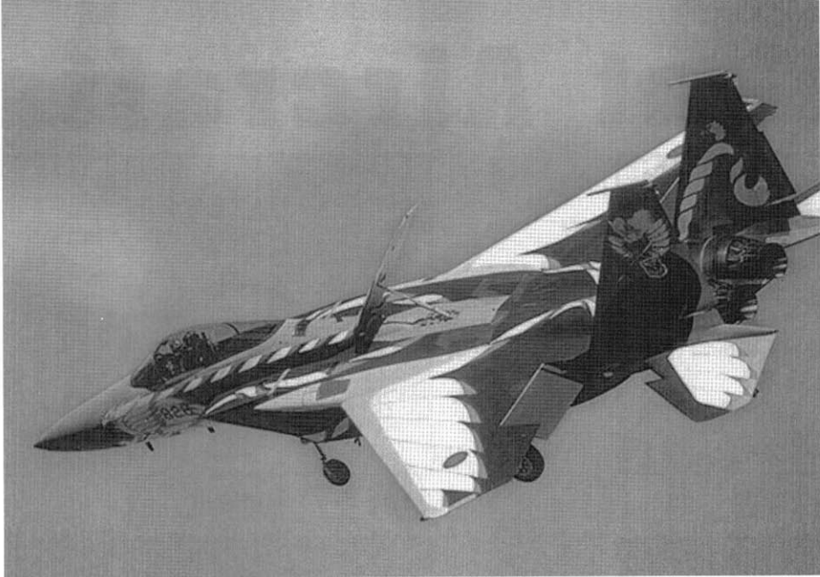
A specially painted 204 Hikotai F-15J (42-8828) prepares to land during an air show in Japan. The landing gear is extended and the speed brake is fully deployed at a 45° angle. The yellow, red, white, and blue eagle scheme celebrated the Squadron's 30th Anniversary in 1991. (JASDF)
