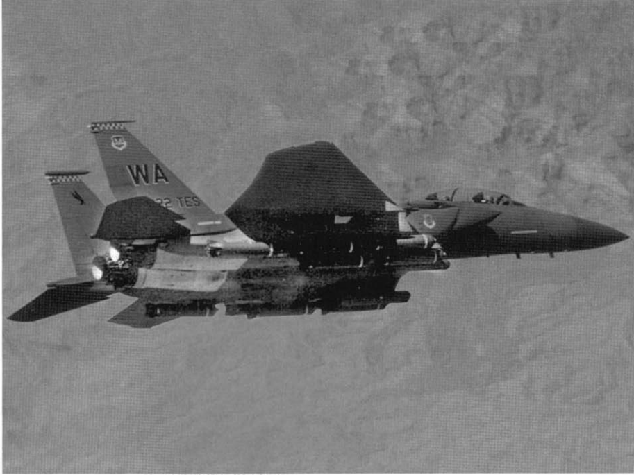
A F-15E from the 422nd Test and Evaluation Squadron (TES), 57th Wing flies a test mission from Nellis AFB, Nevada. The Eagle is fitted with Mk 7 dispensers (Mk 20 Rockeye cluster bomb units) on the CFT stations. The tail band consists of yellow and black checks and the WA tail code and unit designator are black with white shadowing. (USAF)
