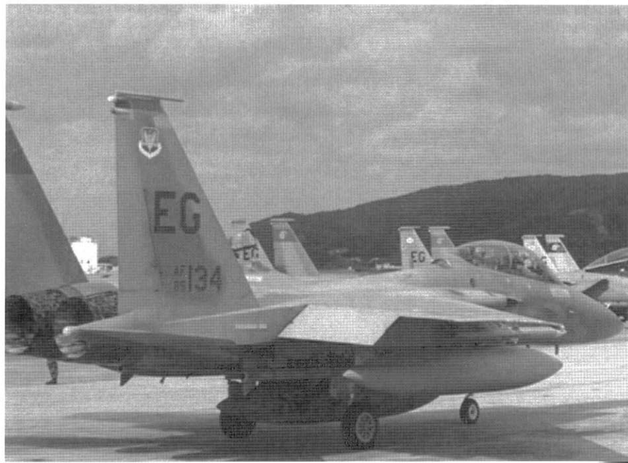
An F-15D-40-MC (85-0134) warms up its engines prior to a training mission at a forward deployed location. The wing flaps are lowered to their maximum 30° setting for pre-flight checks. The flaps are normally lowered for landing and when hydraulic power has bled off after engine shutdown. This Eagle is assigned to the 60th FS, 33rd FW from Eglin AFB and has a red tail band painted above the Air Combat Command (ACC) insignia. (USAF)
