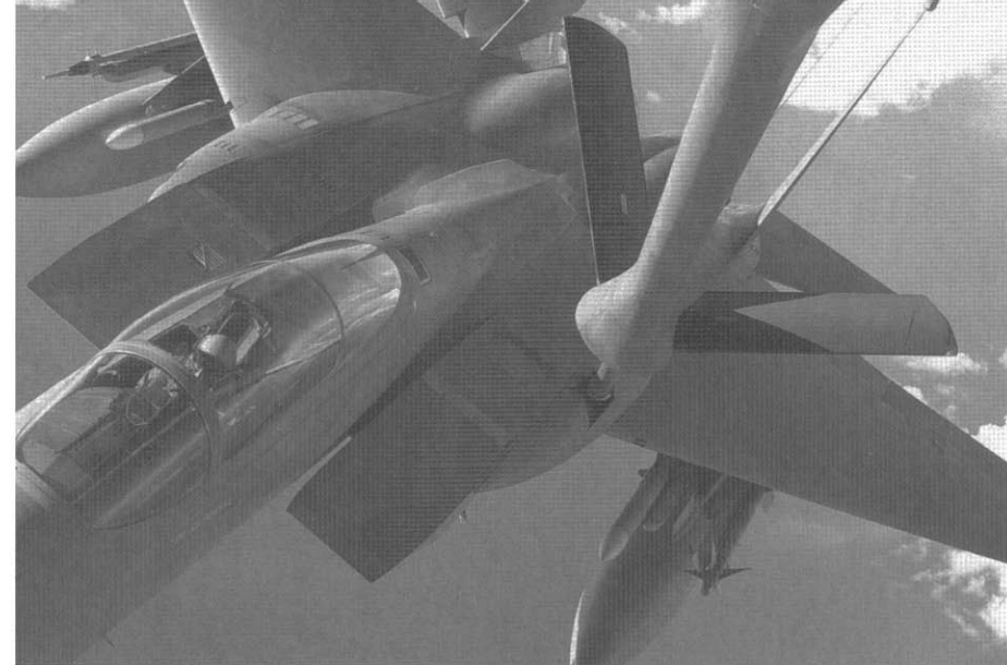
An F-15C receives fuel from a KC-135 tanker aircraft. The boom is 'flown' into the receptacle by the tanker's boom operator, using two controllable vanes on the boom's end. In-flight refueling greatly extends the F-15C's range to where it is limited only by the pilot's endurance. (USAF)
