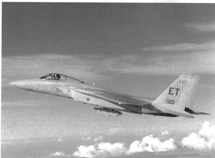
This F-15A-17-MC (76-0101) was assigned to the 3246th Test Wing at Eglin AFB. It carries a centerline mounted Westinghouse/Loral ALQ-131 (Deep) Electronic Countermeasures (ECM) pod during tests in the 1980s. The ECM pod is designed to jam radar signals and give false readings to enemy radar systems. The fin stripe is white with red 'shock' diamonds. (USAF)
