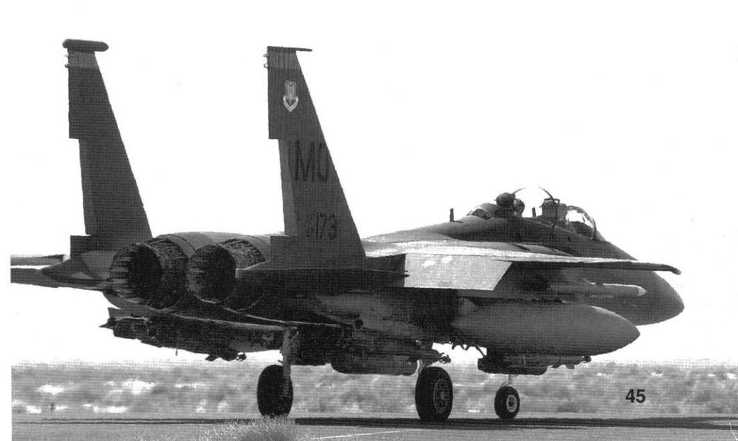
A forward deployed F-15E-43-MC (87-0173) from the 391st FS taxis out to an active runway prior to taking off on a mission over Afghanistan in 2001. This Eagle is armed with 2000 pound GBU-27 laser guided bombs and AIM-120 AMRAAM air-to-air missiles. The tail band is orange with black tiger stripes. The 322nd Air Expeditionary Group controlled the 391st FS during Operation ENDURING FREEDOM. (USAF)
