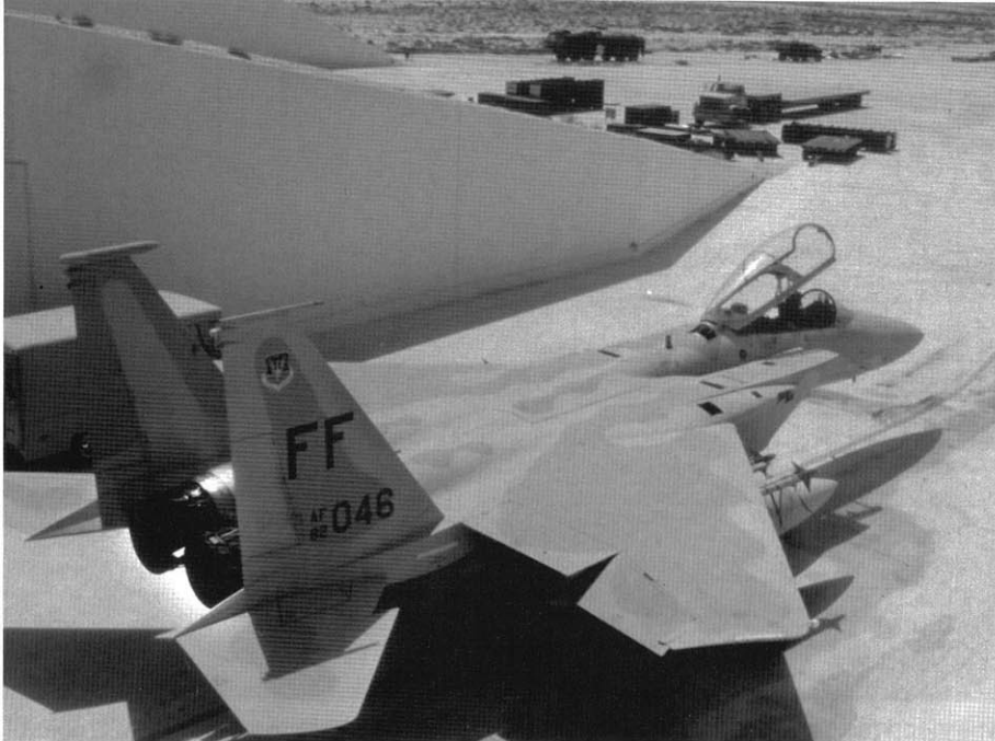
An F-15D-34-MC (82-0046) from the 21st TFS, 1st TFW sits in a revetment at Dhahran, Saudi Arabia in November of 1990. The Squadron deployed from Langley AFB, Virginia for Operation DESERT SHIELD. The aircraft is fitted with AIM-9 Sidewinders and 600 gallon external fuel tanks. MIM-109 Patriot Surface-to-Air Missiles (SAMs) in the background protected the airfield from Iraqi Scud missile attacks. (McDonnell Douglas)
