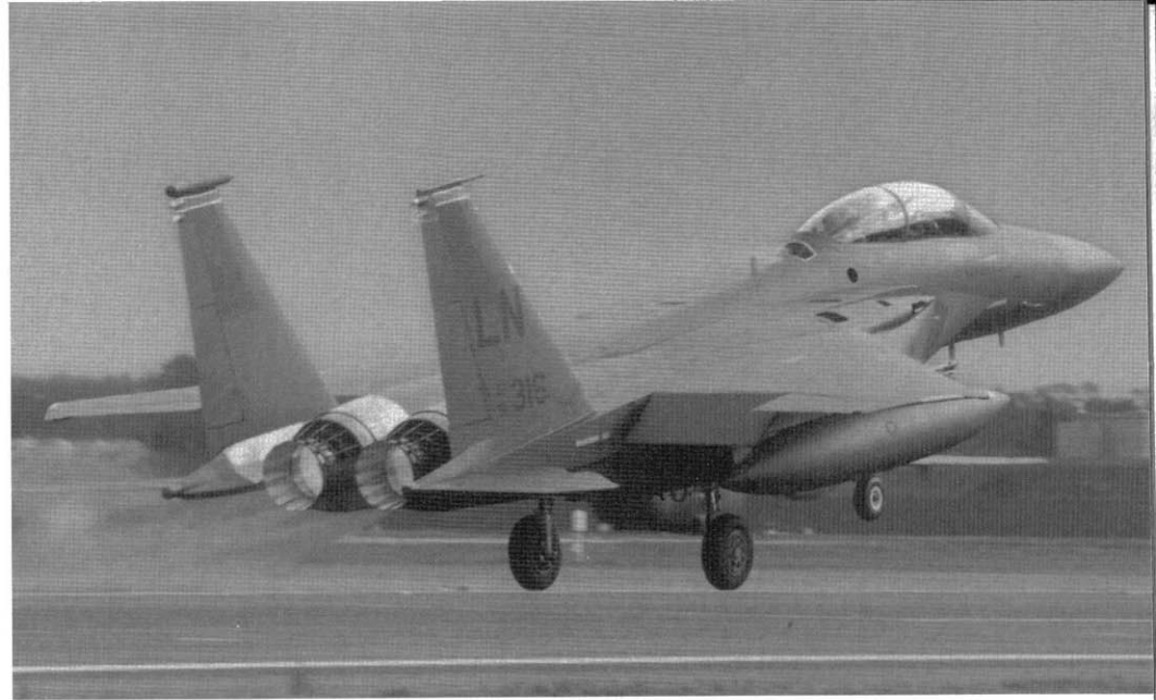
An F-15E (91-0316) from the 494th FS, 48th FW launches from RAF Lakenheath for Central Asia to support Operation ENDURING FREEDOM in late 2001. The Eagle is equipped with three 600 gallon fuel tanks and it carries no external armament. The Squadron's tail band is red outlined in white. The 48th FW is the only F-15E unit based outside the Continental US (CONUS). (USAF)
