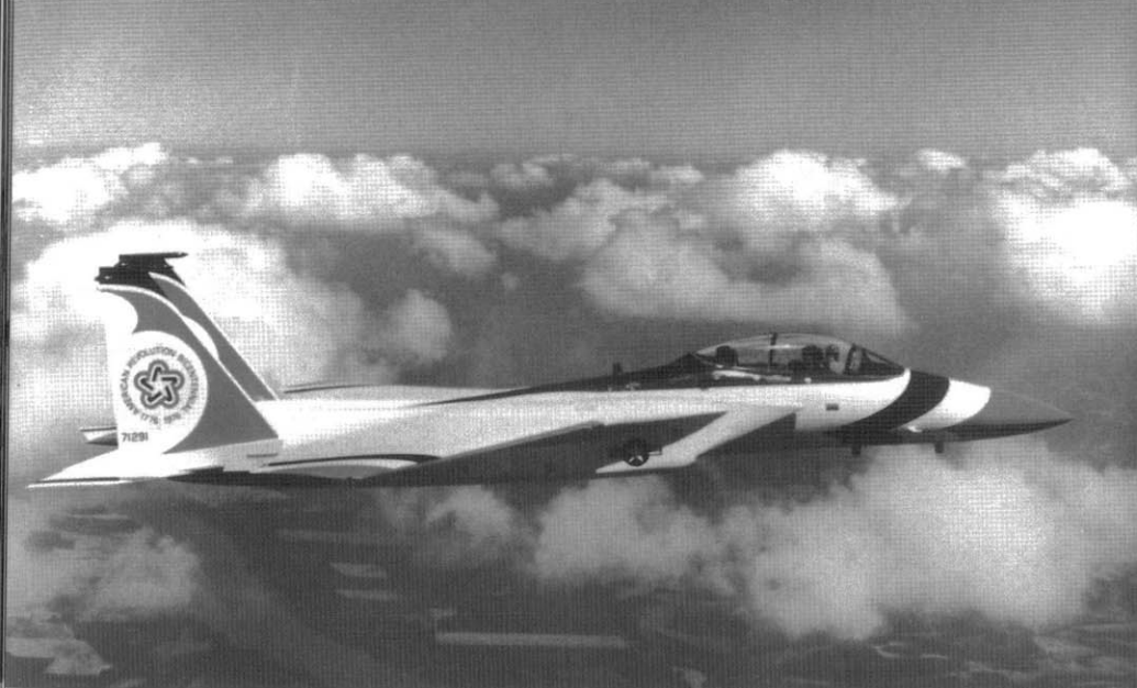
The second F-15B-4-MC (71-291) was painted with the American Revolution Bicentennial emblem on the vertical stabilizer in 1976. The nose, wing tips, and tail surfaces are progressively painted red, white, and blue. This aircraft is not fitted with the 20mm cannon in the starboard wing root, which was normally found on F-15Bs. The Eagle was flown on a world tour to demonstrate its capabilities and drum up sales to foreign countries. (USAF)
