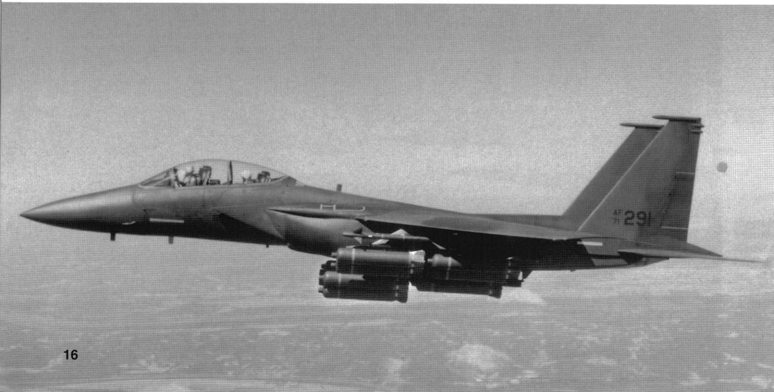
The second F-15B-4-MC (71-291) was painted with the American Revolution Bicentennial emblem on the vertical stabilizer in 1976. The nose, wing tips, and tail surfaces are progressively painted red, white, and blue. This aircraft is not fitted with the 20mm cannon in the starboard wing root, which was normally found on F-15Bs. The Eagle was flown on a world tour to demonstrate its capabilities and drum up sales to foreign countries. (USAF)
