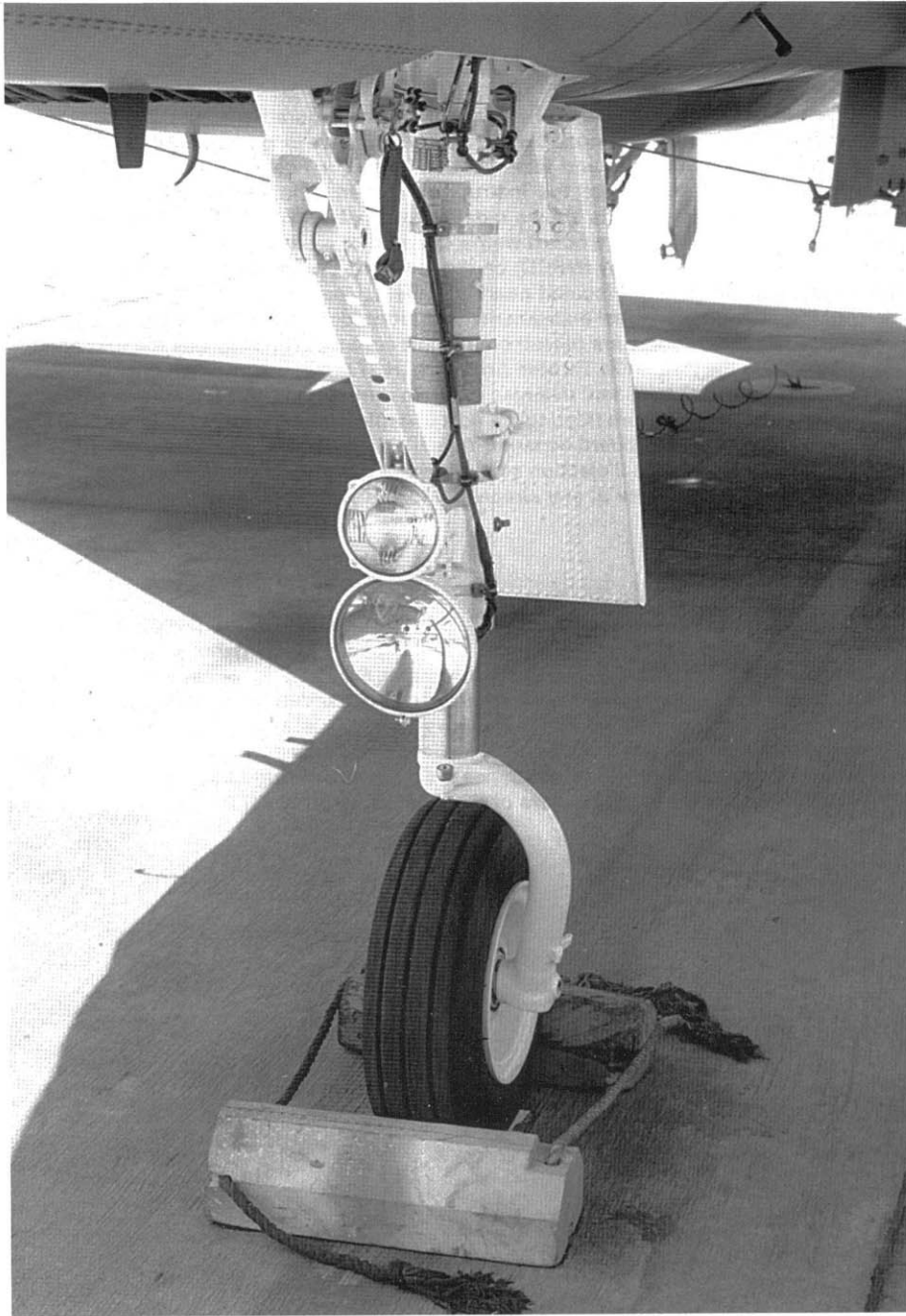
The F-15C nose landing gear consists of a single main strut and wheel. The gear retracts forward into the fuselage. Taxi (upper) and landing (lower) lights are mounted on the strut for use at night and in bad weather conditions. F-15 landing gears, wells, and door inner surfaces are Glossy White (FS17875) to aid in detecting hydraulic leaks. (Lou Drendel)
