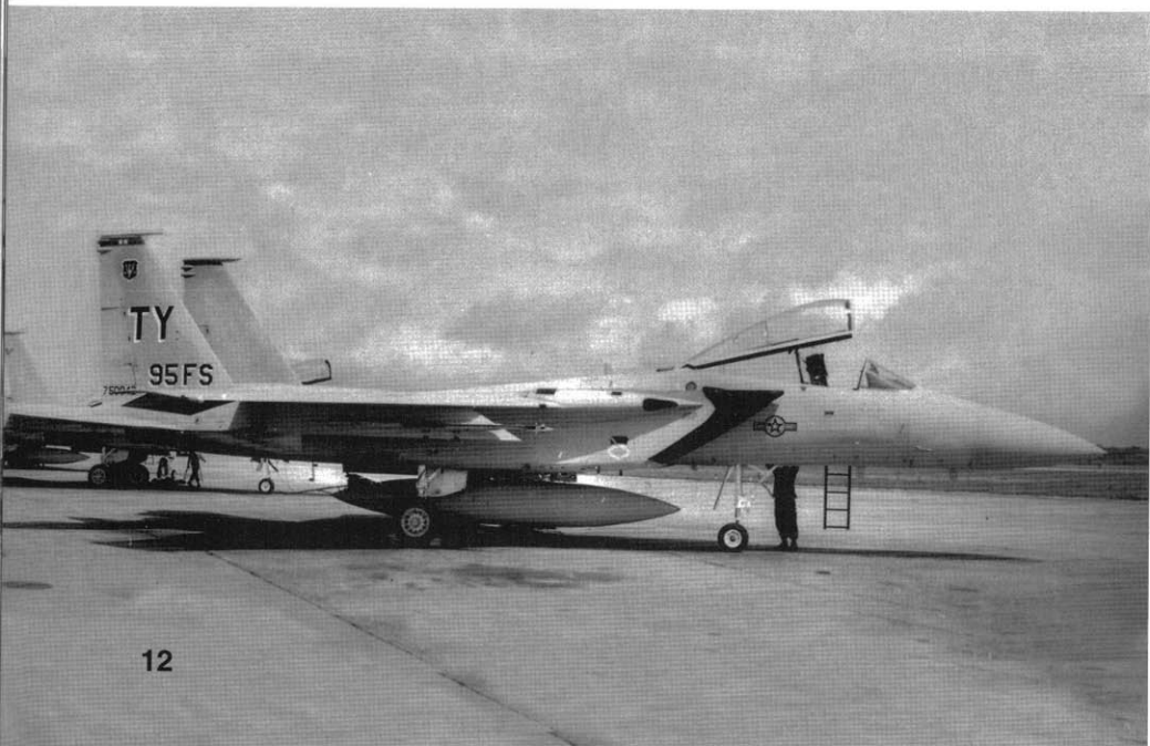
This F-15A-13-MC (75-0042) is marked as the 'flagship' (Squadron Commander's aircraft) of the 95th FS, 325th FW at Tyndall AFB. Two white stars are painted on the blue tail band, above the Air Combat Command (ACC) insignia. The Wing insignia is placed on the starboard intake side. Covers placed over the intake prevent 'FOD' (Foreign Object Damage) from entering the engine intakes. (AI Adcock)
