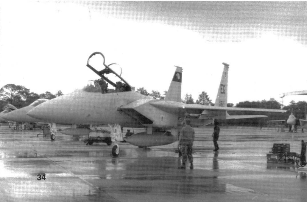
The last F-15D built was this F-15D-41-MC (86-0182), assigned to the 59th FS, 33rd FW. This Eagle is being readied for flight from Eglin and will be flown solo with no 'back seater.' The aircraft is armed with an AIM-9 Sidewinder on the number eight (inner port) wing pylon station. (AI Adcock)
