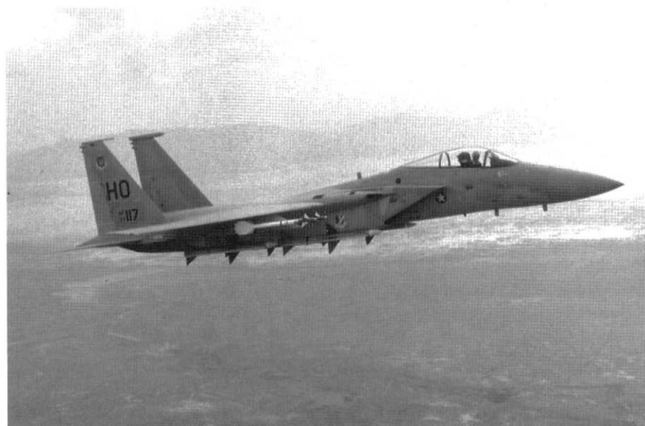
An F-15A-19-MC (77-0117) from the 8th Tactical Fighter Squadron (TFS), 49th Tactical Fighter Wing flies over the White Sands Missile Test Range, New Mexico in 1980. The Wing is based at nearby Holloman AFB. This Eagle is fully armed with four AIM-7 Sparrow and four AIM-9 Sidewinder missiles. The Squadron (now the 8th Fighter Squadron) currently flies the Lockheed F-117A Nighthawk 'stealth fighter.' (USAF)
