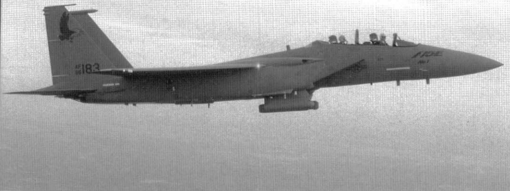
The first F-15E (86-0183) makes a test flight from McDonnell Douglas's St. Louis facility in 1986. The aircraft is fitted with LANTIRN navigation and targeting pods under the engine intakes. This Eagle variant is powered by two Pratt & Whitney F-100 PW-229 low bypass turbofan engines, which each produce over 29,000 pounds of thrust. (McDonnell Douglas)
