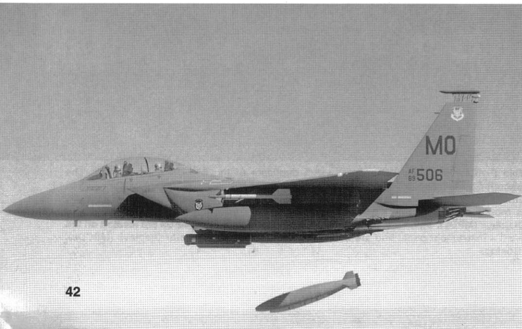
A 391st FS F-15E (89-0506) drops a pair of 2000 pound Mk 84 'iron' bombs during a test flight. The bombs can be accurately placed on the intended target utilizing the LANTIRN navigation and radar targeting pods under the engine inlets. The 391st FS 'Bold Tigers' was the first F-15E squadron deployed to Central Asia during Operation ENDURING FREEDOM in the fall of 2001. (USAF)
