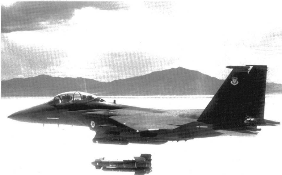
A 550th TFTS F-15E-43-MC (87-0187) drops twelve 500 pound Mk 82 bombs on the Goldwater Test Range in June of 1989. These weapons were released from tangentially mounted pylons fitted to the Conformal Fuel Tanks (CFTs). Markings on the vertical stabilizer indicate this F-15E is the 'flagship' of the 550th Aircraft Maintenance Unit (AMU), which coordinates aircraft maintenance for the 550th TFTS. (McDonnell Douglas)
