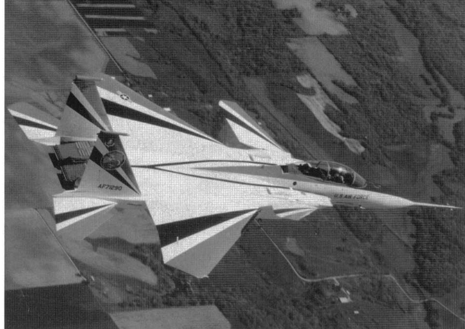
The NF-15B STOL/MTD first flew with the thrust vectoring nozzles on 10 May 1989. Horizontal stabilizers from a McDonnell Douglas F/A-18 Hornet were mounted on this aircraft's engine inlets. These stabilizers served as canards to increase maneuverability. A test instrumentation boom mounted on the F-15B's nose recorded flight data for the test pilot and for engineers on the ground. (McDonnell Douglas)
