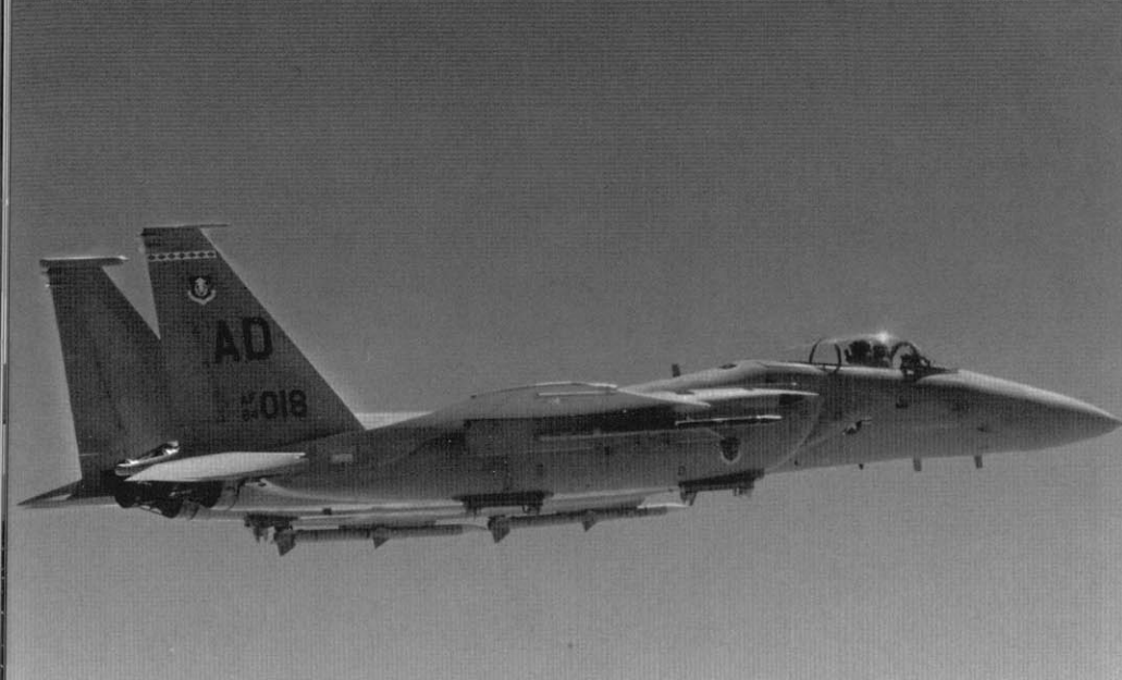
This F-15C-38-MC (AD, 84-0018) flies on a test mission from Eglin AFB. The aircraft is assigned to the 3246th Test Squadron, whose white tail band has red shock diamonds. Two AIM-120 AMRAAM missiles are carried on the port fuselage CFTs, while orange fairings for cameras are mounted on the starboard CFTs. These cameras recorded the missiles' release from the aircraft. (USAF)
