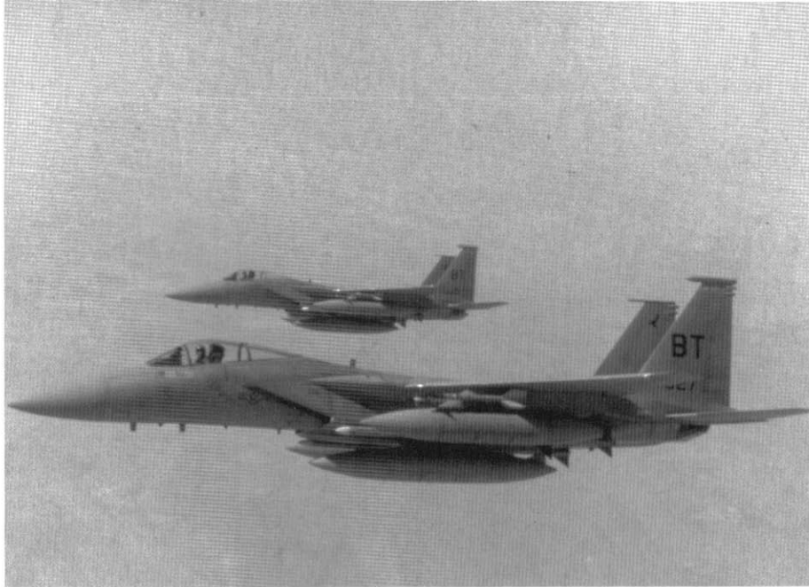
Two 36th TFW F-15C fly a Combat Air Patrol (CAP) over northern Iraq during the 1991 Persian Gulf War. Both Eagles are armed with AIM-7 Sparrows and AIM-9 Sidewinders and carry three 600 gallon (2271.2 L) external fuel tanks. The near aircraft is F-15C-38-MC (84-0027) of the Wing's 53rd TFS. Captain Benjamin Powell flew this Eagle when he shot down an Iraqi MiG-23 and a Mirage F1EQ with AIM-7s on 27 January 1991. (USAF)
