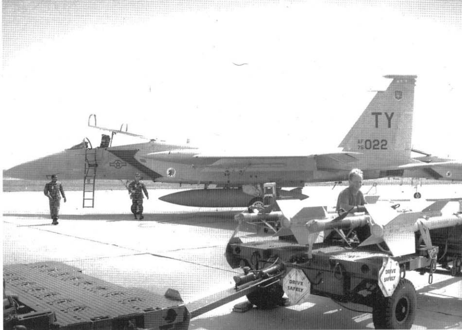
Munitions handlers approach the missile handling trailer to lift and carry the AIM-9 Sidewinder to a waiting 2nd FS F-15A (75-0022). The Squadron insignia appears on the port air intake, whose opening is covered by a tarpaulin. A 600 gallon fuel tank is mounted on the centerline stores pylon. This F-15A will soon be over the Gulf of Mexico stalking a QF-4E Phantom drone. (AI Adcock)
