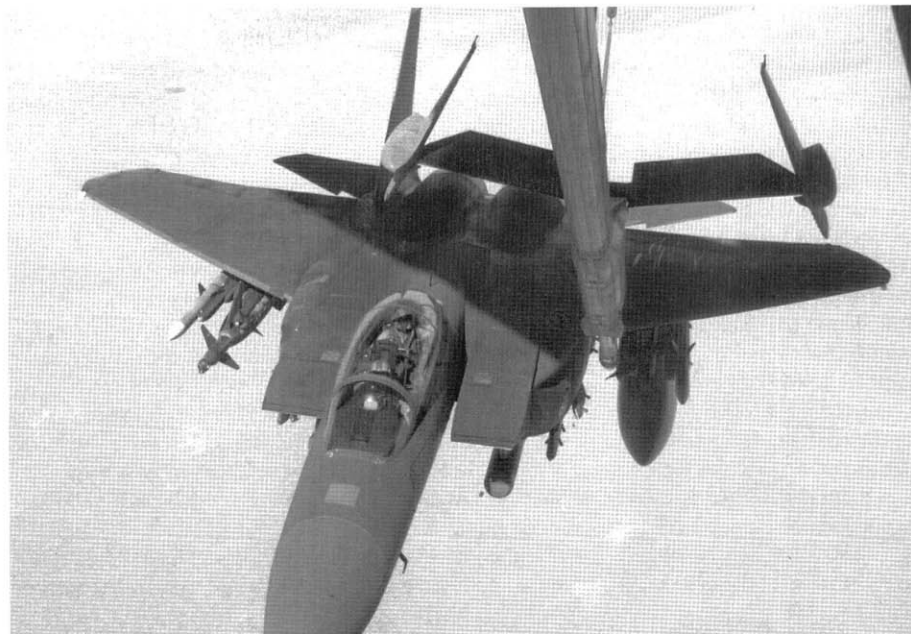
A 391st FS F-15E maneuvers under a McDonnell Douglas KC-10A Extender tanker to take on fuel over Afghanistan during Operation ENDURING FREEDOM. The F-15E is armed with two AIM-120 AMRAAMs and two AIM-9 Sidewinders, with one 2000 pound GBU-10 Paveway laser guided bomb on the starboard wing pylon. A 600 gallon (2271.2 L) fuel tank is fitted to the port wing pylon. (USAF)
