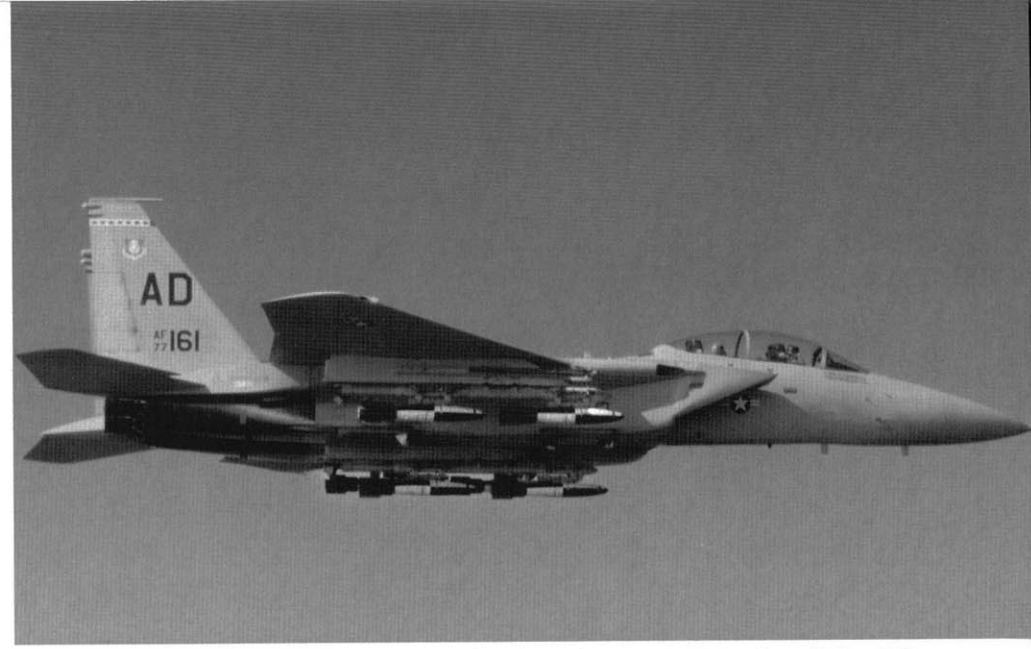
This F-15B-19-MC (77-0161) is assigned to the 3246th Test Wing (TW) at Eglin AFB, Florida. The Wing flies a mix of various aircraft to test and evaluate current and future weapons for the USAF. This Eagle appears to be armed with 500 pound (226.8 kg) Mk 82 bombs painted black and white for photographic purposes. Red shock diamonds are painted on the white tail band. (USAF)
