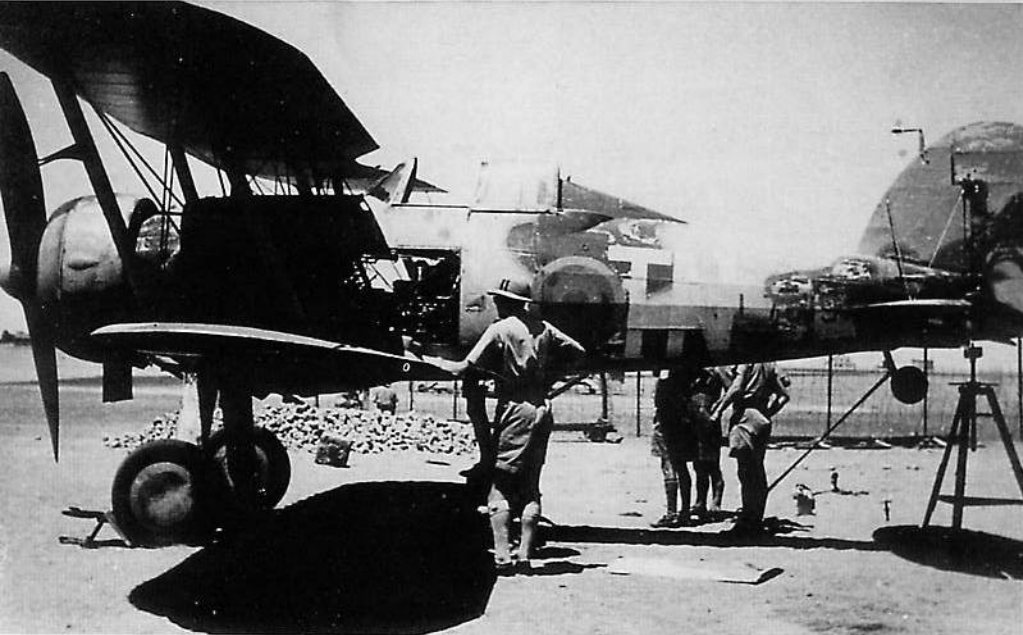
Mechanics rigged this No 112 Squadron Gladiator Mk I (L7619) for maintenance in Sudan in early 1941. The fuselage side panels were removed for easy access to interior compartments. Exposure to constant wind and blowing sand took its toll on the hastily applied camouflage finish. (RAF Museum)
