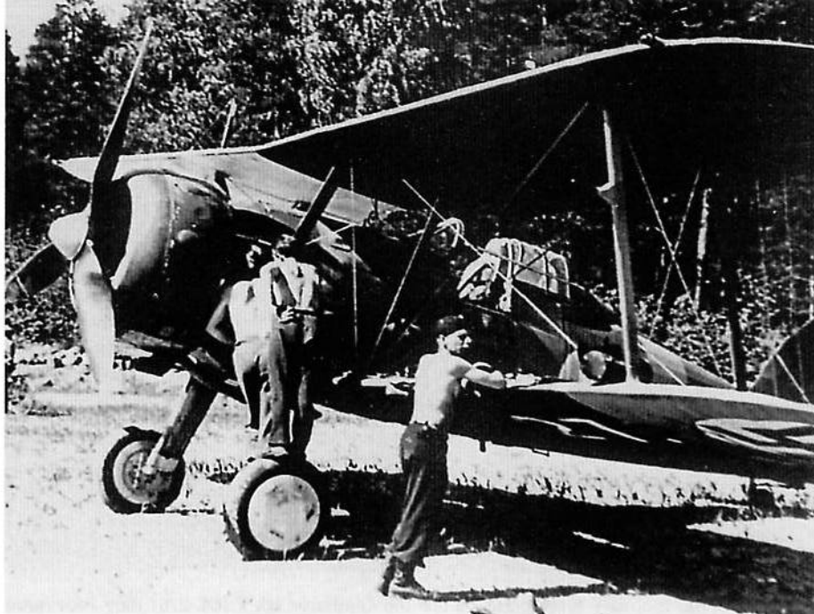
Ground crews attend to a Gladiator II (GL-272) being operated from a sandy beach on Finland's Lake Hoytiainen in June of 1941. The lower wing undersurface tips and aft fuselage band were Yellow (FS33538) for Axis aircraft operating on the Eastern Front. Yellow was painted over the last digit of the lower wing serial number. (Eino Ritaranta)
