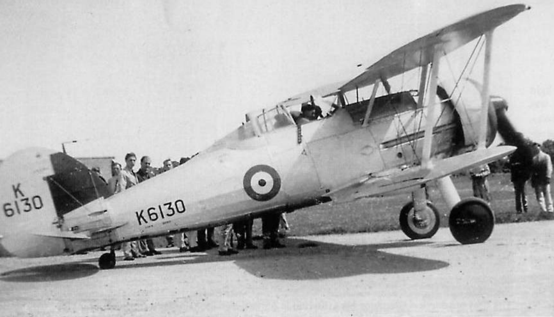
K6130 prepares for its next flight while other pilots and ground crews stand beside its port fuselage. Pre-World War Two RAF aircraft were overall Aluminum, with black serial numbers. The .303 caliber fuselage machine guns were removed, but the weapons were retained under the wings. (A.J. Jackson Collection)
