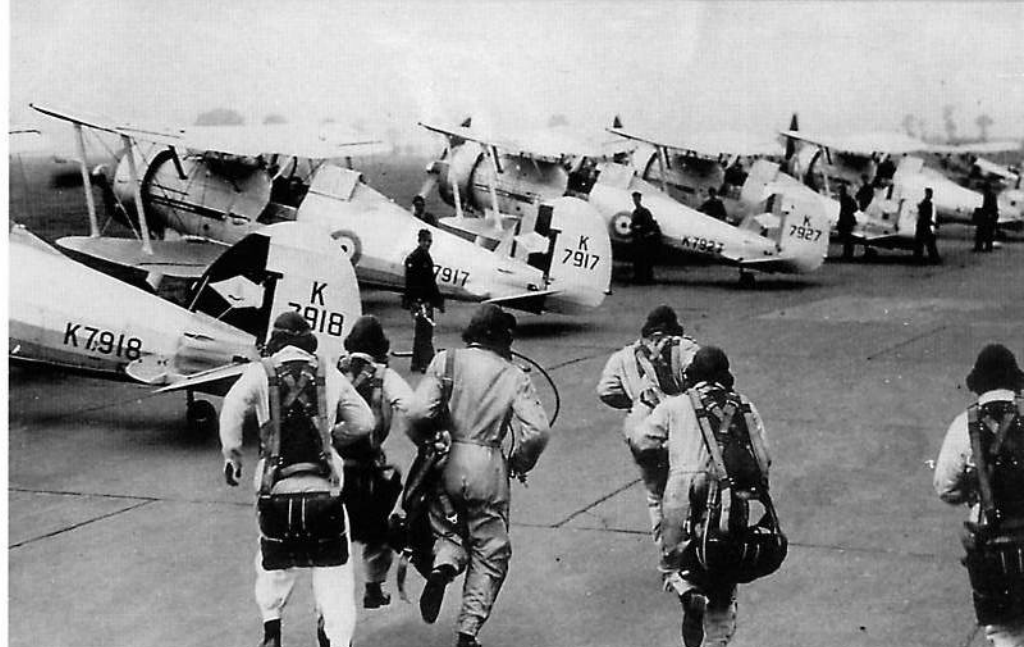
No 54 Squadron pilots race to their Gladiators during an exercise in 1938. Their seat parachutes were later found to be cumbersome and were left in the cockpit or on the wing for the pilots to put on before flight. The parachute's pack nestled into the seat pan and acted as a cushion. These Gladiators display a variety of flight leader fin markings.
