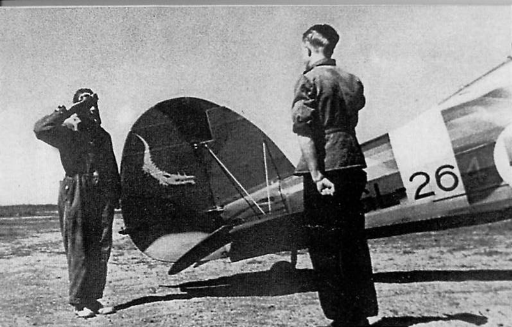
A pilot (left) salutes his mechanic before entering his Gladiator Mk II (GL-264) at Hervas on 28 June 1942. The fighter was assigned to 2nd Flight, LeLv 16, whose alligator insignia is painted on the rudder. By 1942, Finnish Gladiators were repainted Olive Green (FS34096) and black, with Light Blue (FS35414) undersurfaces. (Eino Ritaranta)
