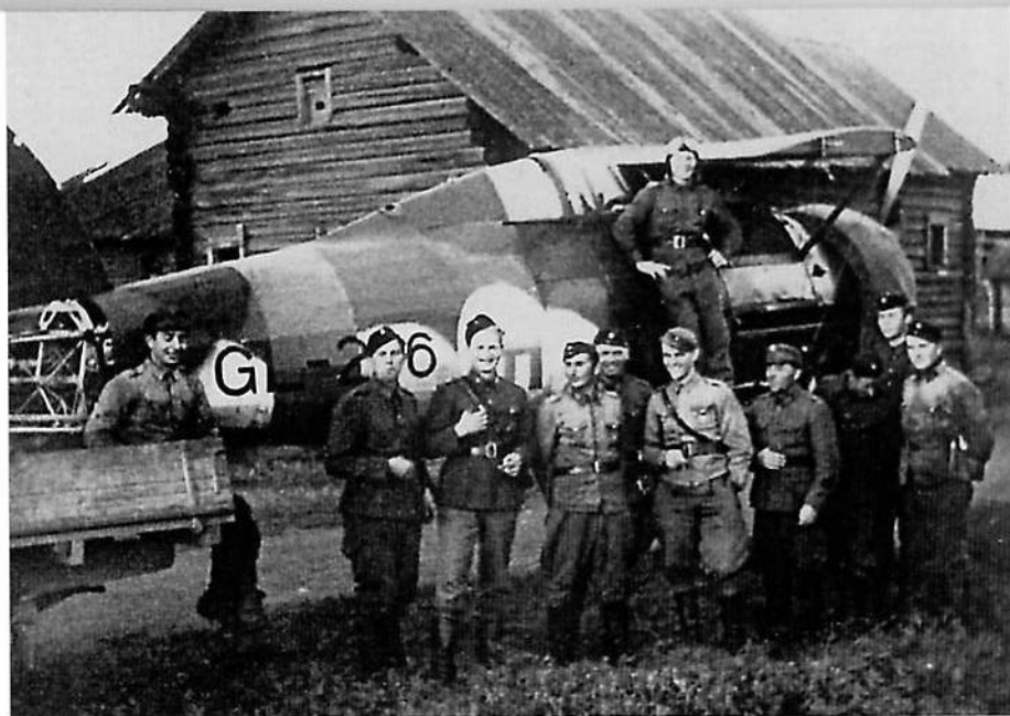
An Ilmavoimat recovery team pose before the Gladiator Mk II (GL-276) they recovered from Sidorova, Russia. The aircraft force landed there after it had engine trouble on 4 September 1943. The pilot, Sgt O. Kuuluvainen, was unhurt in the landing. The recovery team removed the Gladiator's outer wings before towing the aircraft towards the Finnish rear area. (Eino Ritaranta)
