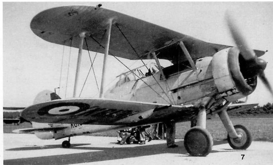
The second Gladiator Mk I (K6130) warms up its engine prior to a check flight. The RAF used this aircraft to qualify the first service Gladiator pilots before assigning it to No 72 Squadron – the first operational unit. A red propeller spinner, wheel discs, and vertical and horizontal stabilizers indicated 'A' Flight Leader's aircraft. The oil cooler mat is mounted on the upper fuselage, directly under the upper wing. (A.J. Jackson Collection)
