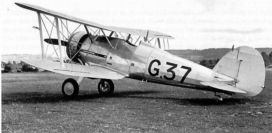
The Gloster SS.37 prototype (G.37) was rolled out of the Gloster factory at Hucclecote, England in September of 1934. This aircraft retained several features from the earlier Gauntlet, including an open cockpit and spatted tail wheel. The SS37 was originally powered by a 530 hp Bristol Mercury IV radial engine. (Via Richard Riding)
