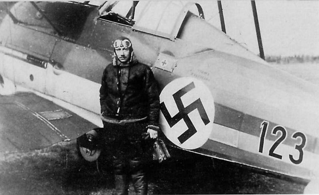
A Latvian pilot poses with his Gladiator Mk I (123). This aircraft was the tenth aircraft Latvia ordered from Gloster. The black serial number is outlined white in a style similar to fuselage numbers painted on Luftwaffe aircraft in World War Two. Just over the pilot's left shoulder is the first aid compartment, which was in a different location from Gladiators flown by other operators. (P.E. Branke via Robert J. Ruffle)
