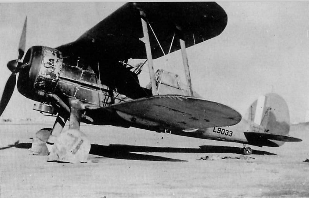
This well-worn Gladiator II (L9033) was assigned to No 5 Squadron, REAF from 1940 until 1942. It is equipped with a Vokes air filter under the engine cowling, which kept sand out of the carburetor. Machine guns are not fitted to the lower wing pods. The aircraft were camouflaged in Dark Earth (FS30118) and Light Earth (FS30257), with Aluminum undersurfaces. (A.J. Jackson Collection)
