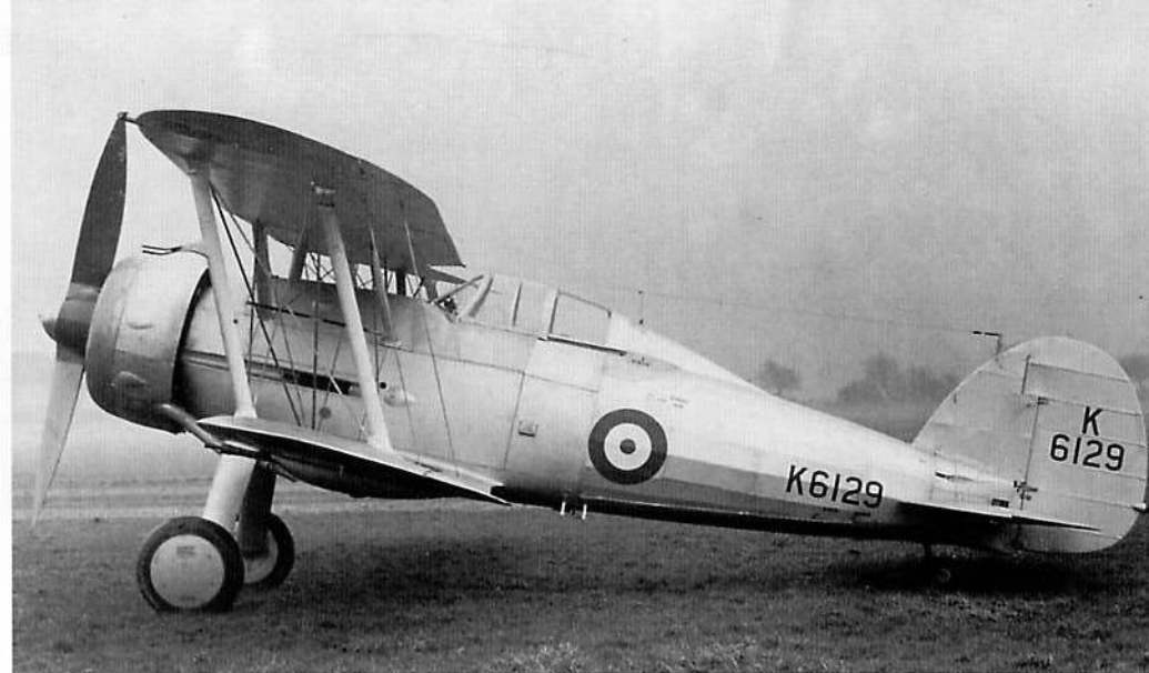
The first production Gladiator Mk I (K6129) is parked outside Gloster's Hucclecote factory. It was powered by an 830 HP Mercury radial engine turning a Watts propeller. Production Gladiators differed from the SS.37 prototype in having a more powerful engine, an enclosed cockpit, and an uncovered tailwheel. The RAF accepted K6129 into service on 16 February 1936. (Via Richard Riding)
