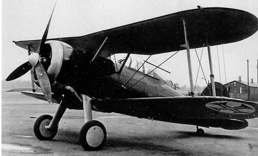
One of Portugal's 15 Gladiator Mk IIs (G5) sits on the ramp at Martlesham Heath, England in 1939. A thermometer was taped to the rear port interplane strut for the aircraft's pre-delivery test flights. Portuguese Gladiators had Dark Green (FS34097) upper surfaces and Light Gray (FS36373) undersurfaces. After test flights in Britain, the aircraft were disassembled and shipped to Portugal, where they were reassembled. (RAF Museum)
