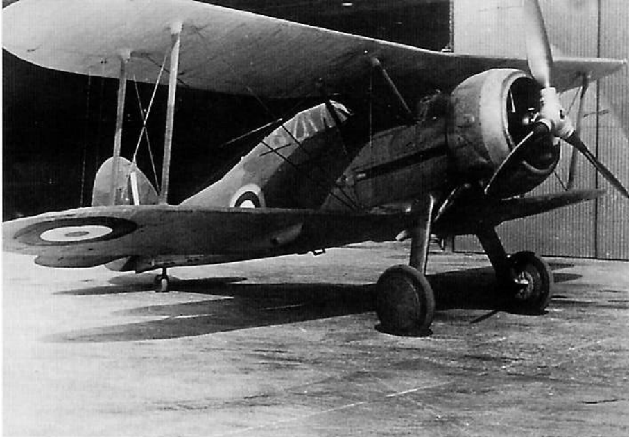
Propeller manufacturer Rotol used this Gladiator Mk I (believed to be K8040) for tests in 1939. The firm evaluated paint and wood blade coverings on a variable pitch propeller. JABLO painted on the uppermost propeller blade tip referred to the blade-covering supplier. (A.J. Jackson Collection)
