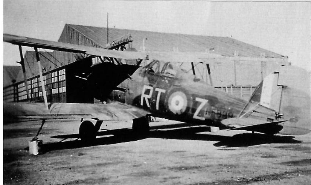
Another Gladiator assigned to No 112 Squadron was this Mk II (RT-Z/N5853). The RAF hastily camouflaged this and other Gladiators in Egypt after war broke out. Cans filled with either sand or concrete were used as mooring weights on this aircraft. The control column was fastened fully back using the pilot's harness, resulting in the up elevator on this Gladiator. (D.M. Hannah via Ray Sturtivant)
