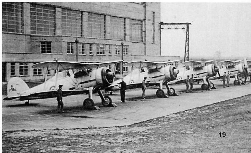
Gladiator Mk Is assigned to No 73 Squadron warm up their engines at RAF Digby in 1938. Mechanics stand near each aircraft to ensure proper engine start before pulling the wheel chocks. Pilots then taxied their Gladiators off the concrete apron onto the grass airfield for takeoff. No 73 was one of five UK-based Gladiator squadrons in RAF service by the fall of 1938. (RAF Digby)
