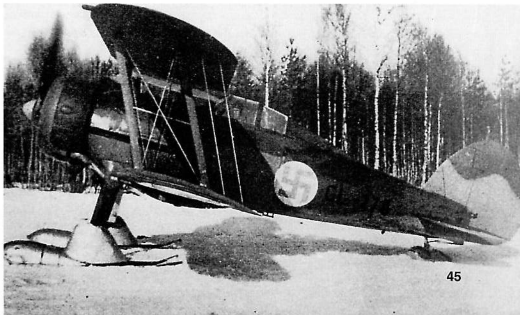
Capt A. Maunula warms up prior to a mission in a Gladiator II (GL-270) of 1 Flight, LLv 12 ( Lentolaivue ; Flying Squadron) at Karhusjarvi in March of 1940. There was no difficulty operating Gladiators on skis. The camouflage was standard RAF green/brown with the undersides of both port wings in black and the starboard wings in white. (Eino Ritaranta)
