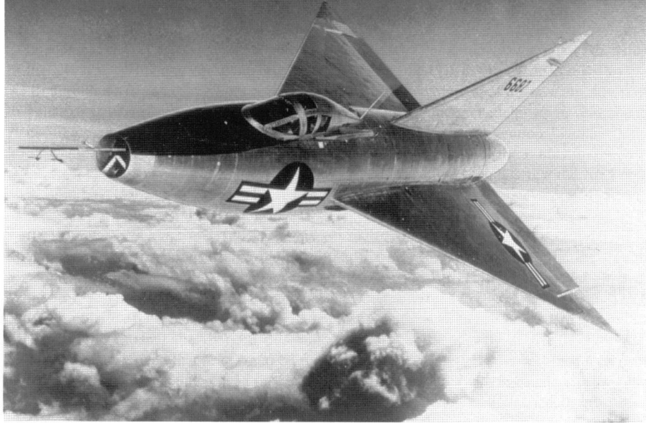
Although severely underpowered, the Convair XP-92A prototype was the world's first true delta wing aircraft, making its first flight 18 September 1948. (AFFTC)
