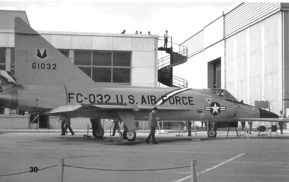
A 32nd FIS F-102A-55 on the ramp during the 1965 Paris Air Show. The 32nd FIS went operational in the F-102A in November 1960. Based at Soesterburg, Netherlands, the 32nd, although assigned to the 86th Fighter Wing in USAFE, was under the operational control of the Royal Netherlands Air Force. The "Case X" wingtips can be clearly seen. (J. Magendie)
