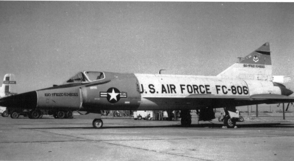
(Below) A YF-102C on the ramp at Sheppard AFB, Texas, in 1955. Two YF-102Cs were modified from F-102As as engineering testbeds for a proposed version of the Delta Dagger intended as a transition to the F-106. This YF-102C (serial 53-1806) was painted overall Aircraft Grey with DayGlo Red nose, wings, and tail surfaces. (Merle Olmsted)
