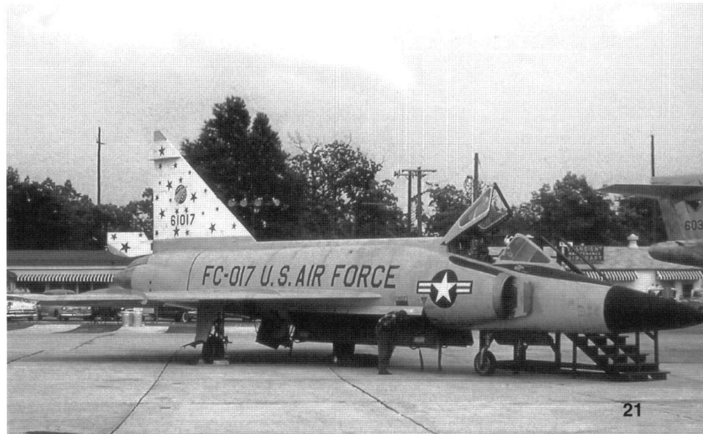
(Below) A 48th FIS F-102A-55 on the ramp at Langley AFB, Virginia, in May 1960. The 48th FIS guarded both Tactical Air Command Headquarters at Langley and U.S. Navy installations in the Norfolk, Virginia, area. The gloss Aircraft Grey (FS 16473) paint shows signs of weathering. The tail is white with blue stars. (Ron Picciani Collection)
