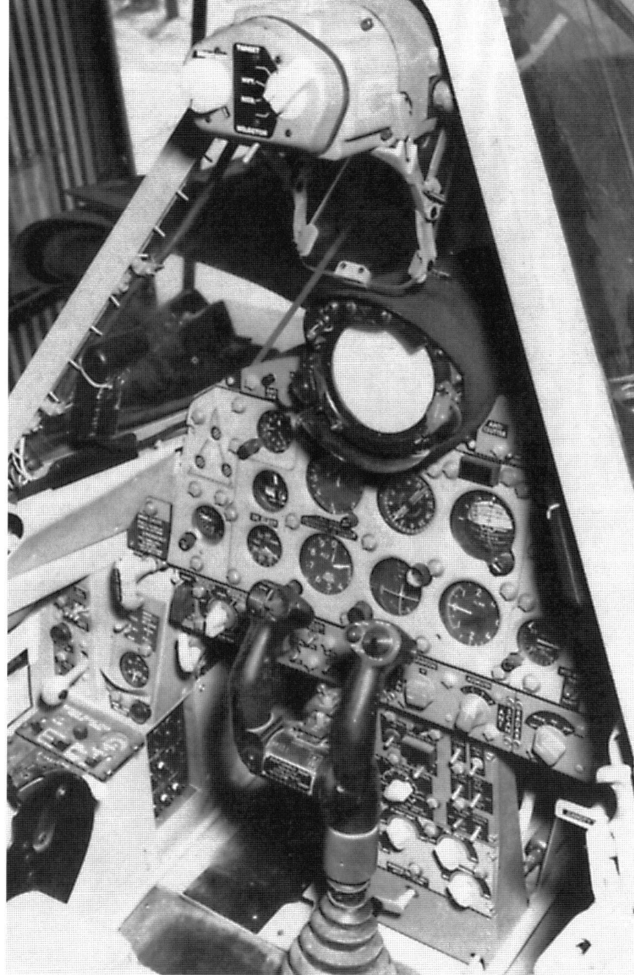
(Above and Right) Cockpit of the F-102A Delta Dagger. The cockpit was painted Light Grey (FS 36473) with Black consoles. (USAF)
