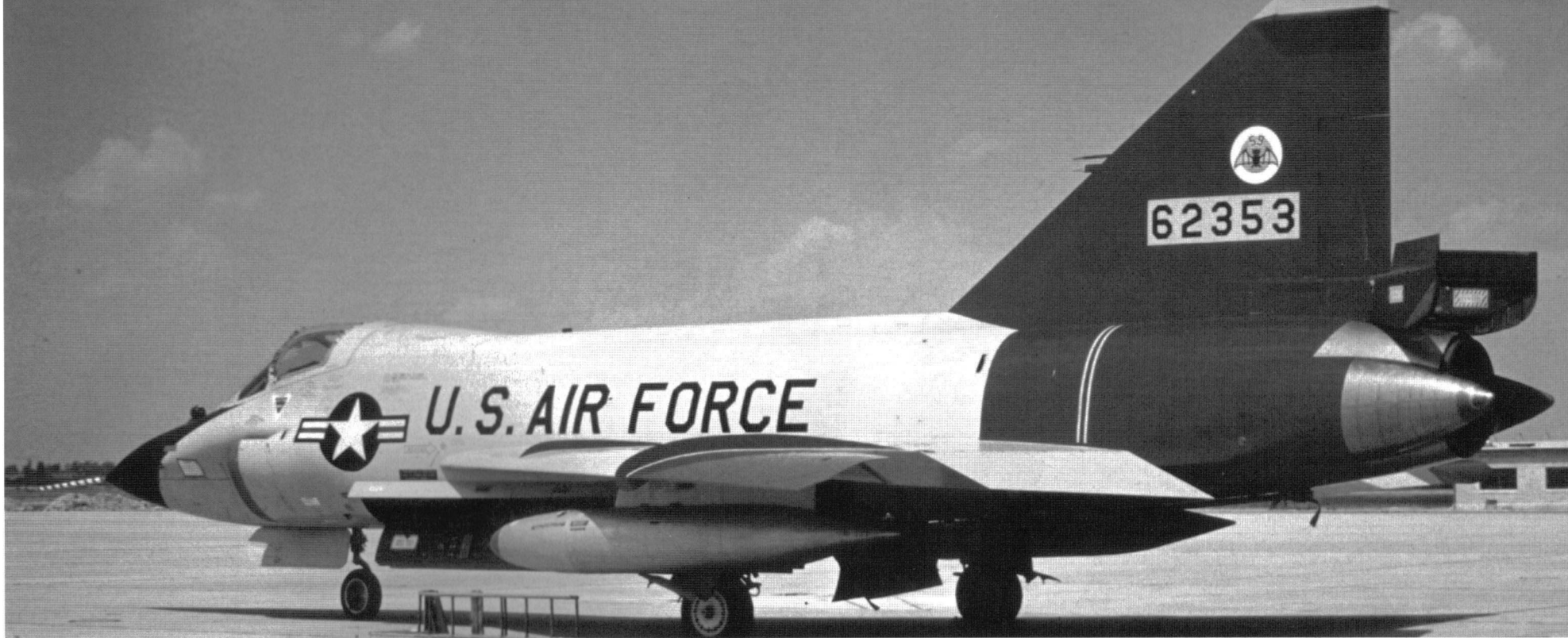
(Above) A 59th FIS TF-102A-41 on the ramp at Andrews AFB during a visit in June 1965. As with the F-102A, the TF-102A had the "Case XX" wing with cambered wingtips added. The 59th FIS was based at Goose Bay, Labrador, and flew the F/TF-102A from May 1960 to December 1966. (Richard Sullivan)
