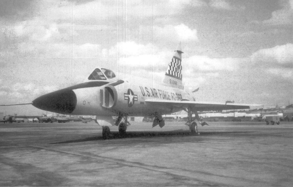
An F-102A-41 from the 16th FIS ready to roll on the flight-line at Naha AB, Okinawa, in 1960. The 16th FIS' Delta Daggers were some of the most colorful, having black-and-white checked tails with blue bands and wing fences. The F-102As from the 16th were transferred to the Hawaii Air National Guard in 1964. (USAF)
