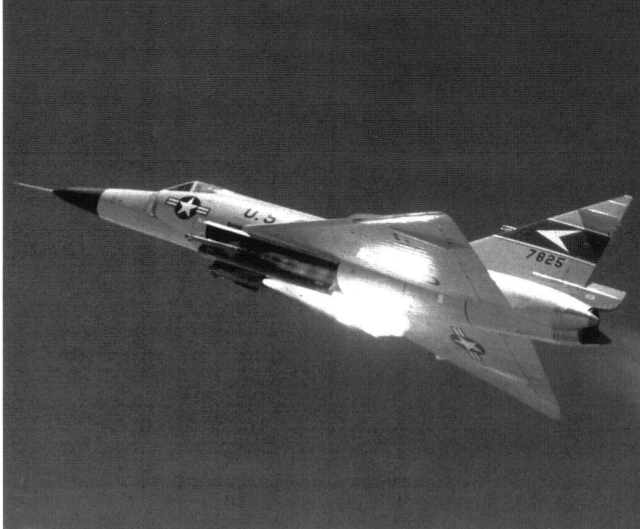
(Above and Below) An F-102A from the 329th FIS fires a volley of AIM-4A radar homing missiles at a target drone over the California high desert range. Normal armament for combat operational F-102As was three AIM-4A radar homing missiles in the forward missile bay, and three AIM-4C infrared heat seeking missiles in the aft missile bay. (Convair)
