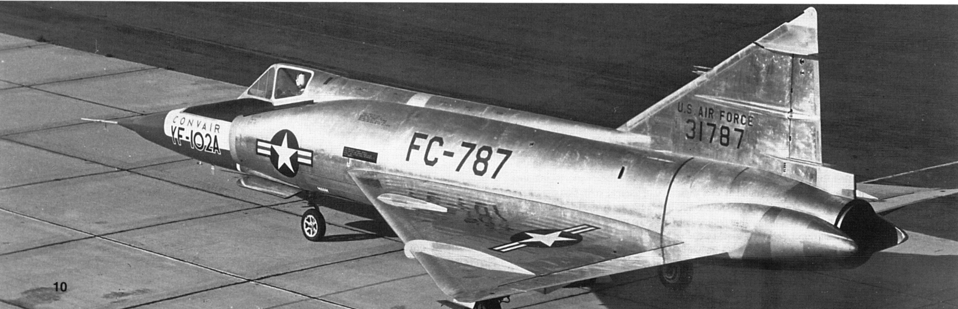
(Below) The YF-102A taxis to the active runway at Lindbergh Field in San Diego. The YF-102A was much different from the earlier YF-102 in having an area-ruled fuselage, commonly called a "wasp waist." (via Robert F. Dorr)
