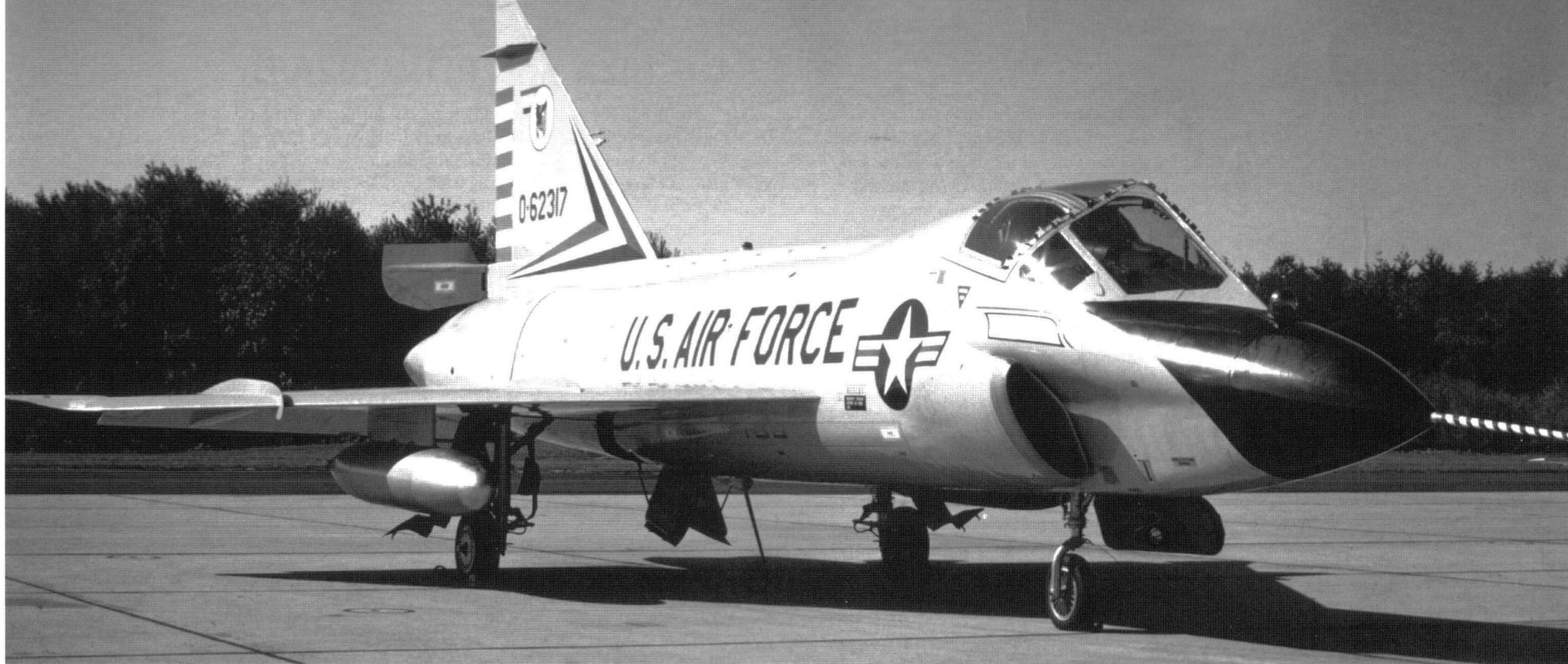
A TF-102A-35 from the Air Defense Weapons Center at Tyndall AFB, Florida in 1968. The ADWC was charged with developing weapons systems, improvements, and tactics for all aircraft types with an air defense mission. The vortex generators that eliminated the
