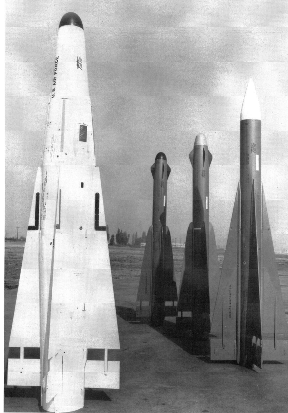
The family of Hughes Falcon missiles. The white missile is the Hughes AIM-26 Super Falcon, which could have either a conventional or nuclear warhead with a 1.5 kiloton yield. Other missiles are AIM-4 Falcons with various seeker heads installed, including radar guided and infra-red homing. (Hughes)
