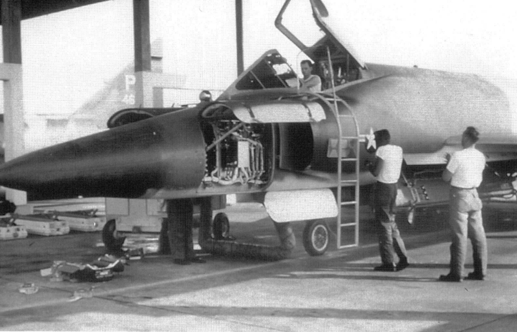
Detachment 5 ground crew perform maintenance on the MG-10 fire control system of a 509th FIS F-102A at Bien Hoa AB, South Vietnam, in April 1968. The F-102 deployments to Southeast Asia were part of Operation CANDY MACHINE, which lasted until September 1968. (E. John Raboin)
