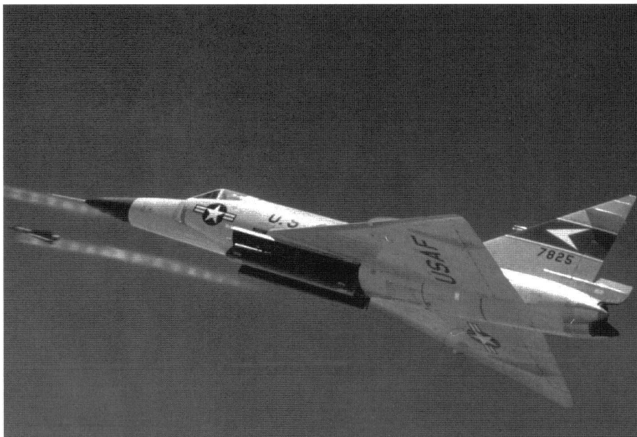
(Above and Below) An F-102A from the 329th FIS fires a volley of AIM-4A radar homing missiles at a target drone over the California high desert range. Normal armament for combat operational F-102As was three AIM-4A radar homing missiles in the forward missile bay, and three AIM-4C infrared heat seeking missiles in the aft missile bay. (Convair)
