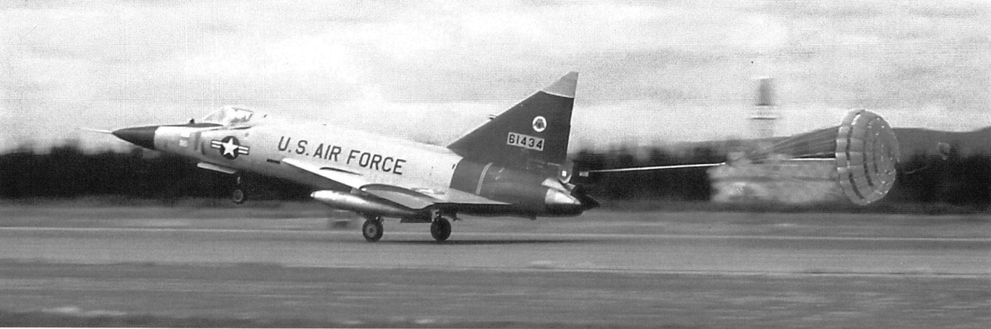
The pilot of this 59th FIS F-102A-80 pops the chute as he touches down at Goose Bay, Labrador, in 1965. Braking parachutes were necessary to slow the F-102 since the airplane did not have landing flaps. Aerodynamic braking was performed by the pilot holding the
