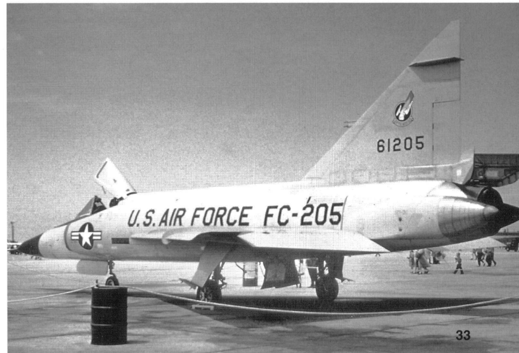
(Right) A 71st FIS F-102A-65 on the ramp at Langley AFB, Virginia, during an air show in 1959. The "Case X" wing with its distinctive upturned tip can be seen. The 71st FIS was based at Selfridge AFB, Michigan. (J. Anderson)
