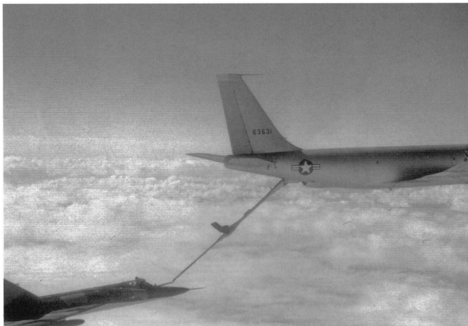
An 82nd FIS F-102A receives fuel from a SAC KC-135A tanker via the fuel probe that was temporarily installed on 82nd FIS Delta Daggers for the trans-Pacific flight to their new home at Naha AB, Okinawa, in 1966. (USAF)
