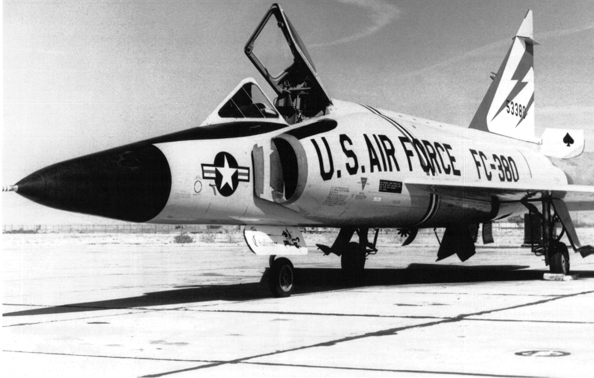
“The Challenger,” an F-102A-45 assigned to the 327th FIS commander at George AFB in 1958. Convair added intake splitter plates to counter a fuselage buzz that was inherent to the early F-102As. The “Ace of Spades” marking on the dive brake doors indicated a flight
