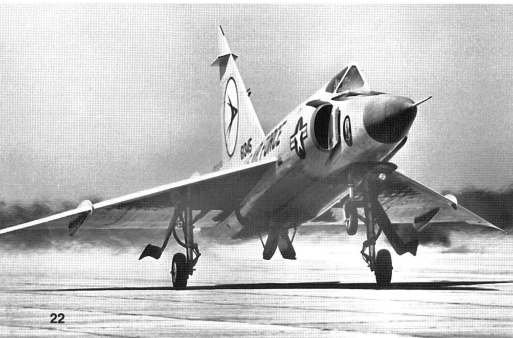
A 318th FIS F-102A-75 in full afterburner scrambles from McChord AFB, Washington, in summer 1958. In afterburner the Pratt & Whitney J57-P-23 engine could produce over 16,000 pounds of thrust. The 318th FIS took over the mission at McChord when the 317th FIS was transferred to Alaska. (USAF)
