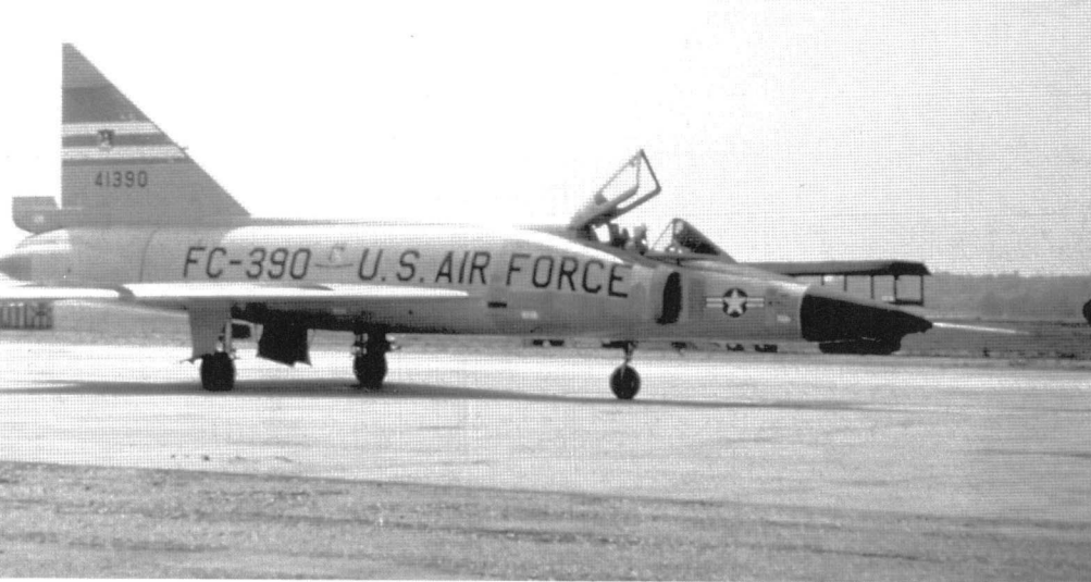
This F-102A-30 is assigned to the Armament Development and Test Center at Eglin AFB, Florida. All new weapons and fire control systems were tested at Eglin's test center, including the MG-10 system and AIM-26 Super Falcon carried by the F-102. Nose, and wing bands are DayGlo Orange, while the tail bands are DayGlo Orange and White. (Author's collection)
