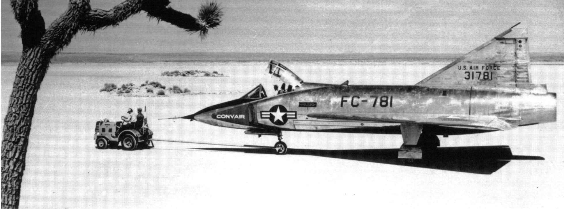
The fifth YF-102 is towed to the flight line at Edward AFB in spring 1954. The fuselage has been extended and greatly enlarged through the tailpipe. The internal weapons bay doors
