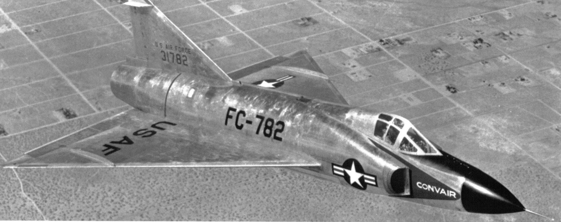
(Above) The sixth YF-102 prototype in flight over Southern California in spring 1954. This YF-102 was the first to have a fiberglass radome. The reshaped air intakes can be seen, as can the heavy framing on the wide canopy and windscreen used on the YF-102s. (via Robert F. Dorr)
