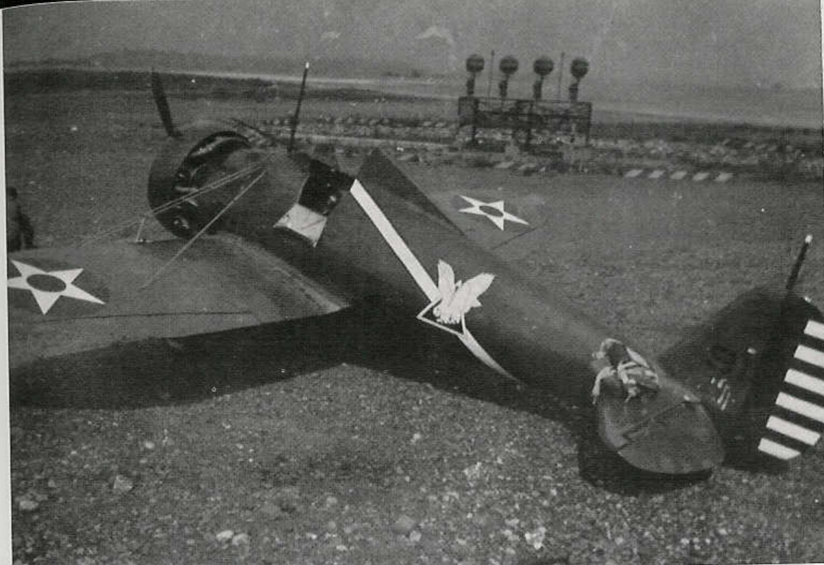
A P-26C of the 17th Pursuit Squadron at Selfridge Field during 1935. The P-26C was basically a P-26A with all the various updates specified for the late production P-26A. A number of these aircraft were re-engined with fuel injected Pratt & Whitney R-1340-33 radials and redesignated as P-26Bs. (Robert Esposito)
