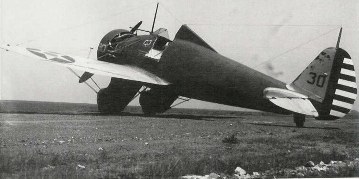
This P-26A (33-130) of the 1st Pursuit Group at Selfridge Field was flown by Lieutenant Harris. The aircraft was suffering from the effects of the harsh winter climate at Selfridge and has some of the Yellow paint on the vertical fin peeling off. The small crest under the windscreen carried the legend "Pilot LT Harris" and immediately under the crest is the legend "Selfridge Field." (Robert Esposito)
