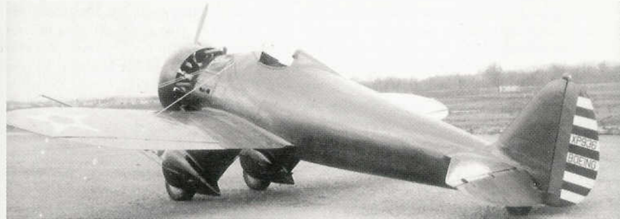
(Above & below) The first XP-936 on the ramp at the Boeing plant in February of 1932, just after the aircraft's official rollout. The rounded wing tips and short headrest was used only on the XP-936 prototypes. The first flight of the XP-936 took place on 10 March 1932, (AFM)
