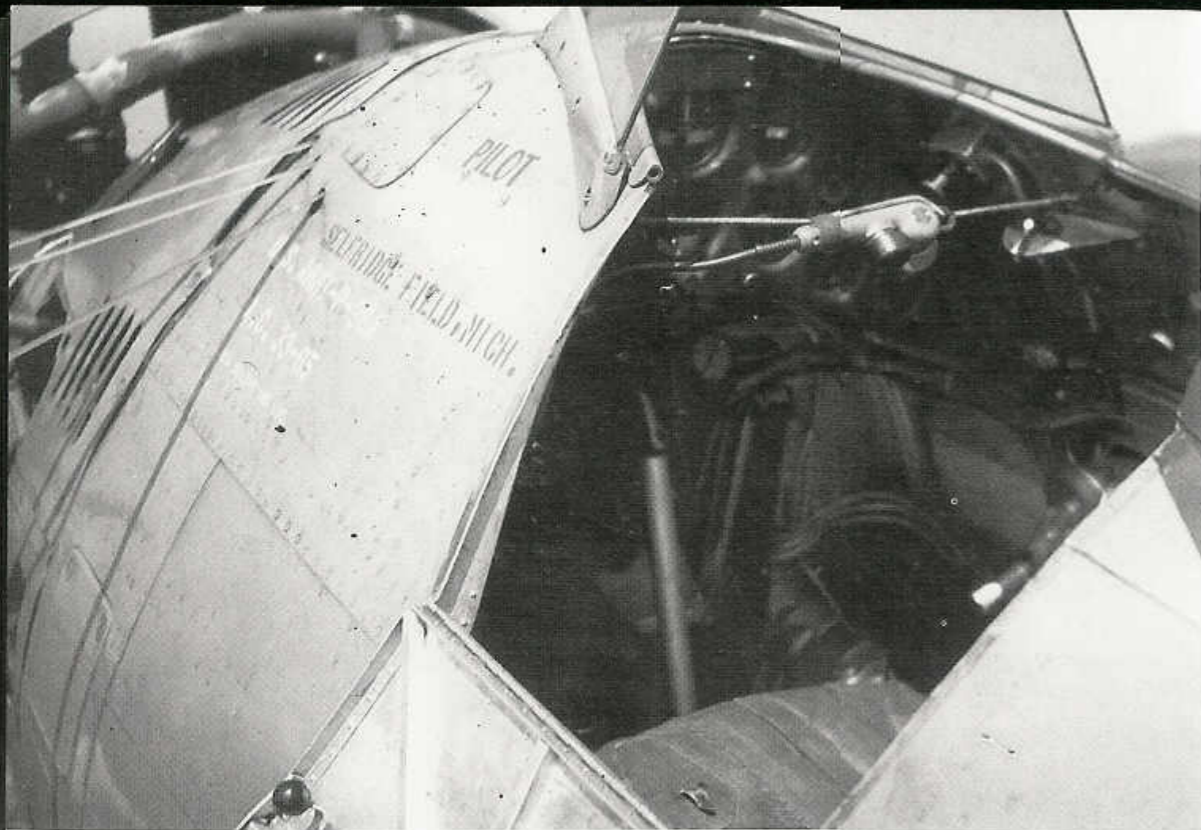
The radio equipment in the P-26 was rather difficult to use. The microphone was hung on an elastic cord stretched across the interior of the cockpit. This P-26A (33-65) was assigned to the 94th Pursuit Squadron at, as the legend on the fuselage states, Selfridge Field, Michigan. (James Binder)
