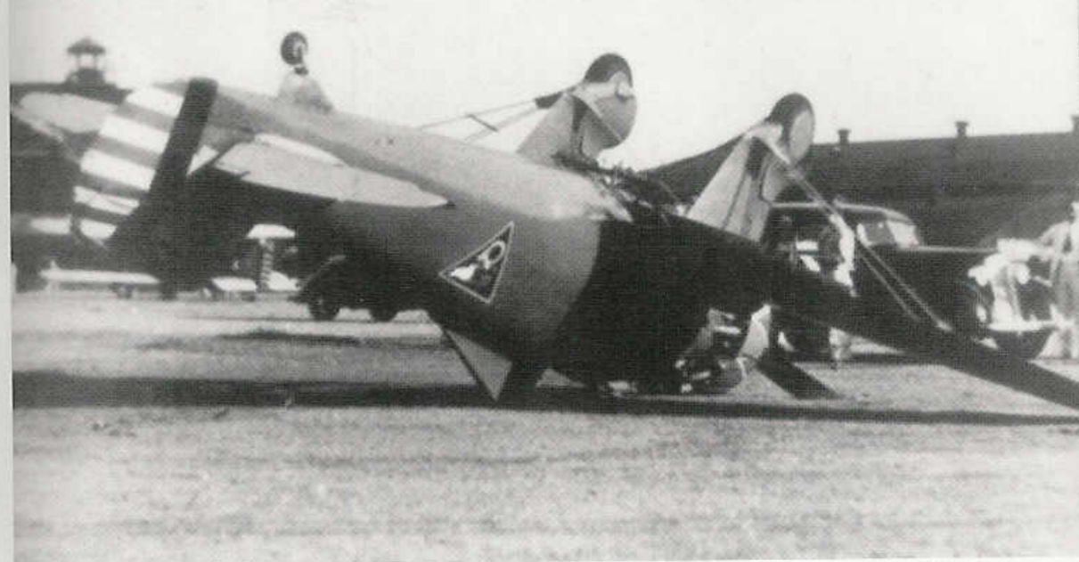
Colonel Ralph Royce, who had commanded the 1st PG at Selfridge Field during 1934, was the commander of the 4th Composite Group at Nichols Field in 1938 when he ground looped on landing, resulting in a typical P-26 turnover. Even though the damage appears great, the P-26 was repaired and was flyable again within a few days. (AFM)
