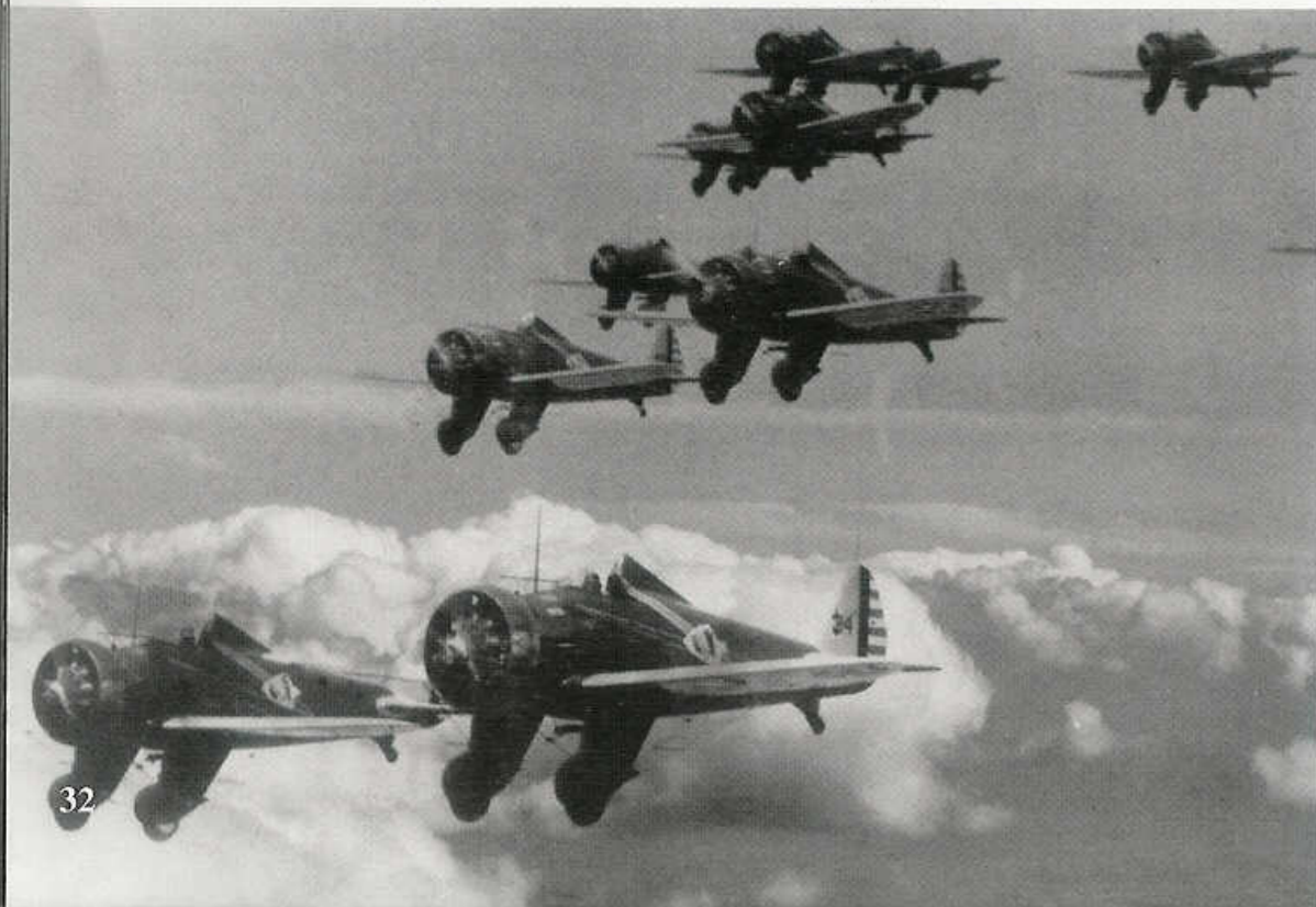
Fourteen P-26s of the 1st Pursuit Group fly formation over Michigan during 1936. This formation included the entire 94th PS, as well as aircraft from the headquarters unit at the rear. All aircraft have the re-designed taller tail wheel structure. (AFM)
