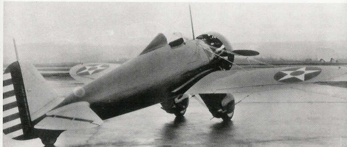
The P-26A was powered by a Pratt & Whitney R-1340-27 Wasp air-cooled radial engine and had a fixed, narrow track landing gear. Both created problems for the pilot -- the engine blocked his view and the landing gear caused many aircraft to ground loop and nose over. (AFM)
