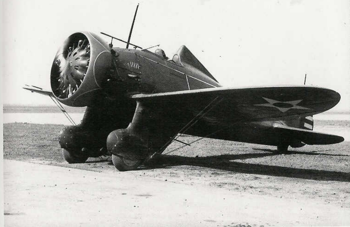
This pair of P-26As of the 77th Pursuit Squadron, 20th Pursuit Group at Barksdale Field, LA during 1934 carry the early style of 20th PG cowl ring markings. The cowl ring had a Red scallop with White trim and the engine facing was also painted Red. The long tube extending from in front of the windscreen was the telescopic gun sight. All P-26 variants were armed with a pair of .30 caliber machine guns mounted in the lower fuselage and firing through the propeller arc. Robert Esposito)
