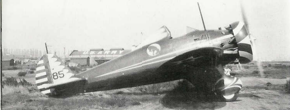
A P-26A (33-85) of the 95th Pursuit Squadron on the ramp at March Field during 1935. Most production P-26As had provisions for radic equipment and armament, although this aircraft does not have the standard telescopic gun sight installed in front of the windscreen. (Vincent Becinati)
