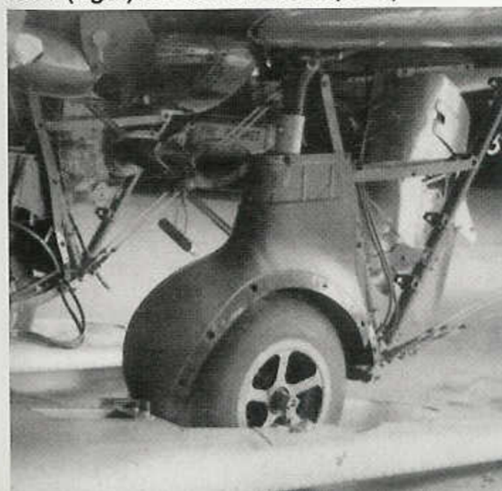
All P-26 aircraft could be fitted with the Type A-9 ski installation for operations from snow covered surfaces. The skis were hydraulically raised (left) for use on dry ground and lowered (right) for use on snow. (AFM)
