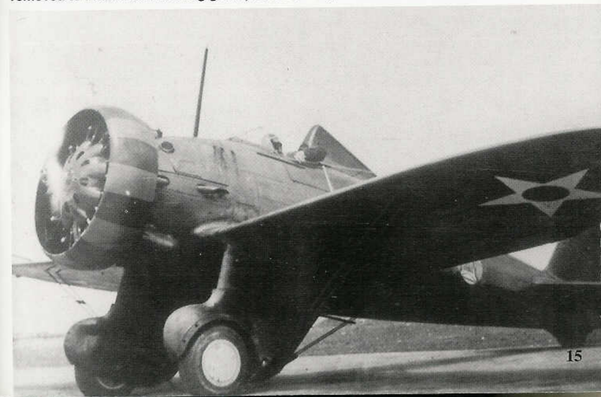
A pilot from the Bolling Field Detachment of Headquarters Command watches his instruments as the Pratt & Whitney R-1340 Wasp warms up during 1934. The Bolling Field P-26 has a Dark Blue and Yellow Townend ring cowling. The main landing gear fairings were removed to install a ski landing gear. (Peter Bowers)
