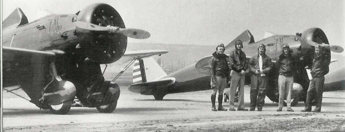
Army Air Corps pilots on the ramp at Boeing Field during 1934, ready to deliver these brand new P-26As to the 17th Pursuit Group at March Field. At the time, the P-26A was the hottest thing in the air with a top speed of 234 mph. (AFM)
