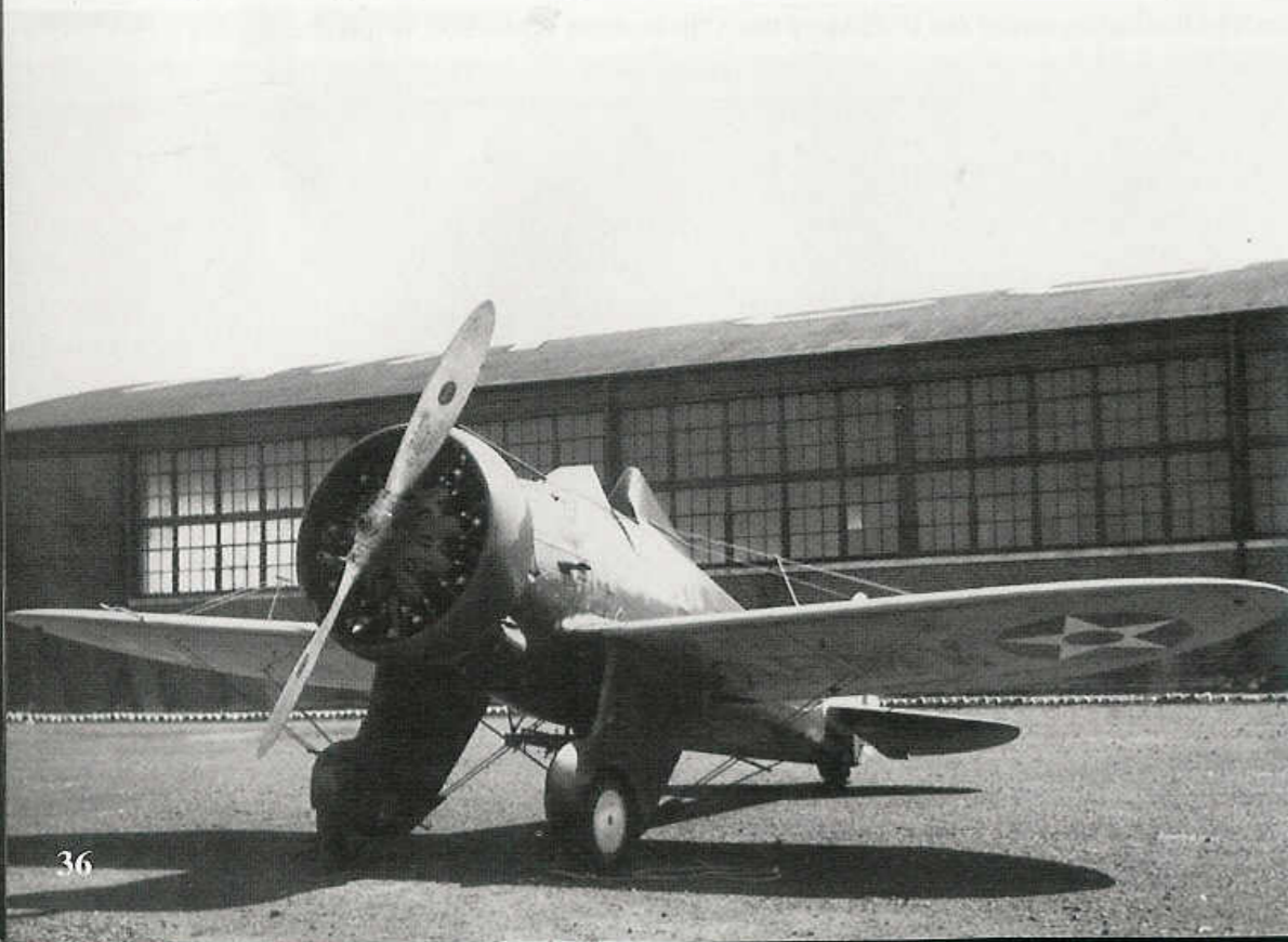
This P-26 is one of the P-26Cs (33-191) converted to P-26B standard with the fuel injected R-1340-33 engine. The aircraft carried no radio antenna masts when parked on the ramp at Newark Airport during 1936, even though most P-26s were radio-equipped. (Jack Binder)
