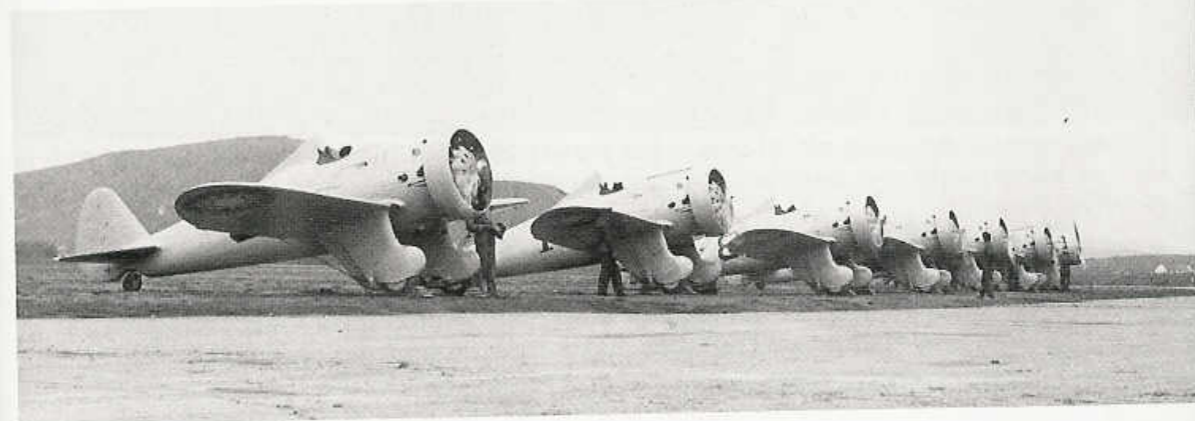
(Above & Below) Ten production Model 281s were delivered to the Nationalist Chinese Air Force during early 1936. All were initially painted in overall Light Gray, with a large Black number on the side and Chinese insignia above and below both wings. (Norman Poncetti)
