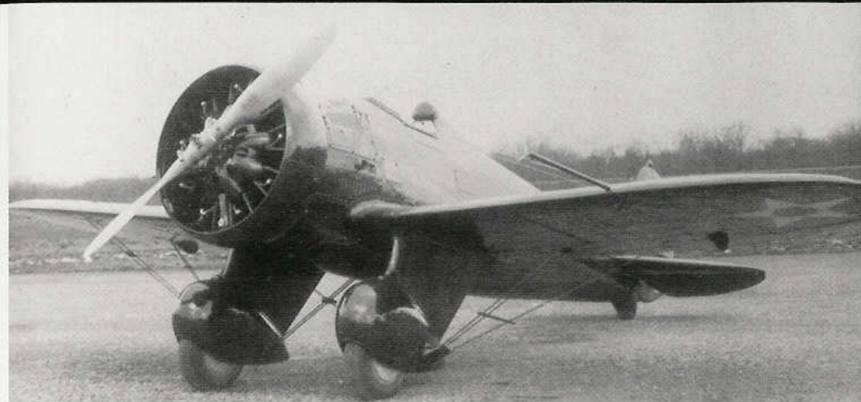
(Above & below) The first XP-936 on the ramp at the Boeing plant in February of 1932, just after the aircraft's official rollout. The rounded wing tips and short headrest was used only on the XP-936 prototypes. The first flight of the XP-936 took place on 10 March 1932, (AFM)
