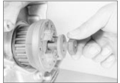
7.11a Remove the crankshaft sprocket retaining bolt . . .
