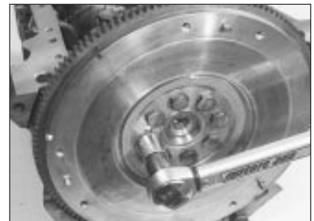
17.12 . . . then refit the flywheel, and tighten the bolts to the specified torque
