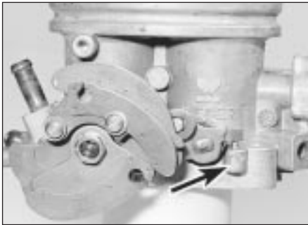
14.6a Secondary throttle adjusting screw (arrowed) . . .
