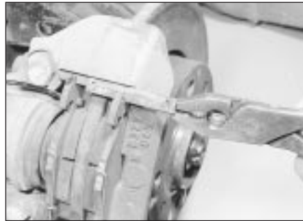
4.5b . . . then slide the pad retaining plate from the caliper - Bendix caliper
