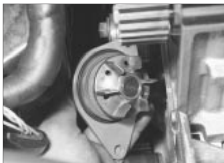
7.6a Withdraw the coolant pump . . .
