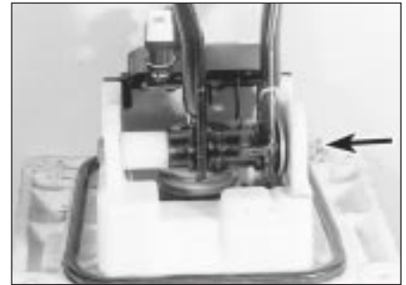
14.4 Pedal pivot bolt and nut (arrowed)
