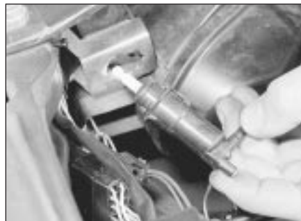
7.4 Removing a cable-operated headlight adjuster
