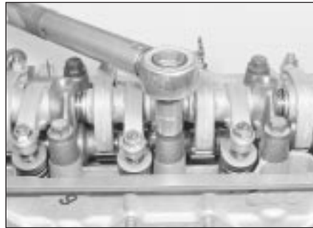
11.37b Working in the sequence shown, tighten the head bolts first to the stage 1 torque setting . . .
