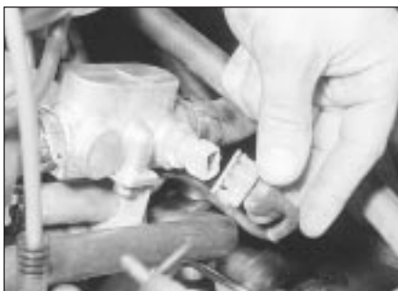
14.48 Disconnecting the injection thermistor wiring
