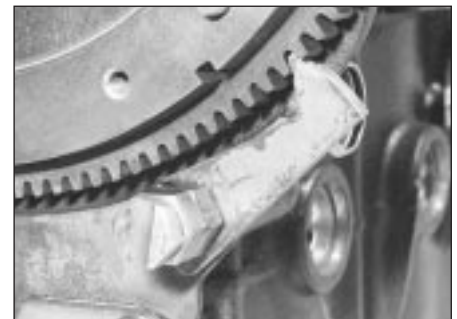
5.3 Use a fabricated tool like this one to lock the flywheel ring gear and prevent crankshaft rotation
