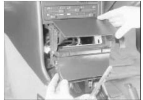
30.36b ... then withdraw the housing
