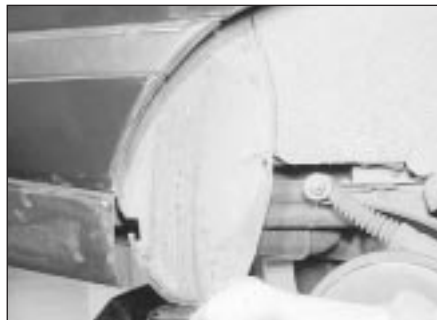
7.2 Removing a rear wheel arch liner
