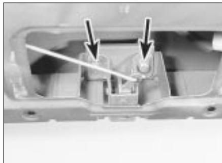
19.9 Tailgate lock securing bolts (arrowed)
