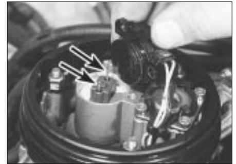
15.3c On refitting, ensure cap terminals are aligned with injector pins (arrowed)
