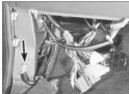
30.18 Unbolt the earth lead (arrowed) from the footwell
