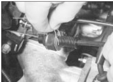
7.9 Adjusting the accelerator cable
