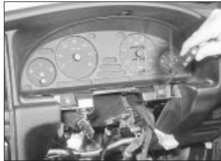
9.21 Unscrew the lower instrument panel securing screws
