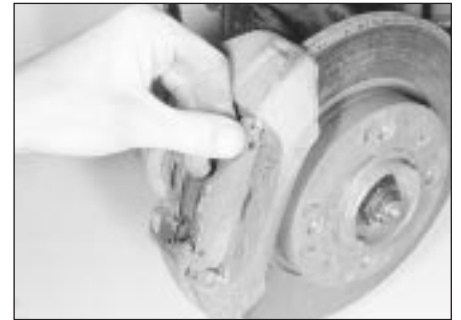
4.6 Withdrawing the outer brake pad - Bendix caliper
