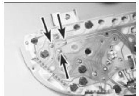
10.9 Fuel gauge securing nuts (arrowed)
