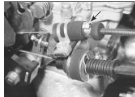
9.10 Choke cable-to-rubber collar retaining clip (arrowed)
