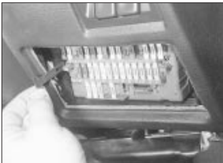
3.11a Pull out the securing clip . . .
