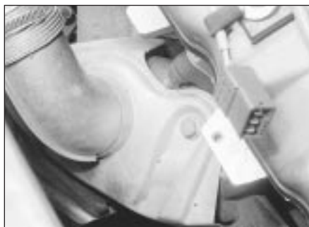
3.8a Hot-air collector plate on exhaust manifold (XU engine)
