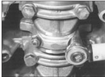
19.22a On XU series engines, tighten the big-end bearing cap nuts to the stage 1 specified torque, then fully slacken them and tighten them to the stage 2 torque . . .
