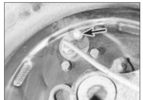
2.12b Bleed nipple (arrowed) on rear wheel cylinder
