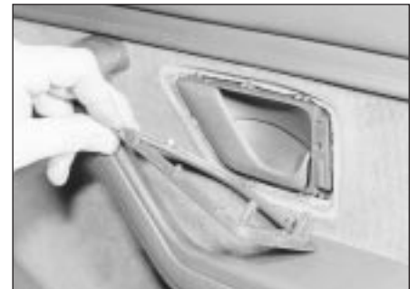
13.2 Removing the door interior handle surround
