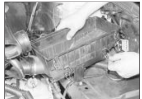
2.4 Removing the air cleaner housing
