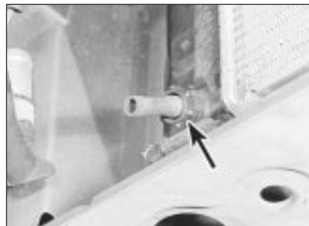
20.3 Radiator drain outlet (arrowed)
