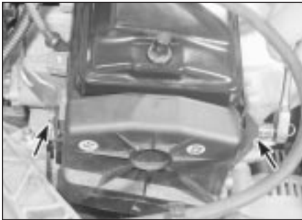
5.1a Undo the two retaining bolts (arrowed) . . .
