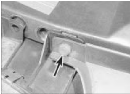
25.3 ... and the upper securing bolts (arrowed)
