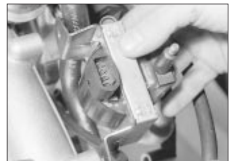
3.5d Removing the ignition coil and bracket on the Motronic ignition system
