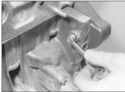
7.8 . . . and the spindle locknut, then release the belt tension by turning the tensioner cam spindle
