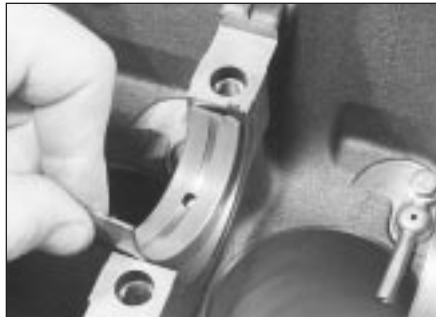
11.21 Remove the upper main bearing shells from the cylinder block/crankcase, and store them with their lower shells
