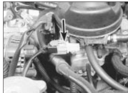
16.3 Injector wiring connector (arrowed)
