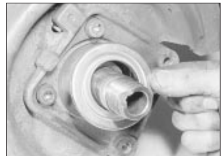
10.6c . . . and the oil seal support cup
