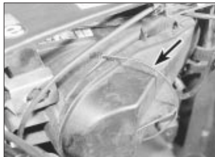
5.2 Headlight rear cover securing clip (arrowed)
