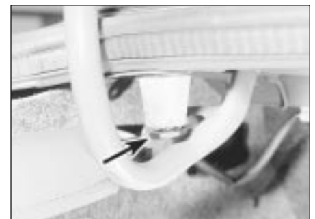
16.6 Rubber stop (arrowed) under boot lid hinge arm
