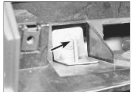
30.23 Upper facia securing bolt (arrowed)
