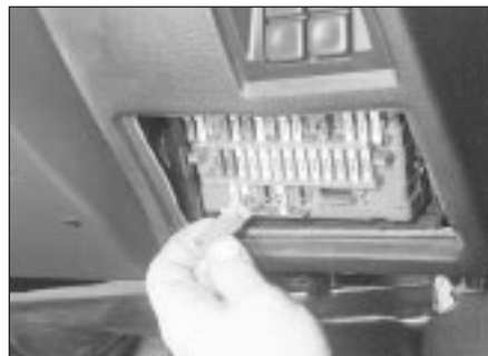
3.7 Removing a fuse using the plastic tool
