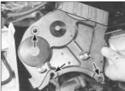
5.3 . . . then undo the three bolts (locations arrowed) and remove the centre belt cover
