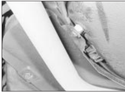
16.15 Heat shield on the underside of the fuel tank
