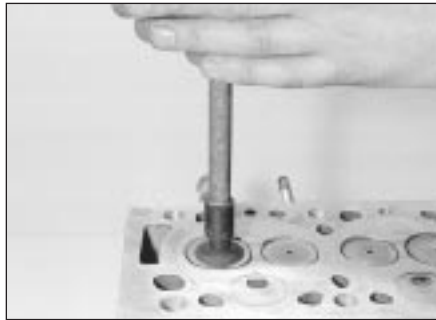
8.14 Grinding-in a valve
