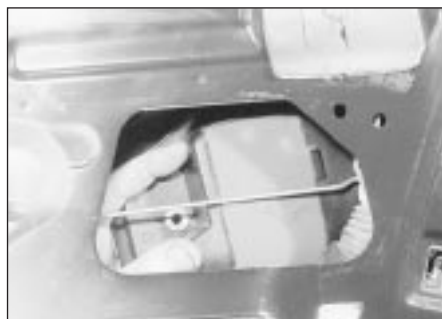
14.7c . . . and withdraw the plastic shield - later model
