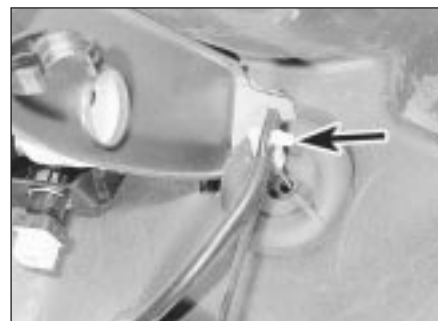
7.4 Accelerator cable connection to accelerator pedal (arrowed)
