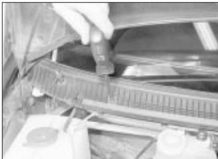
25.9 Unscrew the grille panel securing screws
