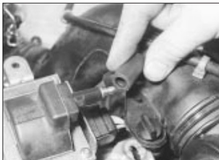
3.4a . . . then disconnect the HT lead . . .
