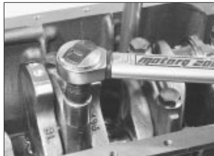
18.74a With all bearing caps correctly installed, tighten their retaining nuts and bolts to the specified torque . . .
