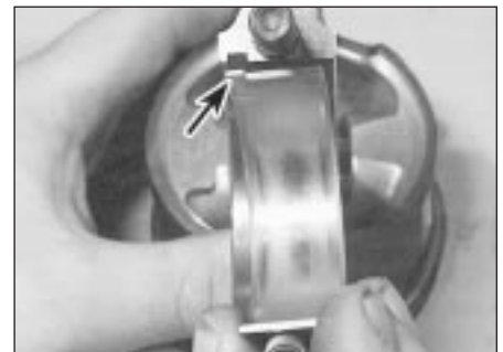
19.5 Fitting a bearing shell to a connecting rod - ensure tab (arrowed) engages with the recess in the connecting rod
