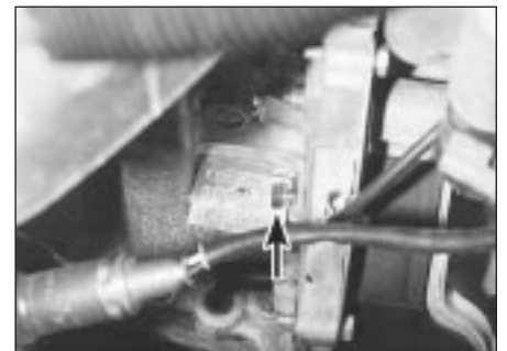
3.4 Insert a 6 mm bolt (arrowed) through hole in cylinder block flange and into timing hole in the flywheel . . .
