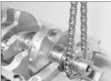
18.42 Refitting the oil pump drive chain and sprocket - TU aluminium block engine
