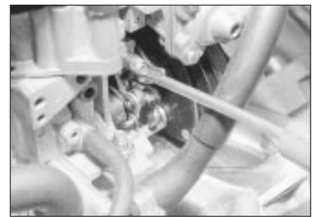
10.4b Idle speed adjustment screw
