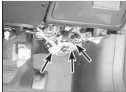
30.41b . . . then disconnect the three wiring connectors (arrowed)
