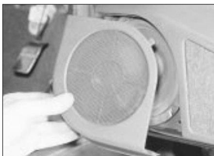
21.2b . . . and remove loudspeaker cover panel from the door - models up to 1992
