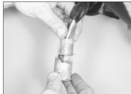
18.8c . . . and slide out the ignition switch
