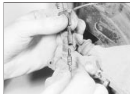
4.2 Disconnecting the pad wear sensor wiring connector
