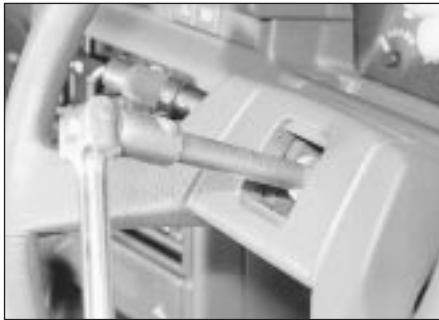
16.4 Unscrewing the steering wheel nut
