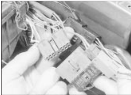
11.7a Disconnecting the front light wiring connectors - models up to 1992
