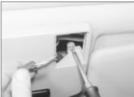
20.31 Removing a roof console securing screw
