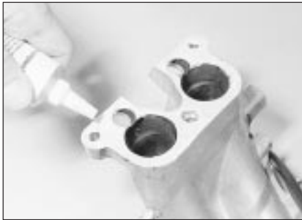
18.12a Applying jointing compound to the inlet manifold
