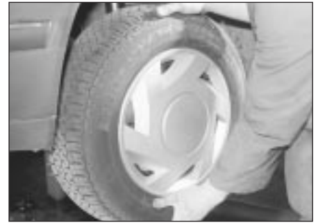
16.4 Check for wear in the hub bearings by grasping the wheel and trying to rock it
