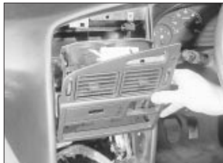
11.15 . . . then withdraw the housing
