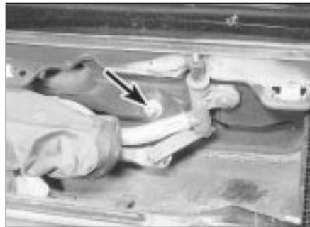
30.70 Facia securing nut (arrowed) in scuttle
