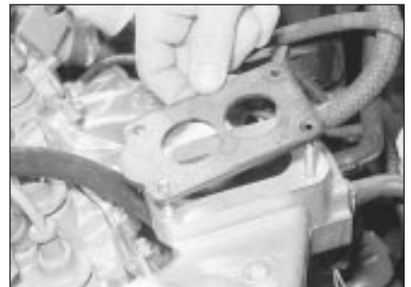
12.11 Removing the insulating spacer
