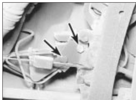
21.4 Rear brake pressure-regulating valve securing bolts (arrowed)
