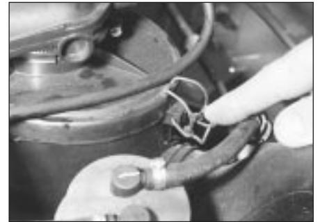
21.2a . . . then release the air cleaner lid retaining clips, and the duct clip . . .
