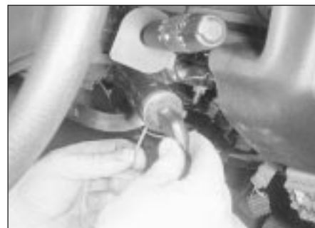
18.6 Depress the lock retaining lug, whilst pulling out the lock using the key
