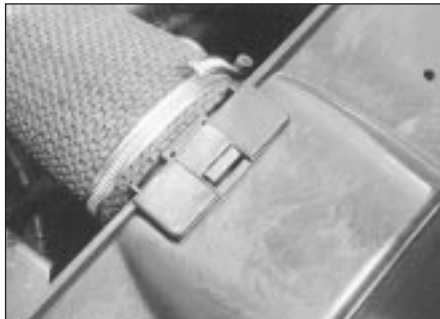
4.4 Inlet air duct connection to the front crossmember
