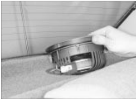
21.13 Removing the rear loudspeaker - Saloon models
