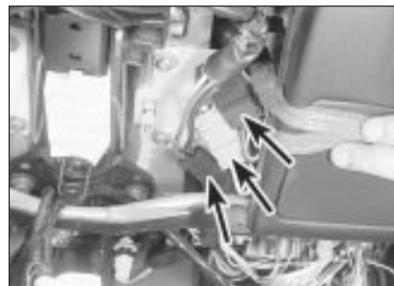
17.8 Ignition switch wiring connectors (arrowed) - models from 1993
