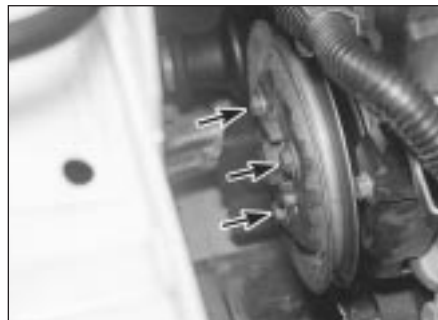
5.6a Undo the three retaining bolts (arrowed) . . .
