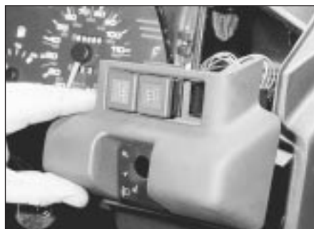
9.6 Withdrawing the driver's side upper facia panel
