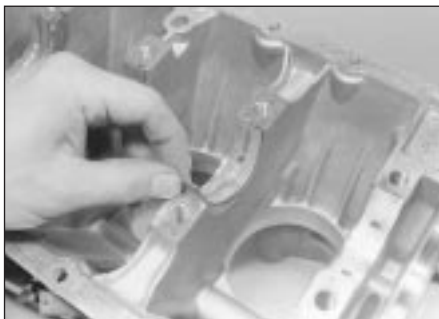
18.20 On TU series engines, note that the grooved bearing shells are fitted to Nos 2 and 4 main bearing journals
