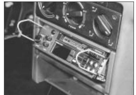
20.3 . . . then insert the removal tools . . .
