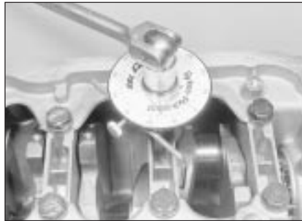
18.45b . . . then angle-tighten them through the specified stage 2 angle
