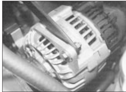
7.4a Slacken and remove the alternator upper mounting bolt . . .
