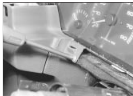
9.5 Removing the upper centre facia panel securing screw - models up to 1992
