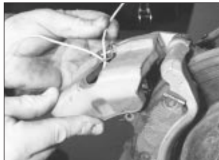
4.23 . . . then refit the caliper, feeding the pad wiring through the caliper aperture
