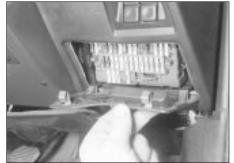
3.3c Removing the fusebox cover - later models
