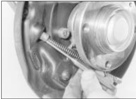
19.19 Tapping the handbrake cable sheath end fitting from the brake backplate
