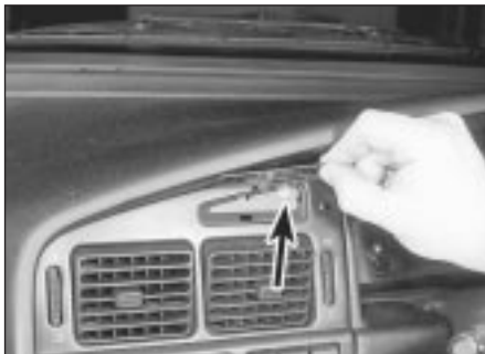
30.37 Prise out the blanking plate to expose the ventilation nozzle housing upper securing screw (arrowed)
