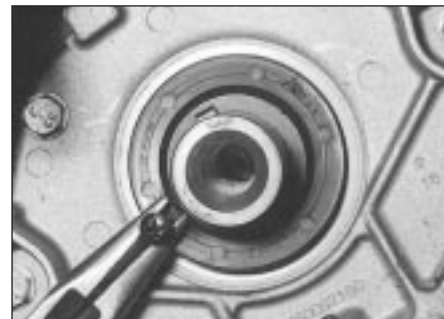
16.2 Using a self-tapping screw and pliers to remove the crankshaft oil seal
