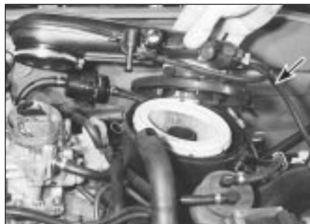
2.2b . . . and remove the duct, disconnecting the air temperature control valve hose (arrowed)
