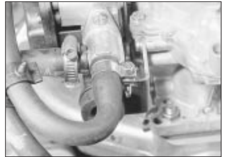
12.6a Automatic choke coolant pipe connection . . .
