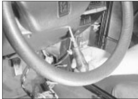
28.4a Remove the securing screws . . .
