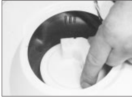
10.1 Removing the fuel gauge sender unit
