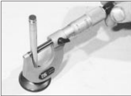
8.11 Measuring a valve stem diameter
