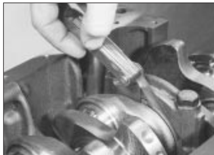
14.3 Checking crankshaft endfloat using feeler gauges
