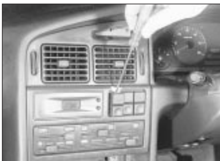
30.39a Prise the switches from the housing ...
