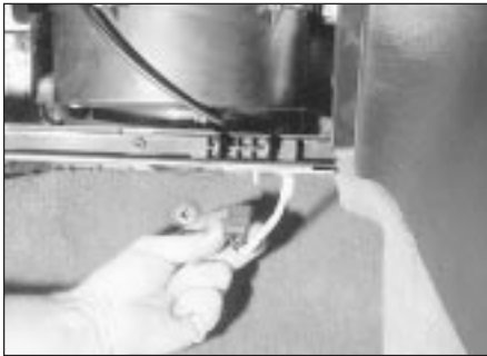
9.59 Disconnect the blower motor wiring plug
