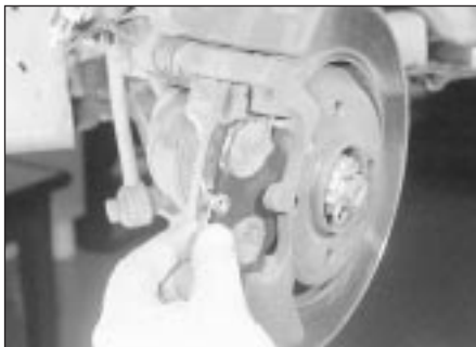
4.22 Ensure that the brake pads are fitted the correct way around, with friction material facing the disc . . .
