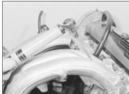
18.12d Tightening the manifold securing bolts
