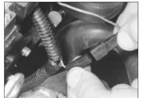
3.3 On breakerless ignition models, disconnect the capacitor wiring connector, and release the TDC sensor connector . . .
