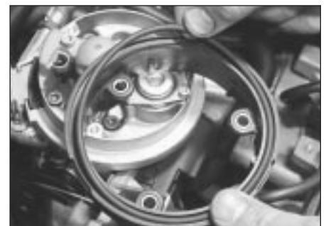
15.15b . . . then lift off the plastic ring and recover the sealing ring
