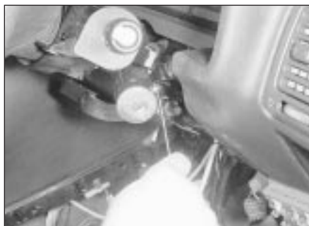
18.5 Unscrewing the lock securing screw
