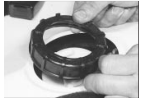
9.11 Unscrew the locking ring . . .
