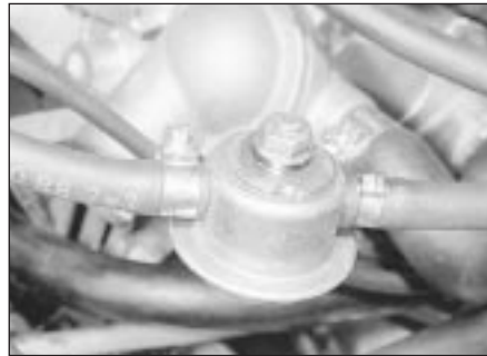
14.40 Fuel pump damper showing fuel hose connections
