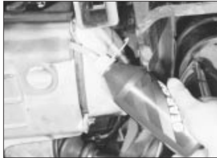
26.4 Topping-up the transmission oil level
