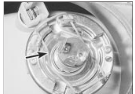
5.4a Release the spring clip (arrowed) . . .
