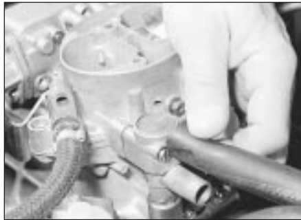
12.5 Disconnecting the float chamber breather pipe
