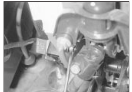
30.19 Remove the bolt securing the relay bracket to lower steering column bracket
