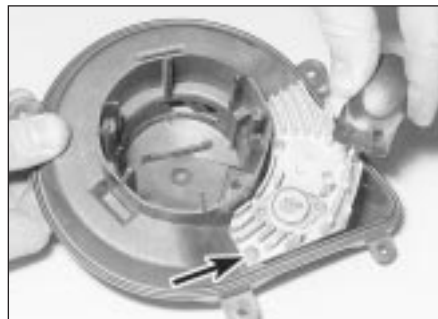
9.68a . . . then remove the securing screws . . .
