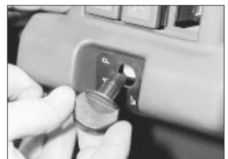
9.5 Prise off the headlight adjuster switch knob
