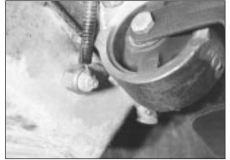
15.1 The oil temperature sensor is screwed into the sump
