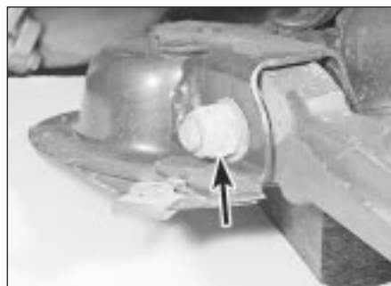
6.4 Lower arm front pivot nut (arrowed)
