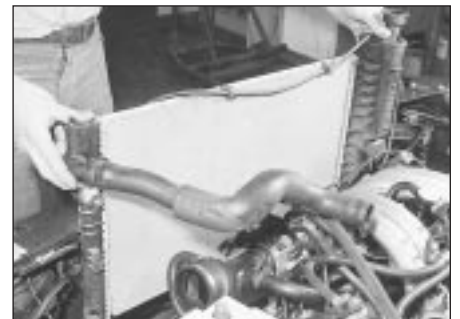
3.11 Lifting out the radiator
