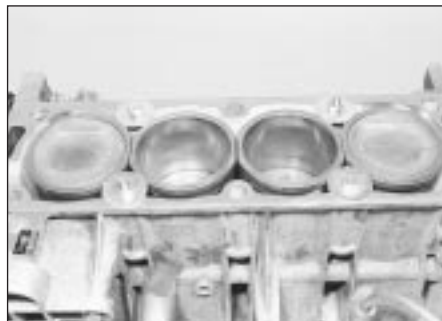
12.21 Cylinder liners clamped in position using suitable bolts and large flat washers
