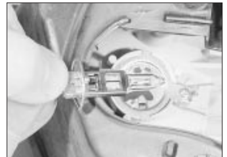
5.23b Removing a headlight-mounted driving light bulb
