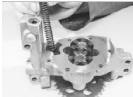
14.5b . . . then lift off the cover and remove the spring . . .
