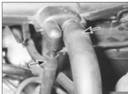
2.1 On the TU engine disconnect the vacuum and breather hoses (arrowed) from the front of the duct . . .
