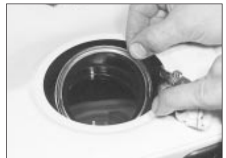
9.12b . . . and recover the rubber sealing ring
