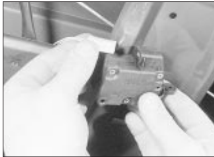
20.9 Disconnecting the wiring plug from the tailgate lock motor
