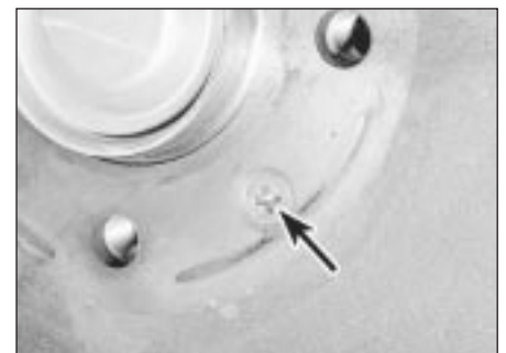
9.2 Rear brake drum retaining screw (arrowed)
