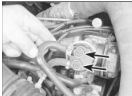
4.3 Arrows on raised fuel pump unions indicate the direction of fuel flow
