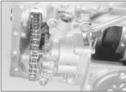
13.2 Oil pump is retained by three bolts
