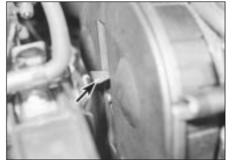
6.24 Timing belt upper (outer) cover retaining clip (arrowed) - 1998 cc 16-valve models
