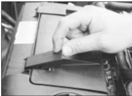
21.14b . . . and release the retaining clips
