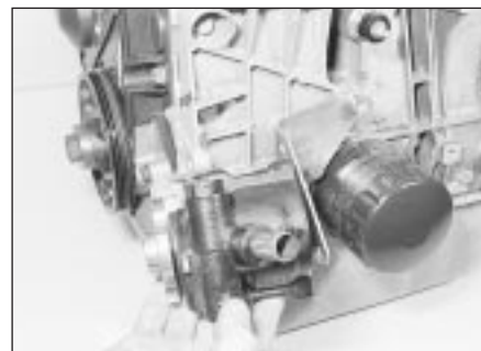
22.9b . . . and remove the pump - XU5 and XU9 engines (engine removed for clarity)
