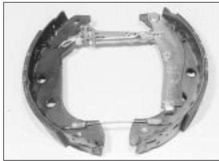
6.19c Front view of early type Bendix shoe assembly correctly assembled - removed from backplate for clarity
