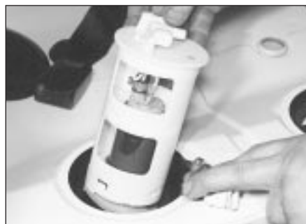
9.12a . . . then lift out the fuel pump . . .
