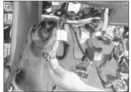
30.60 Unplug the main wiring harness connectors
