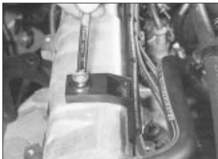
4.5 On 1580 cc and 1905 cc models, undo the retaining bolts/nuts and move the HT lead retaining clips clear of the head cover
