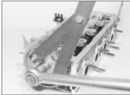
8.43 Using a home-made tool for retaining the camshaft sprocket whilst the sprocket bolt is tightened (TU engine shown)
