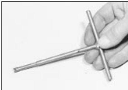
6.6a Forked tool for removing early type Bendix shoe retainer springs
