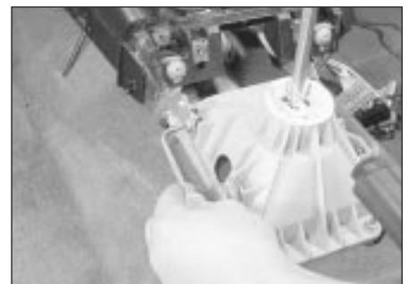
30.67 Unscrew the centre fascia lower securing bolts
