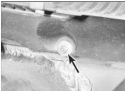
30.20 Facia securing nut (arrowed) in scuttle
