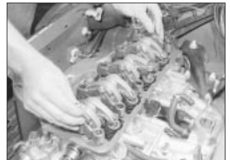
11.34 . . . and refit the rocker arm assembly
