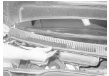
25.11 Removing the scuttle grille panel
