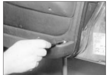
13.10 Removing the rear door trim panel securing screw - later model
