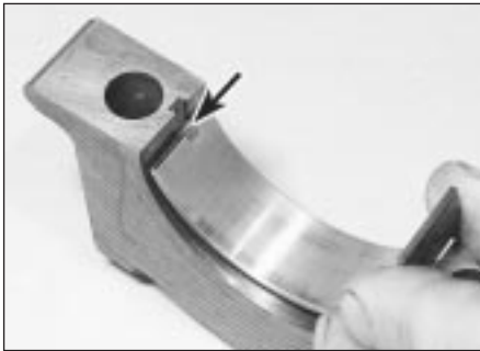
18.34 On XU engines, all the lower shells have a plain bearing surface. Ensure tab (arrowed) is correctly located in the cap
