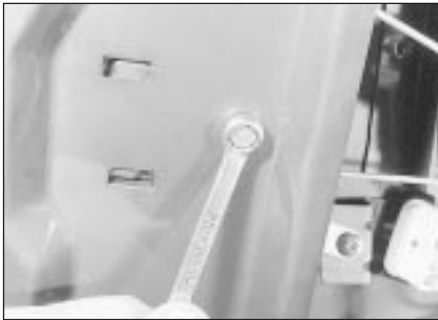
20.8 Unscrewing the tailgate lock motor securing bolt
