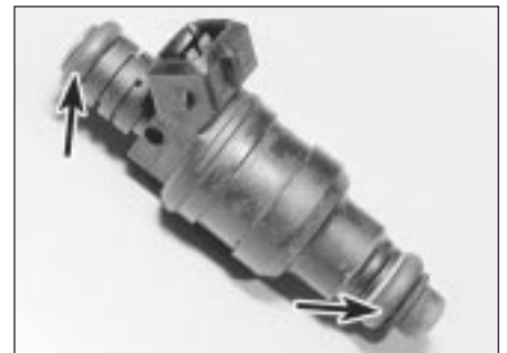
14.30 Injector O-ring seals (arrowed)
