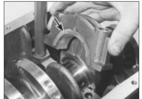
11.19 Removing No 2 main bearing cap. Note the thrustwasher (arrowed)
