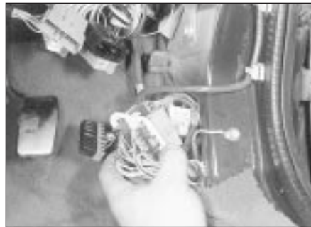
30.43 Pull the connector bracket from the footwell
