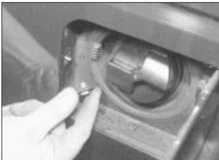
20.24a Remove the bolt securing the fuel filler flap lock motor to the body
