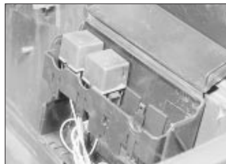
3.14d Relays in engine compartment relay box - models up to 1992
