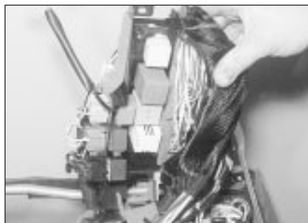
3.14c Main relay box located behind fusebox at rear of fascia - models from 1993 (viewed with fascia removed and inverted)
