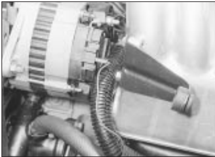
7.2 Connections on the rear of the alternator
