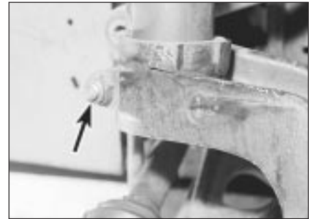
2.12 Hub carrier-to-suspension strut clamp nut (arrowed)
