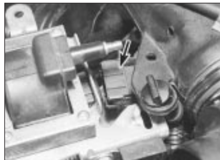
3.4b . . . and wiring connector (arrowed) from the ignition HT coil
