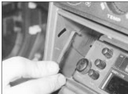
20.2 Remove the plastic trim panels from the sides of the radio/cassette player . . .
