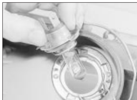
5.4b . . . then withdraw the headlight bulb
