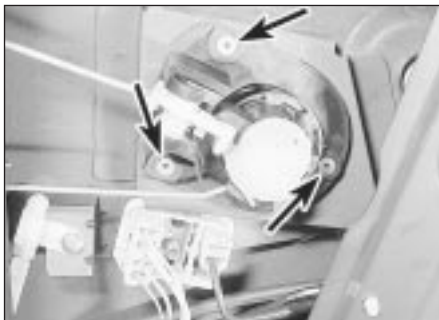
19.4 Tailgate lock cylinder securing rivets (arrowed)
