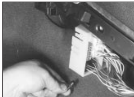
30.48 Release the connector block from the bracket on the driver's side of the fascia
