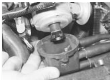
4.2c . . . and remove the cap from the end of the distributor
