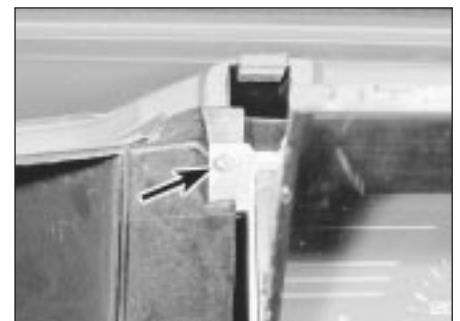
9.8 Instrument panel securing screw (arrowed)
