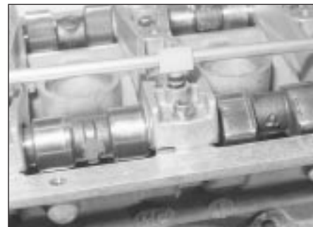
10.55 Take care not to displace the O-rings when refitting the oil supply pipe to the camshaft bearing caps
