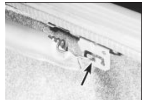
16.2 Note which slots (arrowed) the ends of the boot lid assister springs are positioned in before disconnecting them
