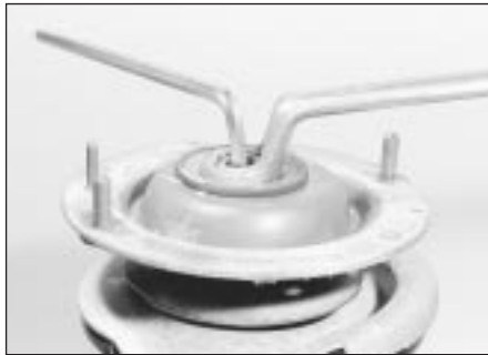
5.3 Counterhold the piston rod and unscrew the top mounting nut
