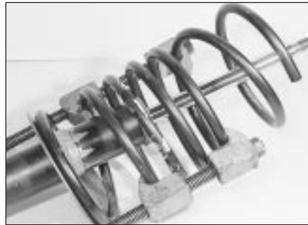
5.10a Refit the coil spring, with the compressors in position . . .
