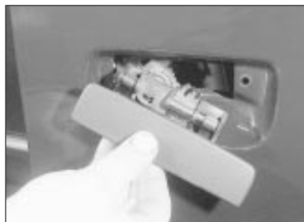
14.8 Withdrawing the exterior door handle
