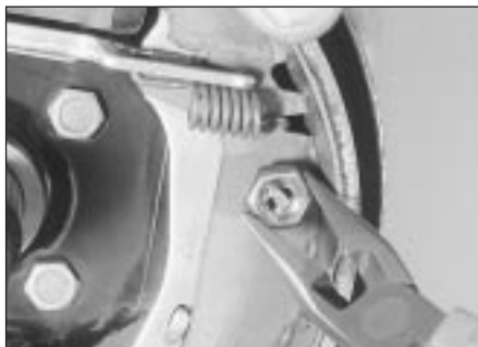
6.7 Removing a later type Bendix shoe retainer spring
