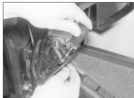
22.4 Loosen the clamp screw and release mirror adjuster knob from the trim plate
