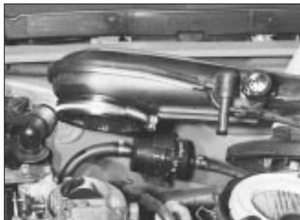
21.2b . . . and remove the duct, positioning it clear of the air cleaner housing
