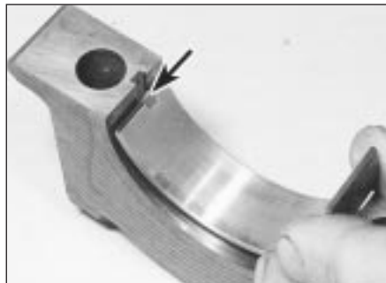
18.54 Ensure tab (arrowed) is located in the cap when fitting the bearing shells
