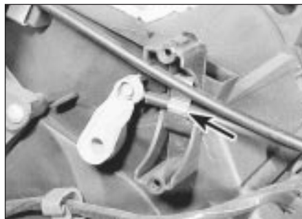
9.28 Heater control cable metal spring clip (arrowed) at heater unit
