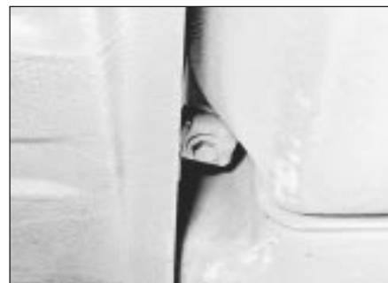
6.9 Fuel tank support strap bolt
