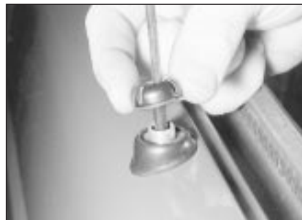
22.15a Unscrew the ring nut . . .
