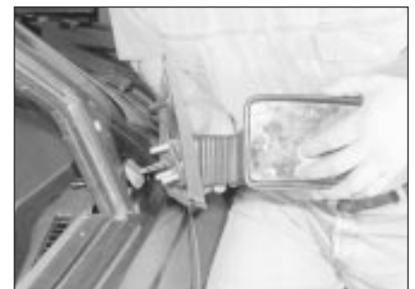
22.6b . . . and withdraw the mirror
