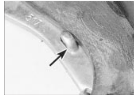
9.9 Check that the handbrake lever stop-peg (arrowed) is against the shoe edge
