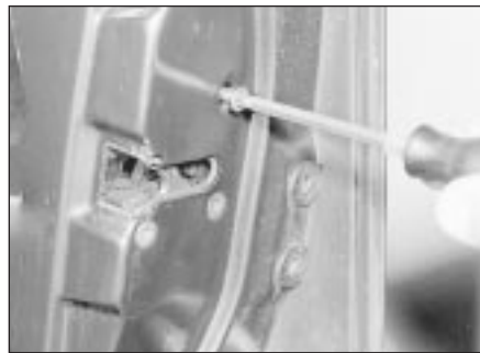
14.16 Remove the door lock securing screws
