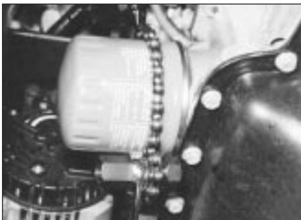
3.8 Using an oil filter removal tool to slacken the oil filter
