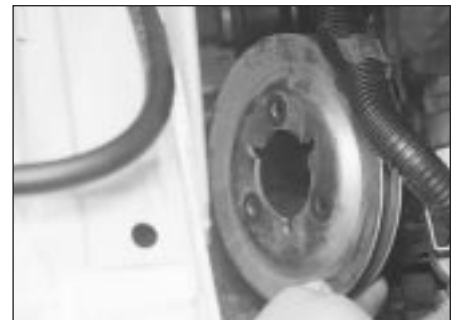
5.6b . . . and remove the crankshaft pulley
