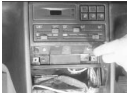
30.38a Remove the two screws from the front of the ventilation nozzle housing ...
