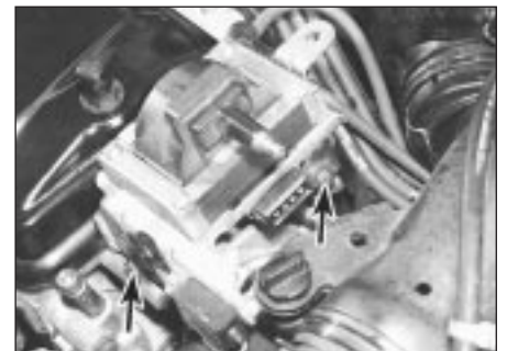
3.5a Undo the two retaining bolts (arrowed) . . .
