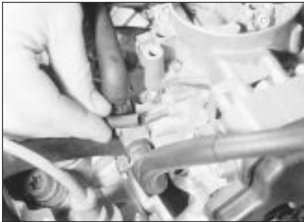
12.4 Disconnecting the distributor vacuum pipe
