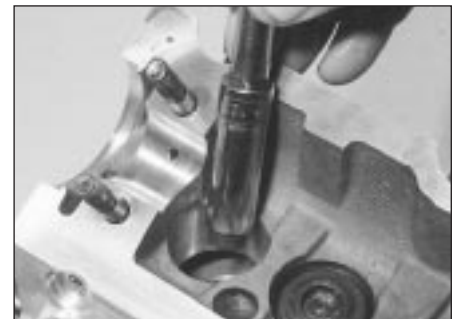
9.2 Fitting a valve stem oil seal using a socket
