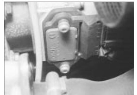
5.2 On breakerless ignition systems the amplifier unit is mounted on the side of the distributor body
