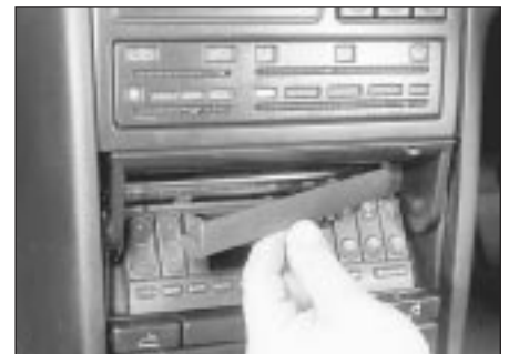
20.12 Prise the trim panel from the top of the radio/cassette player
