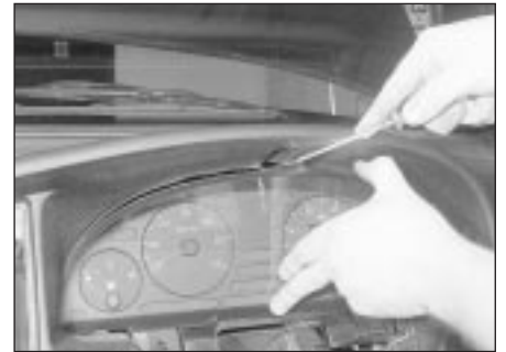
9.22 Lever the upper securing clip down . . .
