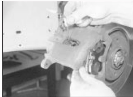
4.20 Pivot the caliper upwards away from the brake pads - Girling caliper
