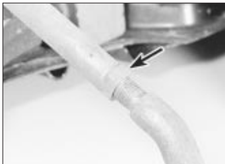
22.33 Track rod end locknut (arrowed)
