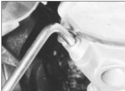
26.3 Using a square-section wrench to unscrew the transmission filler/level plug (MA transmission shown)
