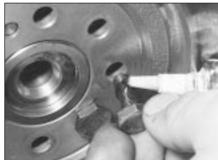
17.10 If the new flywheel bolt threads are not supplied with their threads pre-coated, apply locking compound to them . . .
