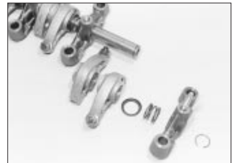
10.4 Remove the circlip, and slide the components off the end of the rocker arm
