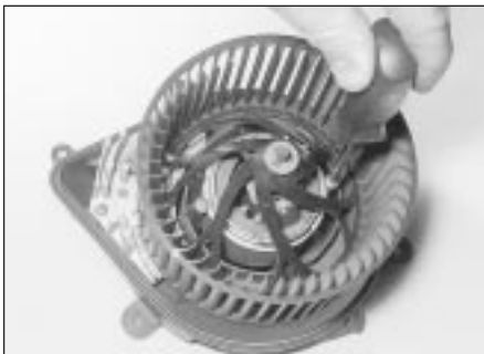
9.65a Remove the securing screws . . .
