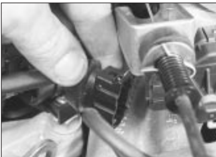
12.3b . . . the injector wiring loom connector and the stepper motor
