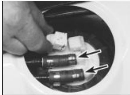
9.9 Unplug the wiring connector then release the fuel feed and return hoses (arrowed) from the fuel pump
