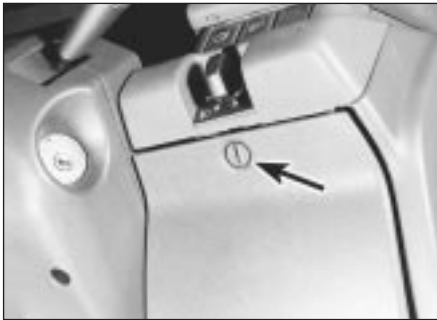
3.3a Release the securing clips (arrowed) . . .
