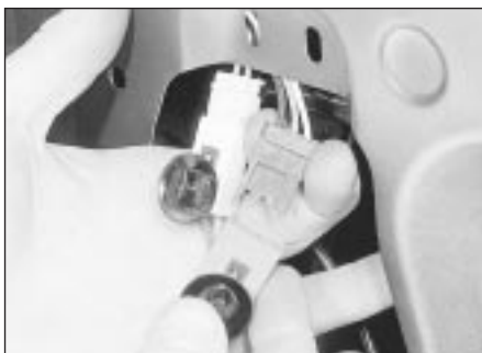
22.3 Disconnecting the door mirror wiring connectors
