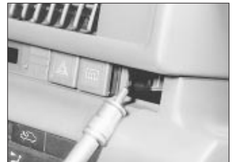
9.3a . . . and remove the visor securing screws
