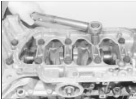
18.45a Tighten ten 11 mm main bearing bolts to the stage 1 torque setting . . .
