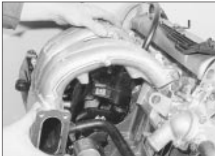
18.12c Fitting the inlet manifold
