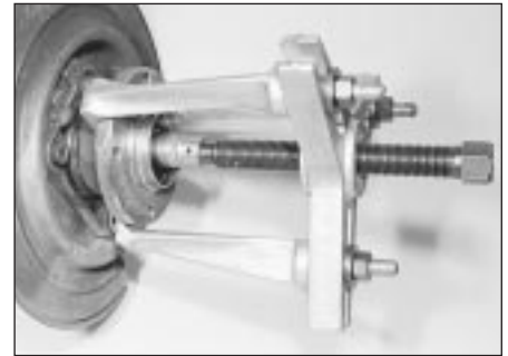
10.6a Using a puller to draw the rear hub assembly from the stub axle
