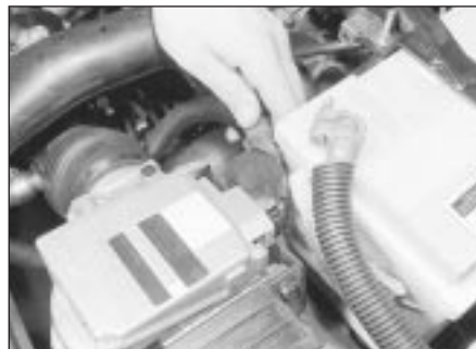
2.1 Disconnecting the airflow meter multi-plug (Bosch L3.1-Jetronic)
