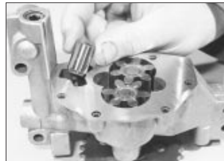
14.5c . . . and relief valve piston, noting which way round it is fitted
