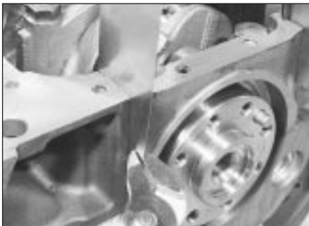
18.73b Removing a metal strip from No 1 main bearing cap using a pair of pliers
