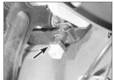
22.1 Stop-light switch (arrowed) on brake pedal bracket
