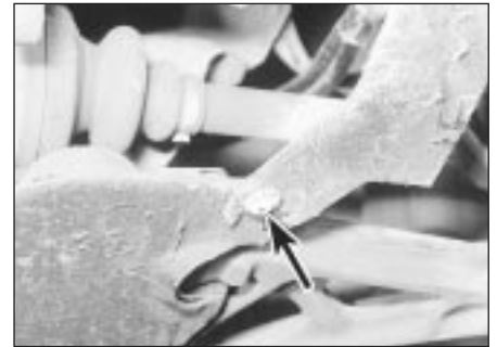
9.6 Remove the (arrowed) screws securing the underbody shields to the subframe
