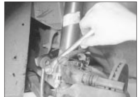
4.5 Unscrewing the hub carrier-to-suspension strut clamp bolt
