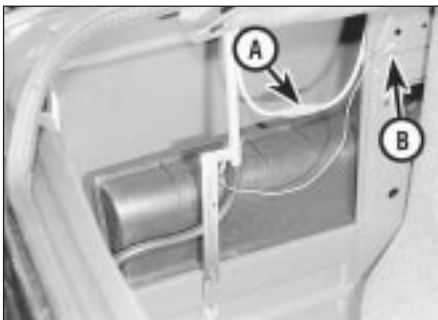
22.13 Aerial lead (A) and earth wire (B) - Saloon (rear wing-mounted manual aerial)
