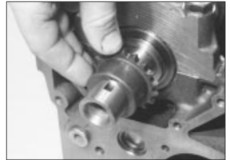
11.16b . . . then slide off the drive sprocket . . .
