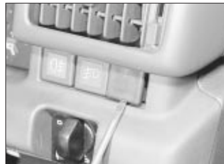
9.2 Prise out the blanking plates . . .
