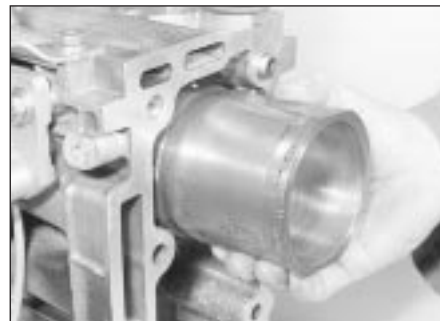
12.18a On aluminium block engines, remove each liner . . .
