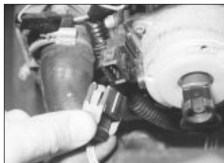
4.3a Disconnect the distributor wiring connector . . .
