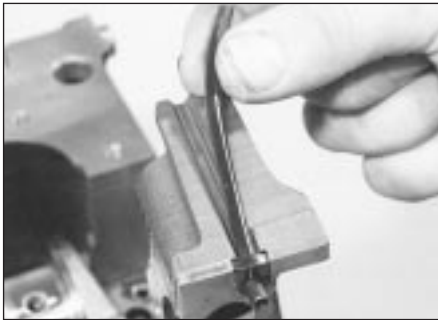
18.72a Fitting a sealing strip to No 1 main bearing cap
