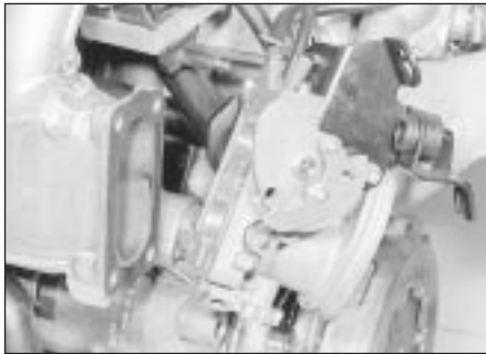
12.8 Removing the throttle housing
