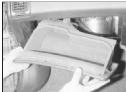
28.14 . . . and withdraw the glovebox - models from 1993
