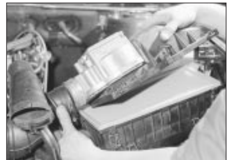
21.8 Lifting off the top cover
