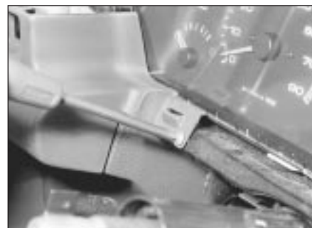
9.7 Remove the upper centre facia panel securing screw
