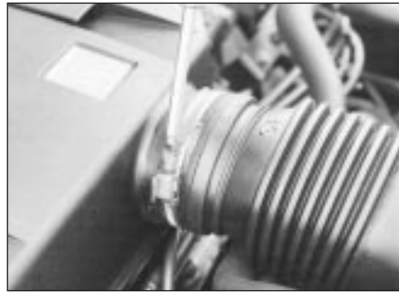
21.13 Disconnect the intake duct from the front of the cylinder head cover . . .
