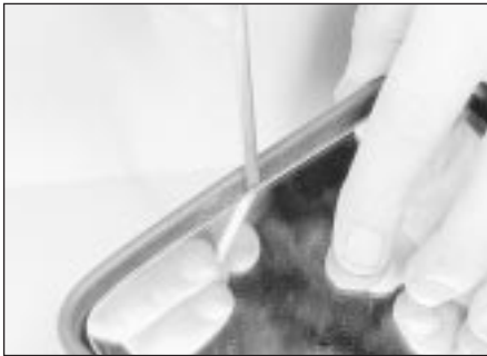
22.9 Releasing a mirror glass locking ring
