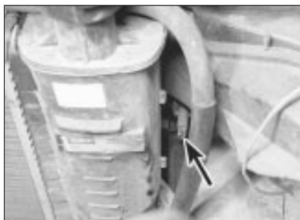
8.2b Headlight beam horizontal fine adjuster (arrowed)
