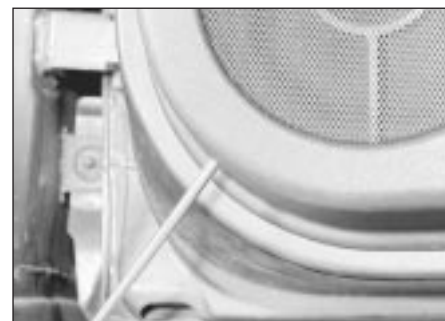
21.2a Release the securing clip . . .
