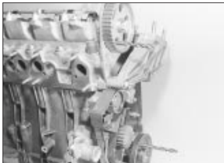
3.13 Camshaft sprocket and crankshaft pulley locking pins in position (1580 cc model shown)
