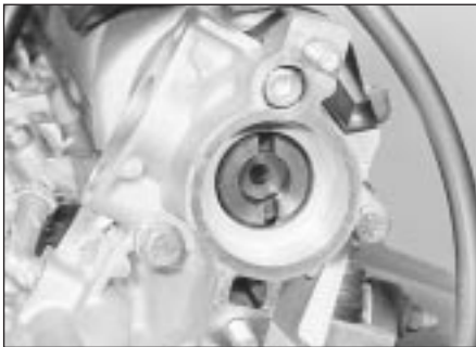
4.10 Off-set drive slots on the camshaft
