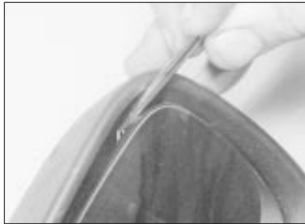
22.10a Prise ends of the clip apart (seen with mirror removed and inverted) . . .
