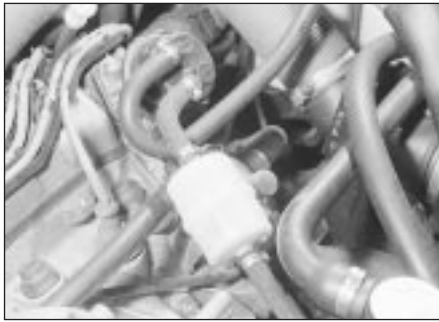
8.1 Fuel filter location on carburettor models
