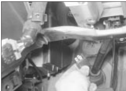
30.62a Pull the relay out of its connector . . .
