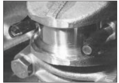
10.6 To protect the crankshaft journals, tape over the connecting rod stud threads prior to removal
