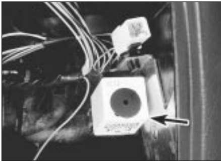
13.2 "Lights on" warning buzzer (arrowed) - models up to 1992
