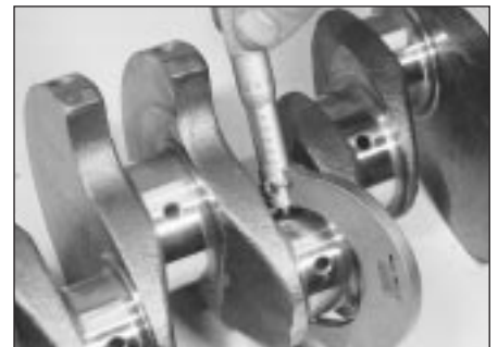
14.10 Measuring a crankshaft big-end journal diameter
