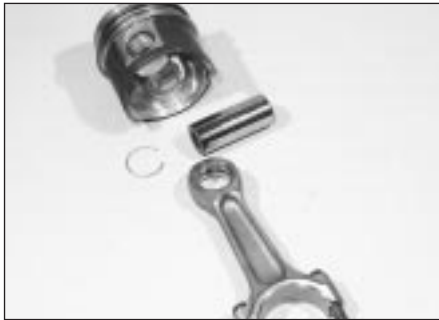
13.15c Piston and connecting rod components
