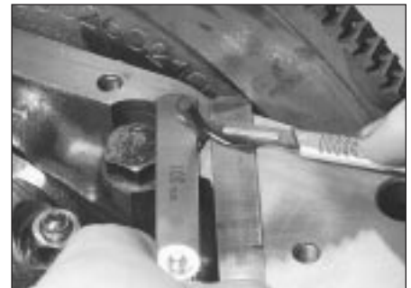
18.74b . . . then trim the sealing strips, so that they protrude above the cylinder block mating surface by approximately 1 mm
