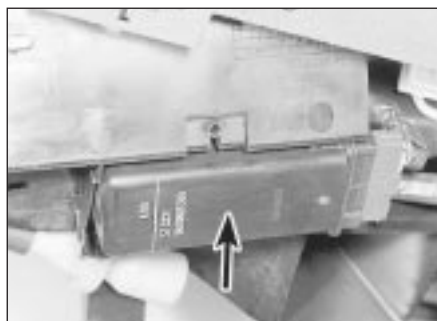
20.1 Central locking electronic control unit (arrowed) viewed with glovebox removed - models up to 1992
