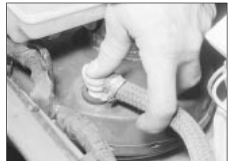
15.7 Pulling the vacuum check valve from the servo
