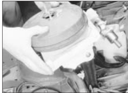
15.15 Removing the vacuum servo/pedal bracket assembly
