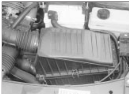
21.7 Air filter housing cover located in the left-hand front of the engine compartment
