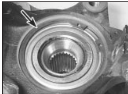
3.3 Front hub bearing retaining circlip (arrowed)
