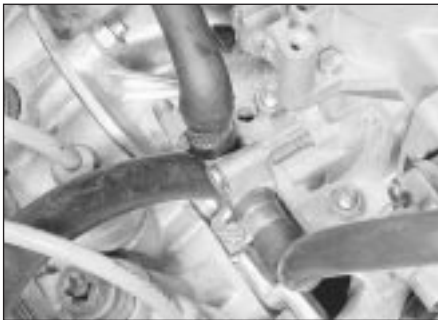
12.6b . . . and base heating pipes
