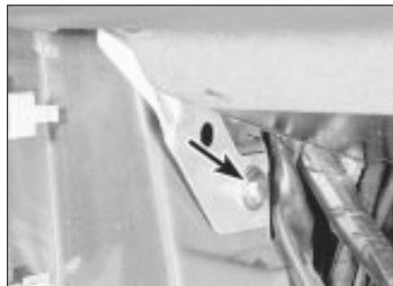
30.21 Lower facia mounting bracket-to-footwell bolt (arrowed)
