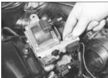
3.5b . . . and remove the coil and mounting bracket from the cylinder head
