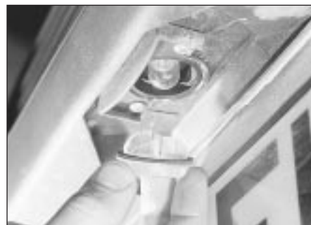
5.39 Prise the lens from the bumper . . .
