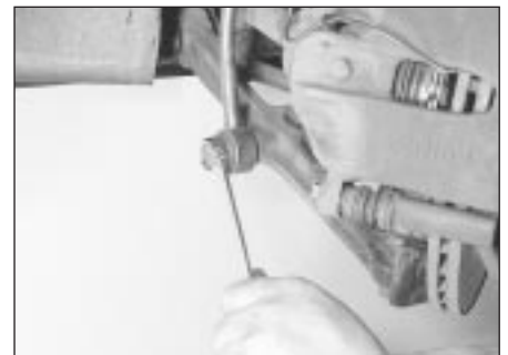
6.2 Remove the bolt securing the anti-roll bar drop link to the lower arm
