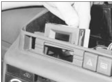
11.5 Removing the clock - models up to 1992
