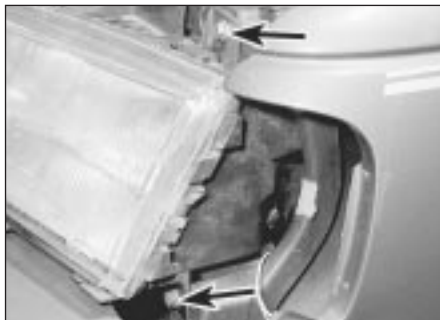
7.8 Outer headlight securing bolts (arrowed)
