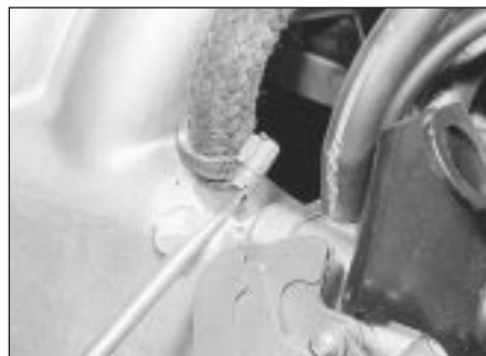
18.3 Disconnecting the brake servo vacuum hose
