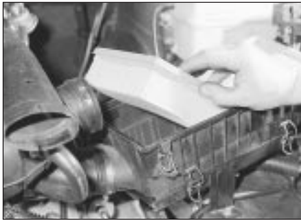
21.9 Removing the air filter element
