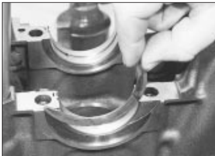
18.53 Fitting a thrustwasher to No 2 main bearing upper location
