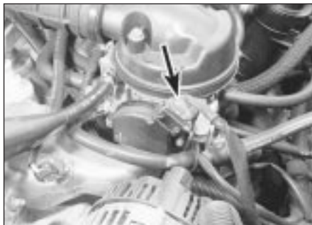
16.14 Throttle potentiometer wiring connector (arrowed)
