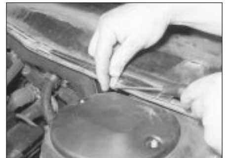
30.64a Remove the securing clip . . .
