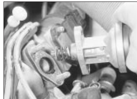
4.5 Removing the fuel pump (XU engine)
