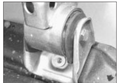
5.26a Undo front mounting through-bolt
