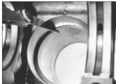
23.6 Checking piston ring gaps
