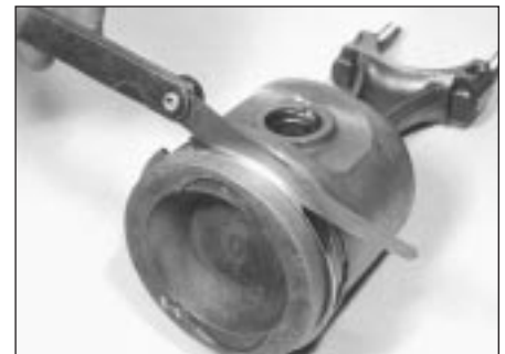
23.7b Checking piston ring-to-groove wall clearance
