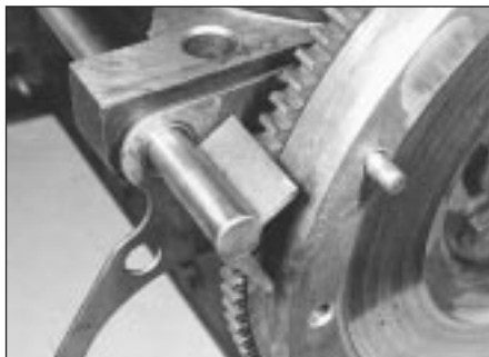
13.2 One method of holding the flywheel stationary
