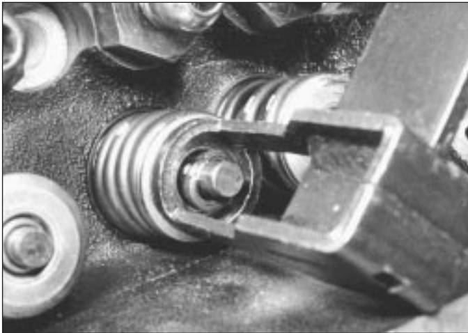
11.2a Compressing a valve spring to remove split collets
