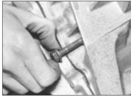
6.6a Undo securing bolts (recessed bolt shown) . . .
