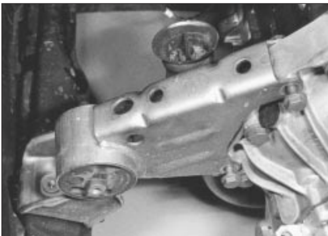
5.26b Unbolt and remove mounting unit
