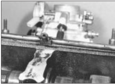
10.7 Removing oil spray tube
