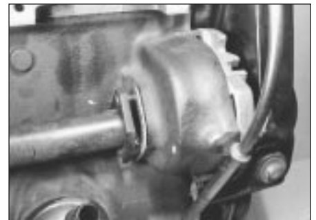
8.1d Removing engine rear coolant pipe
