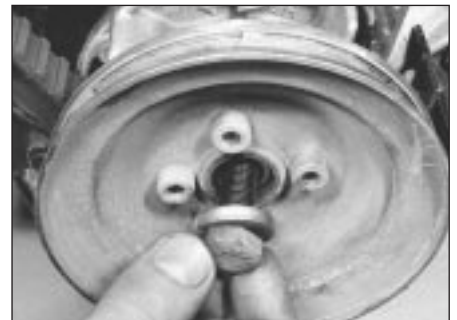
12.7 Removing crankshaft sprocket bolt and washer
