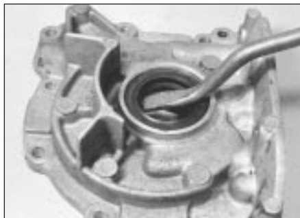
31.1 Prising out oil pump oil seal
