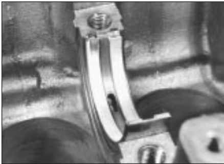
29.2 Fitting centre main bearing shell
