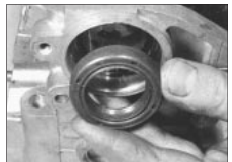
10.15 Removing camshaft oil seal
