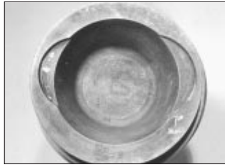
17.5 Piston crown showing arrow which points to timing belt end of engine
