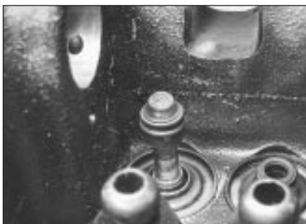
34.4 . . . then fit the new oil seal
