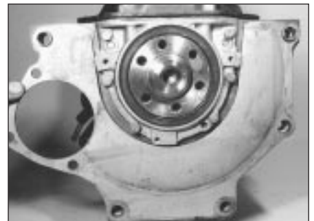
13.4 Removing engine plate
