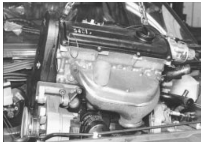
5.28 Lifting out engine/gearbox unit
