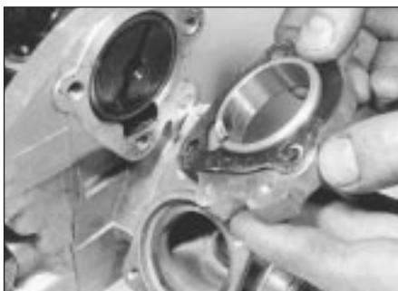
10.13 Removing distributor flange
