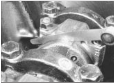
17.4 Checking connecting rod endfloat
