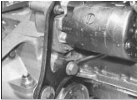
6.3 Starter motor and exhaust support bracket
