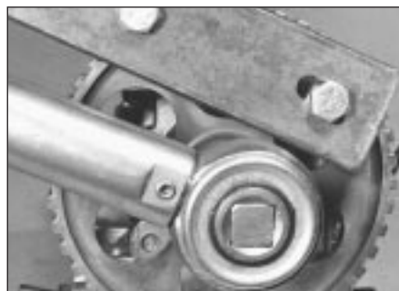
35.5 Method of tightening camshaft sprocket bolt
