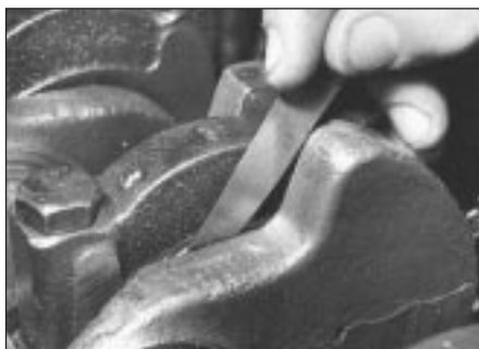
15.3 Checking crankshaft endfloat at No. 3 main bearing
