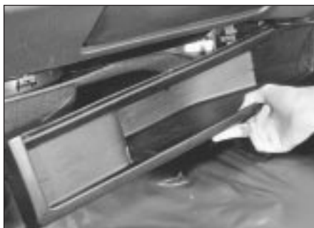
8.6a Removing parcel shelf . . .
