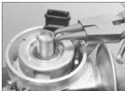
7.4a Remove the locking ring and rotor ...
