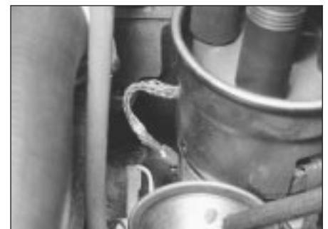
6.2 Transistorised distributor earth lead connection to body (from screen)
