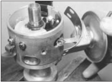
7.5 Vacuum unit removal
