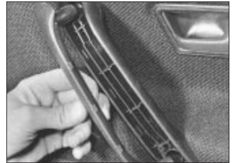
14.3a Removing door pull cover
