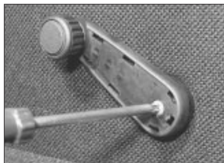
14.4b . . . and handle retaining screw
