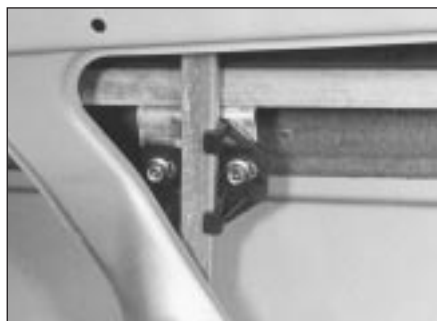
20.3b Lifting plate-to-window channel bolts
