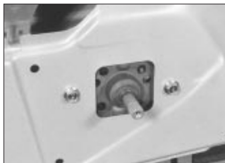
20.3a Window regulator securing bolts
