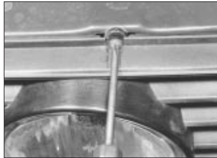
8.2 Undoing front grille retaining screws
