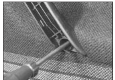
14.3b Removing door pull retaining screws
