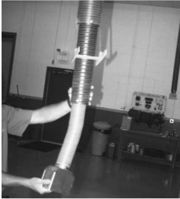
Figure 1-38. Always connect an exhaust hose to the tailpipe of the engine of a vehicle to be run inside a building.
