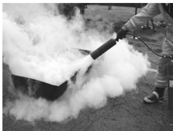
Figure 1-48. A CO 2 fire extinguisher being used on a fire set in an open steel drum during a demonstration at a fire department training center.
