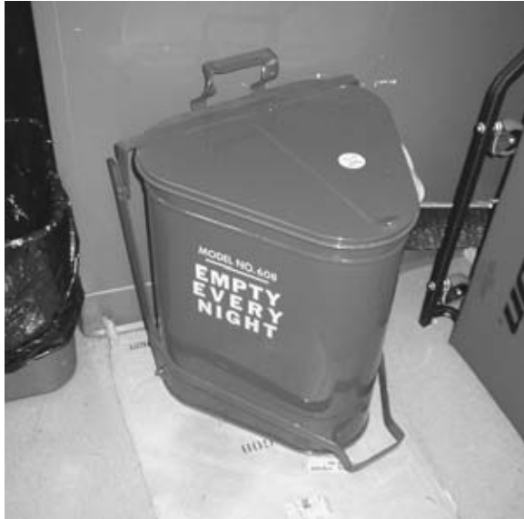
Figure 1-40. All oily shop cloths should be stored in a metal container equipped with a lid to help prevent spontaneous combustion.
