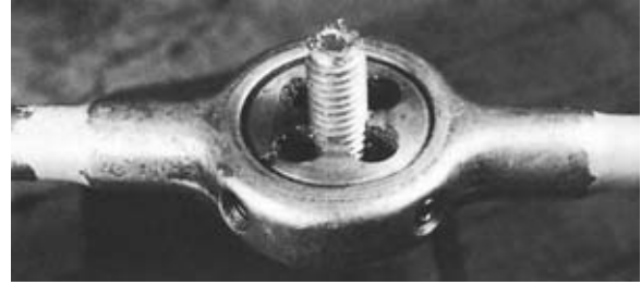
Figure 1-24. Using a die to cut threads on a rod.
