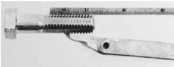
Figure 1-2. Thread pitch gauge is used to measure the pitch of the thread. This is a 1/2-inch-diameter bolt with 13 threads to the inch (1/2–13).
