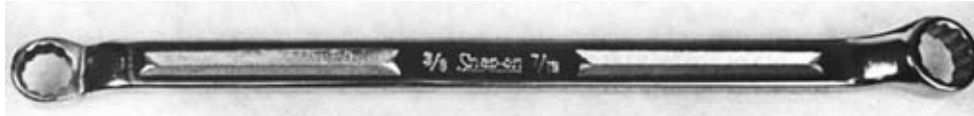
Figure 1-11. Box-end wrench. Recommended to loosen or tighten a bolt or nut where a socket will not fit. A box-end wrench has a different size at each end and is better to use than an open-end wrench because it touches the bolt or nut around the entire head instead of at just two places.
