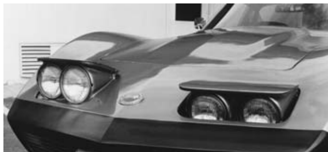
Figure 12-23. Headlamps can be concealed by moving them into and out of the car's bodywork.
