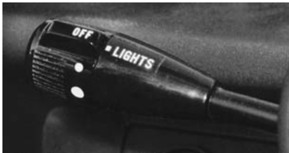
Figure 12-8. Headlamp switches may be mounted on the steering column and operated by a stalk or lever.
