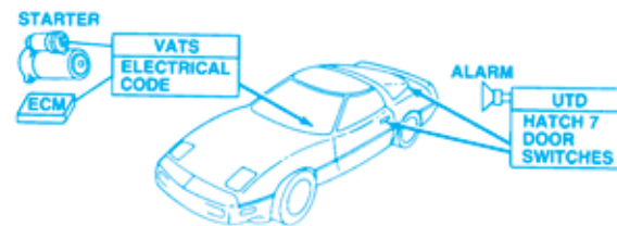
Figure 15-44. Delphi (Delco) VATS system. (GM Service and Parts Operations)
