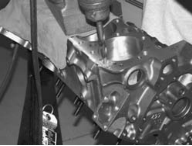
FIGURE 3-30 Drill out the damaged threads with the correct bit.
