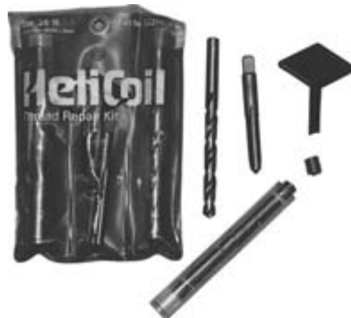
FIGURE 3-27 Helicoil® kits, available in a wide variety of sizes, contain everything needed to repair a damaged hole back to its original size.
