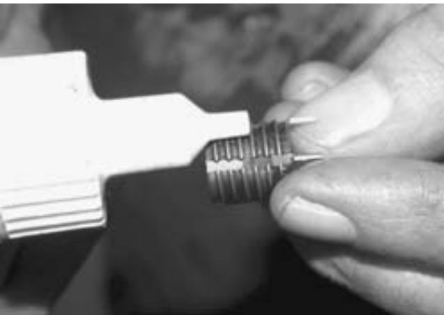
FIGURE 3-32 Put some thread-locking compound on the insert.
