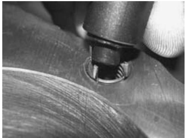
FIGURE 3-33 Use the driver to drive the keys down flush with the surface of the workpiece.
