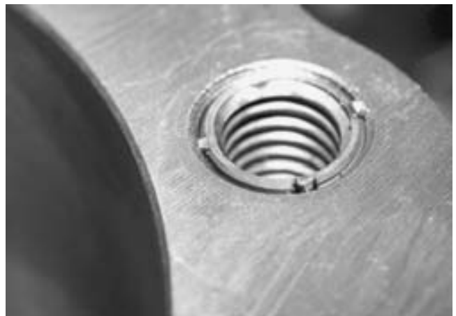
FIGURE 3-34 The insert and insert locks should be below the surface of the workpiece.
