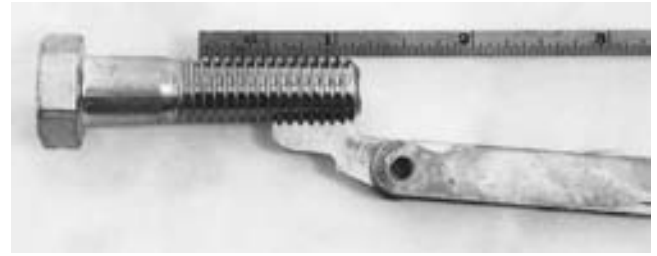
FIGURE 3-2 Thread pitch gauge used to measure the pitch of the thread. This bolt has 13 threads to the inch.
