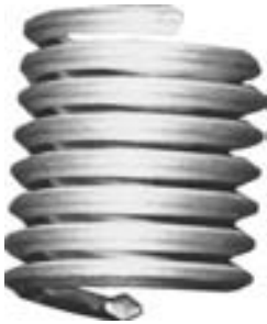
FIGURE 3-25 Helical inserts look like small, coiled springs. The outside is a thread to hold the coil in the hole, and the inside is threaded to fit the desired fastener.
