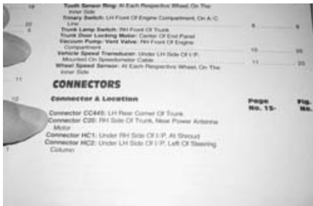
FIGURE 8-14 The component location section of a service manual is very helpful, especially when working on an unfamiliar vehicle.
