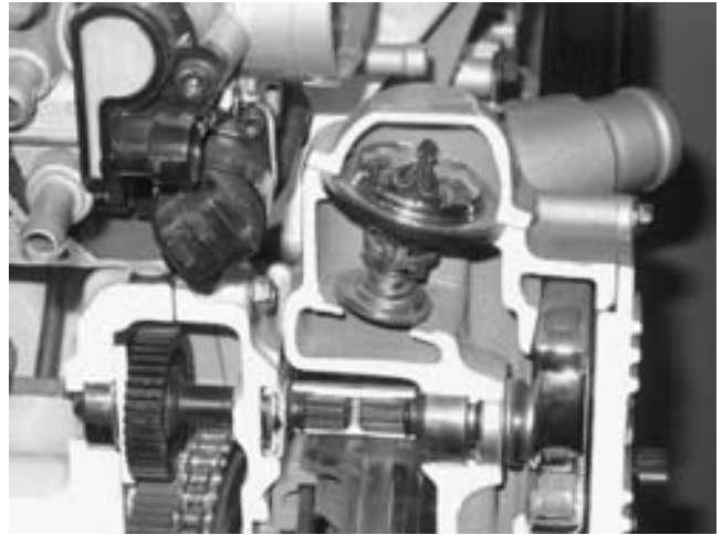
FIGURE 10-3 The coolant temperature is controlled by the thermostat which opens and allows coolant to flow to the radiator when the temperature reaches the rating temperature of the thermostat.
