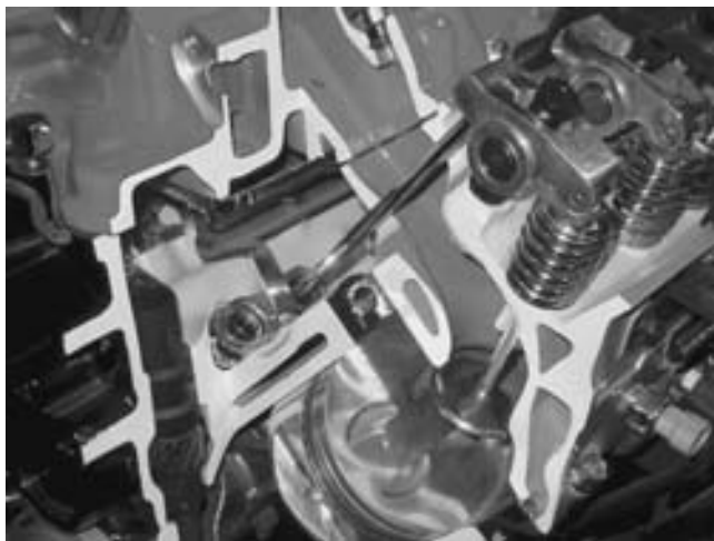
FIGURE 10-11 Cutaway of a V-8 engine showing the lifters, pushrods, roller rocker arms, and valves.
