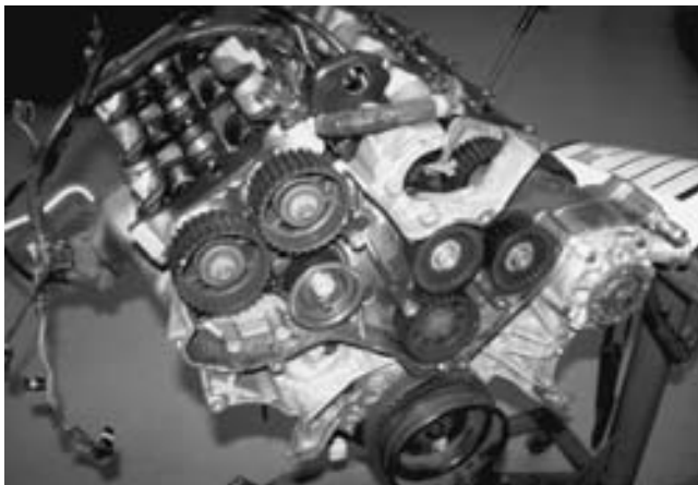
FIGURE 10-13 A dual overhead camshaft (DOHC) V-8 engine with part of the cam cover cut away.
