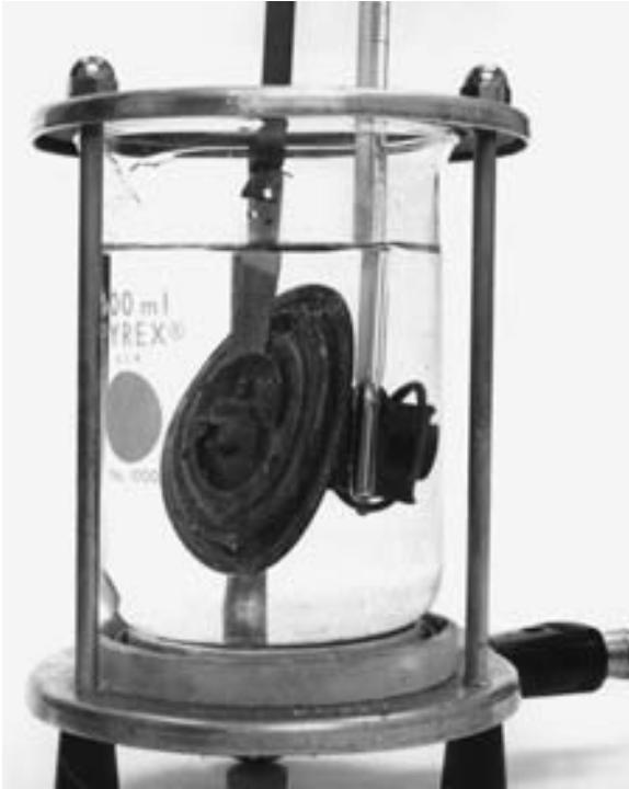
FIGURE 13-10 Setup used to check the opening temperature of a thermostat.
