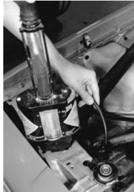
FIGURE 13-15 Checking the freezing and boiling protection levels of the coolant using a hydrometer.
