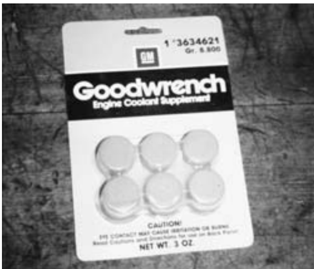
FIGURE 13-40 General Motors recommends that these stop-leak pellets be installed in the cooling system if the coolant is replaced on some engines, especially the Cadillac 4.1, 4.5, and 4.9 L, V-8s.
