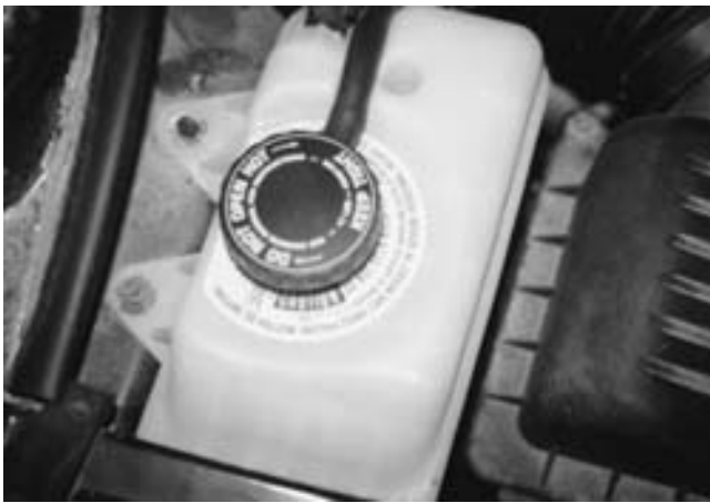
FIGURE 13-22 Some vehicles use a surge tank, which is located at the highest level of the cooling system with a radiator cap.
