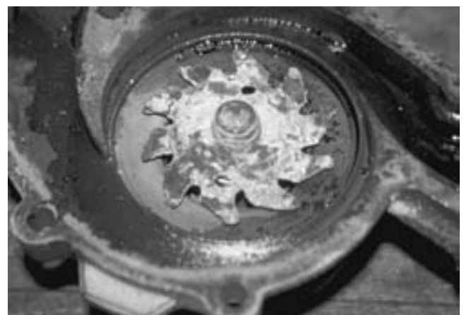
FIGURE 13-32 This severely corroded water pump could not circulate enough to keep the engine cool. As a result, the engine overheated and blew a head gasket.
