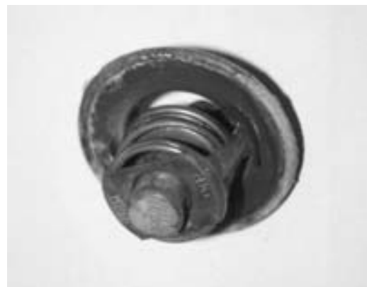
FIGURE 13-7 A thermostat stuck in the open position caused the engine to operate too cold. The vehicle failed an exhaust emission test because of this defect.
