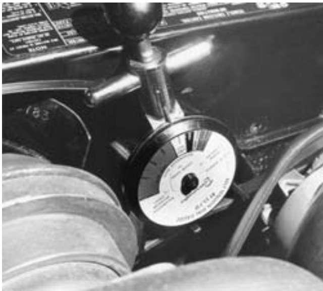
FIGURE 13-42 Drive belt tension is critical for the proper operation of the water pump, as well as the generator (alternator), air-conditioning compressor, and other belt-driven accessories. A belt tension gauge should be used to make certain that accurate belt tension is achieved when replacing or retensioning any belt.
