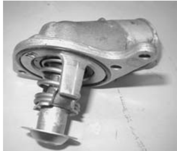
FIGURE 13-11 Some thermostats are an integral part of the housing. This thermostat and radiator hose housing is serviced as an assembly. Some thermostats simply snap into the engine radiator fill tube underneath the pressure cap.
