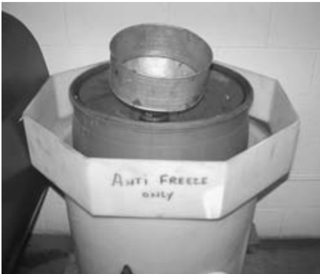
FIGURE 13-16 Used antifreeze coolant should be kept separate and stored in a leak-proof container until it can be recycled or disposed of according to federal, state, and local laws. Note that the storage barrel is placed inside another container to catch any coolant that may spill out of the inside barrel.
