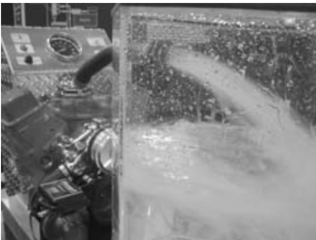
FIGURE 13-28 A demonstration engine running on a stand, showing the amount of coolant flow that actually occurs through the cooling system.
