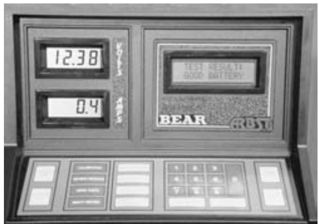
FIGURE 15-13 A Bear Automotive starting and charging tester. This tester automatically loads the battery for 15 seconds to remove the surface charge, then waits 30 seconds to allow the battery to recover, then again loads the battery. The display indicates the status of the battery.
