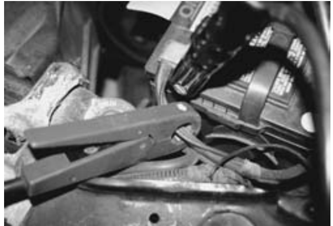
FIGURE 15-26 When connecting an inductive ammeter probe, be certain that the pickup is over all wires. The probe will work equally well over either all positive or all negative cables, because all current leaving a battery must return.
