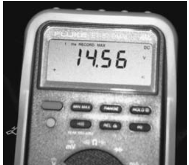
FIGURE 15-23 The digital multimeter should be set to read DC volts; the red lead is connected to the battery positive (+) terminal and the black meter lead is connected to the negative (-) battery terminal.
