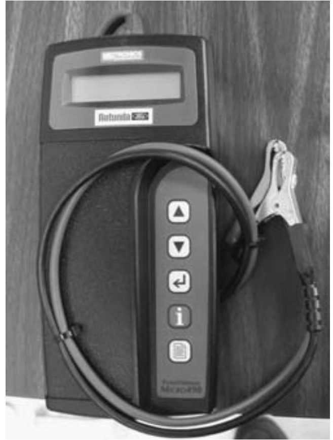
FIGURE 15-14 A typical electronic battery tester which, depending on the model, can also be used to test the starting and the charging systems.
