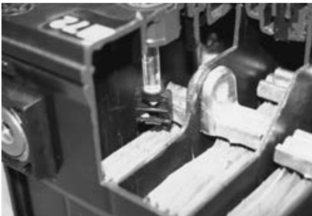
FIGURE 15-6 Cutaway of the battery showing the charge indicator. If the electrolyte level drops below the bottom of the prism, the sight glass shows clear (light). Most battery manufacturers warn that if the electrolyte level is low on a sealed battery, the battery must be replaced. Attempting to charge a battery that has a low electrolyte level can cause a buildup of gases and possibly an explosion.
