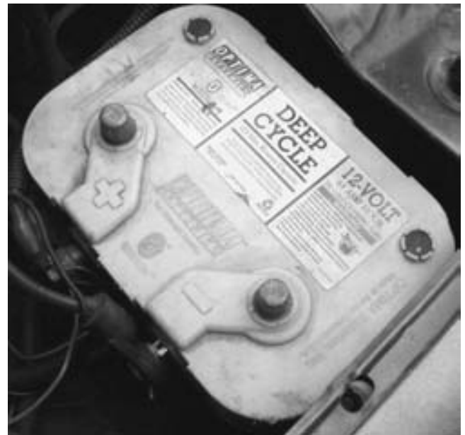
FIGURE 15-7 An example of an AGM battery. An AGM battery requires a special charger that allow the battery to be charged at a high current (ampere) rate but not over 15 volts. Conventional chargers often exceed 16 volts.
