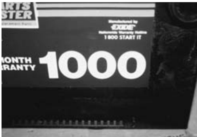
FIGURE 15-8 This battery has a cranking amperes (CA) rating of 1000, which means that this battery is capable of supplying 1000 amperes to crank an engine for 30 seconds at a temperature of 32°F (0°C) at a minimum of 1.2 volts per cell (7.2 volts for a 12-volt battery).
