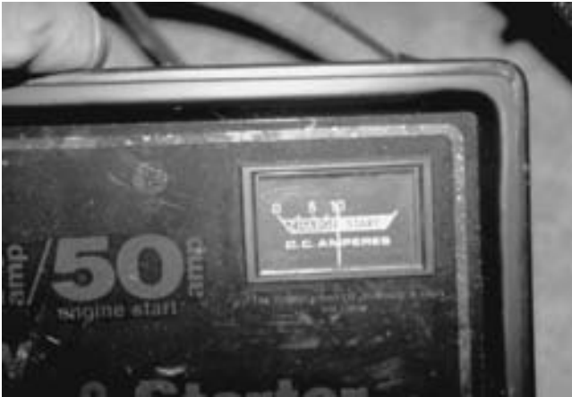
FIGURE 15-15 This battery charger is charging the battery at a 10-ampere rate. A slow rate such as this is easier on the battery than a fast charge that may overheat the battery and cause warpage of the plates inside the battery.
