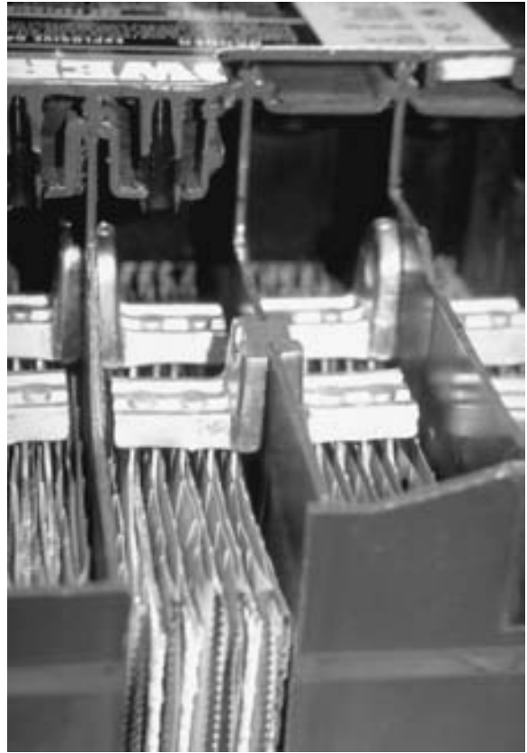
FIGURE 15-1 Photo of a cutaway battery showing the connection of the cells to each other through the partition.
