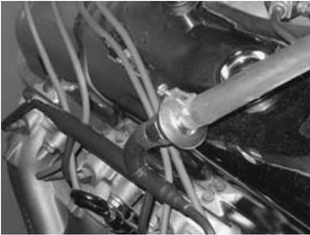
FIGURE 17-24 An AIR exhaust check valve between the rubber air hose and the metal discharge tubes.
