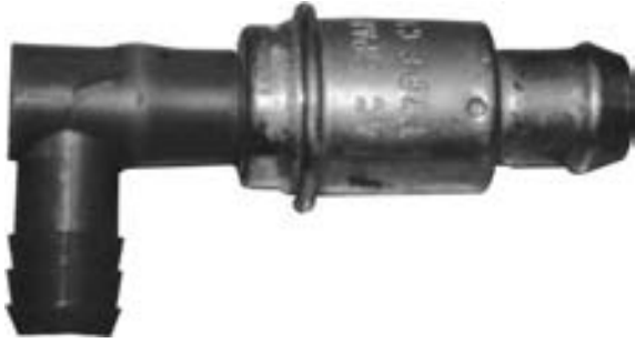
FIGURE 17-19 A typical PCV valve. A defective or clogged PCV valve or hose can cause a rough idle or stalling problem. Because the air flow through the PCV valve accounts for about 20% of the air needed by the engine at idle, use of the incorrect valve for an application could have a severe effect on idle quality.
