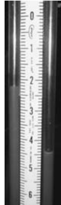
FIGURE 17-21 A water manometer being used to check for a slight vacuum when testing at the oil dipstick tube.
