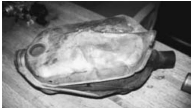
FIGURE 17-36 This catalytic converter blew up when gasoline from the excessively rich-running engine ignited. Obviously, raw gasoline was trapped inside and all it needed was a spark. No further diagnosis of this converter is necessary. However, the fuel and ignition systems would need to be tested and repaired before operating the engine to prevent a recurrence.
