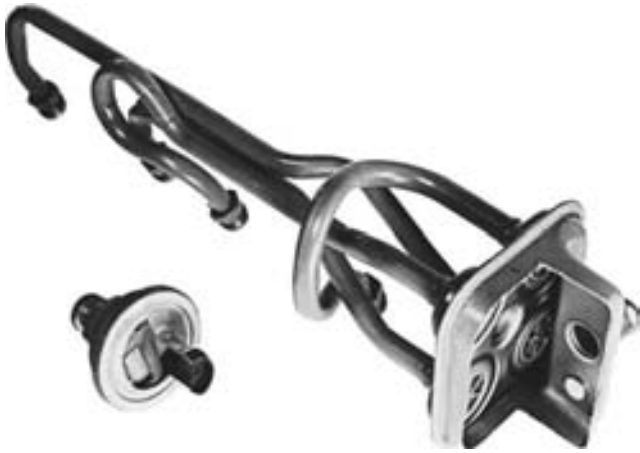
FIGURE 17-28 Cutaway of a pulse air-driven air device used on many older engines to deliver air to the exhaust port through the use of the exhaust pulses acting on a series of one-way check valves. Air from the air cleaner assembly moves through the system and into the exhaust port where the additional air helps reduce HC and CO exhaust emissions.
