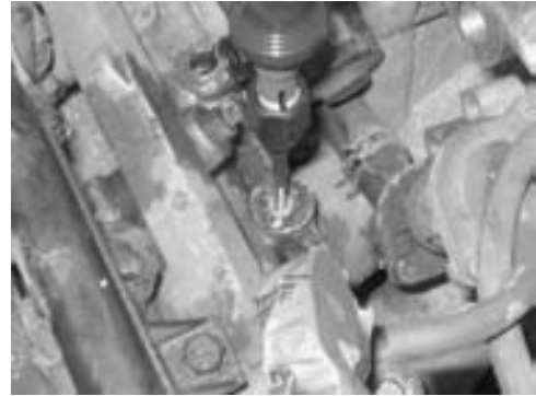
FIGURE 17-11 Removing the EGR passage plugs from the intake manifold on a Honda.
