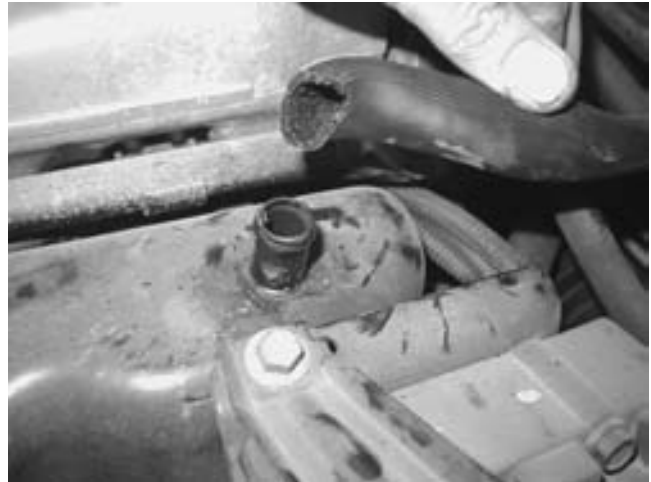
FIGURE 17-18 A visual inspection found this deteriorated PCV vacuum hose.
