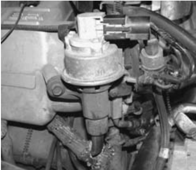
FIGURE 17-4 An EGR valve position sensor on top of an EGR valve.
