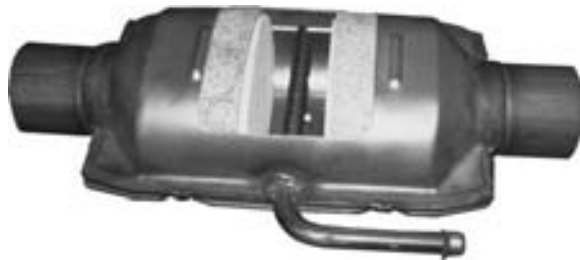
FIGURE 17-32 A cutaway of a three-way catalytic converter showing the air tube in the center of the reducing and oxidizing section of the converter. Note the small holes in the tube to distribute air from the AIR pump to the oxidizing rear section of the converter.
