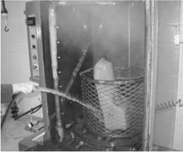
FIGURE 21-17 A pressure jet washer is similar to a large industrial-sized dishwasher. The part(s) is then rinsed with water to remove chemicals or debris that may remain on the part while it is still in the tank.
