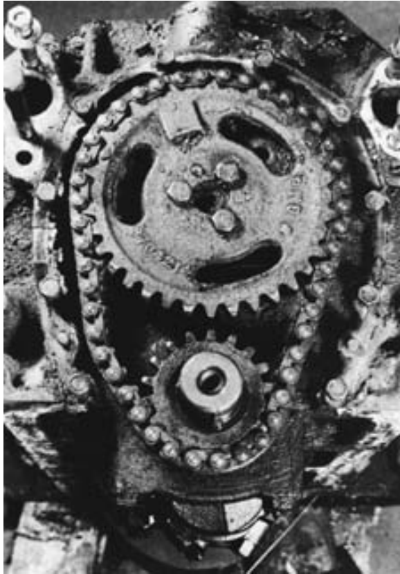
FIGURE 21-10 Worn timing chain on a high-mileage engine. Notice that the timing chain could “jump a tooth” at the bottom of the smaller crankshaft gear where the chain is in contact with fewer teeth. Notice also that the technician placed all of the bolts back in the block after removal of the part. This procedure helps protect against lost or damaged bolts and nuts.
