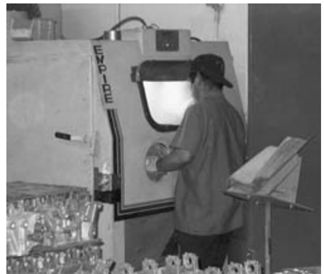
FIGURE 21-19 Small engine parts can be blasted clean in a sealed cabinet.
