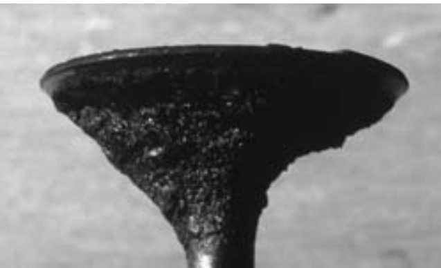
FIGURE 21-14 After removing this intake valve, it became obvious why this engine had been running so poorly.
