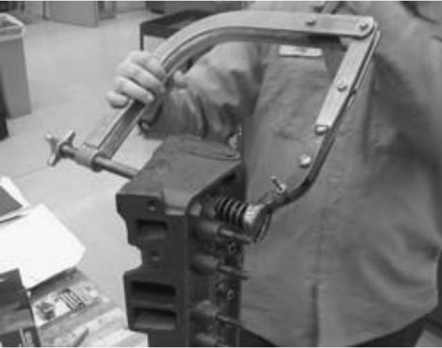
FIGURE 21-13 A valve spring compressor being used to remove the valve keepers (locks).
