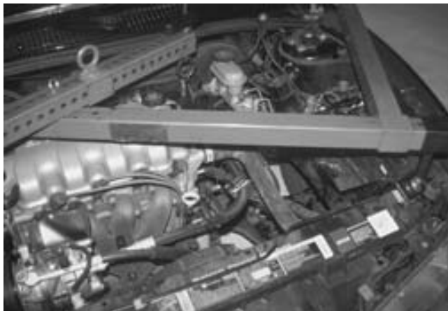
FIGURE 21-2 When removing just the engine from a front-wheel-drive vehicle, the transaxle must be supported. Shown here is a typical fixture that can be used to hold the engine if the transaxle is removed or to hold the transaxle if the engine is removed.
