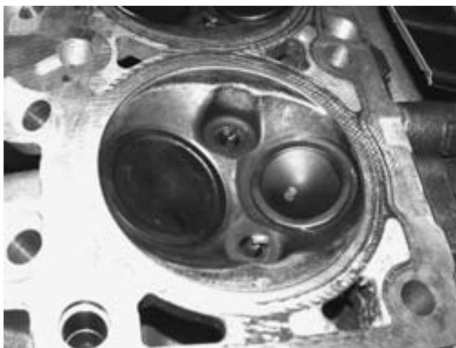
FIGURE 22-4 The combustion chamber of the 5.7 liter Chrysler Hemi cylinder head showing the two spark plugs used to ensure rapid burn for best power and economy with the lowest possible exhaust emissions.
