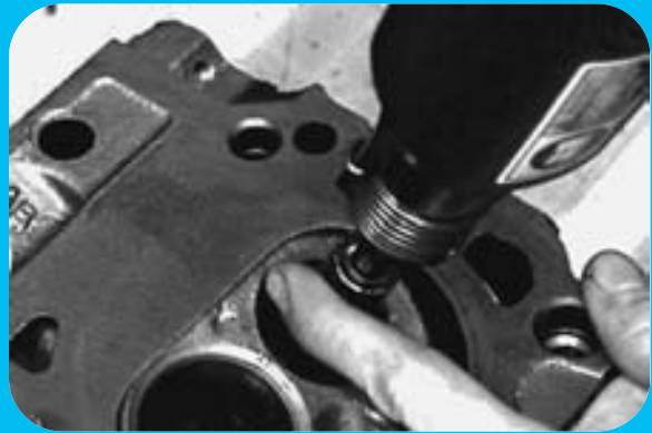
STEP 8 Using an installer to force the thin-wall bronze guide fully into the guide from the combustion chamber side of the head.
