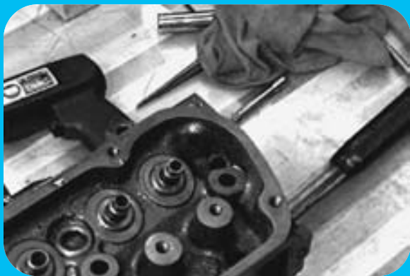
STEP 9 The thin-wall bronze guide insert is longer than the guide and protrudes out of the top of the original guide.
