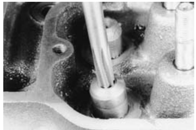
FIGURE 22-35 Reaming a valve guide to be oversize. This permits the use of new valves with oversize stem diameters. Many remanufacturers use this method to save the money and time involved in replacing or knurling valve guides and grinding old valves.
