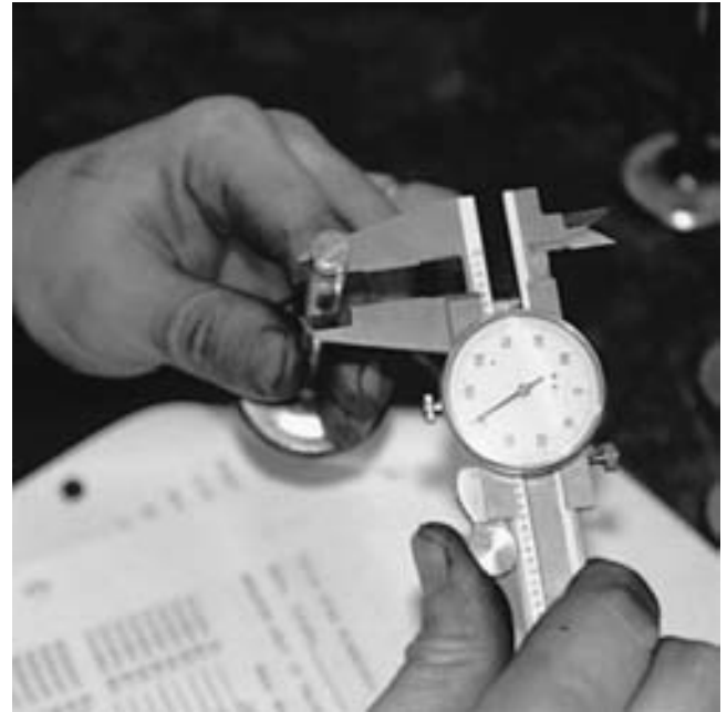
FIGURE 22-34 Using a vernier dial caliper to measure the valve stem diameter of a valve. Subtract the diameter of the valve stem from the inside diameter of the valve guide to determine the valve guide clearance.
