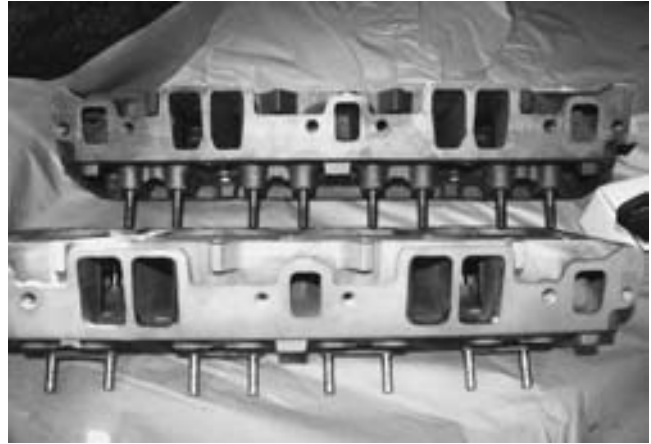
FIGURE 22-16 The top cylinder head is stock and the bottom cylinder head has been ported using two different methods. The first inch from the gasket surface has been ground using a grinder to make the opening in the cylinder head match the intake manifold. The rest of the port between the valve and the gasket surfaces has been enlarged using acid. This acid treatment is a common “trick” used to increase the flow characteristics of a stock class cylinder head. The acid treatment gives the same rough cast-like surface as a completely stock cylinder head.
