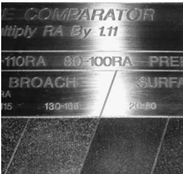
FIGURE 22-28 A commercially available surface finish comparator is often used to judge the surface finish without the expense of an expensive electronic tester.
