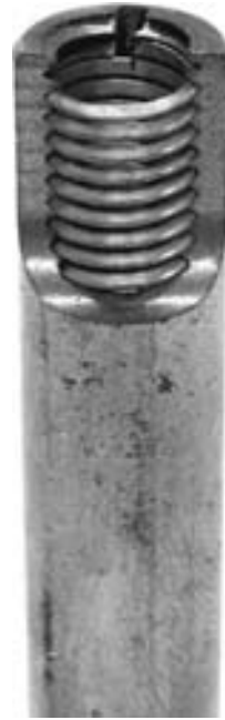
FIGURE 22-42 Installed spiral bronze insert bushing.
