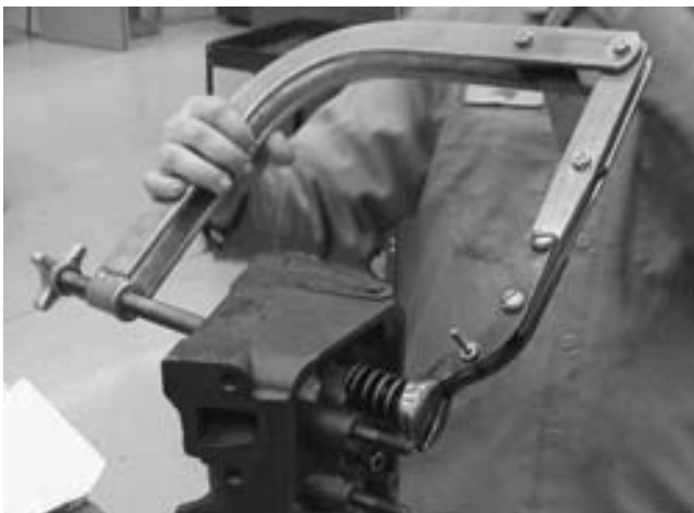
FIGURE 22-21 A valve spring compressor being used to compress the valve springs so the valve locks (keepers) can be removed and the valve removed from the cylinder head.
