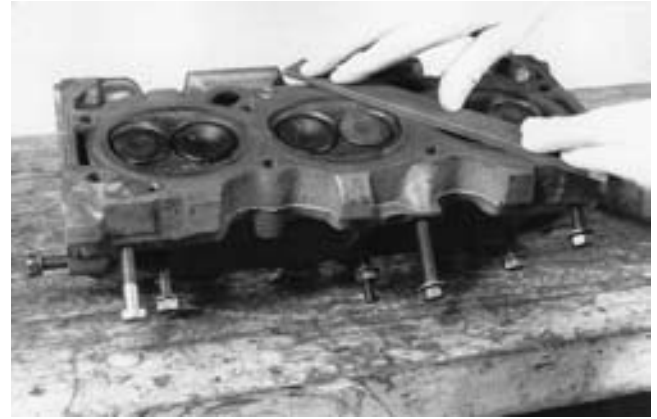
FIGURE 22-23 After scraping the gasket surface with a scraper, use a file and draw across the surface. When a file is drawn across the head sideways, little (if any) material is removed, but burrs and other surface imperfections are removed or highlighted.
