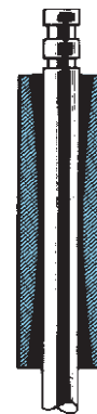
FIGURE 22-31 Valve guides often wear to a bell-mouth shape to both ends due to the forces exerted on the valve by the valve train components.
