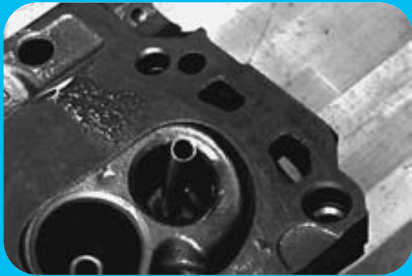
STEP 7 Installing the thin-wall bronze guide insert.
