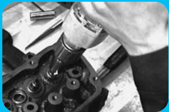
STEP 10 The top of the thin-wall bronze guide insert is then trimmed to the same level as the original integral guide.
