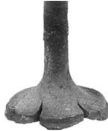
FIGURE 23-18 Badly guttered valve face.
