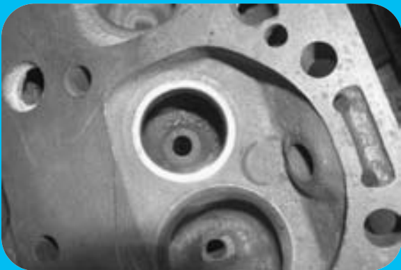
STEP 15 A new valve seat is now ready to be machined or cut.
