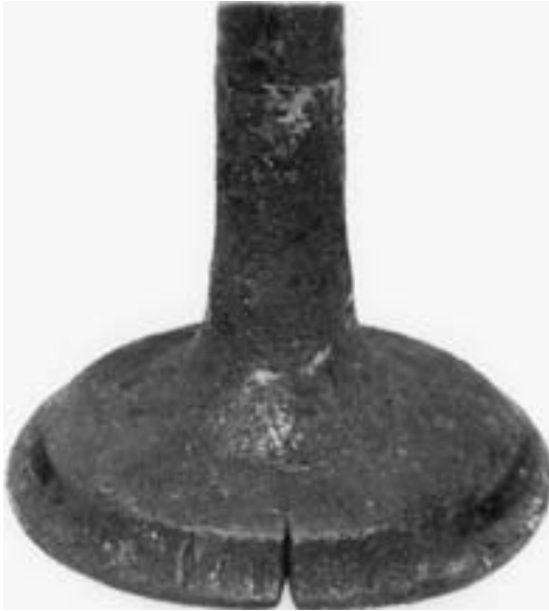
FIGURE 23-12 Valve face guttering.
