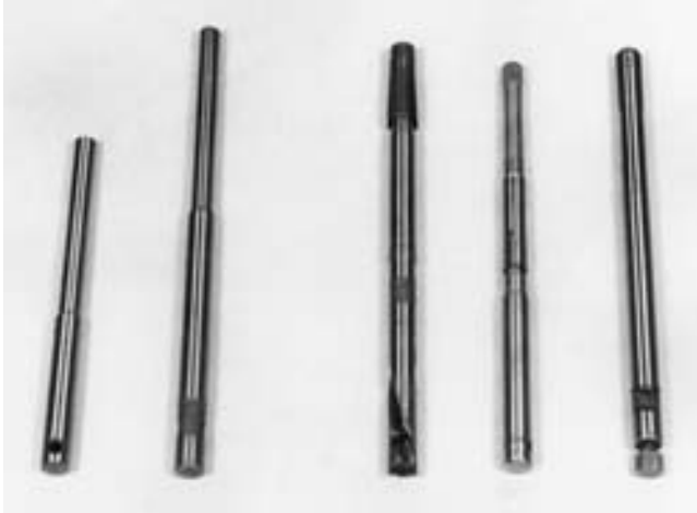
FIGURE 23-53 The two pilots on the left are of a solid tapered type. The three pilots on the right are adjustable (expandable) types.
