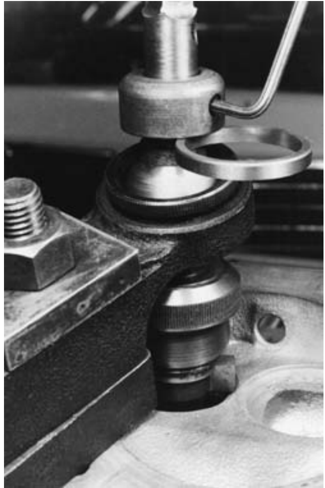
FIGURE 23-67 Adjusting the cutting tool stop ring with the new valve insert as a guide.
