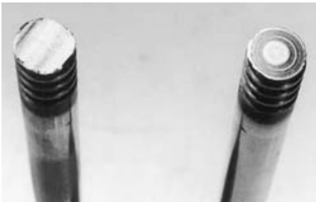
FIGURE 23-26 Excessive valve tip wear.
