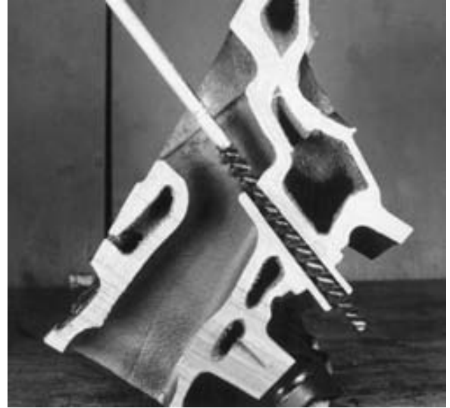
FIGURE 23-54 Sectioned head showing how a brush valve guide cleaner is used.
