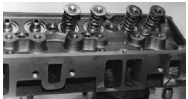
FIGURE 23-86 Cylinder head setup for flow testing. Note the weak valve springs that are strong enough to keep the valves shut, yet weak enough to permit the flow bench operator to vary the intake valve opening amount.
