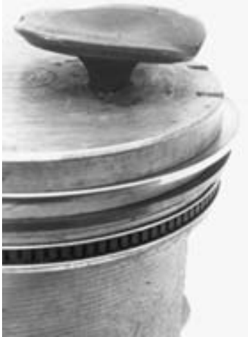
FIGURE 23-23 Everything in the valve train has to be working correctly or an engine can be destroyed. The valve in this engine separated from the retainer at high engine speed, turned around in the cylinder, and punctured the piston.
