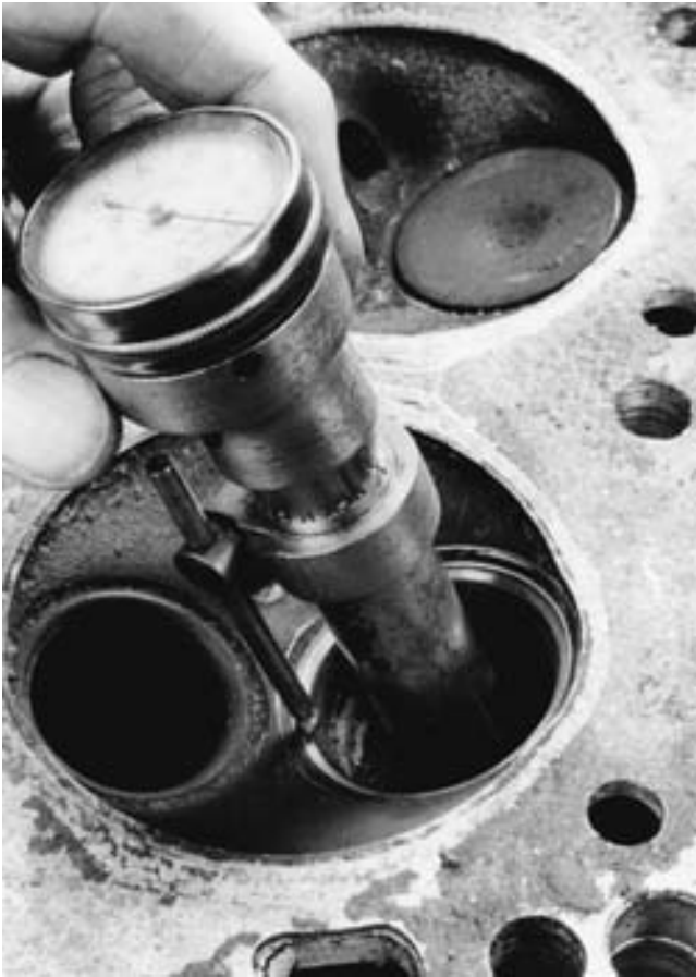
FIGURE 23-61 Typical dial indicator-type of micrometer for measuring valve seat concentricity.
