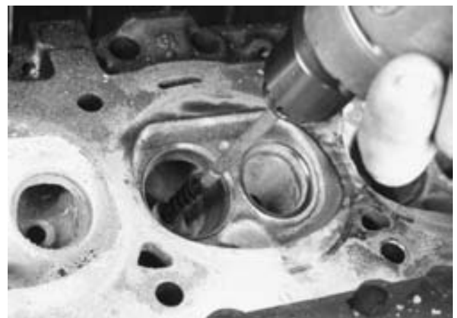
FIGURE 23-55 Using a valve guide brush with an electric drill. This cleaning of the valve guides is very important for proper valve seat reconditioning.
