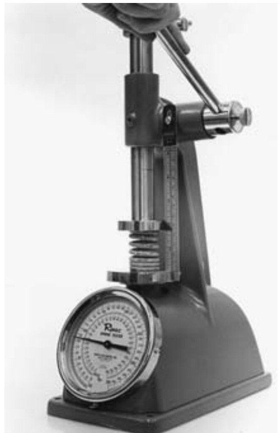
FIGURE 23-32 One popular type of valve spring tester used to measure the compressed force of valve springs. Specifications usually include (1) free height (height without being compressed), (2) pressure at installed height with valve closed , and (3) pressure with valve open the maximum amount and height to specifications.
