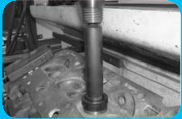
STEP 14 Using the air hammer or press, press the valve seat into the valve pocket.
