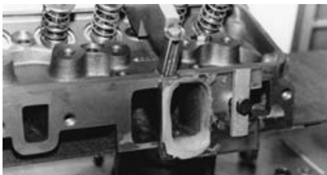
FIGURE 23-87 Modeling clay is installed around the port to duplicate the flow improvement characteristics of an intake manifold.
