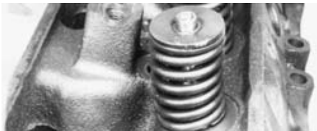
FIGURE 23-31 Out-of-square valve spring. This spring should not be tested further, but should be replaced. A distorted valve spring exerts side loads on the valve, which often causes excessive valve guide wear.
