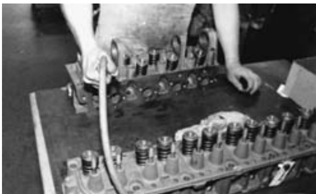
FIGURE 23-64 Testing for leakage past the valves by injecting compressed air into the combustion chamber through the spark plug hole. To prevent leakage at the head gasket surface, the cylinder head is placed on a foam rubber pad.
