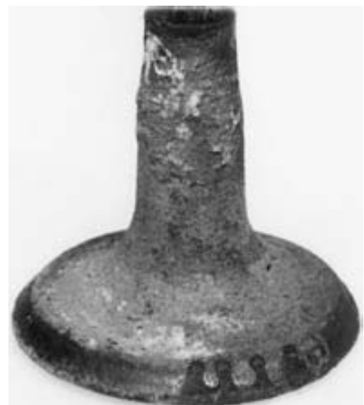
FIGURE 23-11 Valve face burning.
