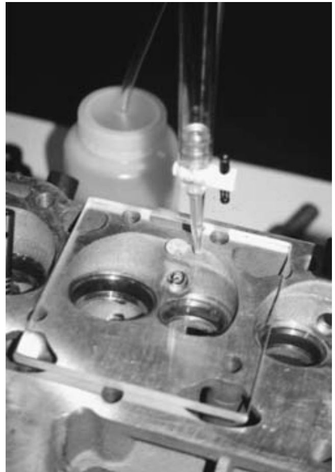
FIGURE 23-80 Setup needed to measure the combustion chamber volume in cubic centimeters (cc).
