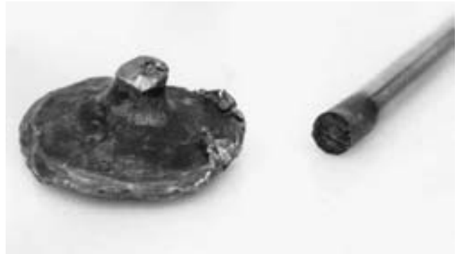
FIGURE 23-21 Valve head broken from the stem.
