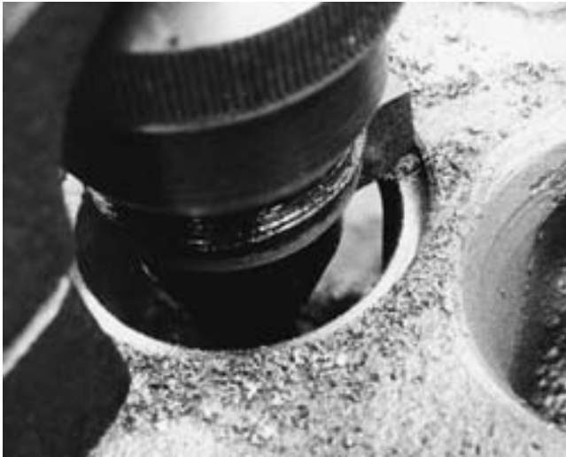
FIGURE 23-68 Seat cutting tool boring out the old eroded valve seat.
