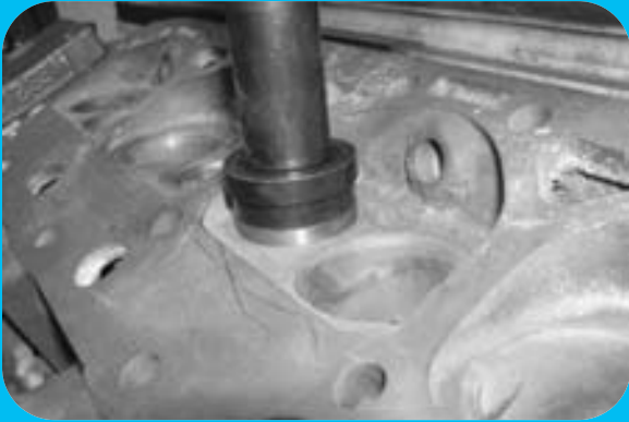
STEP 13 Install the correct size driver onto the valve seat.
