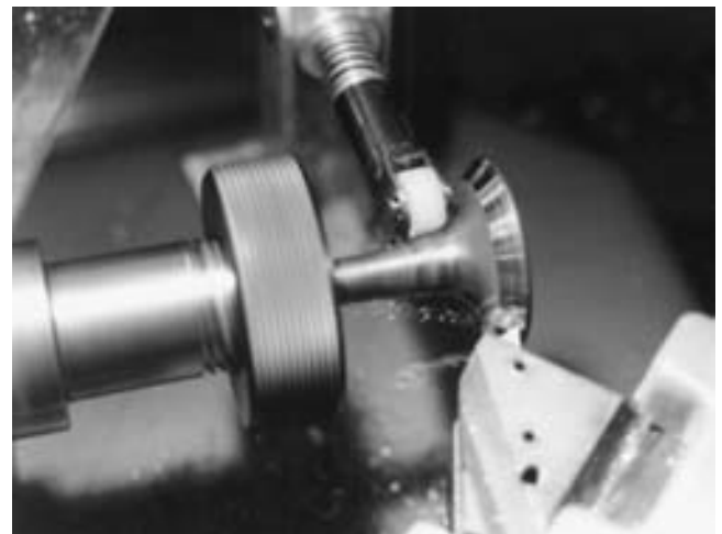
FIGURE 23-44 Refacing a valve on a lathe using a special silicon carbide tool bit. The valve face is smoother than it would have been if the valve had been refaced with a stone.
