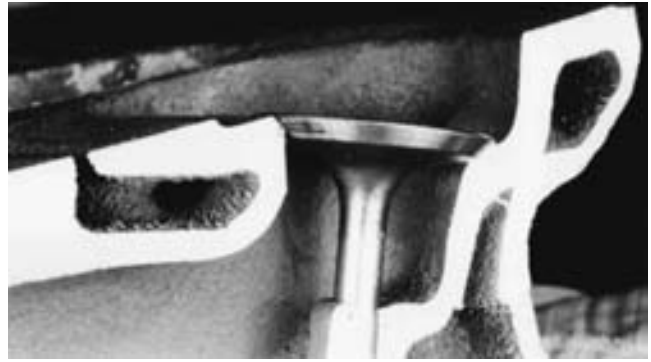
FIGURE 23-62 On this cutaway head, the location of the valve seat is shown where the ink from the felt-tip pen has transferred from the seat to the valve face. Prussian blue can also be used instead of a felt-tip marker.
