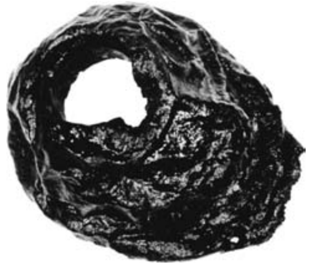
FIGURE 23-79 Poor-quality umbrella-type valve stem seal after several months of use. Note how heat has softened this seal and destroyed its sealing ability.
