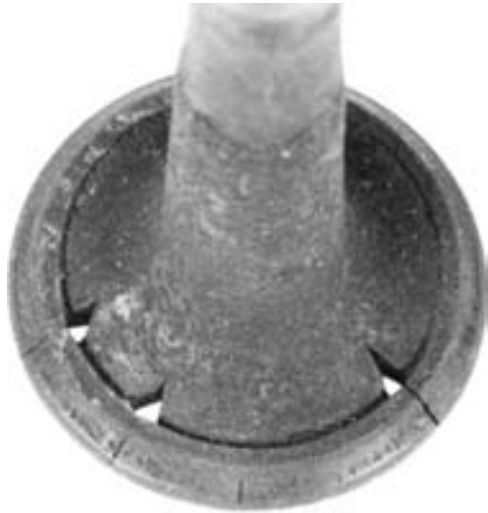
FIGURE 23-19 Hoop stress cracks in a valve head.
