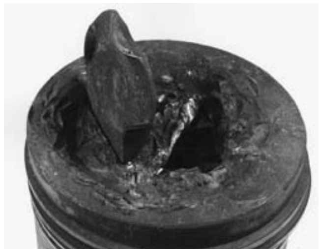
FIGURE 23-22 Broken piston caused by a valve breaking from the stem.
