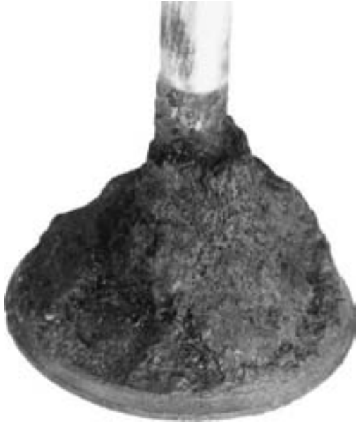
FIGURE 23-16 Intake valve with heavy deposits.
