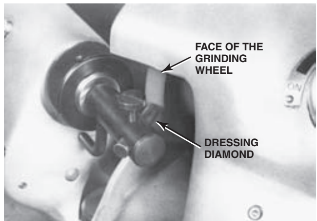
FIGURE 23-40 Dressing the face of the grinding wheel with a diamond dressing tool. This operation helps ensure a good-quality valve face finish.
