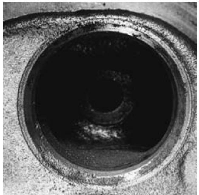
FIGURE 23-65 Badly eroded valve seat.
