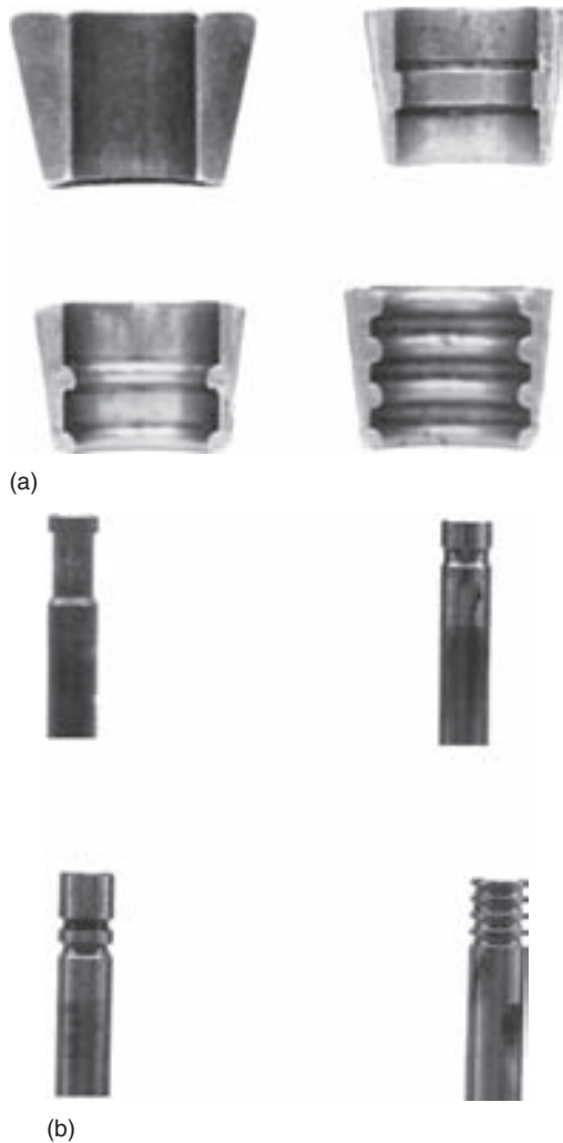
FIGURE 23-33 Valve split lock types (a) and stem grooves (b).
