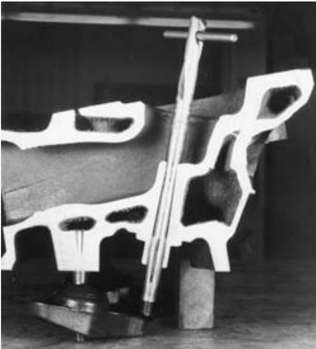
FIGURE 23-56 Expandable pilot shown in the valve guide of a sectioned head to illustrate how the pilot fits.
