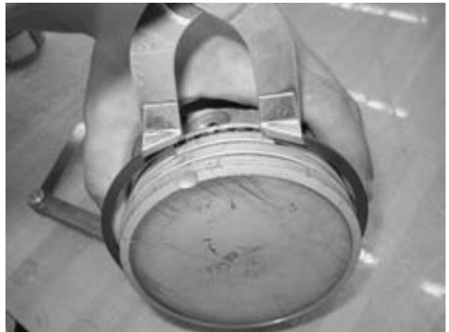
FIGURE 25-49 A typical ring expander being used to install a piston ring.
