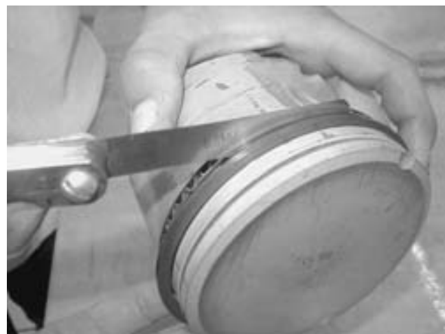
FIGURE 25-46 The side clearance of the piston ring is checked with a thickness (feeler) gauge.
