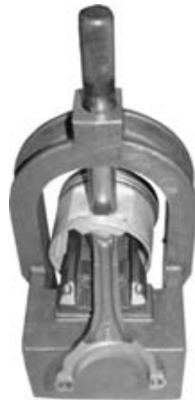
FIGURE 25-31 A press used to remove the connecting rod from the piston.
