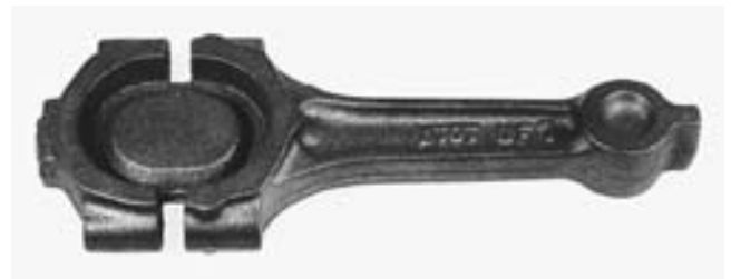
FIGURE 25-34 Rough casting for a connecting rod.
