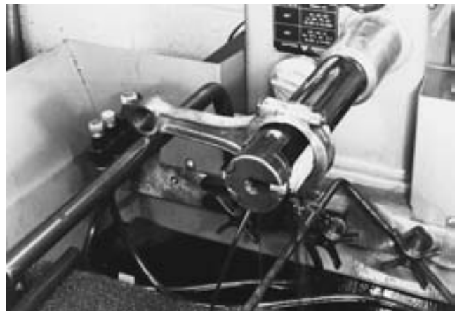
FIGURE 25-43 Resizing the big end of the connection rod with a hone. To help ensure a more accurate and straighter job, hone two connecting rods at a time.
