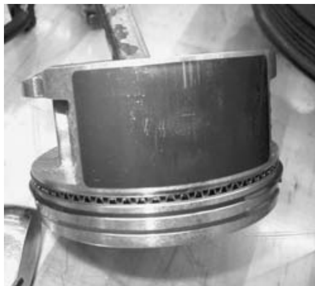
FIGURE 25-7 A moly graphite coating on the skirt of this piston from a General Motors 3800 V-6 engine helps prevent piston scuffing when the engine is cold.
