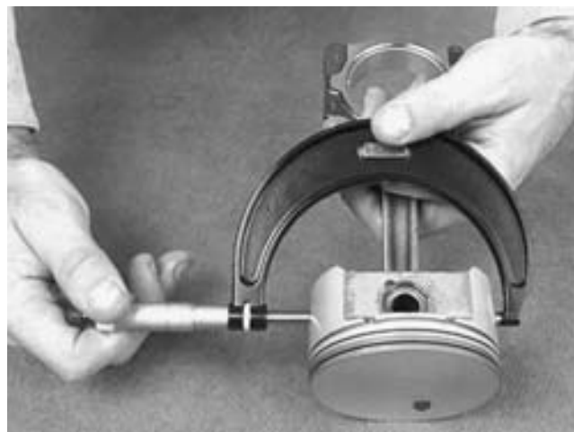
FIGURE 25-6 A piston diameter is measured across the thrust surfaces.
