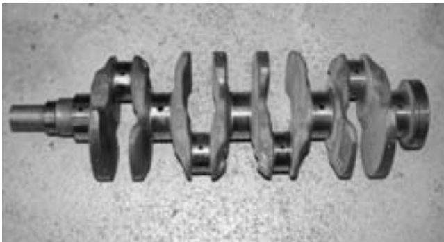
FIGURE 27-10 A fully counterweighted 4-cylinder crankshaft.
