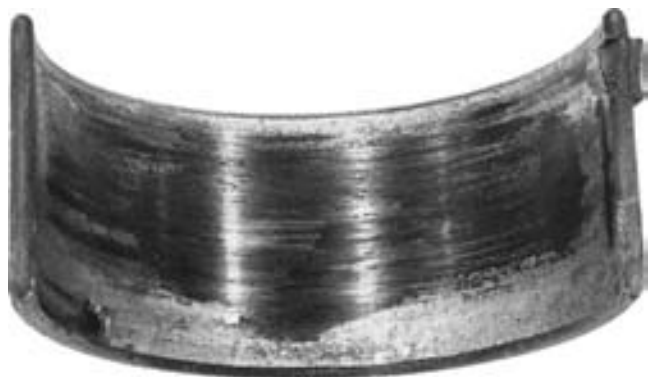
FIGURE 27-31 Bearing wear caused by a misaligned journal. A bent connecting rod could also cause similar bearing wear.
