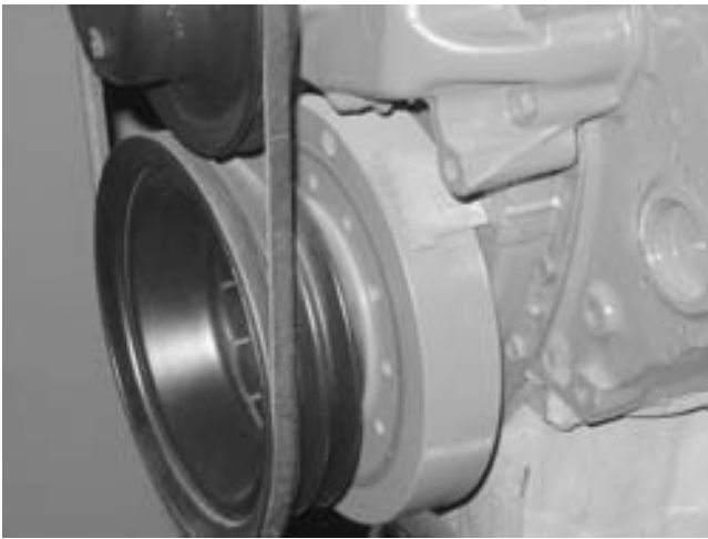
FIGURE 27-13 This Chevy V-8 harmonic balancer also has a line cut into the outer ring that is used to indicate top dead center to set the ignition timing on engines that are equipped with a distributor ignition.
