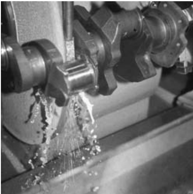
FIGURE 27-21 A crankshaft being ground.
