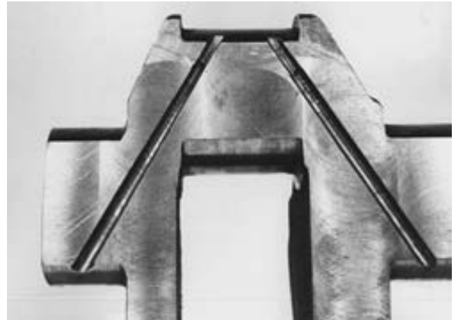
FIGURE 27-16 Crankshaft sawed in half, showing drilled oil passages between the main and rod bearing journals.
