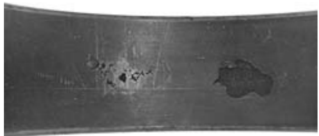
FIGURE 27-30 Bearing material missing from the bearing as a result of fatigue failure.
