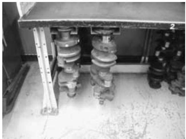
FIGURE 27-47 Crankshafts should be stored vertically to prevent possible damage or warpage. This clever bench-mounted tray for crankshafts not only provides a safe place to store crankshafts but it is out-of-the-way and cannot be accidentally tipped.
