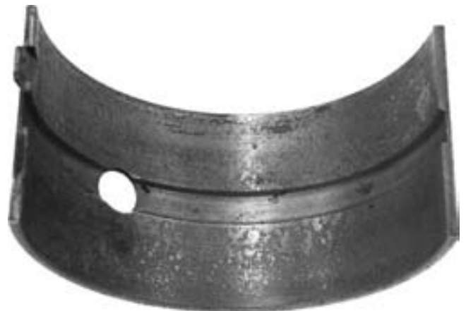
FIGURE 27-33 Foreign particles such as dirt embedded in the bearing material.
