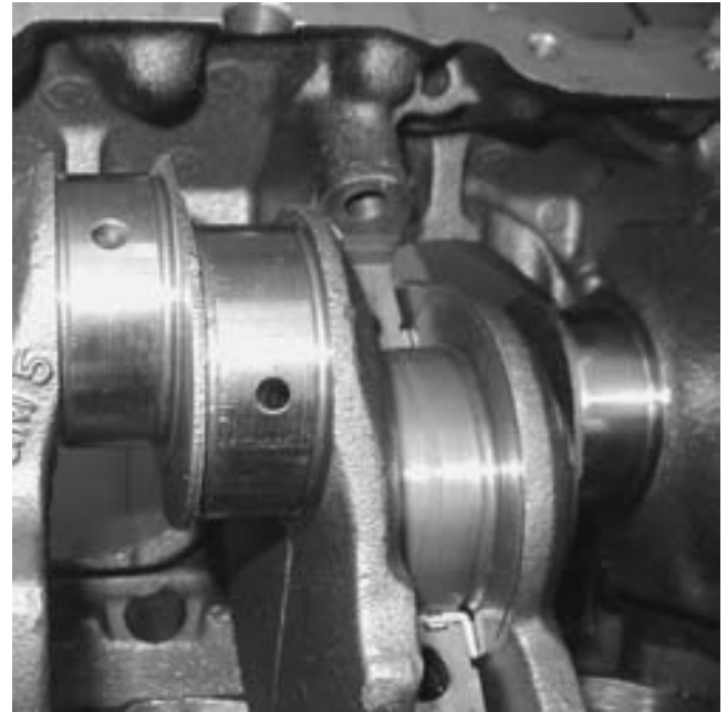
FIGURE 27-4 A ground surface on one of the crankshaft cheeks next to a main bearing supports thrust loads on the crank.
