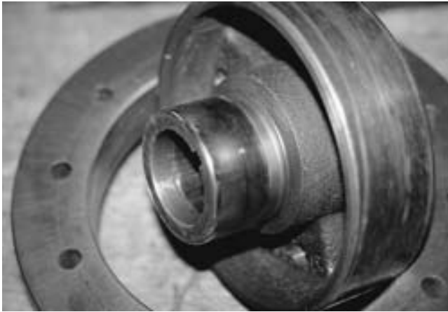
FIGURE 27-15 Harmonic balancer that separated at high engine speed.
