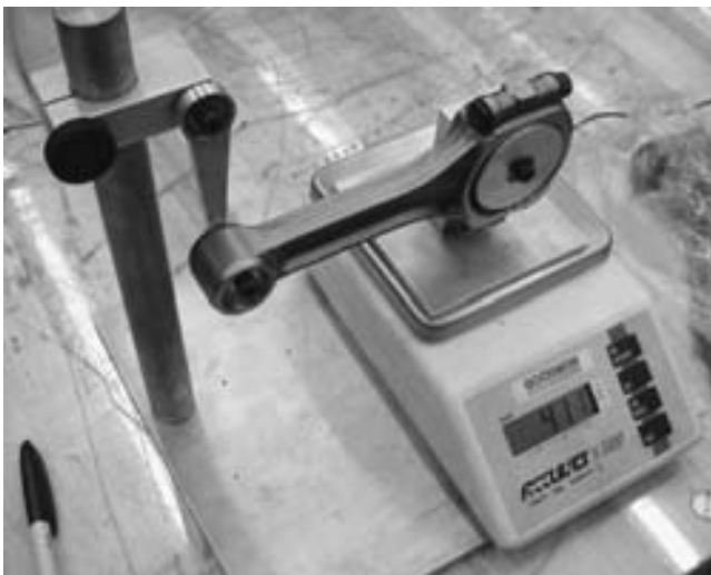
FIGURE 28-5 Weighing the big end of a connecting rod on a scale that keeps it perfectly horizontal so that each end can be weighed separately.
