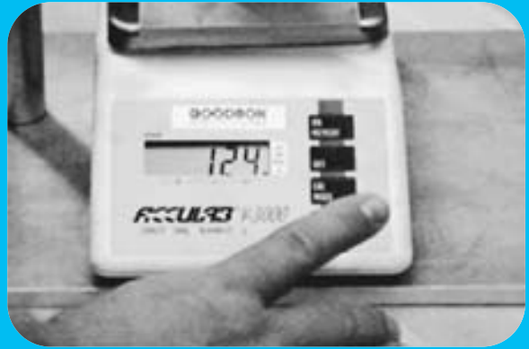
STEP 8 Set the scale to zero, which disregards the weight of the holding fixture. The weight of the holding fixture is called the tare weight.
