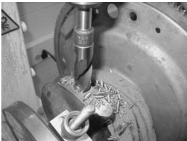
FIGURE 28-9 A drill is usually used to remove weight from the crankshaft to achieve proper balance.
