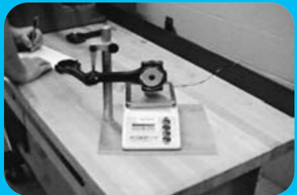
STEP 10 Record all weights from all connecting rods to be used in the engine. Compare the readings and determine where weight must be removed to make all rods weigh the same as the lightest rod in the set.
