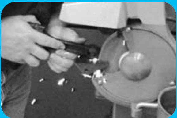
STEP 11 Use a grinder to remove material from the small-end or big-end balancing pad to achieve the proper weight.
