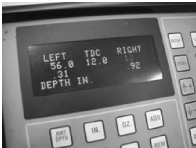
FIGURE 28-8 The display of a crankshaft balancer showing where weight needs to be removed to achieve a balanced assembly.
