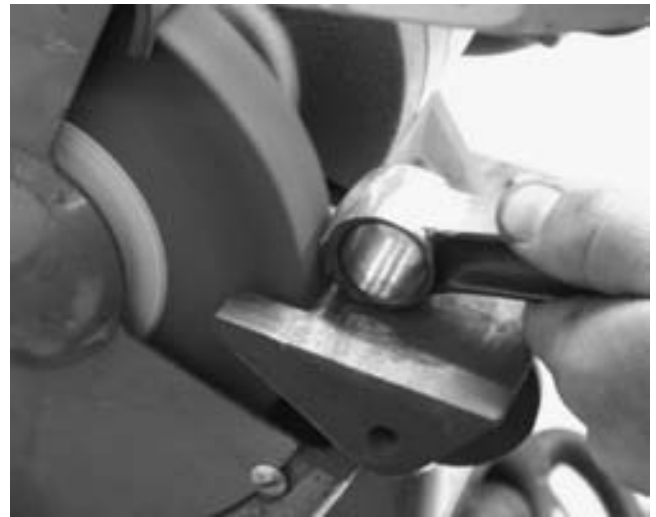
FIGURE 28-6 Removing material from the balancing pad on the small end of the rod to match it to the weight of the small end of the lightest rod being used in the engine.
