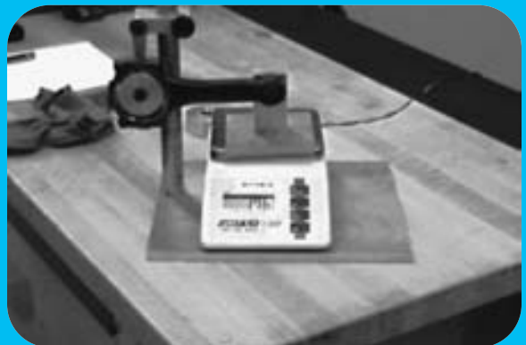
STEP 12 Remeasure the weight of the rod after grinding.
