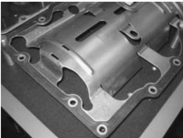
FIGURE 29-10 An oil pan gasket assembly which includes the windage tray is an aftermarket part that can be used to simplify assembly.
