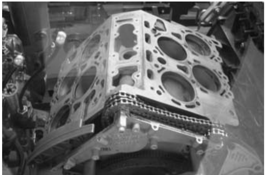
FIGURE 29-1 A uniquely designed W-8 engine installed in some Audi and Volkswagen vehicles. Rebuilding the engine would require detailed service information to be sure that all steps are taken to ensure proper assembly.
