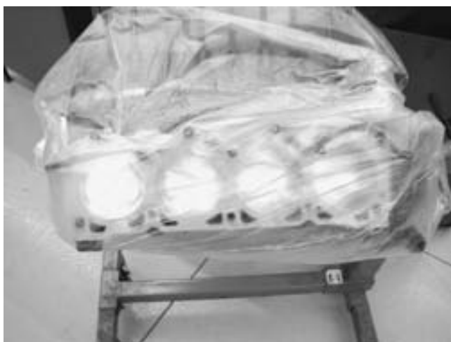
FIGURE 29-8 Placing a plastic trash bag over the engine and tying it shut is an excellent way to keep the engine clean.
