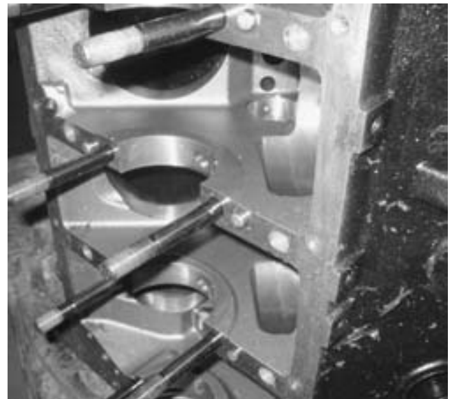
FIGURE 29-3 Main bearing studs installed on a V-8 block.
