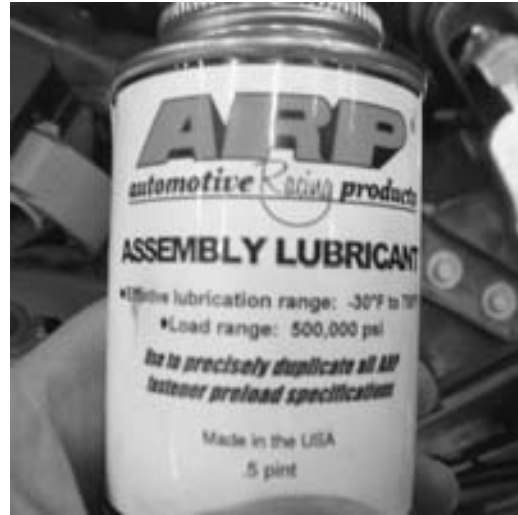
FIGURE 29-11 Special lubricant is specified when using ARP fasteners. This lubricant reduces the friction of the threads and therefore a lower-than-factory-specified torque specification is mandated when using the special lubricant.
