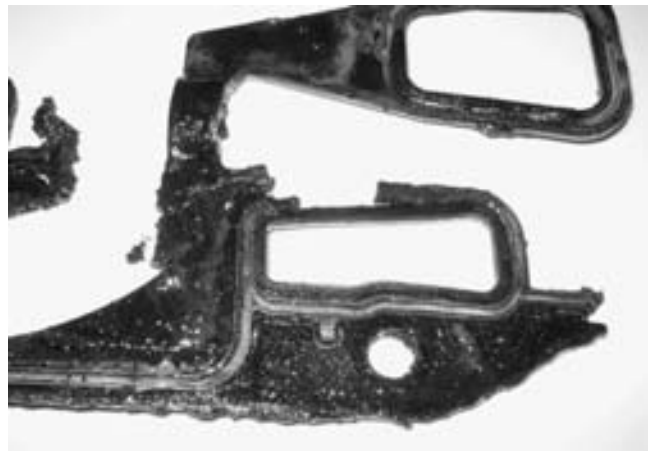
FIGURE 29-12 This intake manifold gasket was damaged due to fretting. Newer designs allow for more movement between the intake manifold and the cylinder head.
