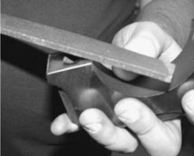
FIGURE 29-2 Deburring all sharp edges is an important step that has to be done to achieve proper engine assembly.
