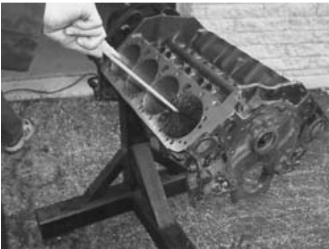
FIGURE 30-1 The best way to clean cylinders is to use soap (detergent) and water and thoroughly clean using a large washing brush. This method floats the machining particles out of the block and washes them away.
