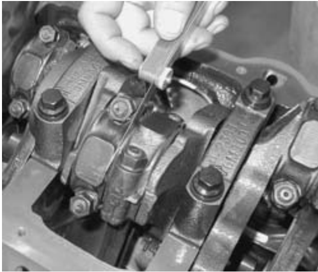
FIGURE 30-32 The connecting rod side clearance is measured with a feeler gauge.
