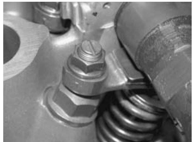
FIGURE 30-50 Most adjustable valves use a nut to keep the adjustment from changing, so to adjust the valves the nut has to be loosened and the screw rotated until the proper valve clearance is achieved. Then the screw should be held while tightening the lock nut to keep the adjustment from changing. Double-check the valve clearance after tightening the nut.
