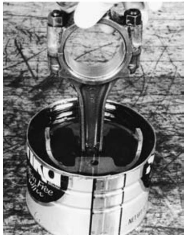
FIGURE 30-25 Dipping the piston, with rings installed, into a container of engine oil is one method that can be used to ensure proper lubrication of pistons during installation in the engine cylinder. This method also ensures that the piston pin will be well lubricated.
