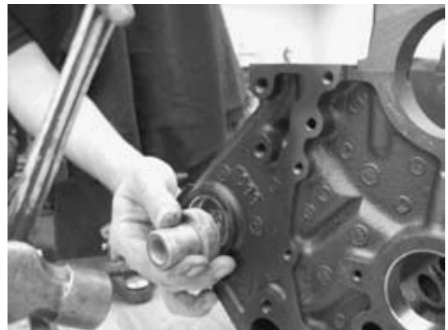
FIGURE 30-6 Sealer should be used on the cup plug before being driven into the block.
