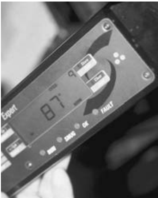
FIGURE 30-46 An electronic torque wrench showing the number of degrees of rotation. These very accurate and expensive torque wrenches can be programmed to display torque or number of degrees of rotation.
