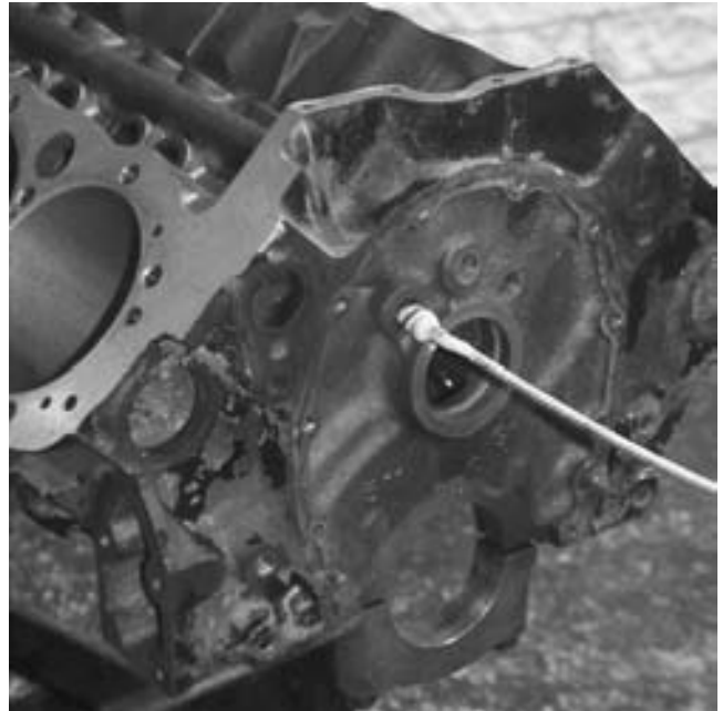
FIGURE 30-2 All oil galleries should be cleaned using soap (detergent) and water using a long oil gallery cleaning brush.
