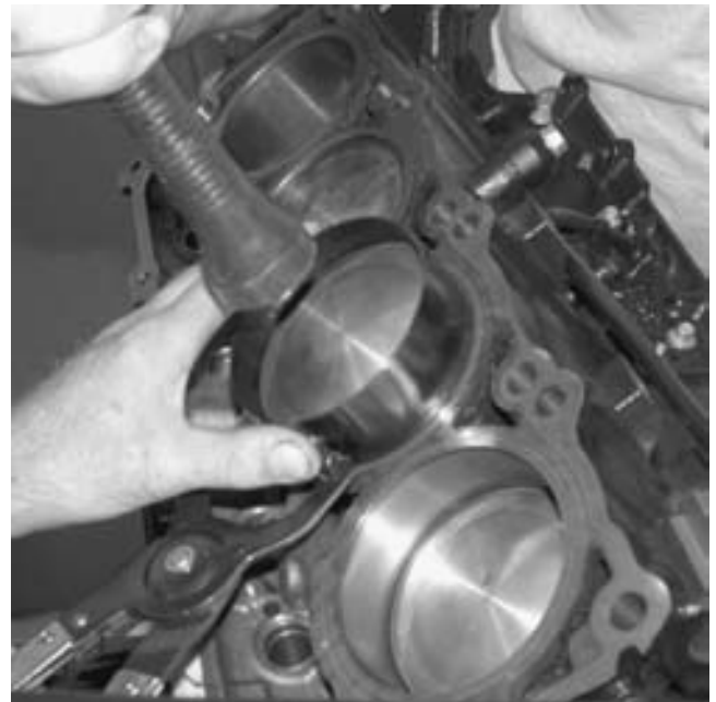
FIGURE 30-30 Installing a piston using a ring compressor to hold the rings in the ring grooves of the piston and then using a hammer handle to drive the piston into the bore. Connecting rod bolt protectors have been installed to help prevent possible damage to the crankshafts during piston installation.
