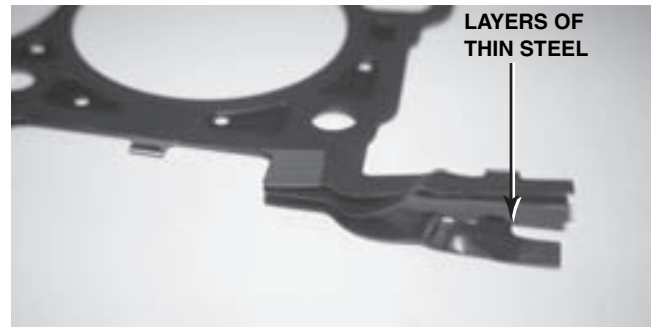
FIGURE 30-39 Multilayer steel (MLS) gaskets are used on many newer all-aluminum engines as well as engines that use a cast block with aluminum cylinder heads. This type of gasket allows the aluminum to expand without losing the sealing ability of the gasket.
