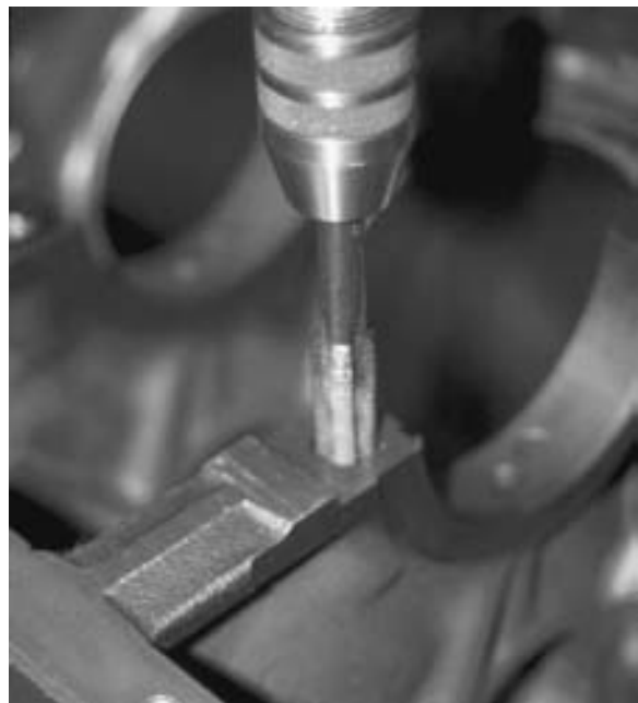
FIGURE 30-3 All threaded holes should be cleaned using a thread chaser or a bottoming tap.
