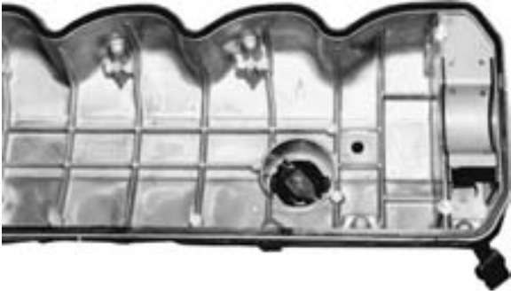
FIGURE 30-55 Typical cast-aluminum cam (valve) cover. Note the rubber gasket in the cast groove of the cover.
