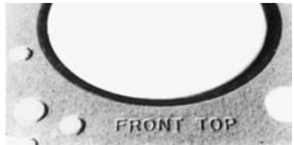
FIGURE 30-40 Typical head gasket markings.
