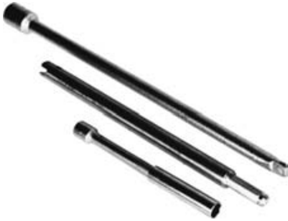
FIGURE 30-59 Drivers used to rotate oil pumps to prelubricate all parts of the engine before installing the distributor and starting the engine.
