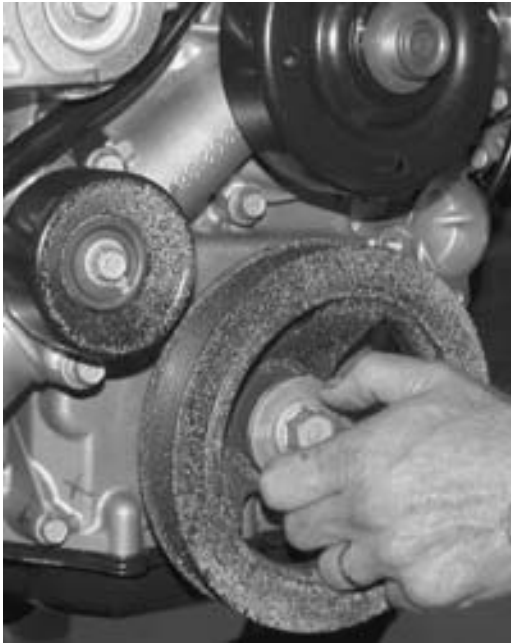
FIGURE 30-57 Installing the harmonic balancer. Always follow the manufacturer's recommended procedure and torque specifications.
