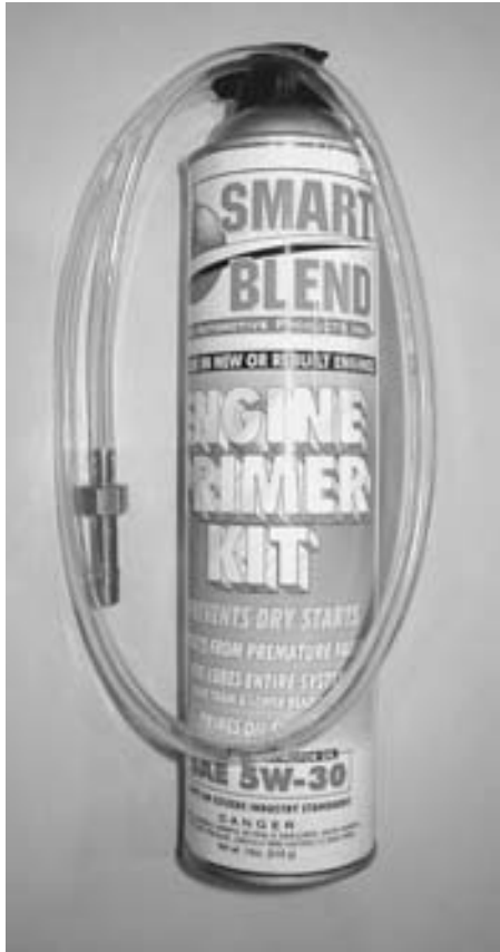
FIGURE 30-60 The engine can be pressurized with engine oil from an aerosol can as shown or from a pressurized oil container designed for preoiling the engine.
