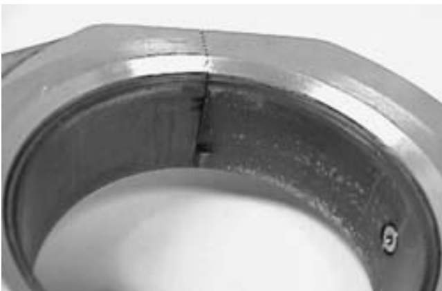
FIGURE 30-23 On V-type engines that use paired rod journals, the side of the rod with the large chamfer should face toward the crank throw (outward).
