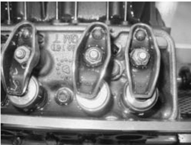
FIGURE 31-1 Prelubricating the engine is a very important step that should be performed before starting the engine. Notice that oil is flowing through the pushrods, over the rocker arms, and onto the valve springs.
