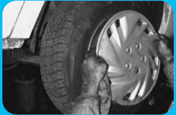
STEP 40 Install the wheel/tire assembly and wheel cover.
