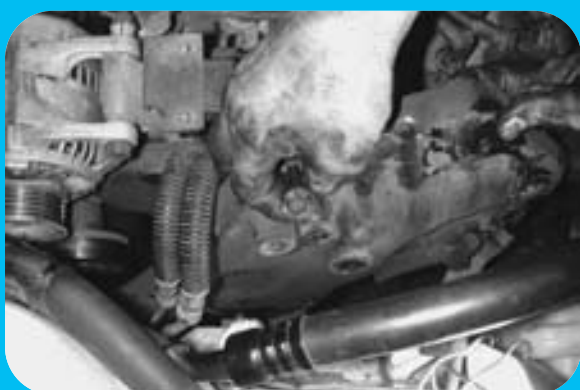
STEP 11 The accessory support plate is removed.
