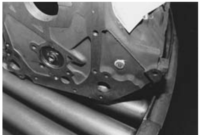
FIGURE 31-5 Most engine rebuilders install a temperature-sensitive device on the engine. These sensors are used by the rebuilders for warranty purposes to record any occurrence of engine overheating. This small disk is glued to the engine block and will pop out if the engine overheats.
