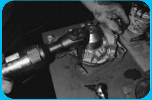
STEP 26 Assembling the new water pump onto the original water pump housing.
