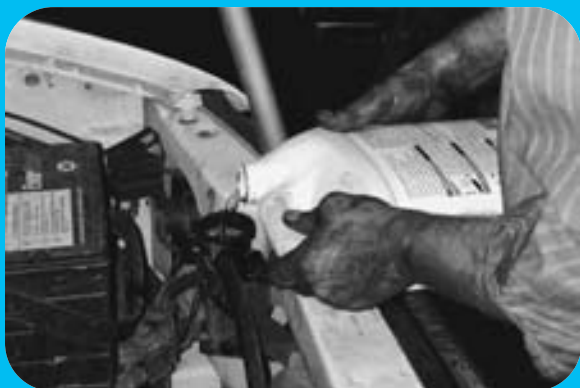
STEP 41 The vehicle is now lowered and the cooling system filled with new coolant.
