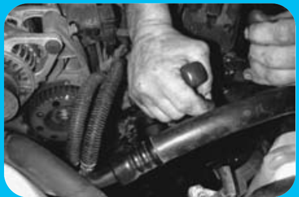
STEP 18 After the water pump retaining bolts have been removed, a screwdriver or pry bar is needed to remove the water pump. (continued)
