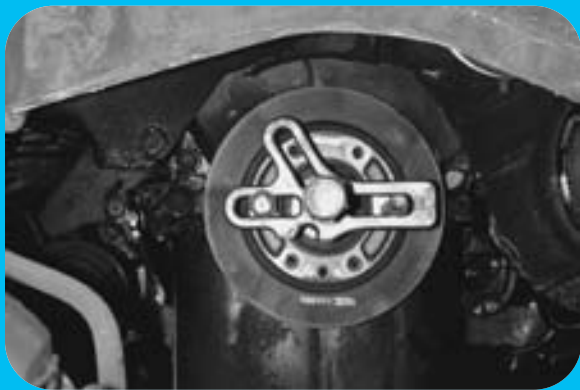
STEP 7 A puller is used to remove the harmonic balancer.
