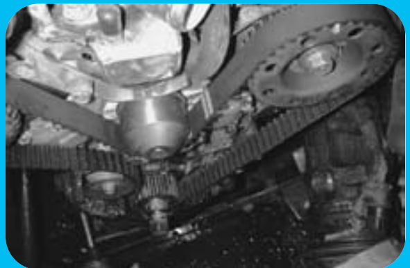
STEP 30 After the water pump is installed, the new timing belt can be installed.
