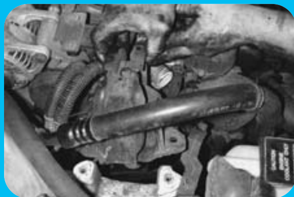
STEP 10 With the engine supported from underneath, the upper engine mount is removed.
