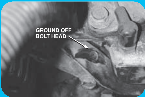
STEP 17 With the bolt head removed, the bracket is lifted up slightly, allowing room to remove the water pump. The bracket is still retained by another bolt.
