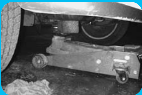
STEP 9 Before removing the upper engine mount, the engine is being supported by a floor jack. Notice that a block of wood is placed between the oil pan and the jack.
