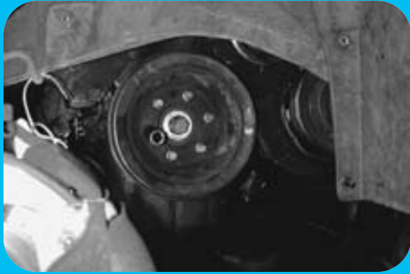
STEP 37 The accessory drive pulley is then installed on the harmonic balancer and the bolts torqued to factory specifications.
