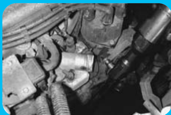
STEP 12 The timing belt cover(s) can now be removed.
