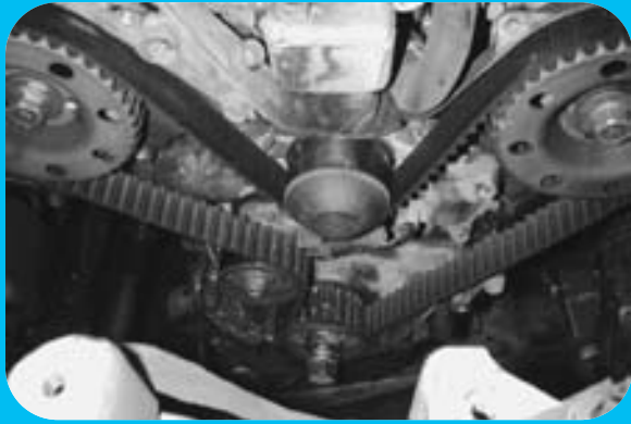
STEP 13 A view of the front of the engine with the timing belt covers removed.
