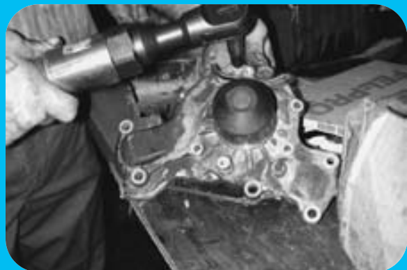
STEP 22 After removing the Phillips screw on the backside, turn the water pump over and remove the rest of the retaining bolts.
