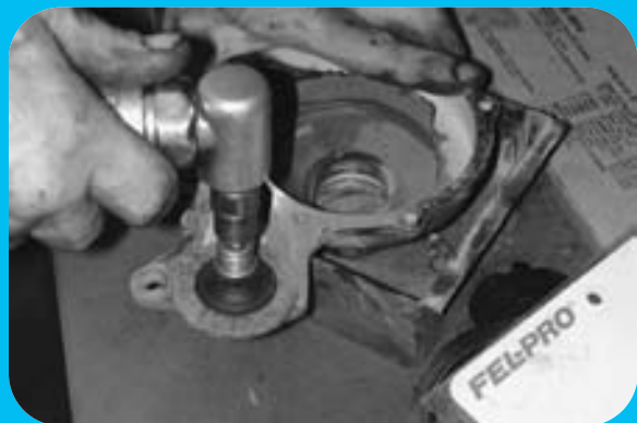
STEP 24 A fiber disc on an air grinder is being used to remove the old gasket material.
