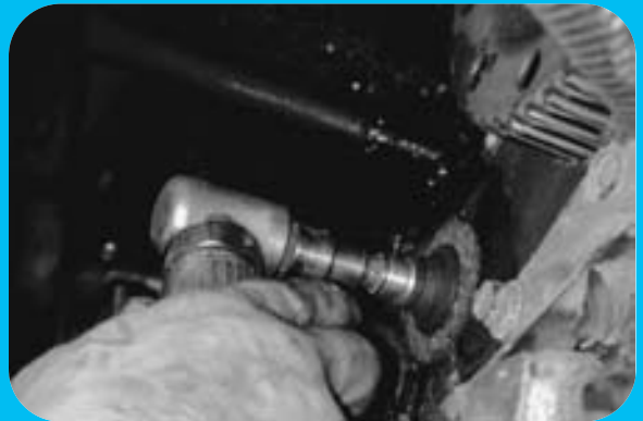
STEP 28 Before installing the water pump, the block has to be cleaned of the old gaskets.
