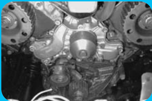
STEP 29 A view of the front of the engine with the replacement water pump installed.
