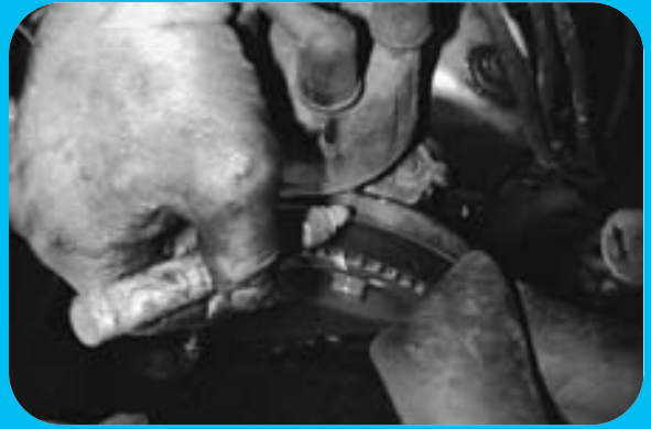
STEP 14 Before removing the timing belt, the wise service technician marks the location of the belt and pulley as a precaution to be sure that the new replacement belt will be placed back into proper time.
