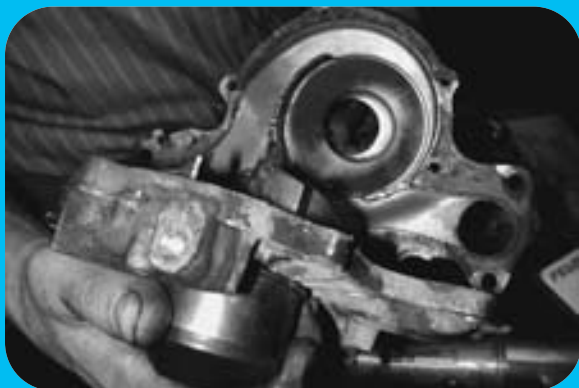
STEP 23 After all retaining bolts have been removed, separate the water pump from the housing.
