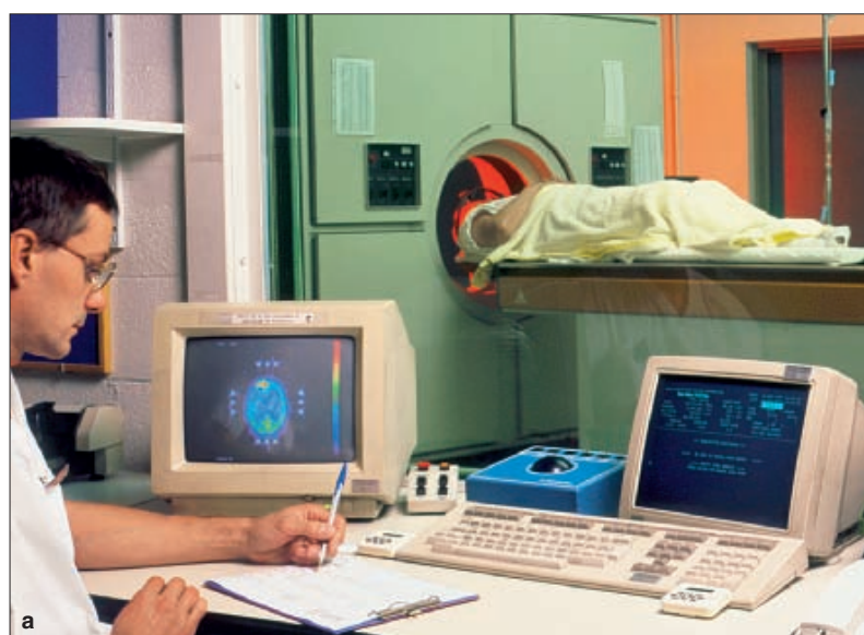
portion of the patient's body being scanned detector ring inside the PET scanner
