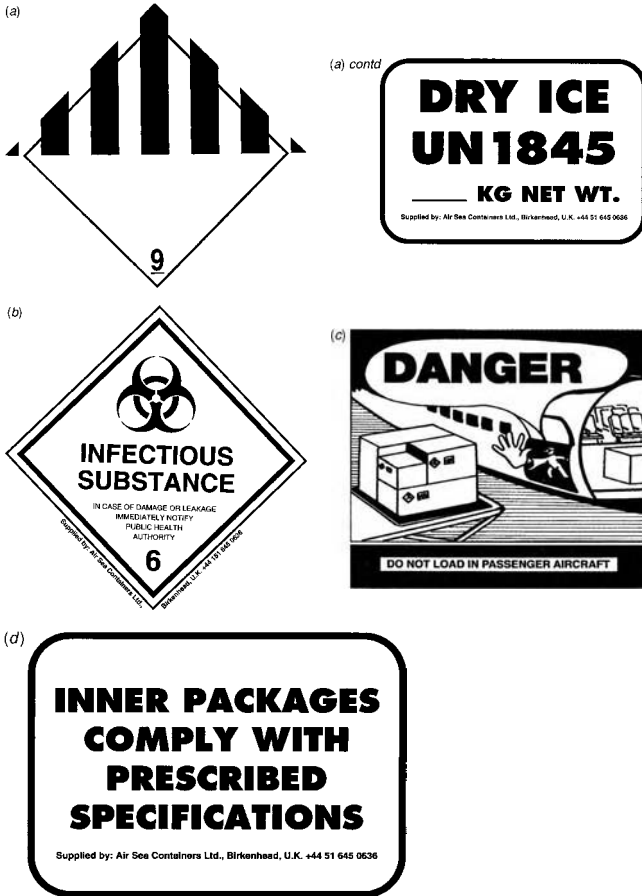
Fig. 14.2. Examples of labels used for mailing of hazardous substances (a) dry ice (b) infectious substance (c) > 50 g or 50 ml of material (d) inner package label.
