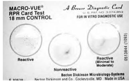
Fig. 7.5. Non-treponemal rapid plasma reagin (RPR) assay to screen for syphilis. The RPR is a standardized flocculation and co-agglutination assay used for serologic detection of T. pallidum infection. Patient's serum is mixed with a charcoal suspension containing cardiolipin antigen. The cardiolipin antigen reacts with 'reagin', an antibody-like substance present in the serum of syphilis patients, to produce a flocculation reaction and co-agglutinate the carbon particles in the assay. This Figure demonstrates typical reactive, minimally reactive (both considered as positive) and non-reactive (negative) results. This non-treponemal test is used to screen for syphilis, but must be confirmed using a treponemal assay (see Fig. 7.6).
