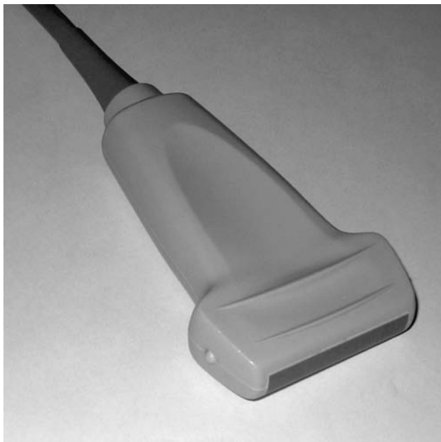
Figure 12.5 A high frequency linear probe
