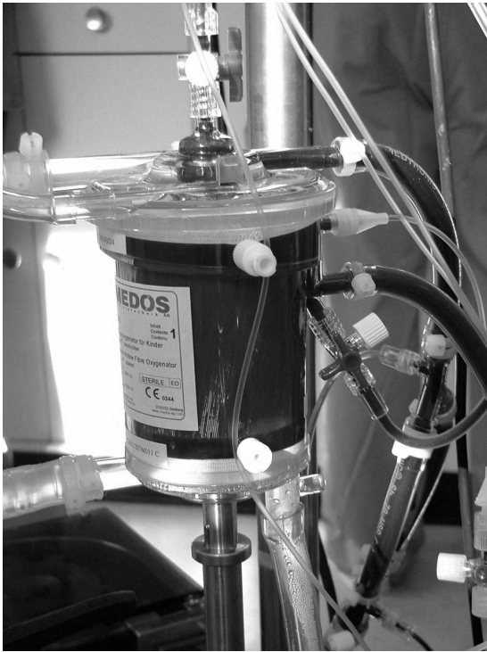
Figure 26.2 Modern Medos™ 2400 coated hollow fiber oxygenator, suitable for infants from 2–10 kg in weight.
