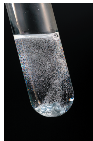
FIG. 5.3 Zinc reacts with hydrochloric acid. Bubbles of hydrogen are formed when a solution of hydrochloric acid comes in contact with metallic zinc. The same reaction takes place if hydrochloric acid is spilled on galvanized (zinc coated) steel. (Andy Washmik.)
