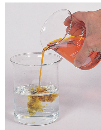
FIG. 5.2 A redox reaction taking place in an acidic solution. A solution of \text{K}_2\text{Cr}_2\text{O}_7 oxidizes \text{Fe}^{2+} to \text{Fe}^{3+} in an acidic solution. At the same time, the orange dichromate ion is reduced to \text{Cr}^{3+} . (Peter Lerman.)
