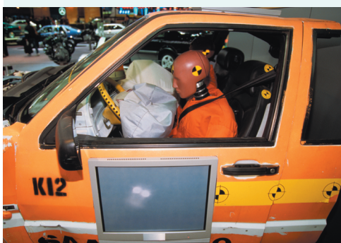
The explosive decomposition of sodium azide releases nitrogen gas, which rapidly inflates an air bag during a crash. (Corbis-Bettmann.)
