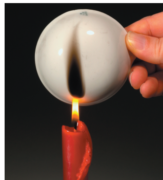
FIG. 5.10 Incomplete combustion of a hydrocarbon. The bright yellow color of a candle flame is caused by glowing particles of elemental carbon. Here we see that a black deposit of carbon is formed when the flame contacts a cold porcelain surface. (Andy Washnik.)
