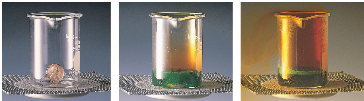
FIG. 5.4 The reaction of copper with concentrated nitric acid. A copper penny reacts vigorously with concentrated nitric acid, as this sequence of photographs shows. The dark red brown vapors are nitrogen dioxide, the same gas that gives smog its characteristic color. (Michael Watson.)
