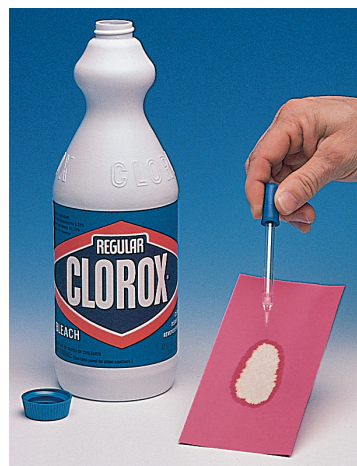
FIG. 5.1 “Chlorine” bleach. This common household product is a dilute aqueous solution of sodium hypochlorite, NaOCl, which destroys fabric stains by oxidizing them to colorless products. (OPC, Inc.)
