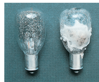
FIG. 5.11 A flashbulb, before and after firing. Fine magnesium wire in an atmosphere of oxygen fills the flashbulb at the left. After being used ( right ), the interior of the bulb is coated with a white film of magnesium oxide. (Robert Capecce.)
