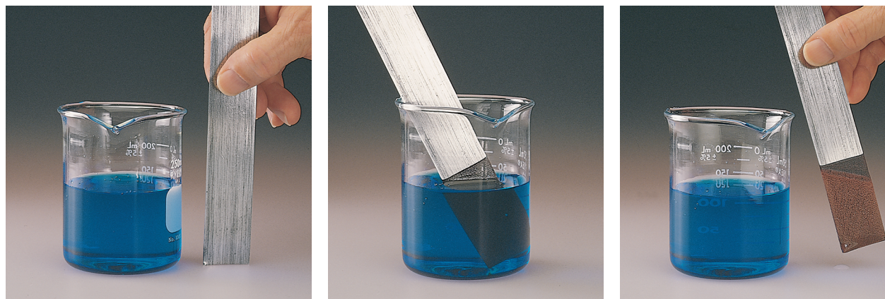
FIG. 5.5 The reaction of zinc with copper ion. ( Left ) A piece of shiny zinc next to a beaker containing a copper sulfate solution. ( Center ) When the zinc is placed in the solution, copper ions are reduced to the free metal while the zinc dissolves. ( Right ) After a while the zinc becomes coated with a red-brown layer of copper. Notice that the solution is a lighter blue than before, showing that some of the copper ions have left the solution. ( Michael Watson. )
