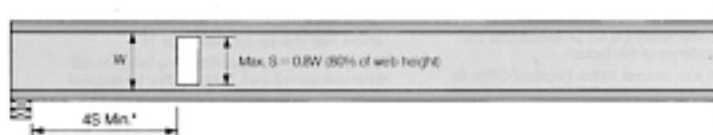
Figure 4. Vertical rectangular hole maximum size and minimum spacing.
