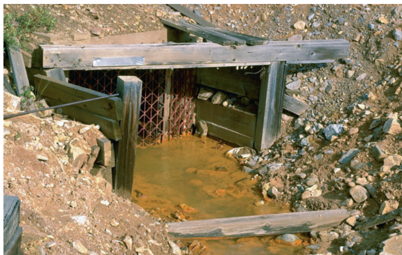
FIGURE 6.12 This water seeping from an abandoned mine in Colorado is an example of acid mine drainage . Acid mine drainage is water with a high concentration of sulfuric acid ( \text{H}_2\text{SO}_4 ) produced by the oxidation of sulfide minerals such as pyrite. When such acid-rich water migrates from its source, it may pollute surface waters and groundwater and cause significant ecological damage. (Photo by Tim Haske/Profiles West/Index Stock Photography, Inc.)
