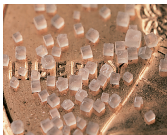
These tiny NaCl crystals (on a penny) show the cubic structure illustrated in Figure 11.5.
