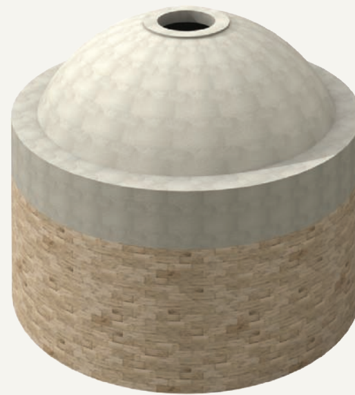
Hemispherical dome with oculus
