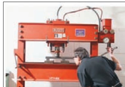
Figure 8-19 Pressure being applied to straighten shaft.
