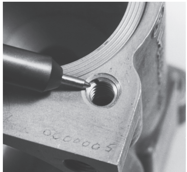
Figure A-36 Stainless steel thread insert used in an aluminium valve housing.
