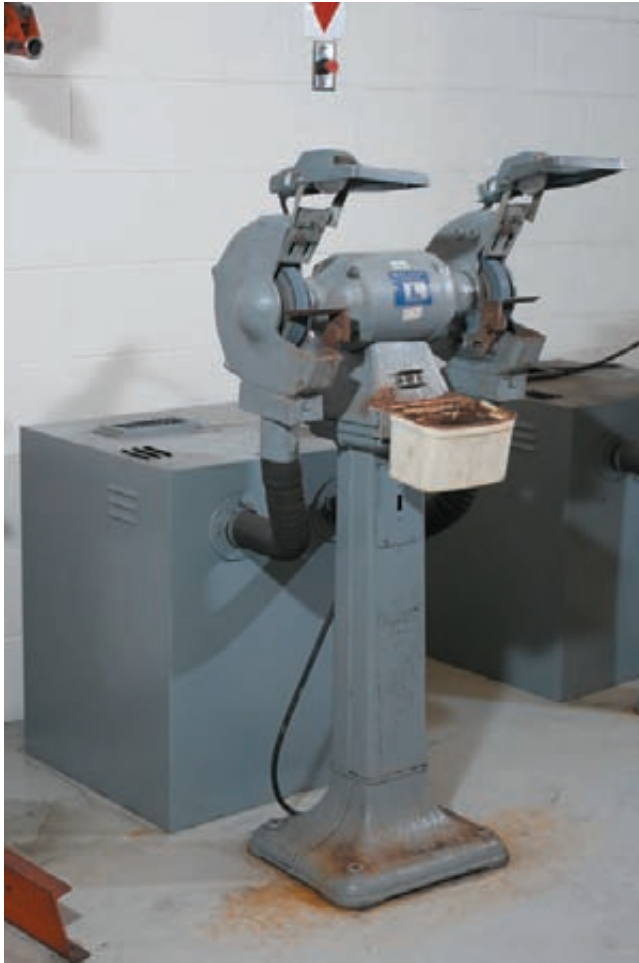
Figure A-5 Vacuum dust collector on grinders.
