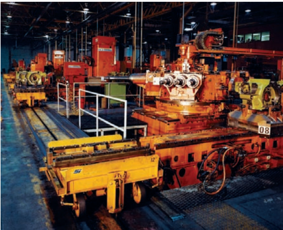
Figure A-4 Parts to be machined are mounted on pallets so that they may be moved from machining center to machining center in different work cells in the flexible manufacturing system (Courtesy of Giddings & Lewis Machine Tools, LLC).
