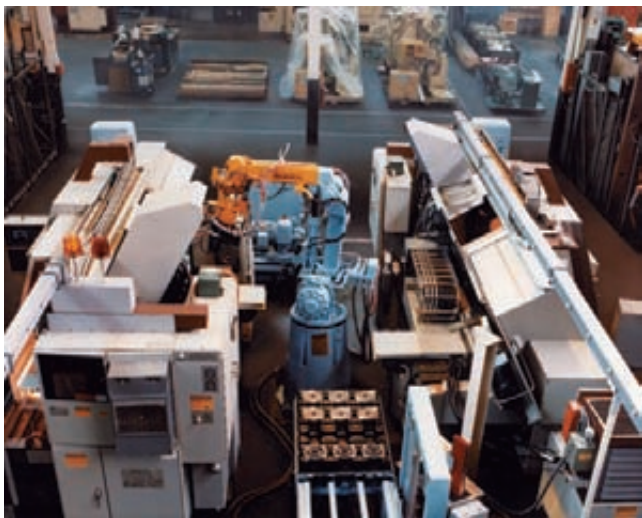
Figure A-1 The machine operator of tomorrow's automated manufacturing industry. A computer-controlled industrial robot loads and unloads parts on a CNC turning center (Courtesy of MAG Industrial Automation Systems LLC).
