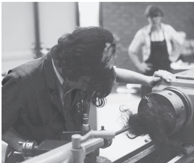
Figure A-10 Long hair may be caught and reeled into the machine.
