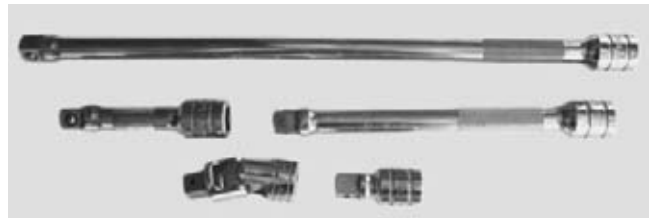
FIGURE 1-18 Various socket extensions. The universal joint (U-joint) (upper left) is useful for gaining access in tight areas.
