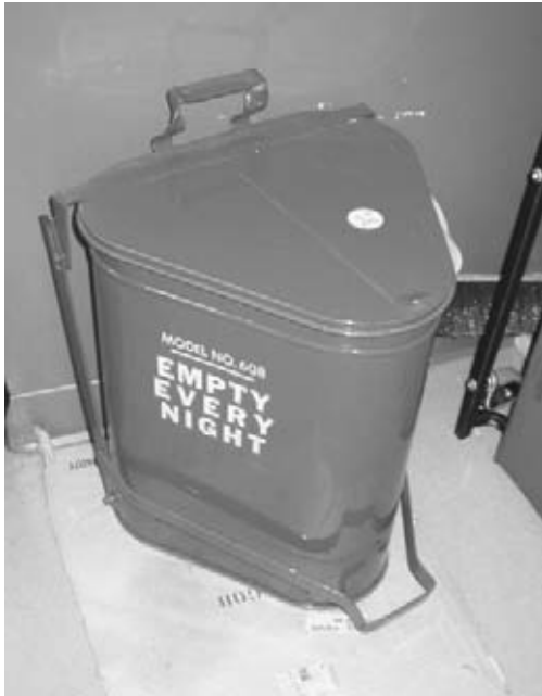
FIGURE 1-37 All oily shop cloths should be stored in a metal container equipped with a lid to help prevent spontaneous combustion. (Courtesy of James Halderman)
