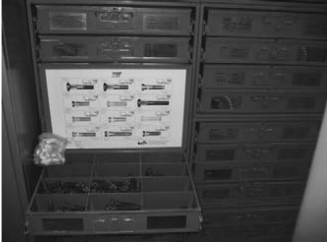
FIGURE 1-13 Every shop should have an assortment of high-quality bolts and nuts to replace those damaged during vehicle service procedures.
