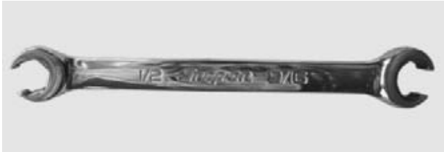
FIGURE 1-21 Flare-nut wrench. Also known as a line wrench , fitting wrench , or tube-nut wrench . This style of wrench is designed to grasp most of the flats of a six-sided (hex) tubing fitting to provide the most grip without damage to the fitting.
