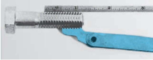
FIGURE 1-9 Thread pitch gauge used to measure the pitch of the thread. This is a 1/2-in. diameter bolt with 13 threads to the inch (1/2–13). (Courtesy of James Halderman)
