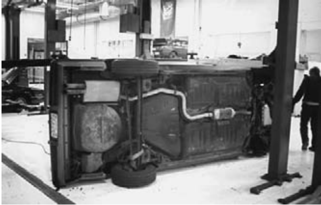
FIGURE 1-39 This vehicle fell from the hoist because the pads were not set correctly. No one was hurt, but the vehicle was a total loss. (Courtesy of James Halderman)
