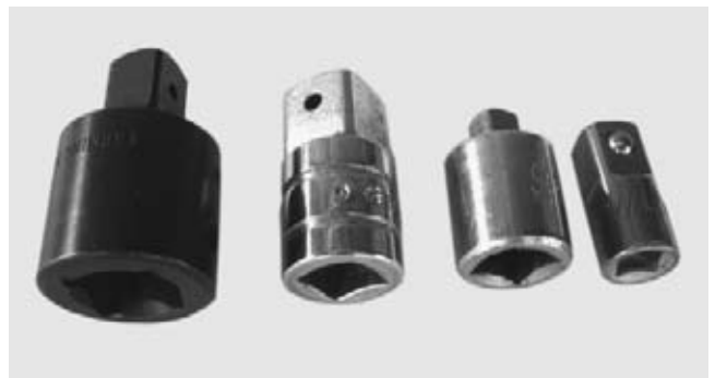
FIGURE 1-19 Socket drive adapters. These adapters permit the use of a 3/8-in. drive ratchet with 1/2-in. drive sockets, or other combinations as the various adapters permit. Adapters should be used carefully where a larger tool could break or damage a smaller-sized socket.
