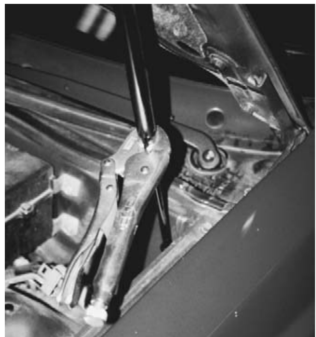
FIGURE 1-36 (a) A crude but effective method to secure a hood is to use locking pliers on the hood strut shaft. Locking pliers should only be used on defective struts because the jaws of the pliers can damage the strut shaft. (b) This commercially available hood clamp has a bright orange tag to help remind the technician to remove the clamp before attempting to close the hood. The hood could be bent if excessive force is used to close the hood with the clamp in place. (Courtesy of James Halderman)
