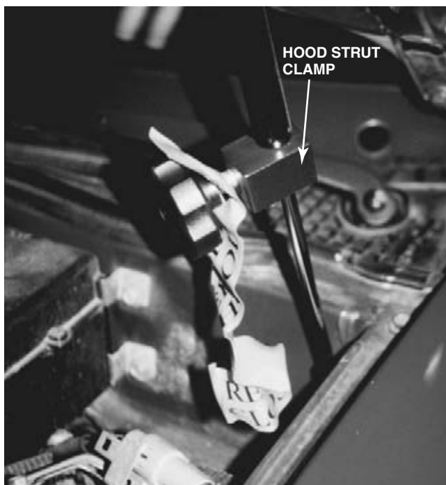
FIGURE 1-36 (a) A crude but effective method to secure a hood is to use locking pliers on the hood strut shaft. Locking pliers should only be used on defective struts because the jaws of the pliers can damage the strut shaft. (b) This commercially available hood clamp has a bright orange tag to help remind the technician to remove the clamp before attempting to close the hood. The hood could be bent if excessive force is used to close the hood with the clamp in place. (Courtesy of James Halderman)
