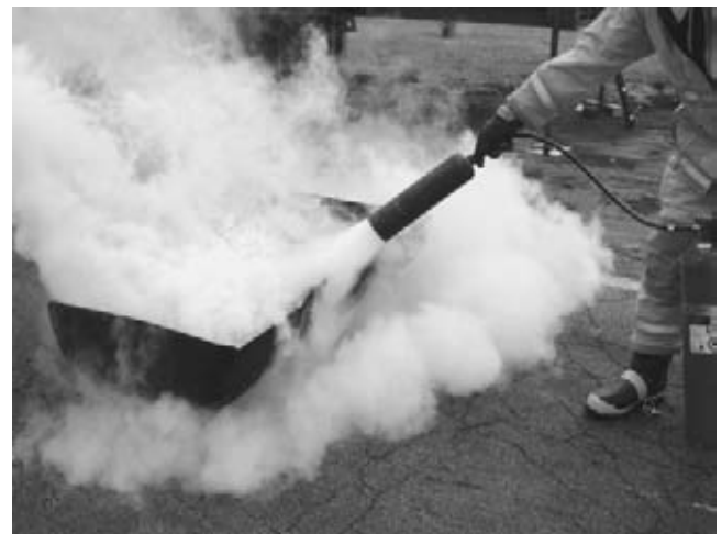
FIGURE 1-44 A CO 2 fire extinguisher being used on a fire set in an open steel drum during a demonstration at a fire department training center. (Courtesy of James Halderman)
