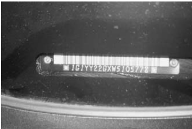
FIGURE 1-1 The vehicle identification number (VIN) is at the top front of the instrument panel and is visible through the windshield. (Courtesy of James Halderman)
