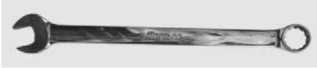
FIGURE 1-20 Combination wrench. The openings are the same size at both ends. Notice the angle of the open end to permit use in close spaces.
