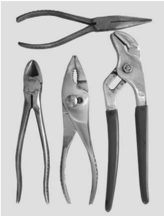
FIGURE 1-22 Assortment of pliers. Slip-joint pliers (center) are often confused with water pump pliers (lower right).
