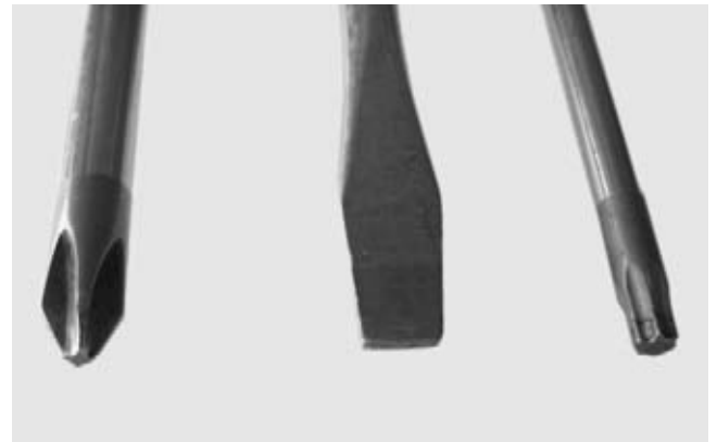
FIGURE 1-24 A flat-blade (or straight-blade) screwdriver (center) is specified by the length of the screwdriver and width of the blade. A Phillips-head screwdriver (left) is specified by the length of the handle and the size of the point at the tip. A Torx screwdriver (right) uses a numerical (#15 or #20) size designation.
