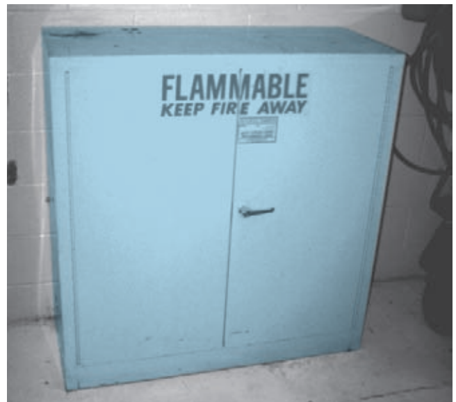
FIGURE 2-4 Typical fireproof flammable storage cabinet. (Courtesy of James Halderman)
