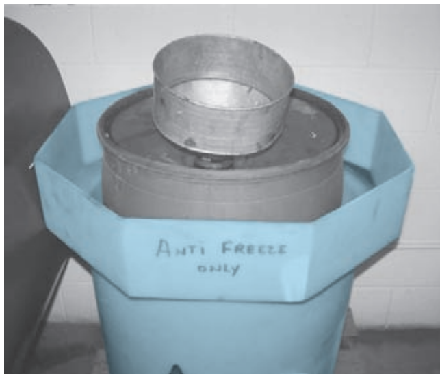
FIGURE 2-6 Used antifreeze coolants should be kept separate and stored in a leak-proof container until it can be recycled or disposed of according to federal, state, and local laws. Note that the storage barrel is placed inside another container to catch any coolant that may spill out of the inside barrel. (Courtesy of James Halderman)
