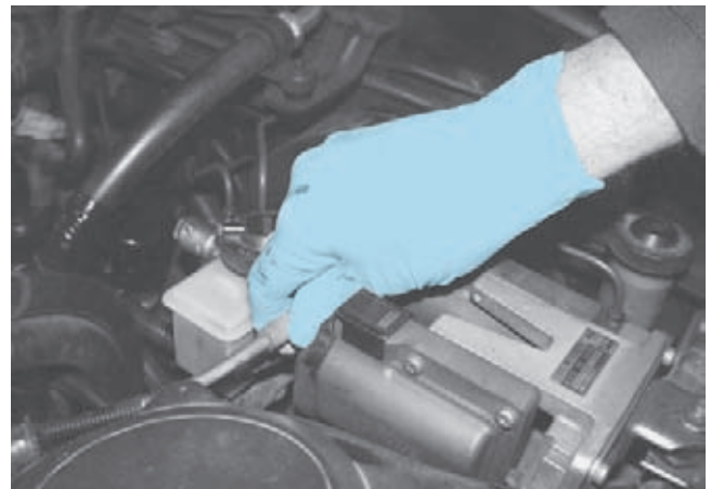
FIGURE 2-3 Protective gloves should be worn whenever working around grease or oil to help prevent possible skin problems. They help keep your hands clean, too! (Courtesy of James Halderman)
