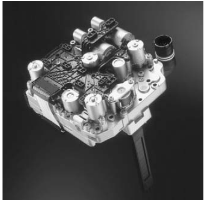
FIGURE 7-17 A dual clutch transaxle uses two clutches to send torque to the gear sets (a). The cutaway view of a DualTronic™ clutch shows the two clutches (b). A DualTronic™ control module (c), a hydraulic valve body with a microprocessor, 11 solenoids, and external electrical connectors. (b and c Courtesy of BorgWarner Inc.)
