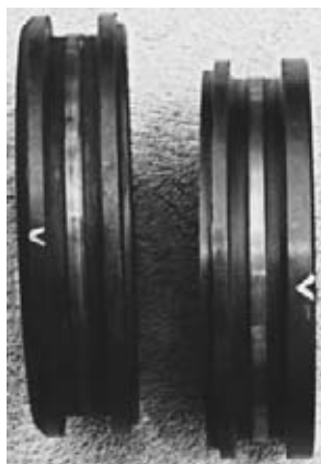
FIGURE 8-58 The technician used a die grinder to place the V-shaped marks on these synchronizer sleeves. They show the front or the position of the particular part.
