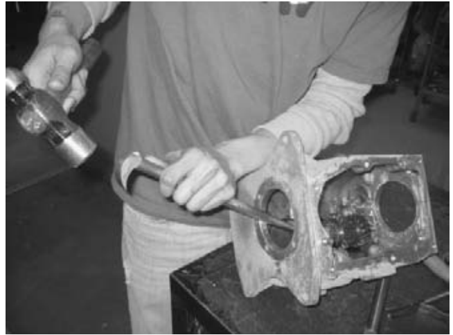
FIGURE 8-44 A recess is provided in the end of this reverse idler gear shaft so that a punch can be used to drive it out of the case.
