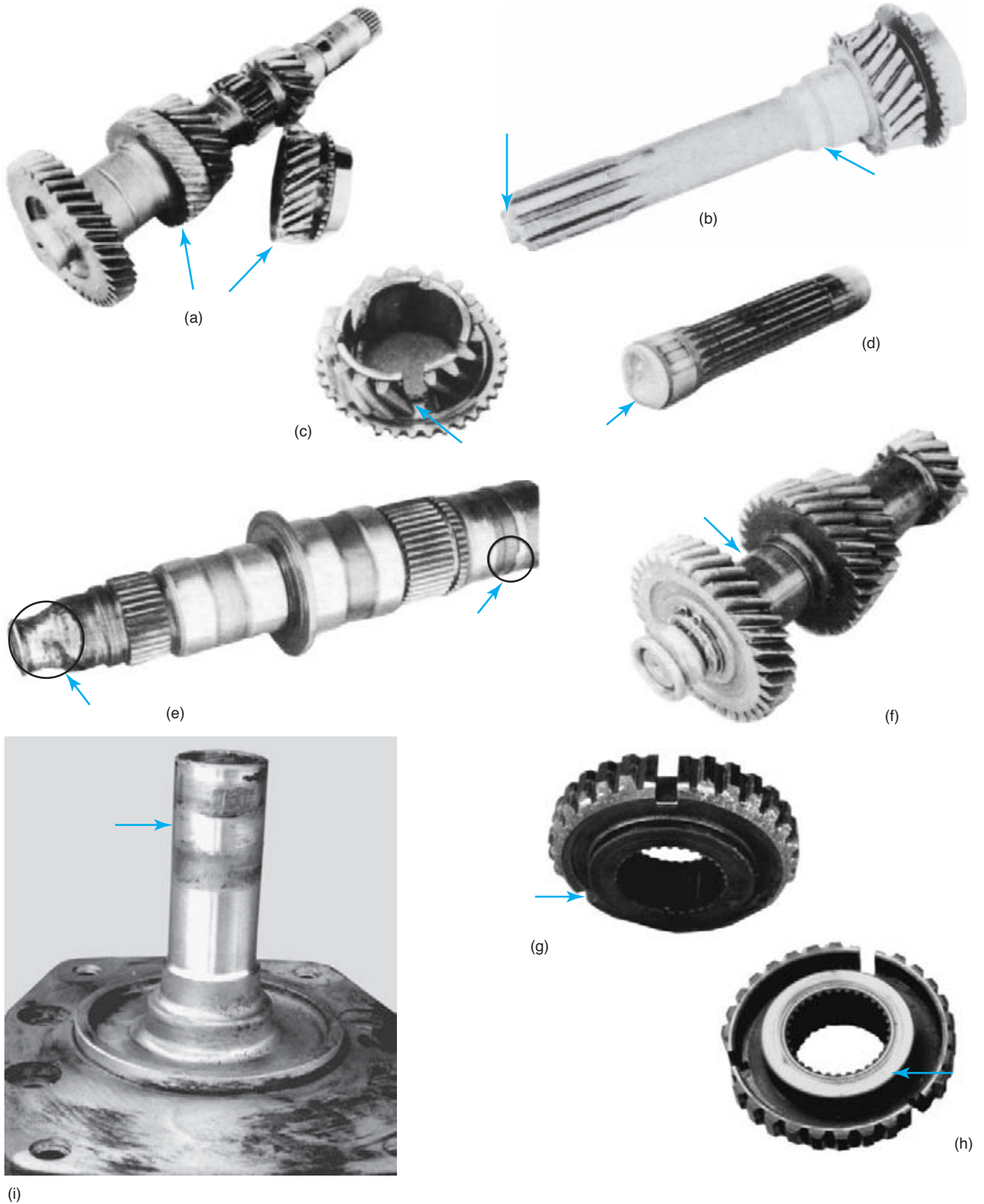
FIGURE 8-48 Some faulty parts, such as the damaged gears (a, b, and c) and broken countershaft (d), are rather obvious; others are also easy to spot, such as the mainshaft (e) or countershaft bearing (f). Some faulty parts, however, look almost normal, like the synchronizer hubs that are broken (g) or have a worn thrust surface (h) or the input bearing retainer that has worn through the hardened surface (i).
