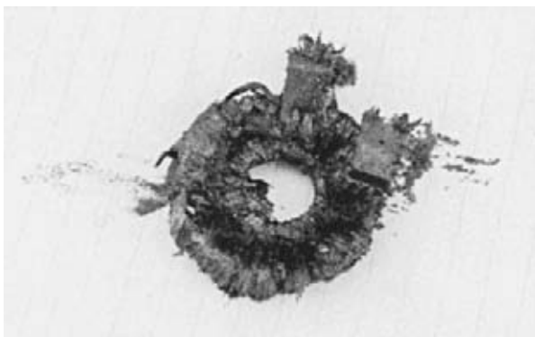
FIGURE 8-46 This case magnet has been removed from a badly worn transmission. Imagine where all this metal came from and the damage that occurred as it passed through the transmission.
