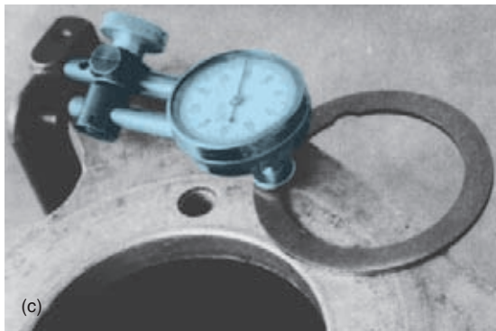
FIGURE 8-93 A selective shim can be measured using an outside micrometer (a) or by setting up a dial indicator to read zero on the case (b) and then sliding the shim under the indicator and reading the size (c).
