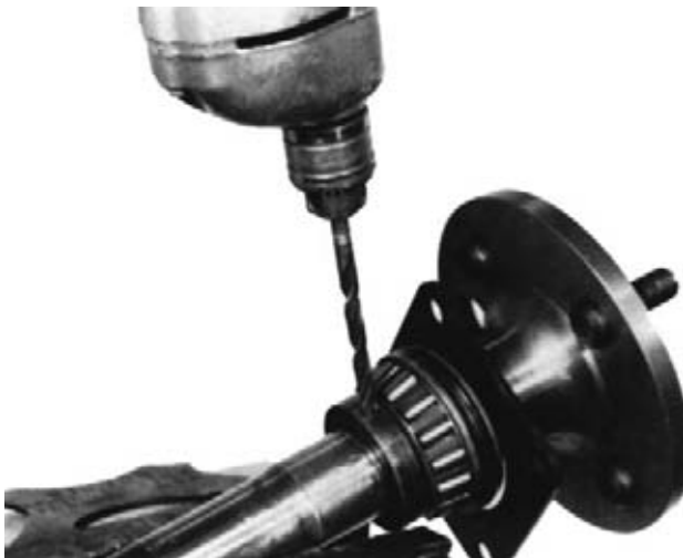
FIGURE 12-37 The axle bearing retainer ring should be cut or stretched using a drill and chisel to make six to eight chisel blows before trying to press the bearing off the axle. (Courtesy of Dana Corporation)
