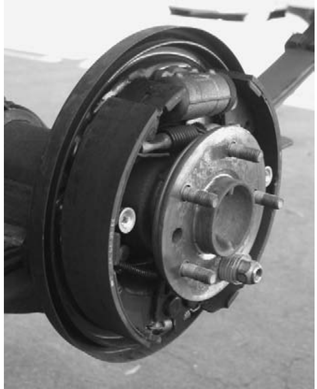
FIGURE 12-44 A new wheel stud is installed by tightening the lug nut against a stack of flat washers.
