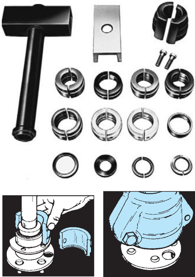
FIGURE 12-38 This tool set encloses the bearing in a collet as it attaches the bearing to the press fixture to allow the safe removal of the bearing. (Courtesy of OTC Tools)
