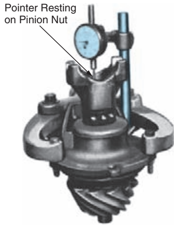
FIGURE 12-74 Drive pinion end play is measured using a dial indicator. (Courtesy of Ford Motor Company)
