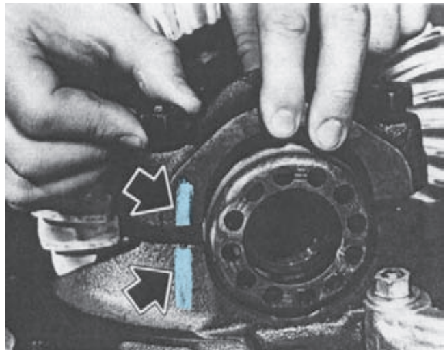
FIGURE 12-78 Start the bearing cap bolts into their threads; the bearing caps should drop into alignment with the threaded adjusters. Be sure to align the bearing cap index marks. (Courtesy of Ford Motor Company)
