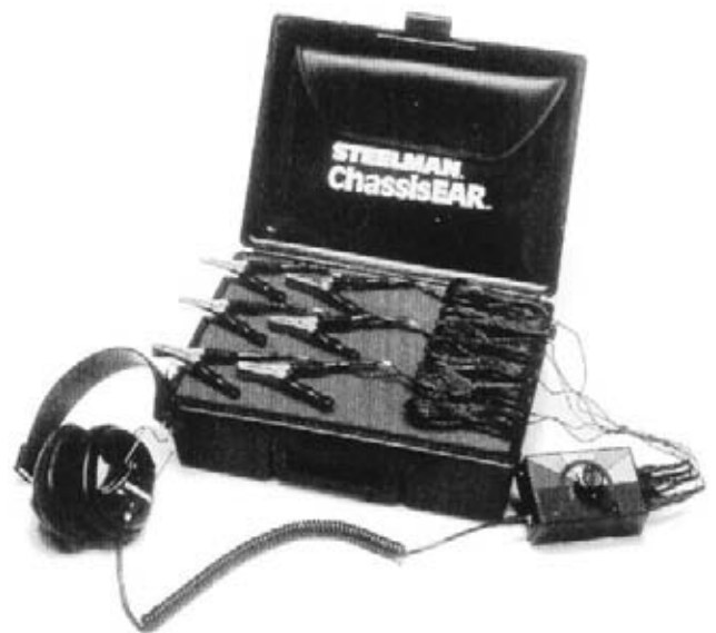
FIGURE 12-5 A Chassis Ear has a microphone attached to each of the six clamps that are connected to various locations under the vehicle. The technician makes a road test while wearing the headset, and turns the selector switch to locate the source of an under-car noise. (Courtesy of Steelman)
