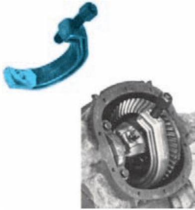
FIGURE 12-19 In some differentials, the pinion shaft lock bolt tends to break during removal. This tool is used to force the differential pinion shaft out, shearing off a broken lock bolt without damaging the differential case. (Courtesy of Borroughs)
