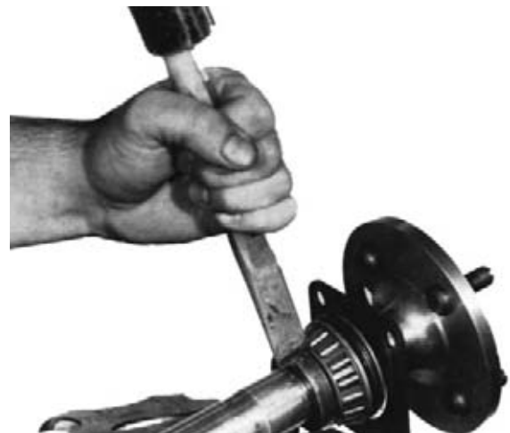
FIGURE 12-37 The axle bearing retainer ring should be cut or stretched using a drill and chisel to make six to eight chisel blows before trying to press the bearing off the axle. (Courtesy of Dana Corporation)
