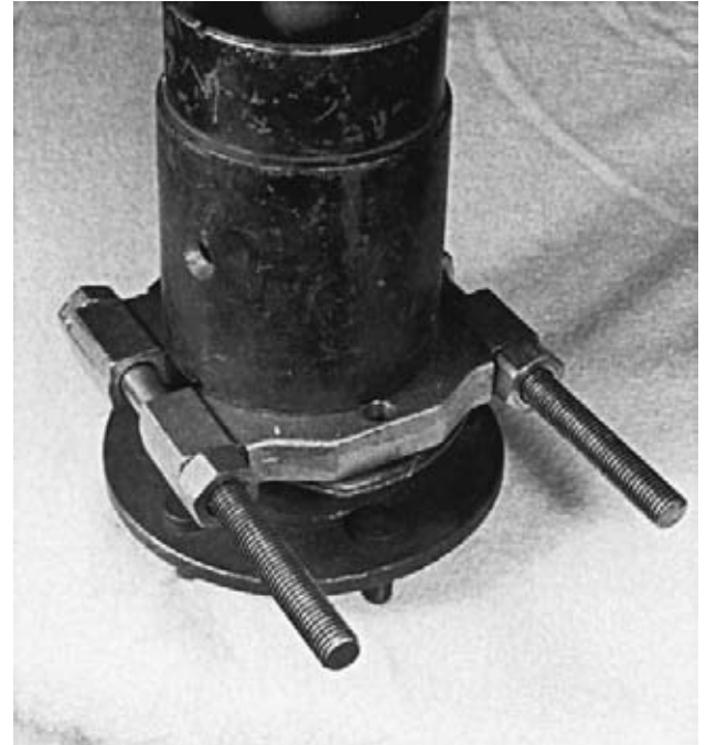
FIGURE 12-36 A bearing could explode as it is being pressed off the axle. An old starter housing can be placed over the bearing as a scatter shield when a bearing separator is used under the bearing. This assembly can be used in a press with relative safety.
