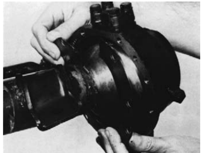
FIGURE 13-29 A closed-end axle encloses the CV joint in a round chamber, keeping it clean and lubricated. (Courtesy of Dana Corporation)
